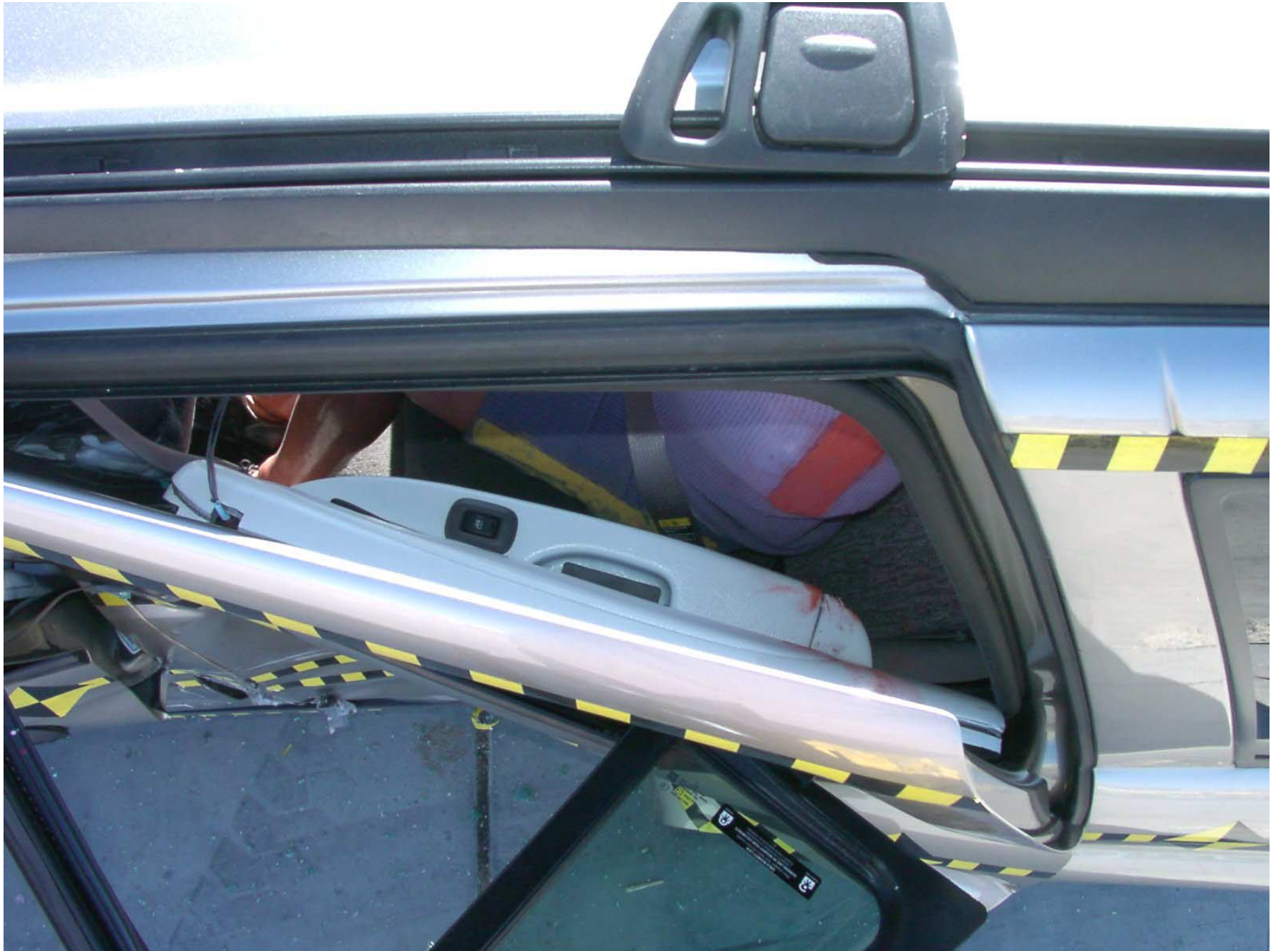
Figure A-35: Passenger Dummy Clearance, Post-Test
