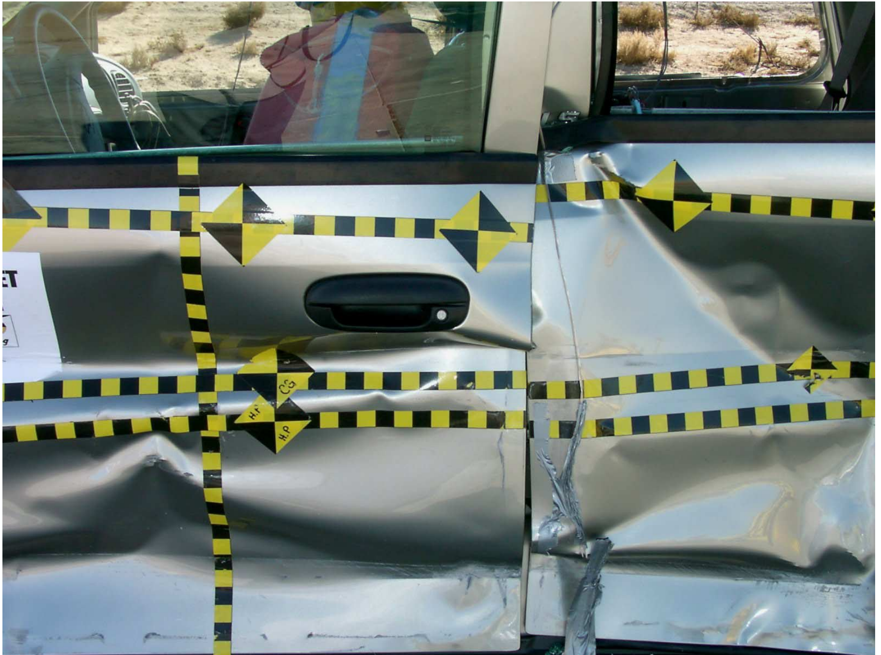
Figure A-19: Left Front Door Closed, Post-Test
