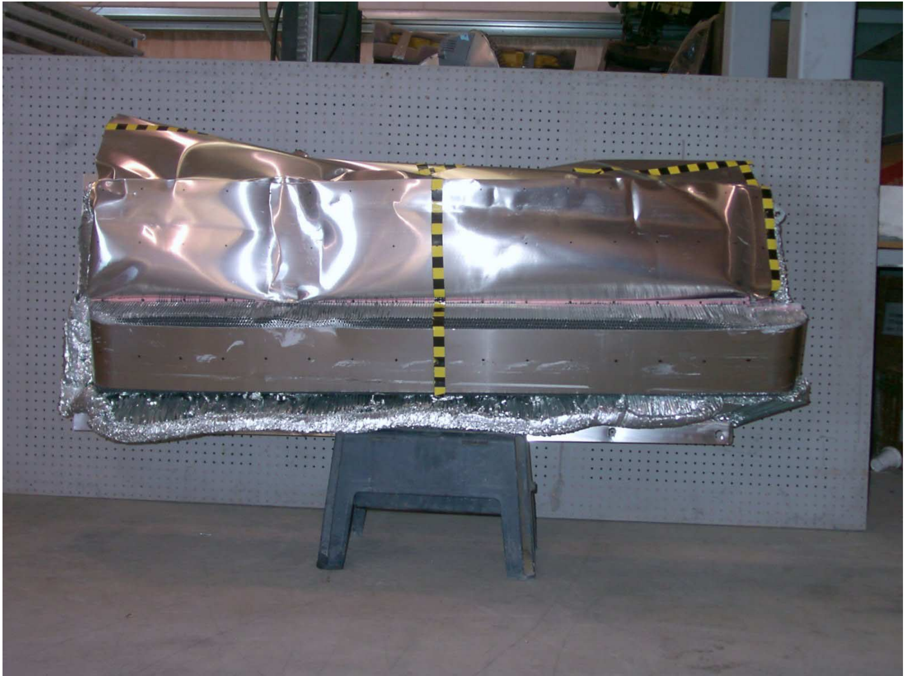
Figure A-41: Front View of Deformable Barrier, Post-Test
