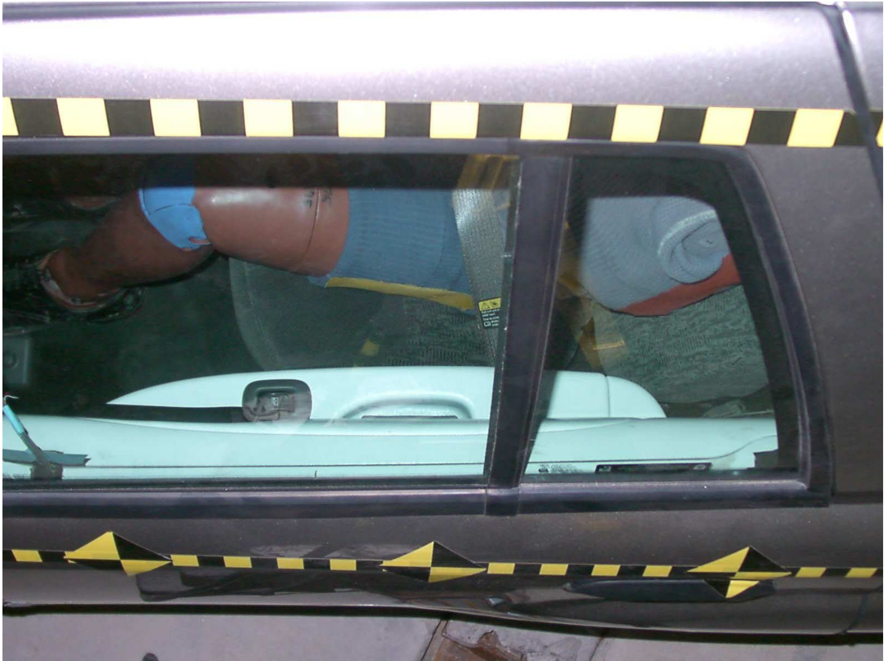
Figure A-34: Passenger Dummy Clearance, Pre-Test
