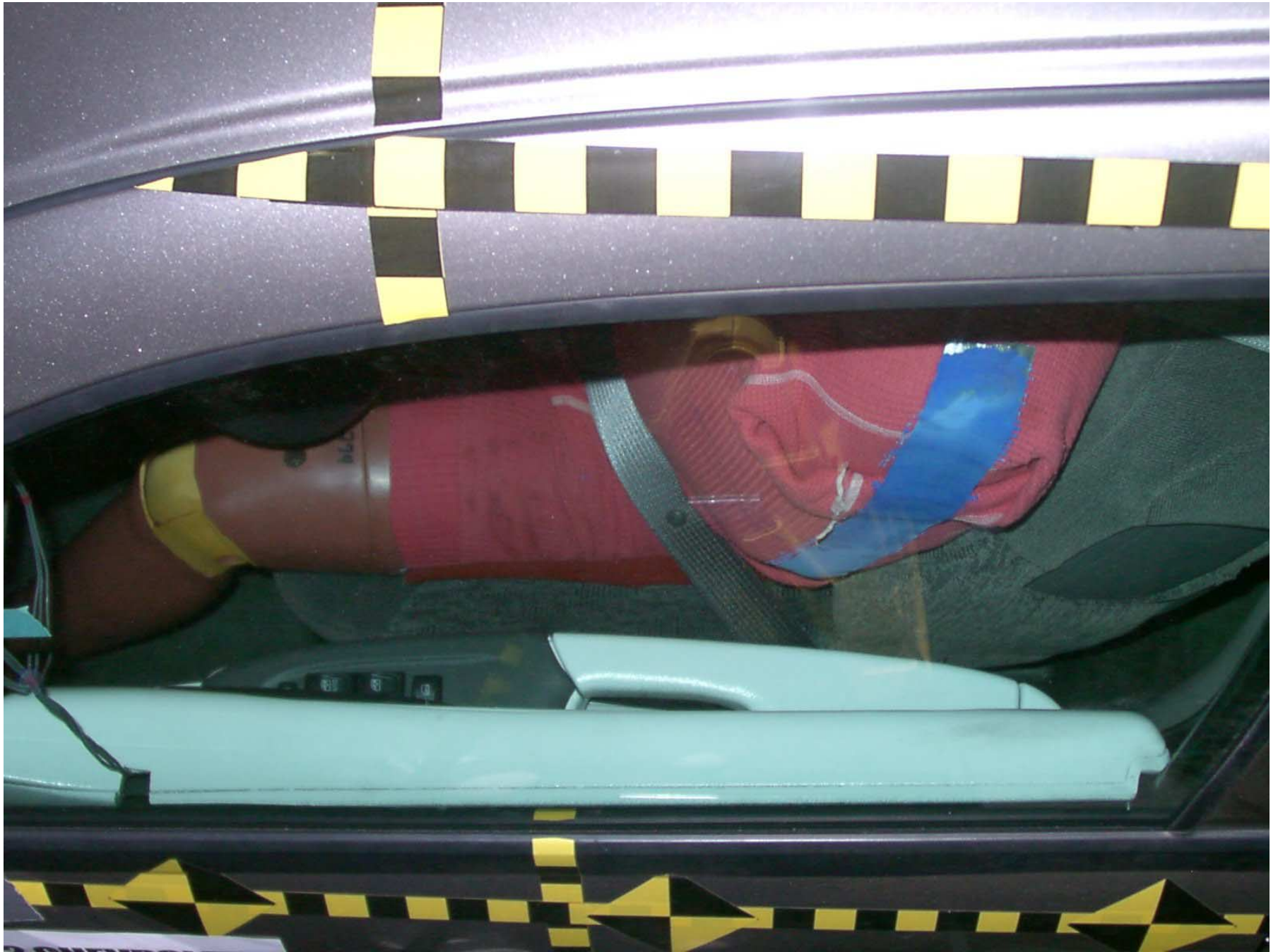
Figure A-25: Driver Dummy Clearance, Pre-Test
