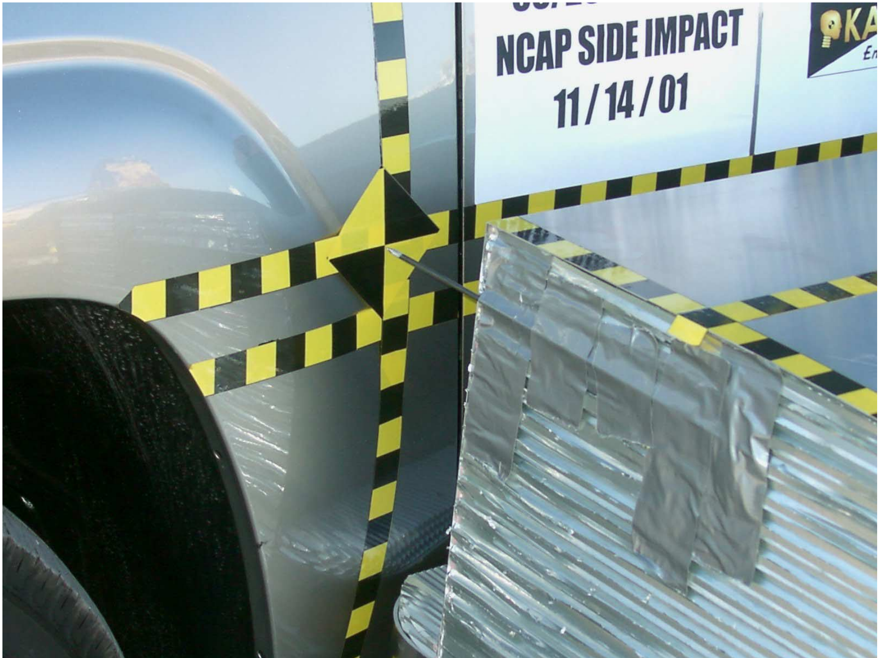
Figure A-16: Impact Point Target Close-up, Pre-Test
