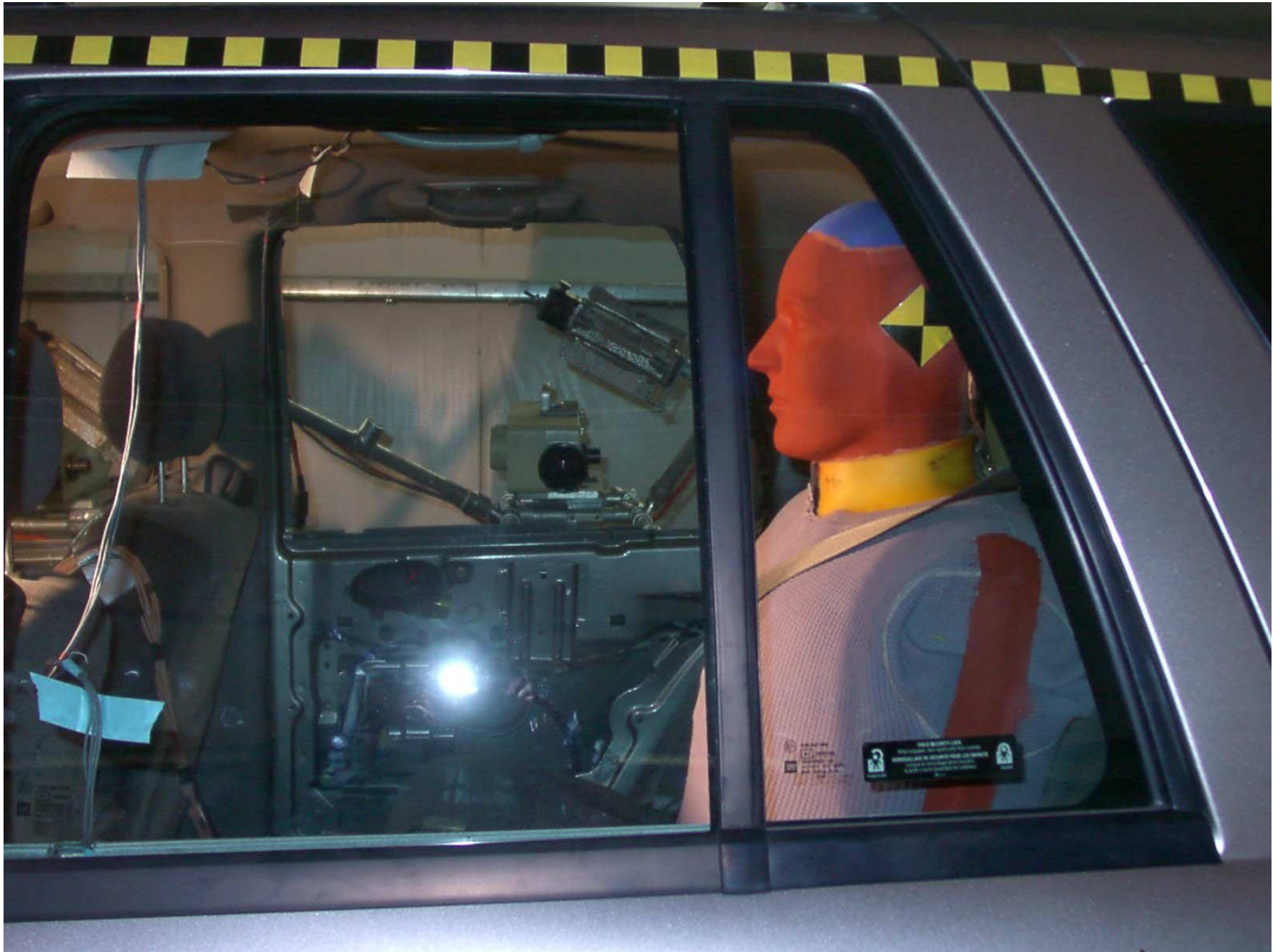
Figure A-32: Passenger Dummy Left Side, Pre-Test
