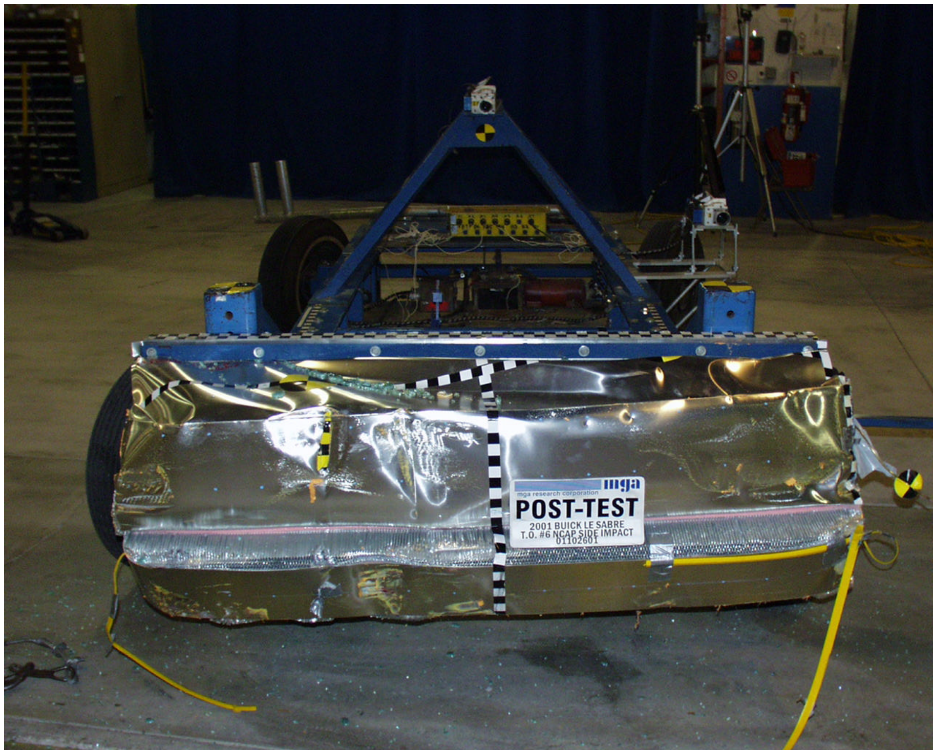
Photo No. A-13 - Post-Test MDB Front View
