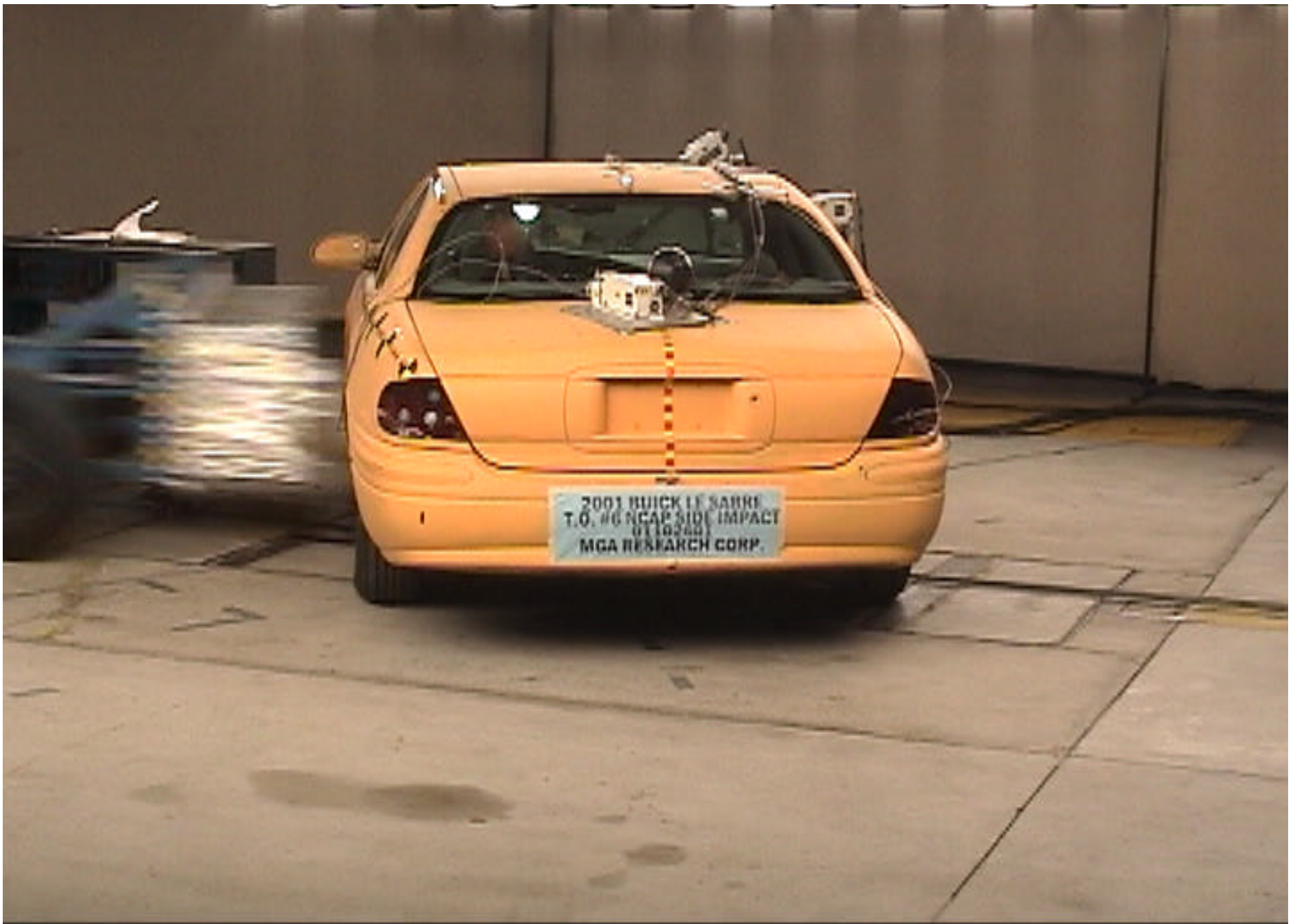
Photo No. A-37 – Impact
