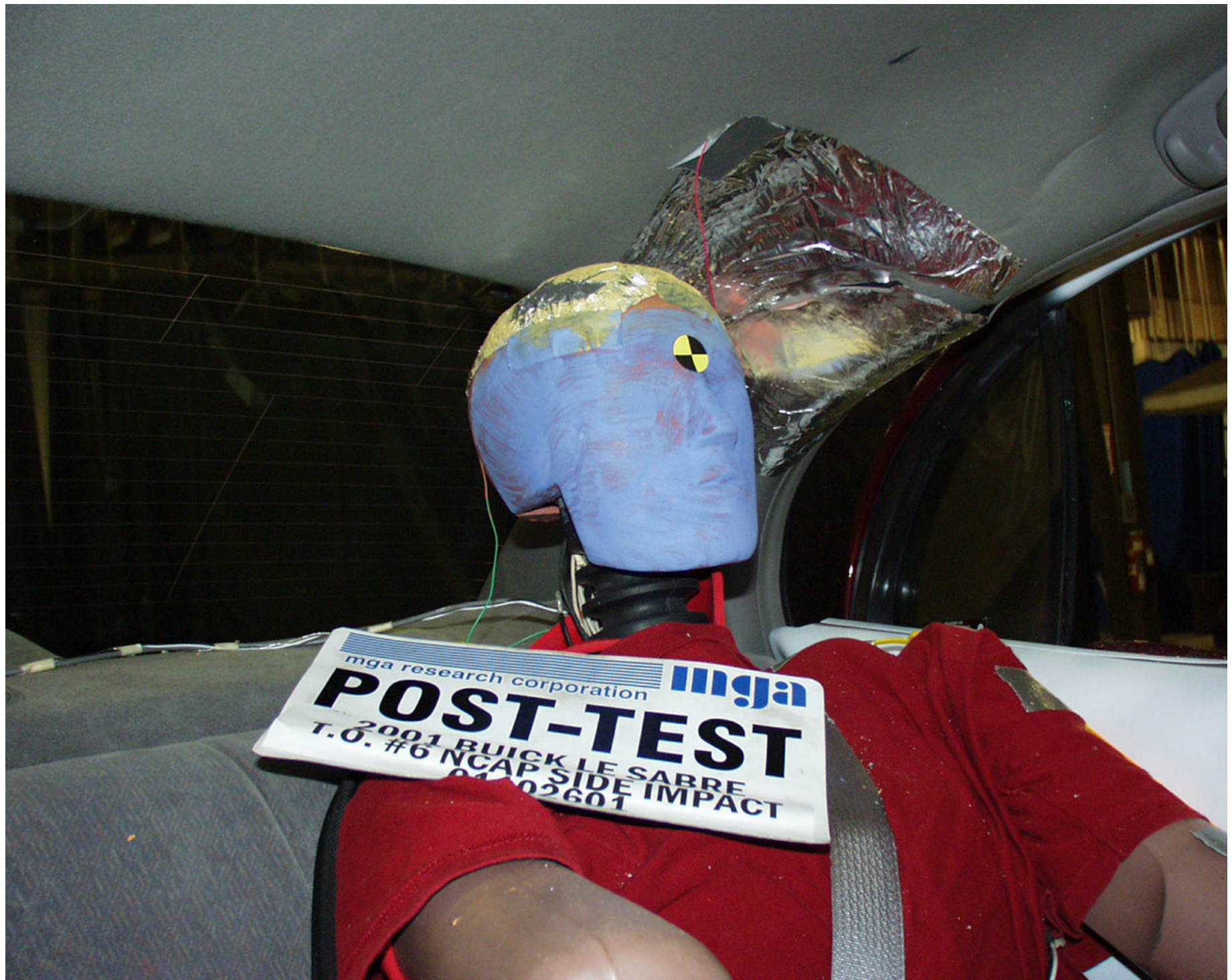
Photo No. A-35 - Post-Test Passenger Head Contact View
