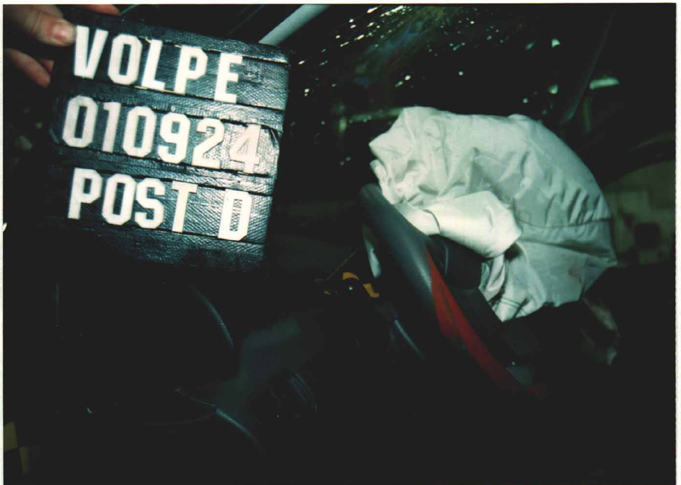
Figure A-62 Post-Test Driver Dummy Chest Contact - View 2
