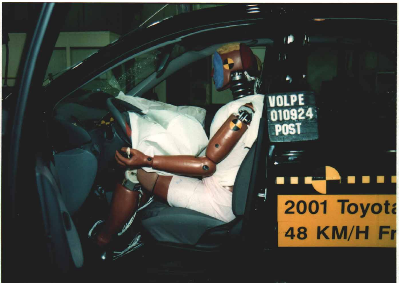
Figure A-40 Post-Test Driver Dummy & Vehicle Interior - View 1
