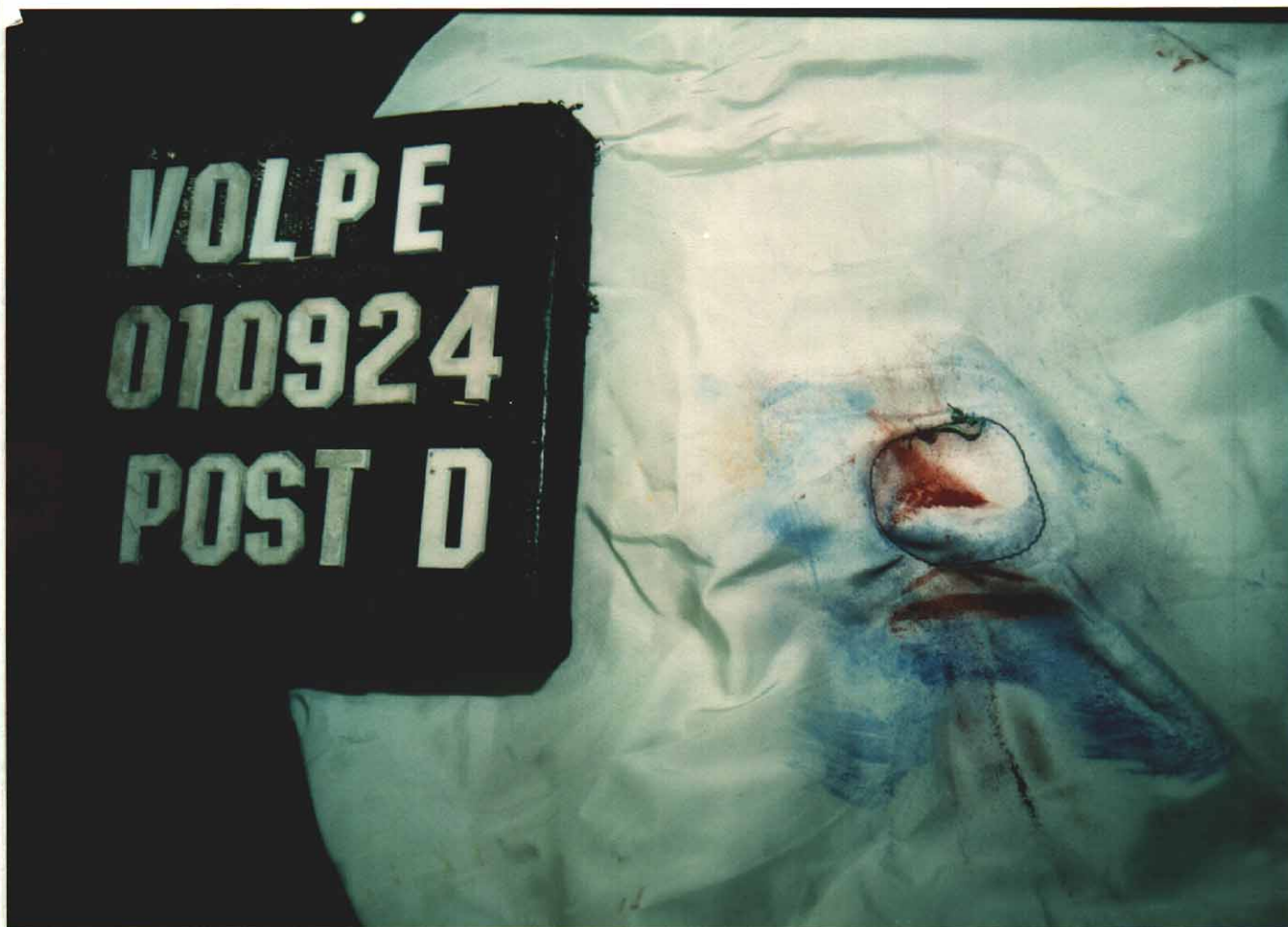
Figure A-57 Post-Test Driver Dummy Head Contact - View 2
