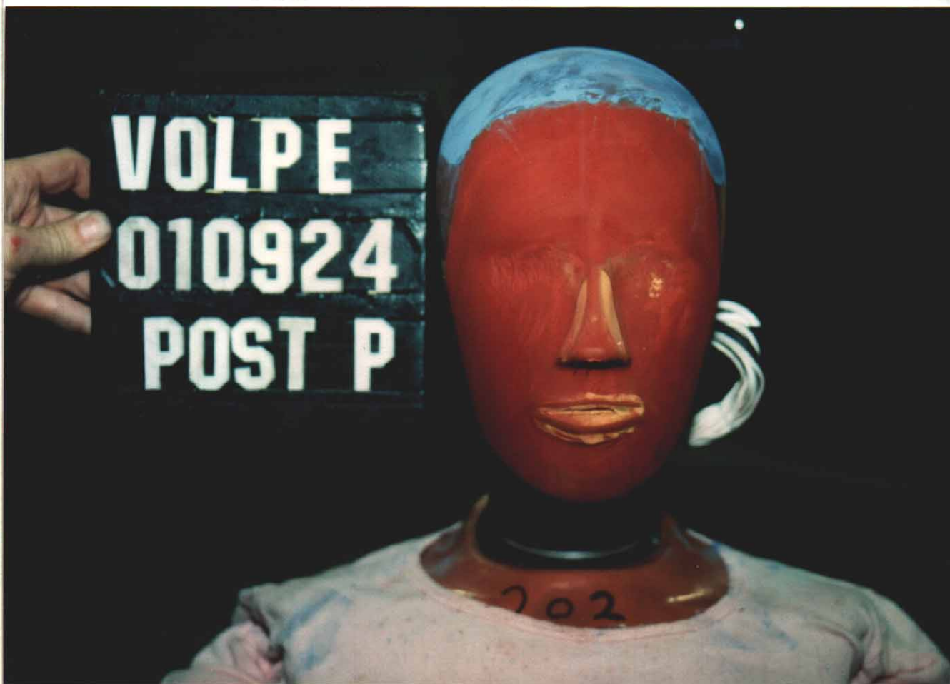
Figure A-67 Post-Test Passenger Dummy Head Contact - View 1
