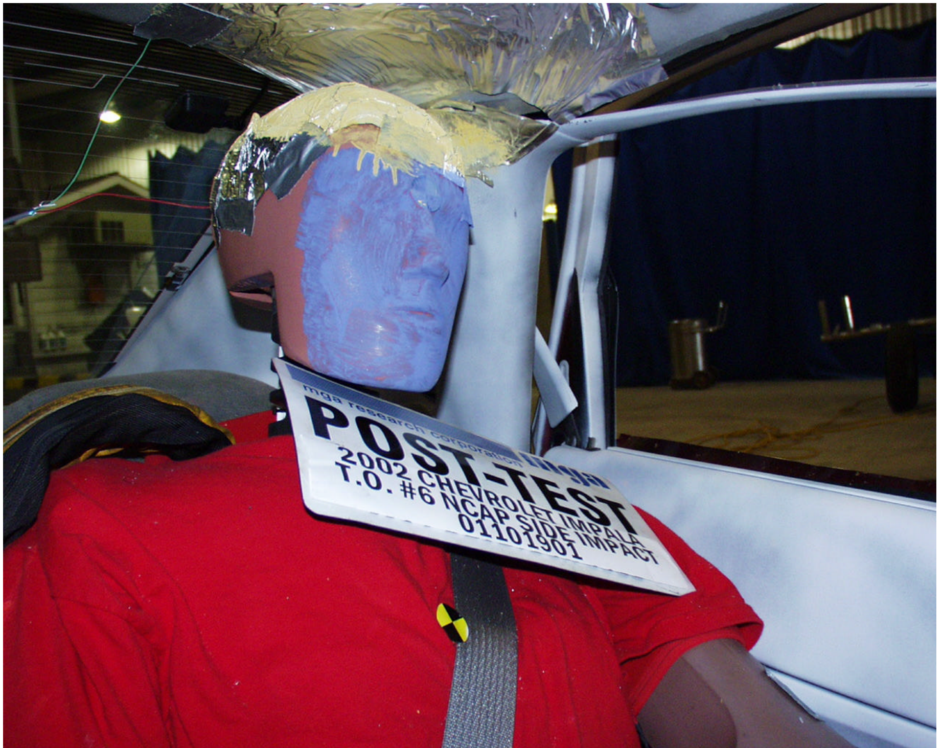
Photo No. A-36 - Post-Test Passenger Head Contact
