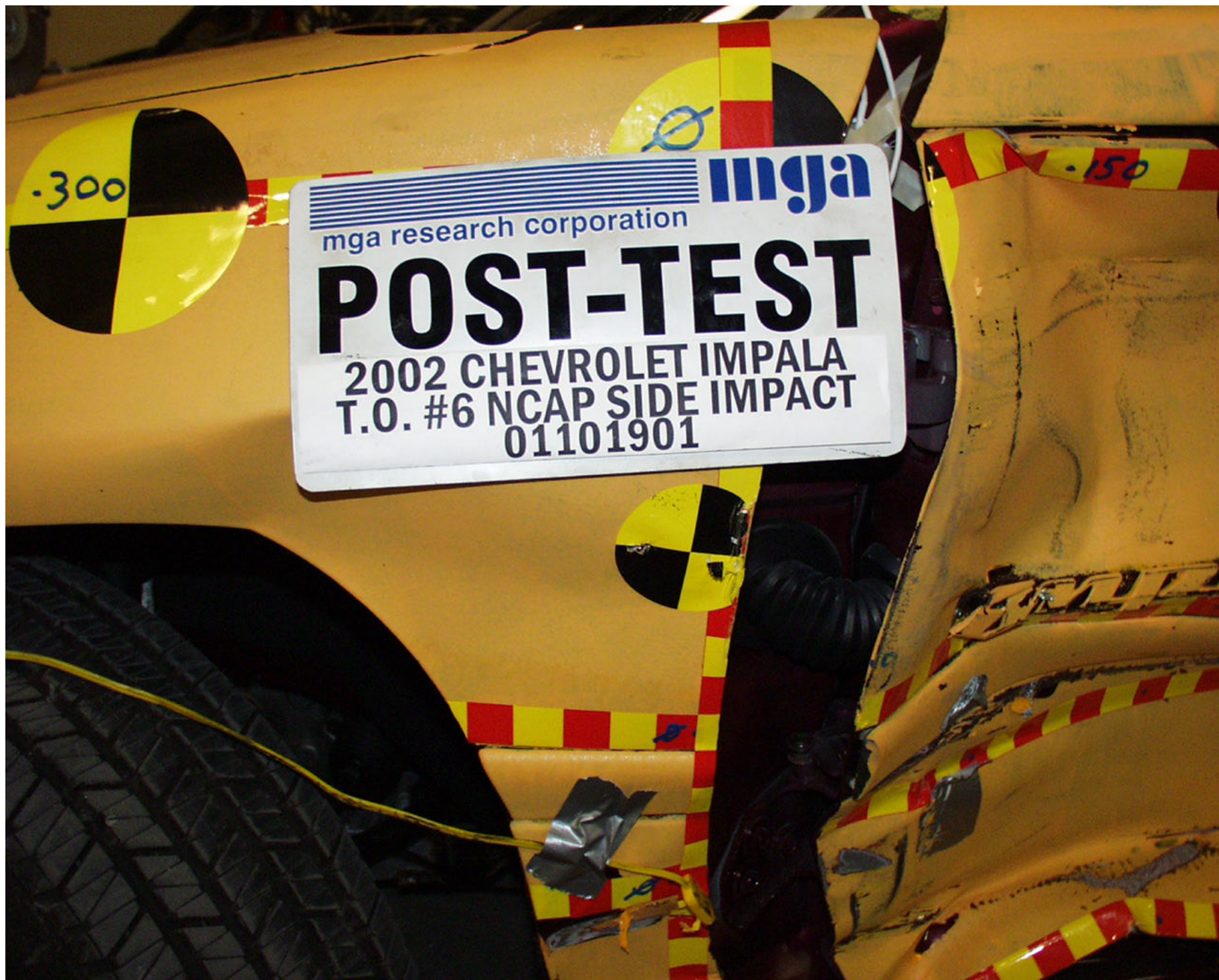
Photo No. A-40 - Post-Test Impact Point
