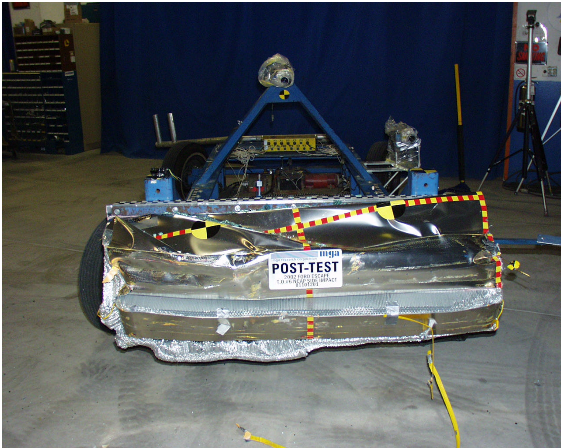
Photo No. A-15 - Post-Test MDB Front View
