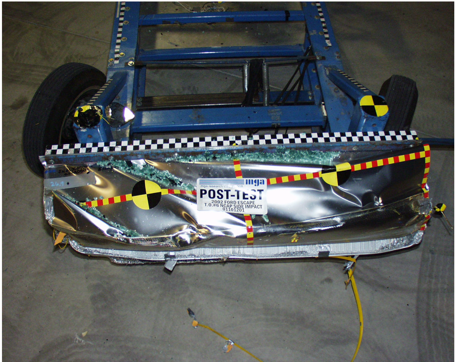
Photo No. A-13 - Post-Test MDB Top View
