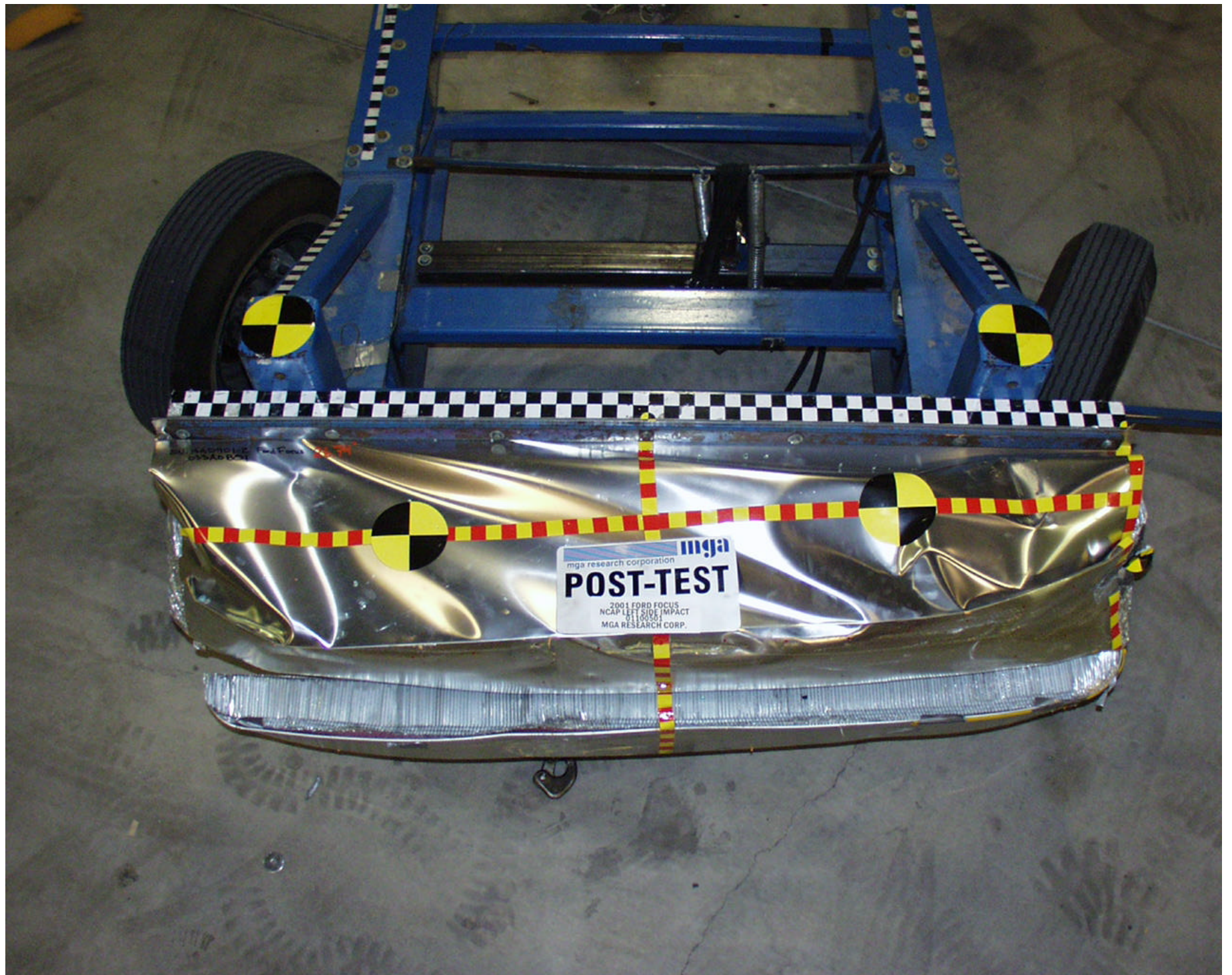
Photo No. A-13 - Post-Test MDB Top View
