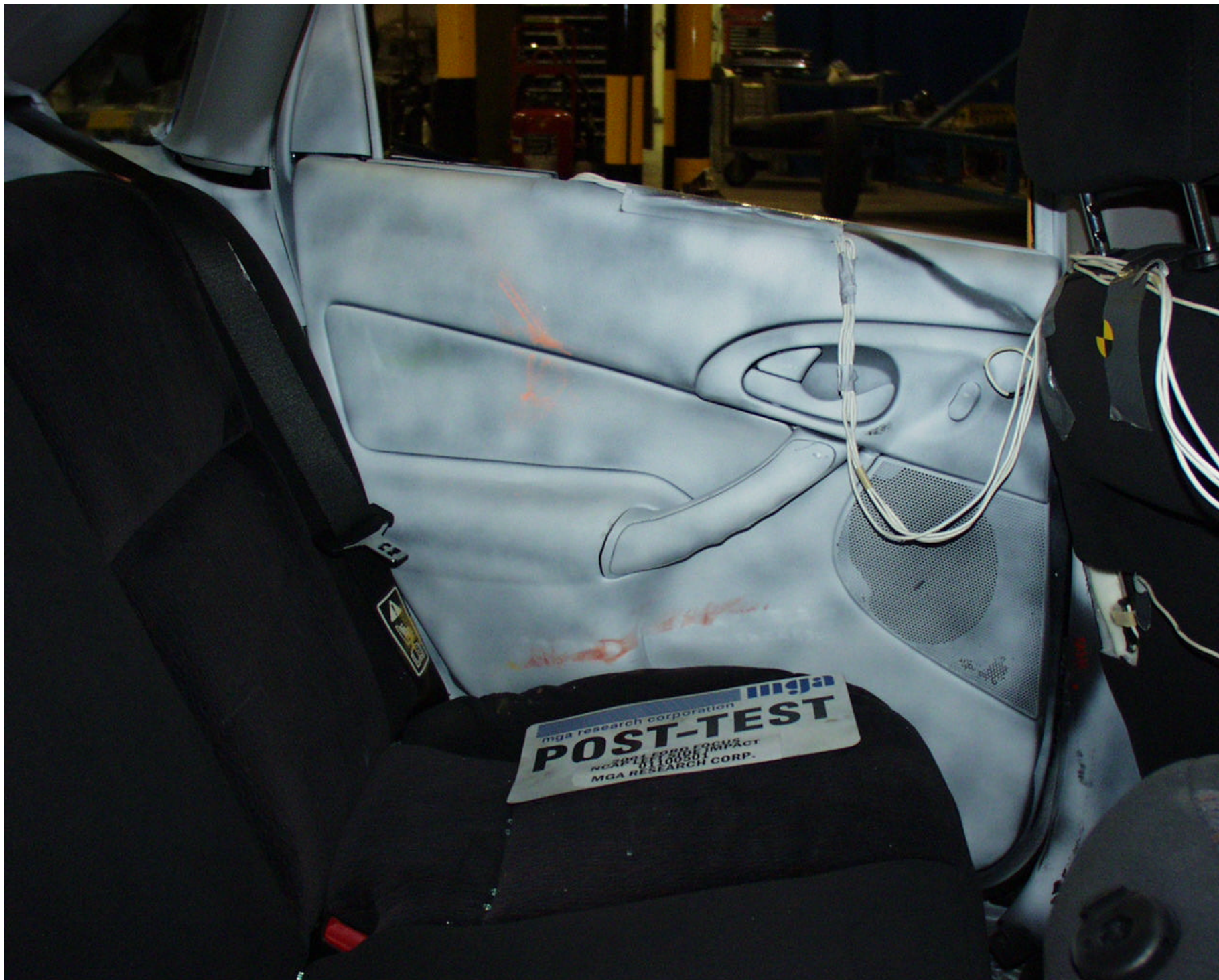
Photo No. A-36 - Post-Test Passenger Contact
