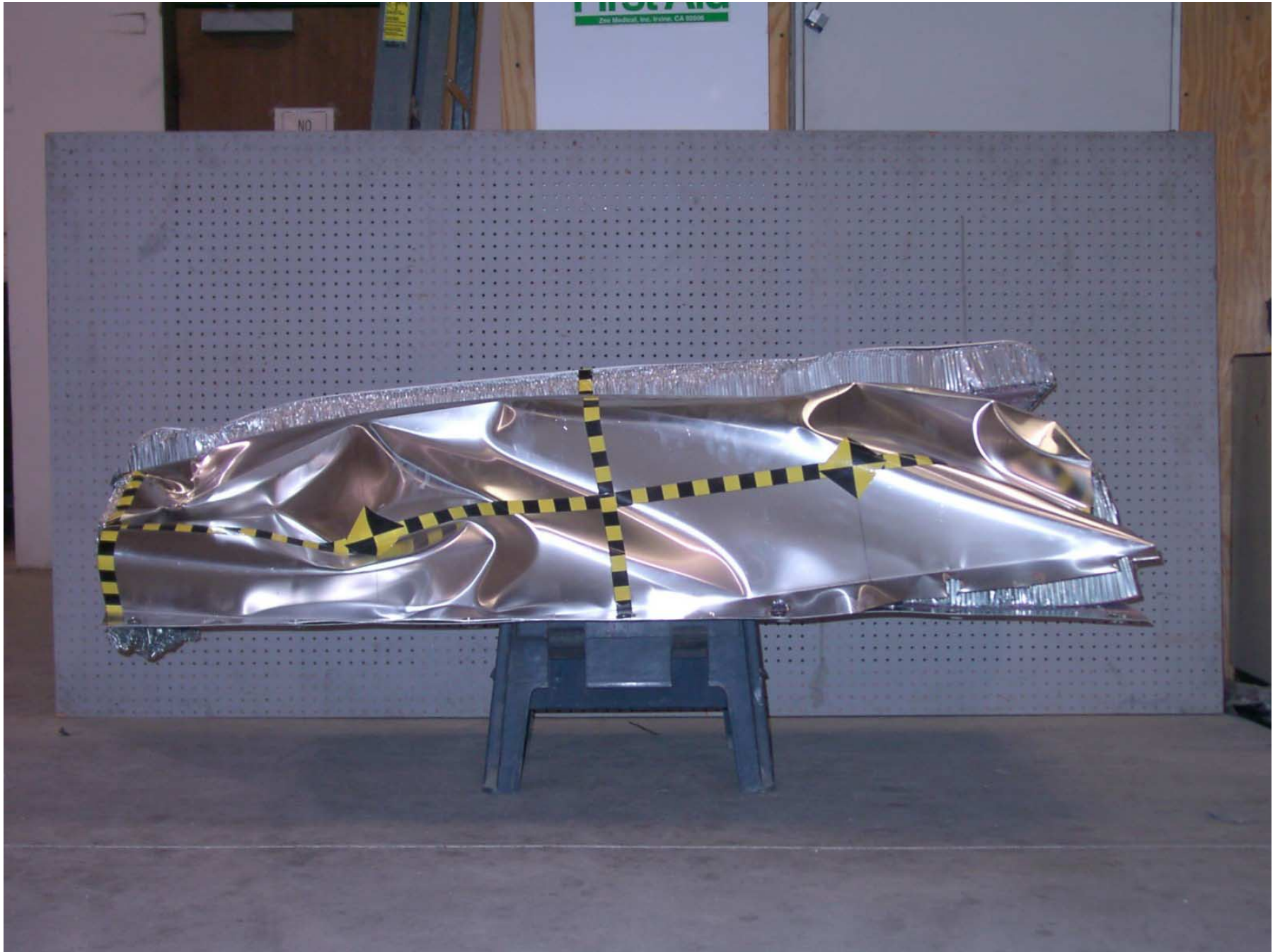
Figure A-43: Top View of Deformable Barrier, Post-Test
