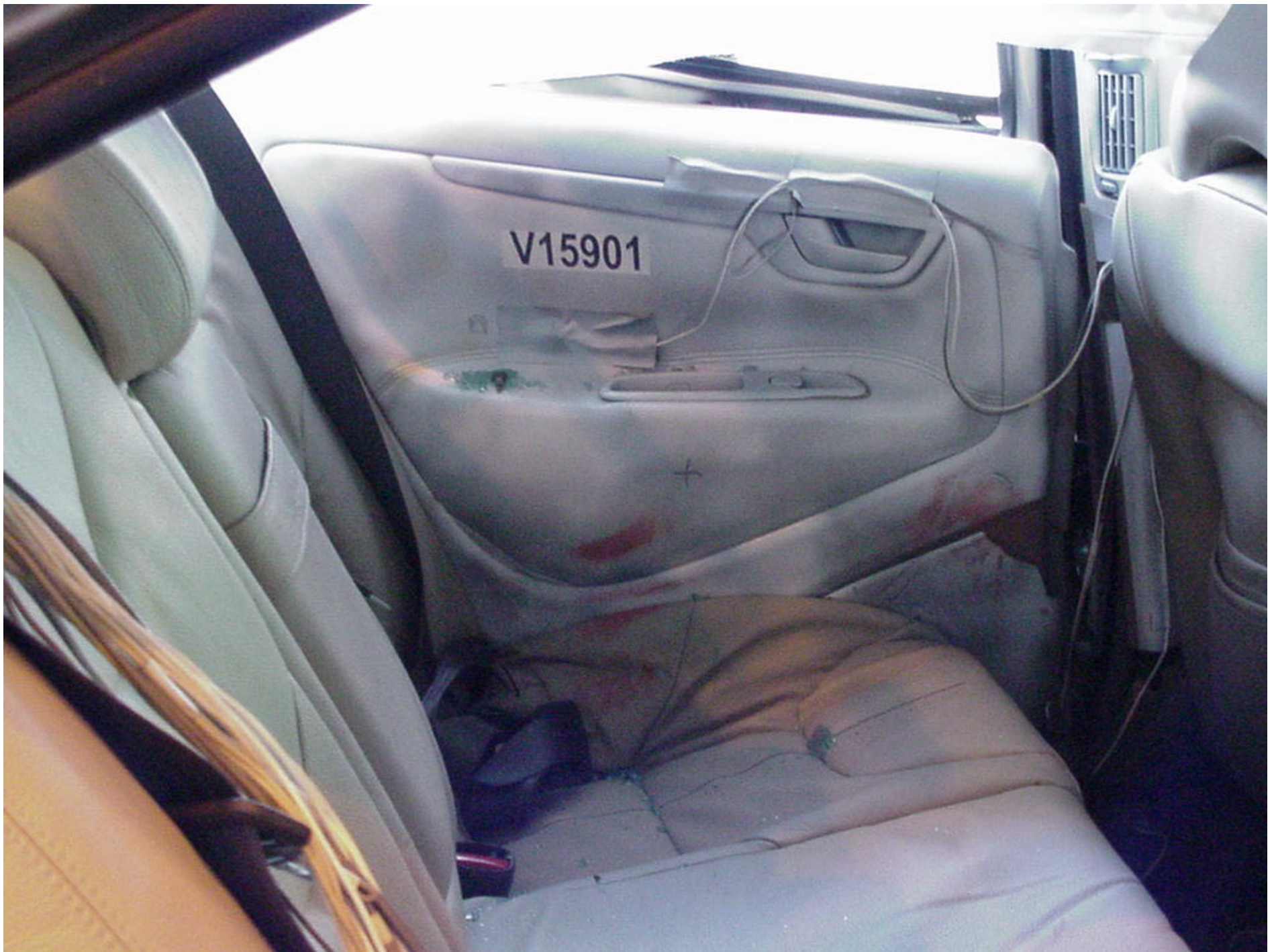
Figure A-28 POST-TEST INTERIOR OF REAR DOOR SHOWING SID IMPACT LOCATIONS
