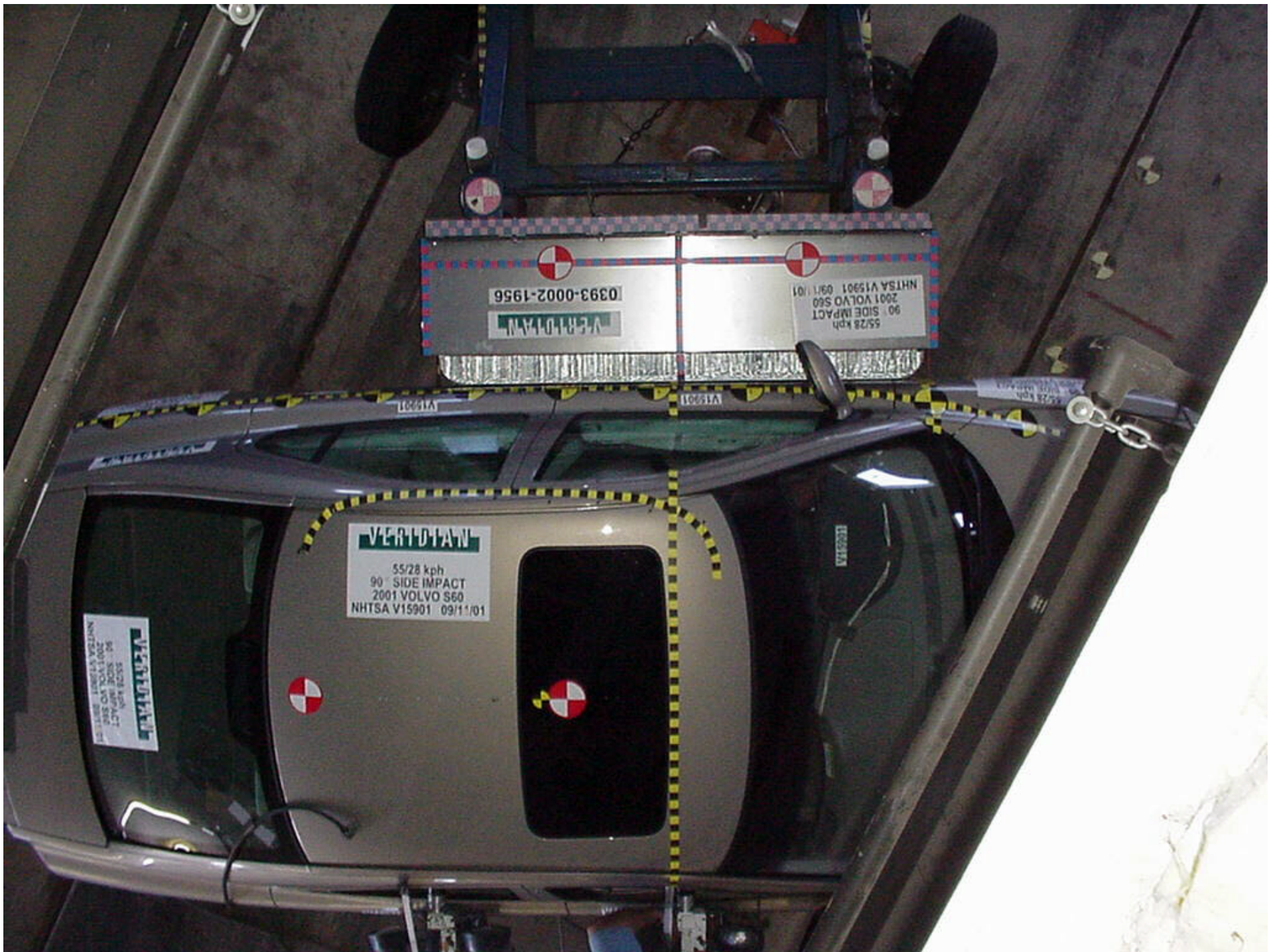
Figure A-15 PRE-TEST OVERHEAD VIEW OF ALIGNED MDB AND VEHICLE
