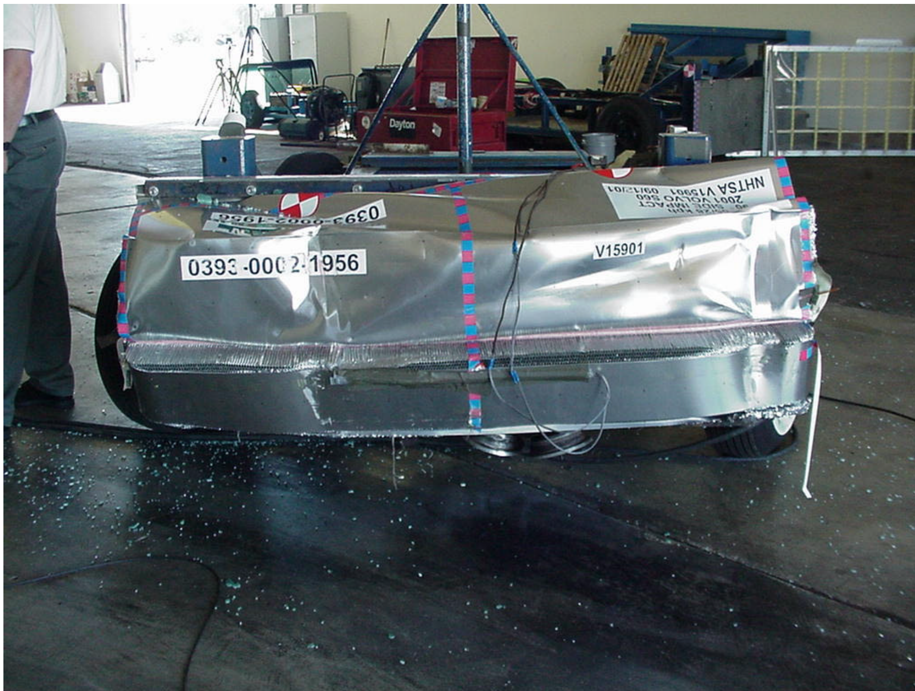
Figure A-8 POST-TEST FRONTAL VIEW OF IMPACTOR FACE
