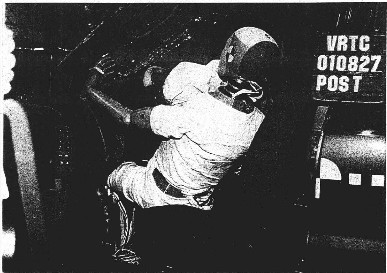
Figure A-47 Post-Test Driver Dummy & Vehicle Interior - View 1
