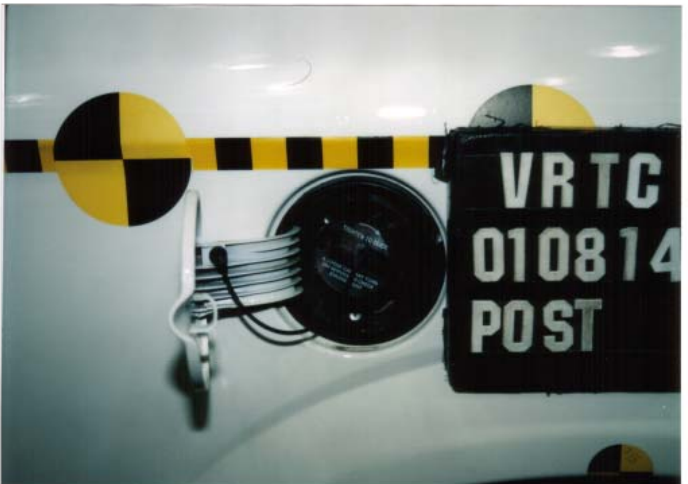
Figure A-42 Post-Test Fuel Filler Cap View
