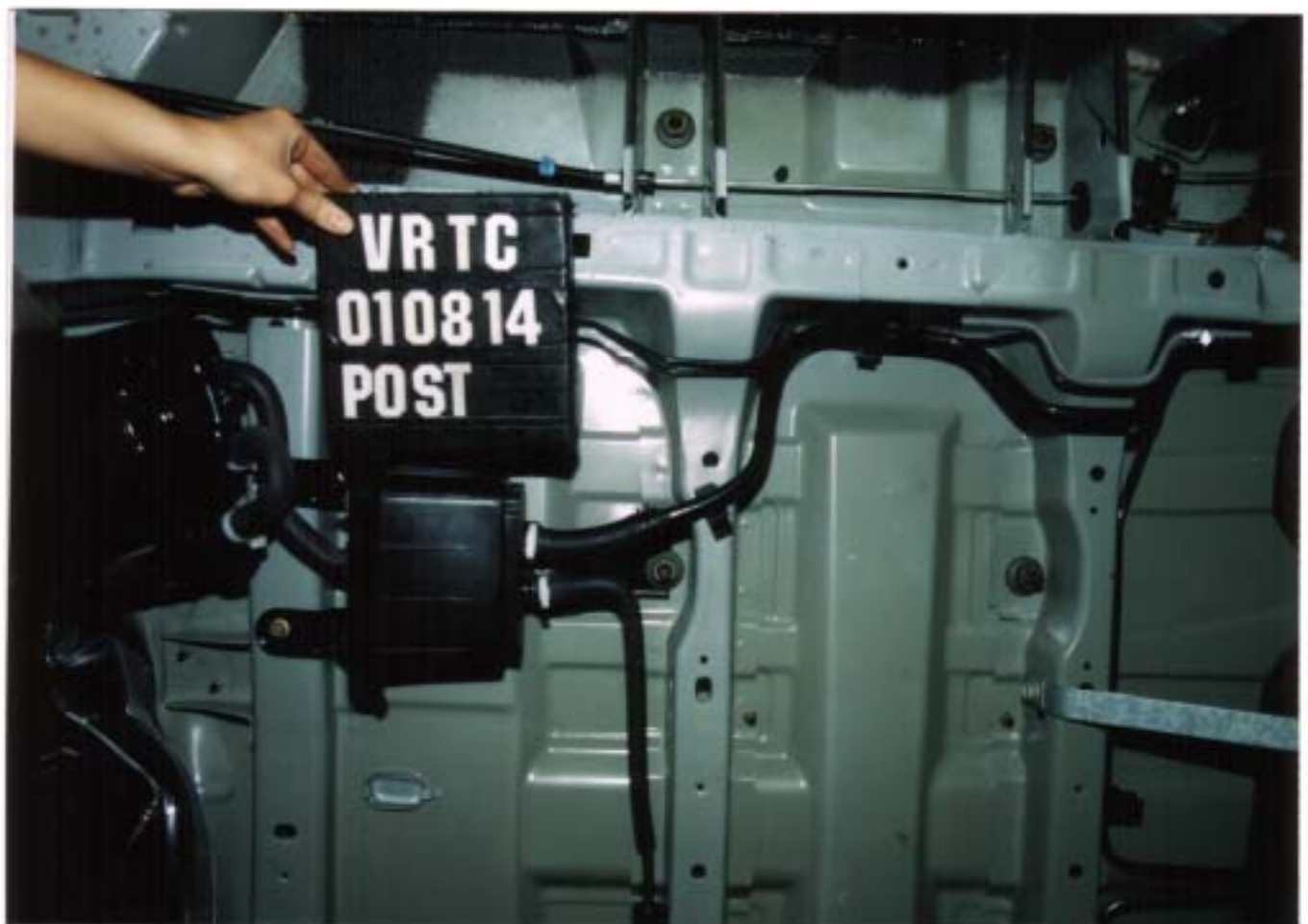
Figure A-38 Post-Test Fuel Lines View
