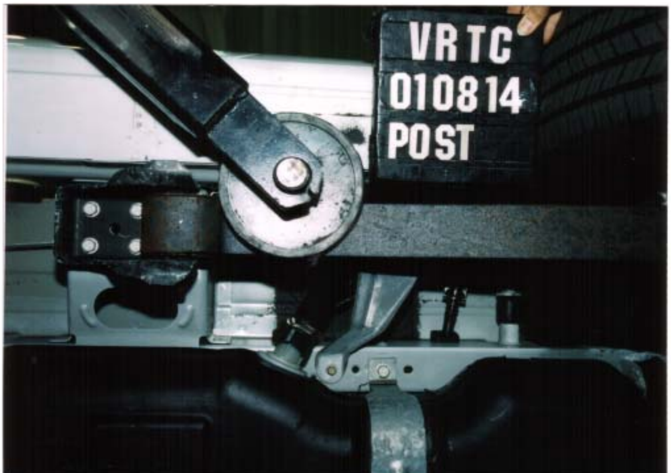
Figure A-40 Post-Test Fuel Filler Neck View
