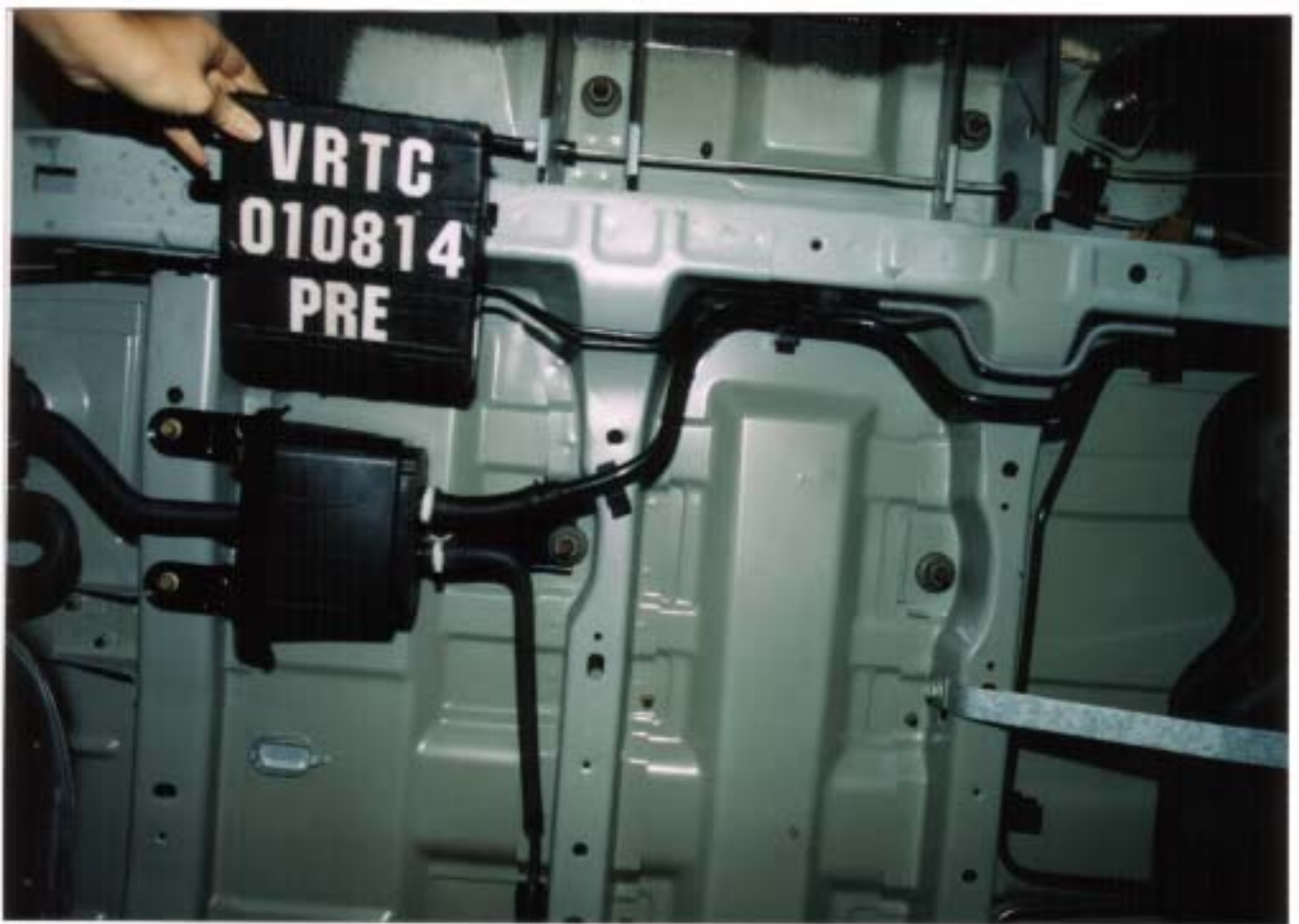
Figure A-37 Pre-Test Fuel Lines View
