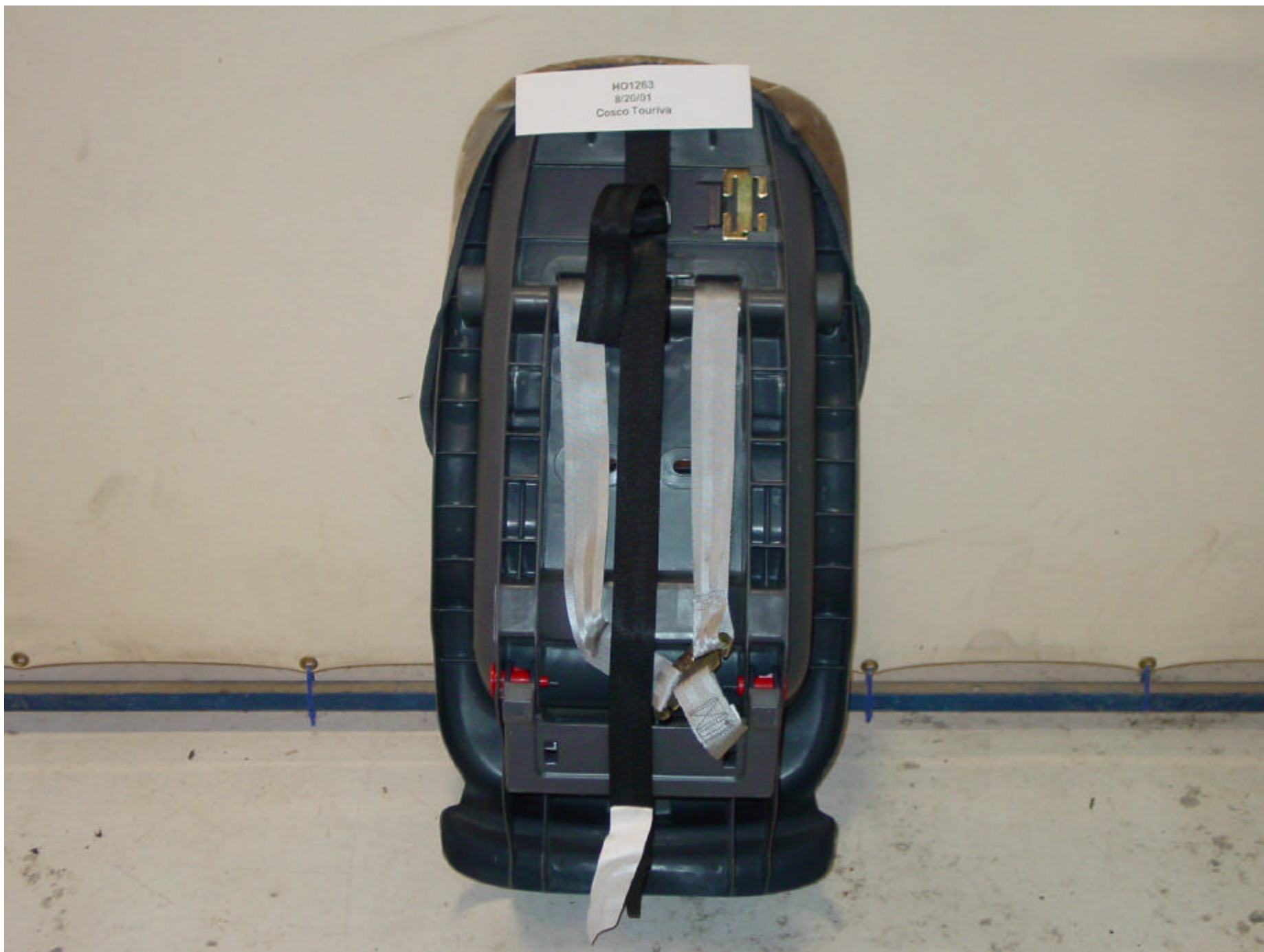
Photo 12 – Post-Test Rear View of Child Seat
