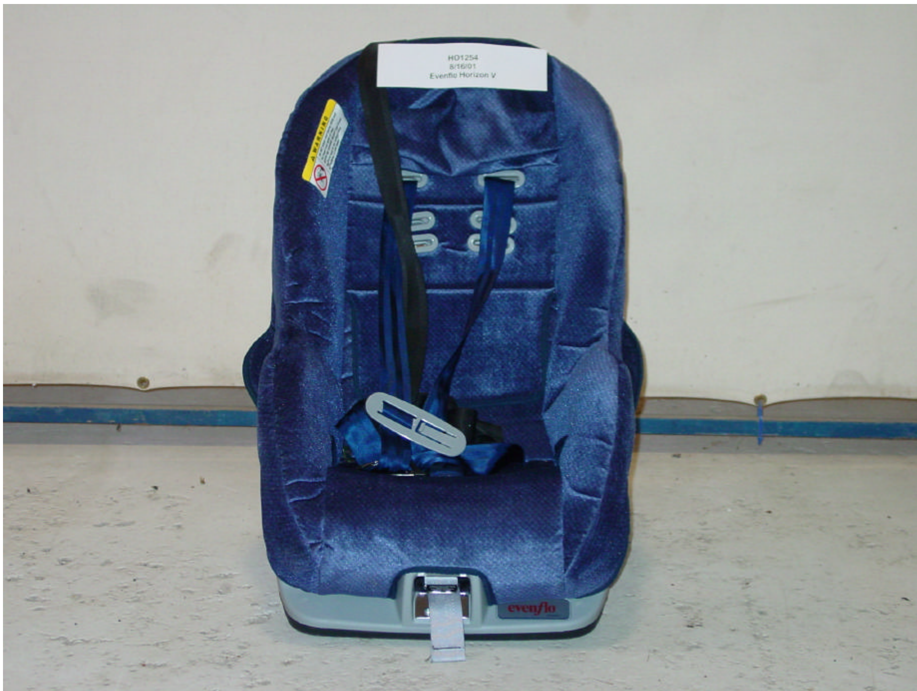
Photo 11 – Post-Test Front View of Child Seat
