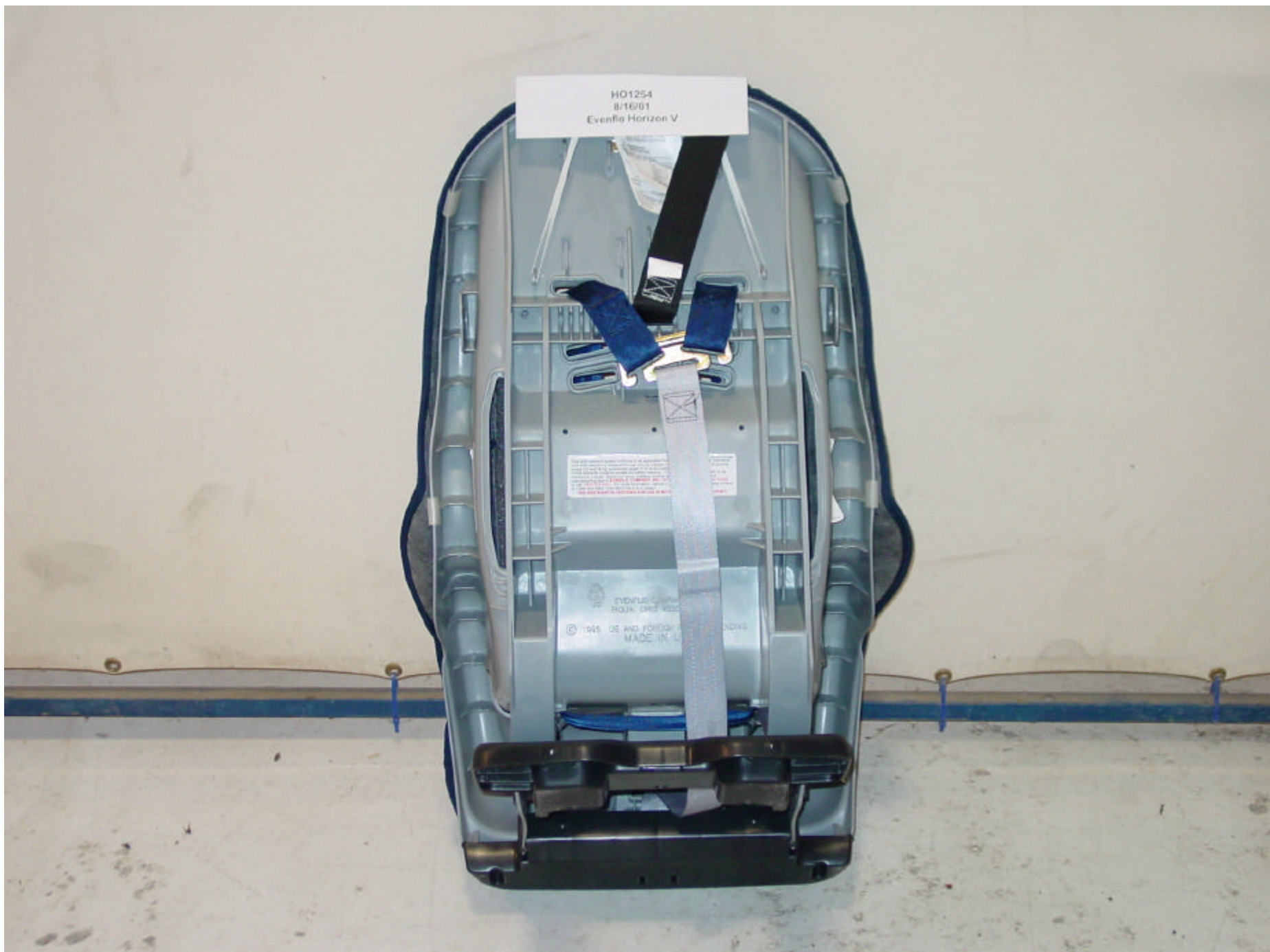
Photo 12 – Post-Test Rear View of Child Seat
