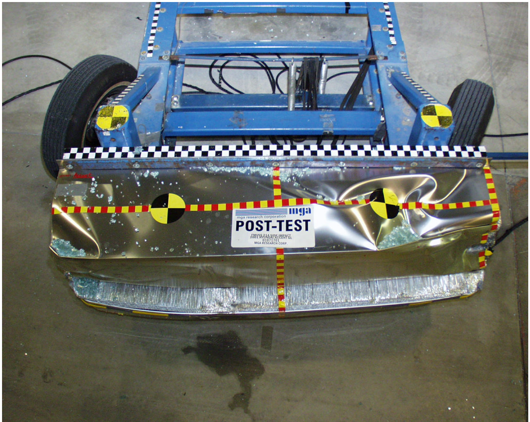
Photo No. A-14 - Post-Test MDB Top View
