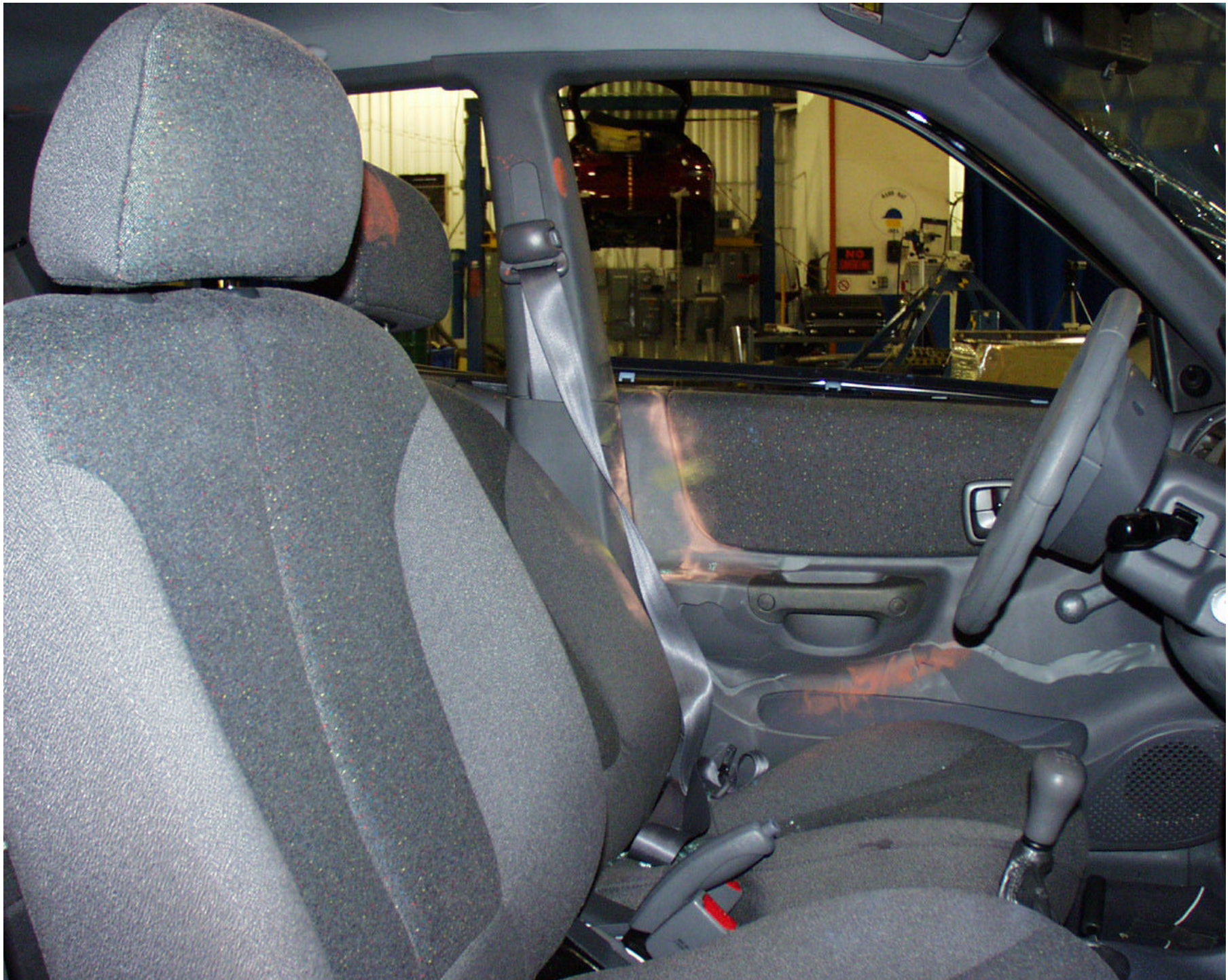
Photo No. A-28 - Post-Test Driver Dummy Contact
