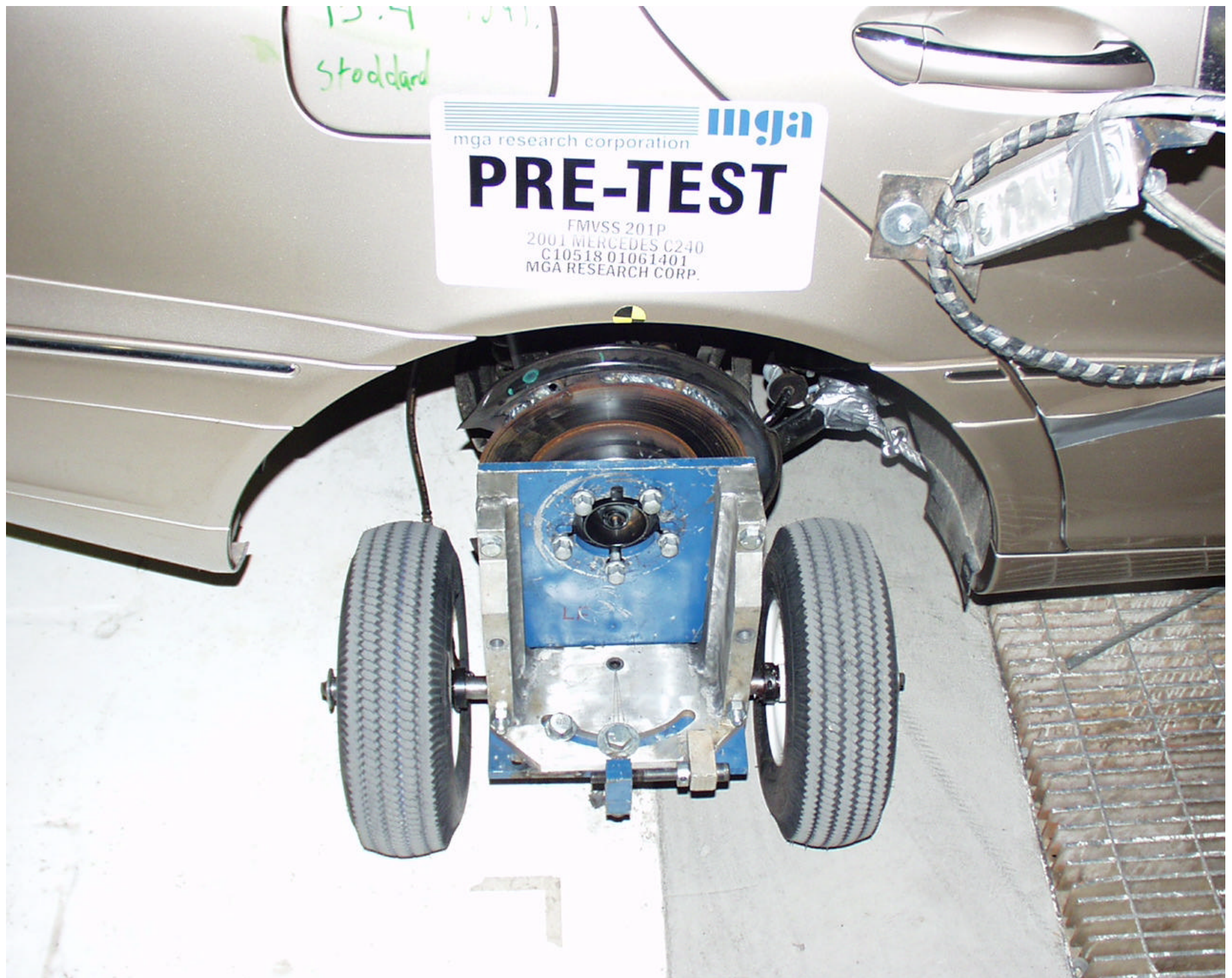
Photo No. A-32 - Pre-Test Right Rear Wheel Dolly
