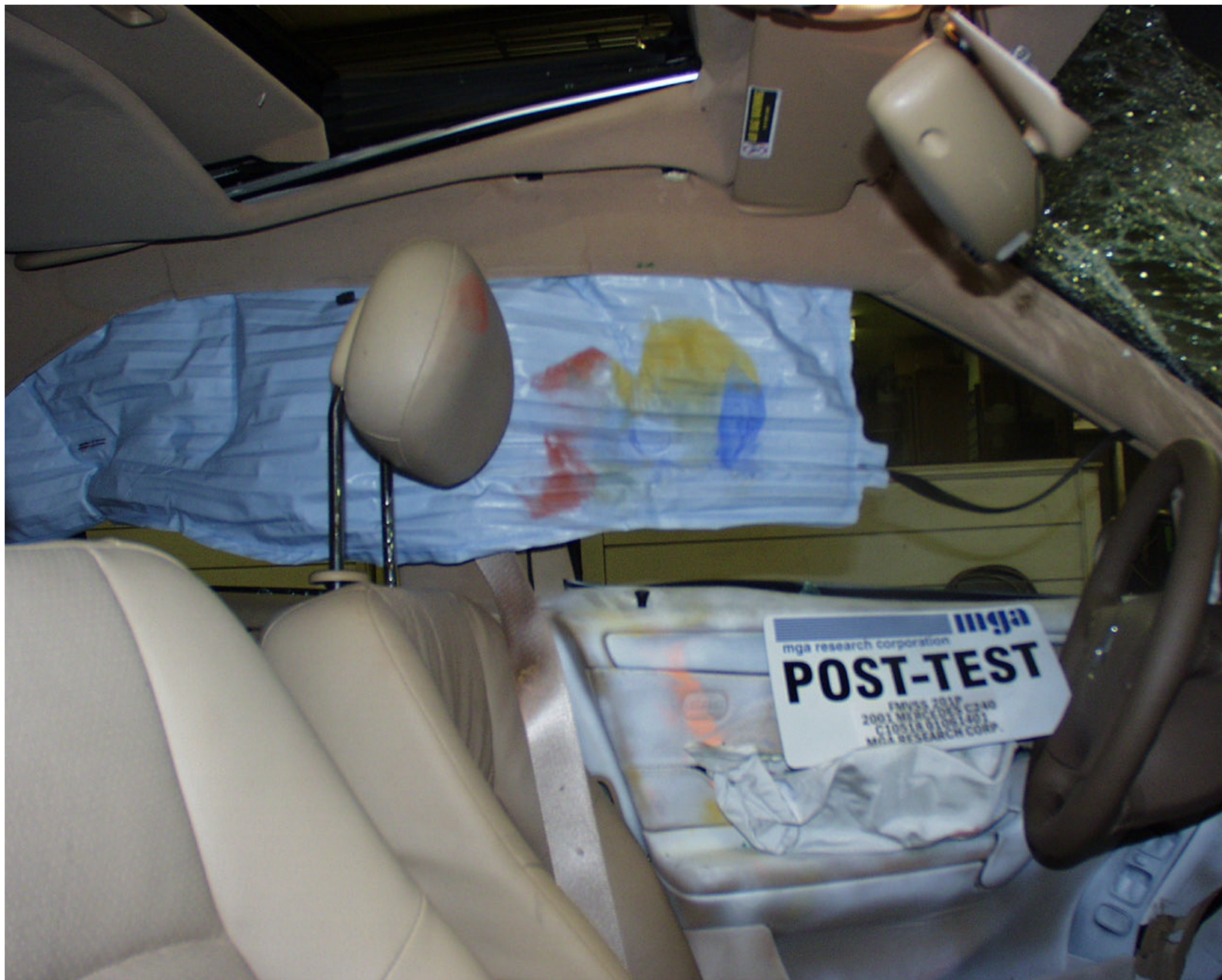
Photo No. A-24 - Post-Test Driver Dummy Head Contact
