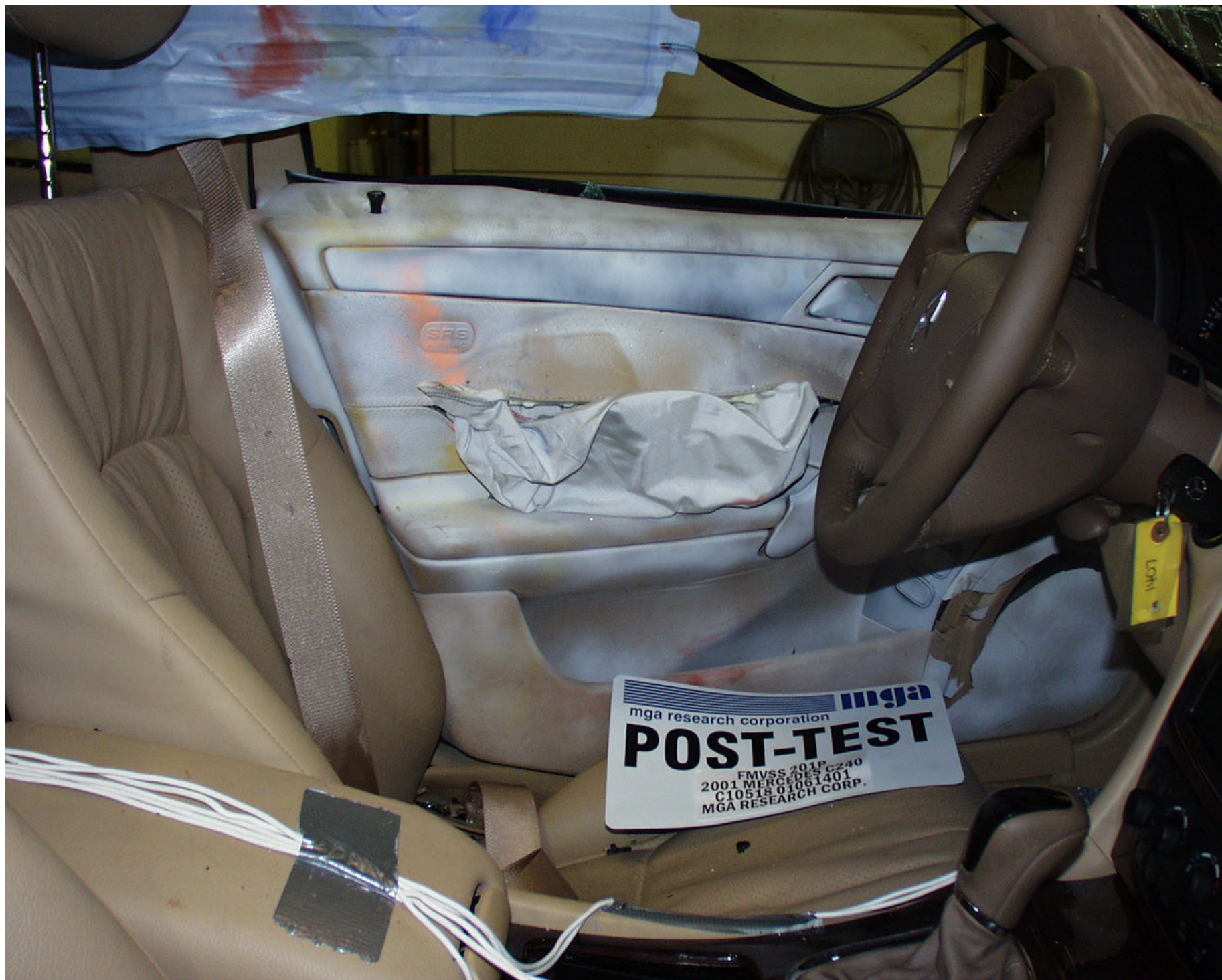
Photo No. A-25 - Post-Test Driver Dummy Thorax Contact
