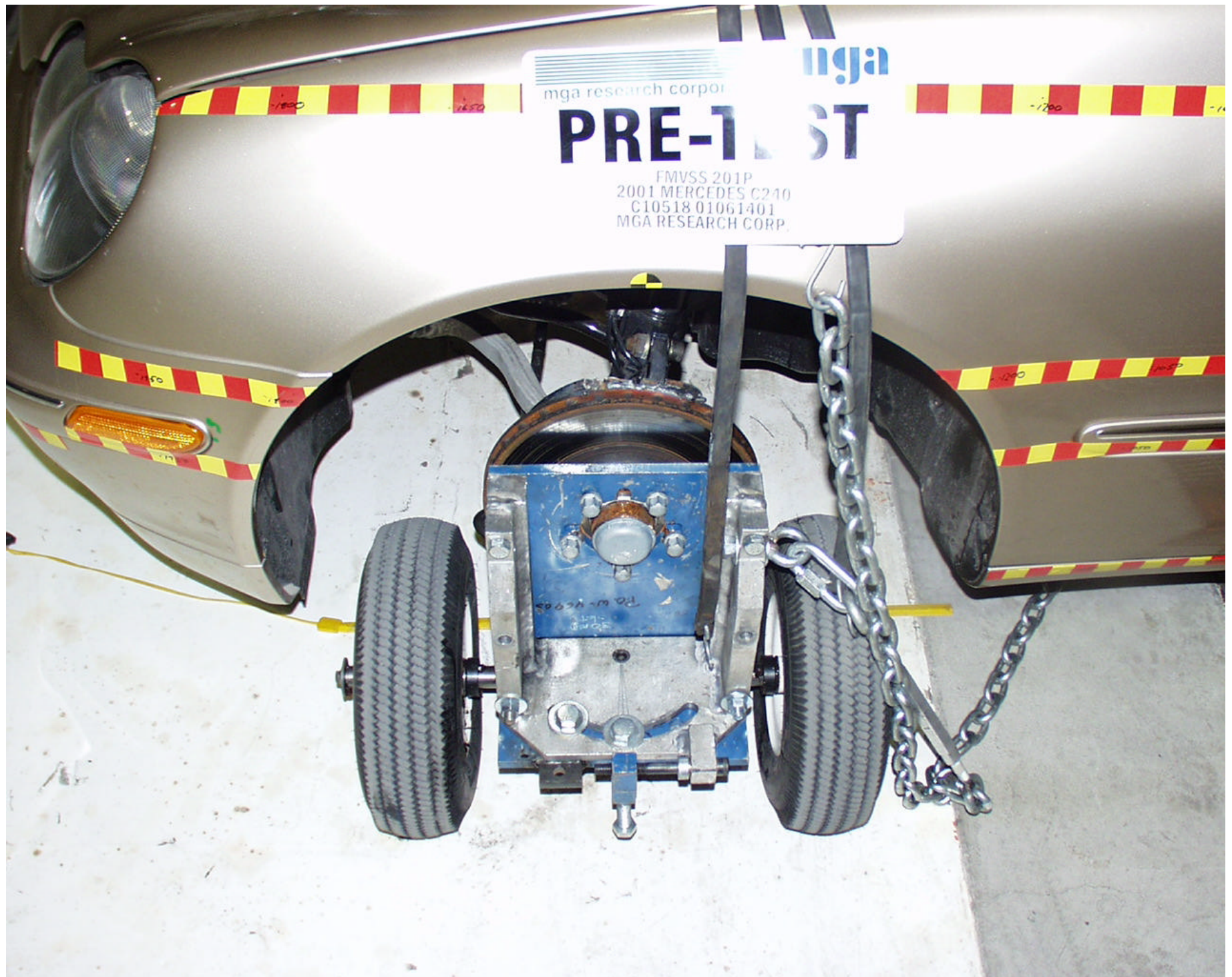
Photo No. A-29 - Pre-Test Left Front Wheel Dolly
