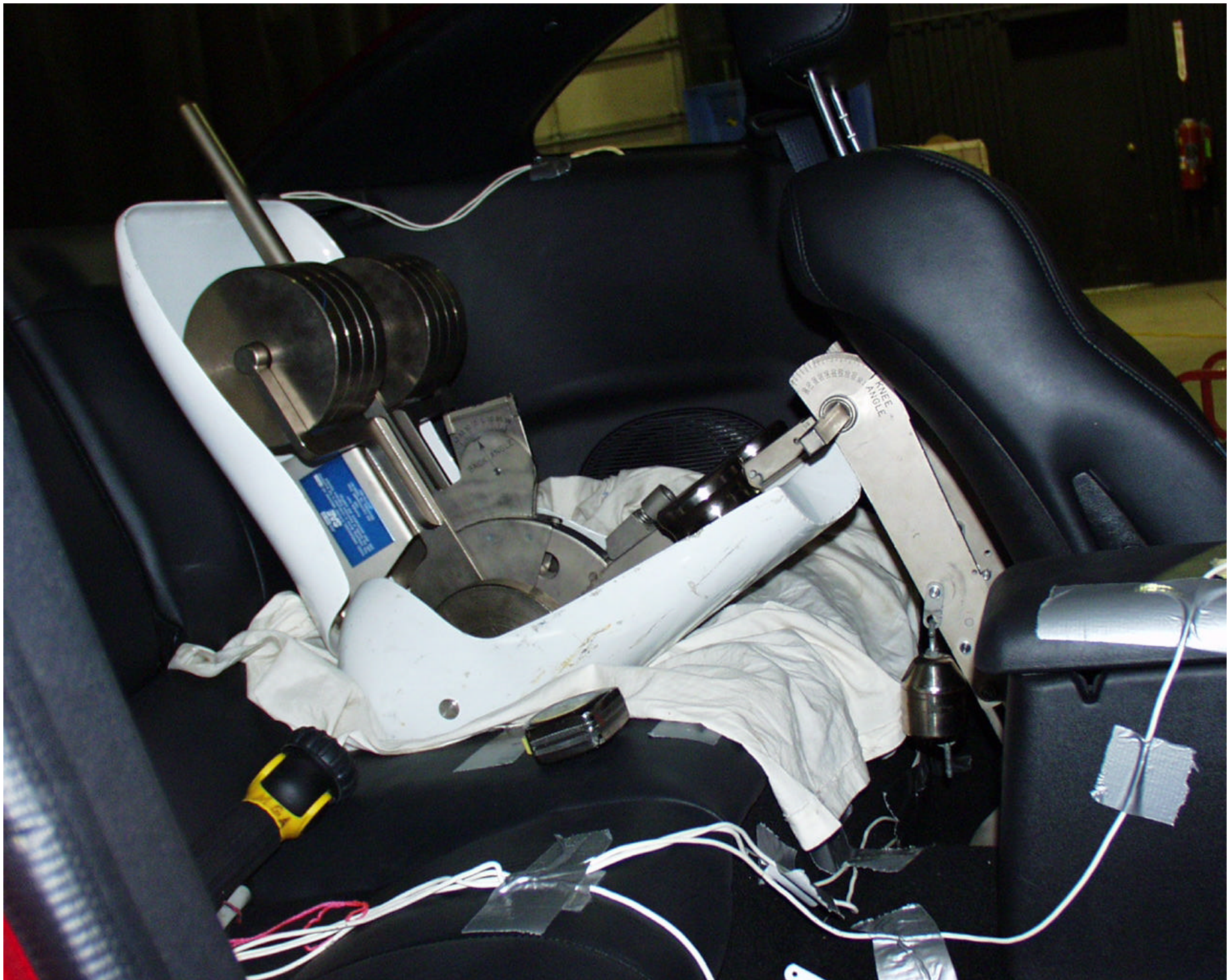
Photo No. A-45 - H-Point Machine Right Side View
