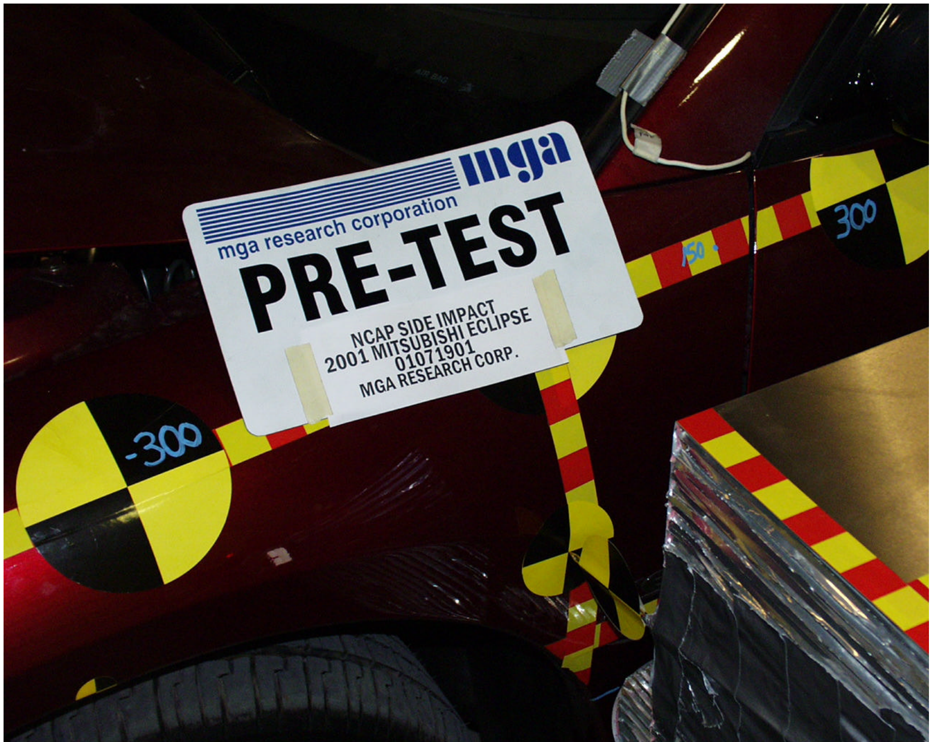
Photo No. A-33 - Pre-Test Left Front Impact Point on Vehicle
