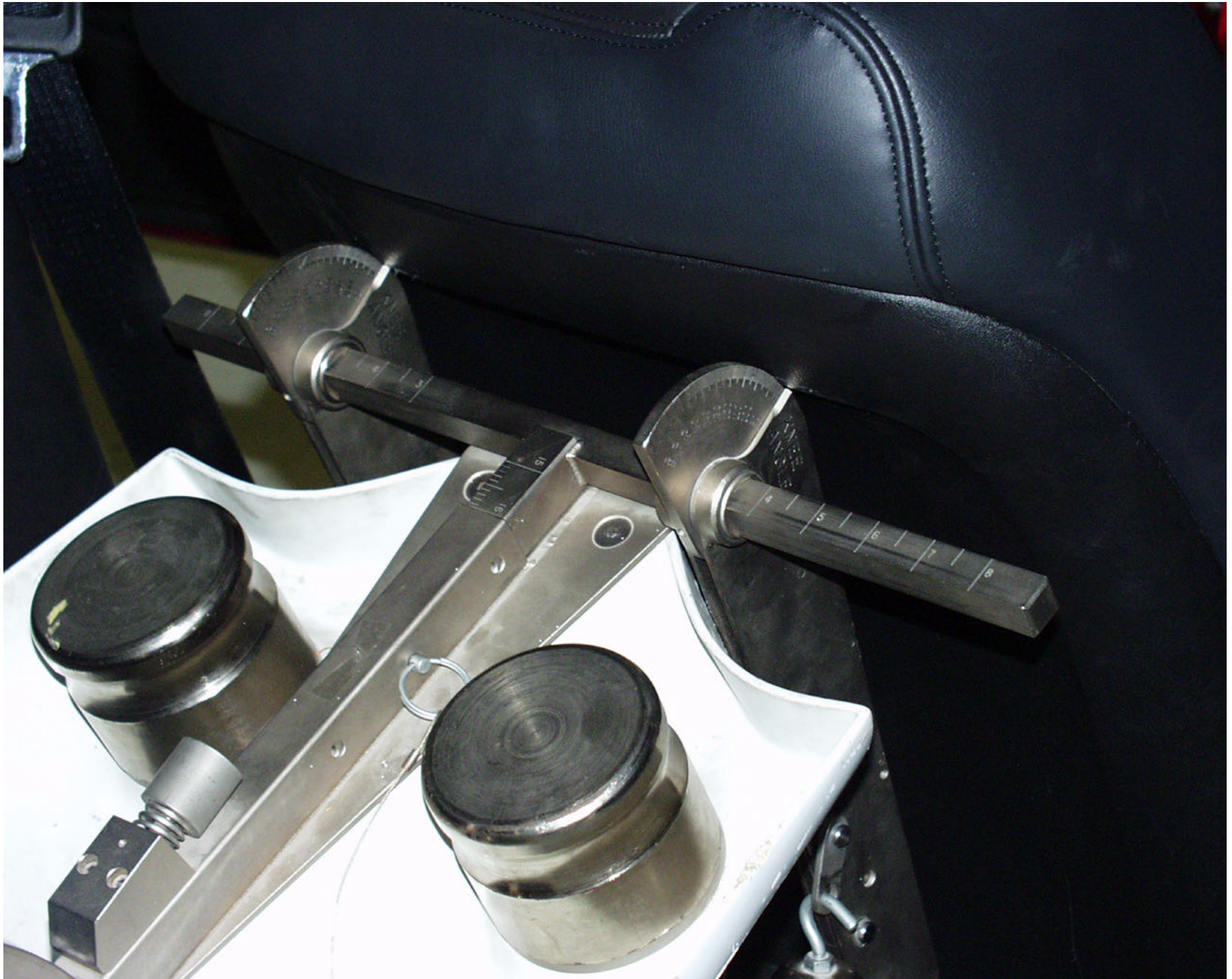
Photo No. A-44 - H-Point Machine Clearance
