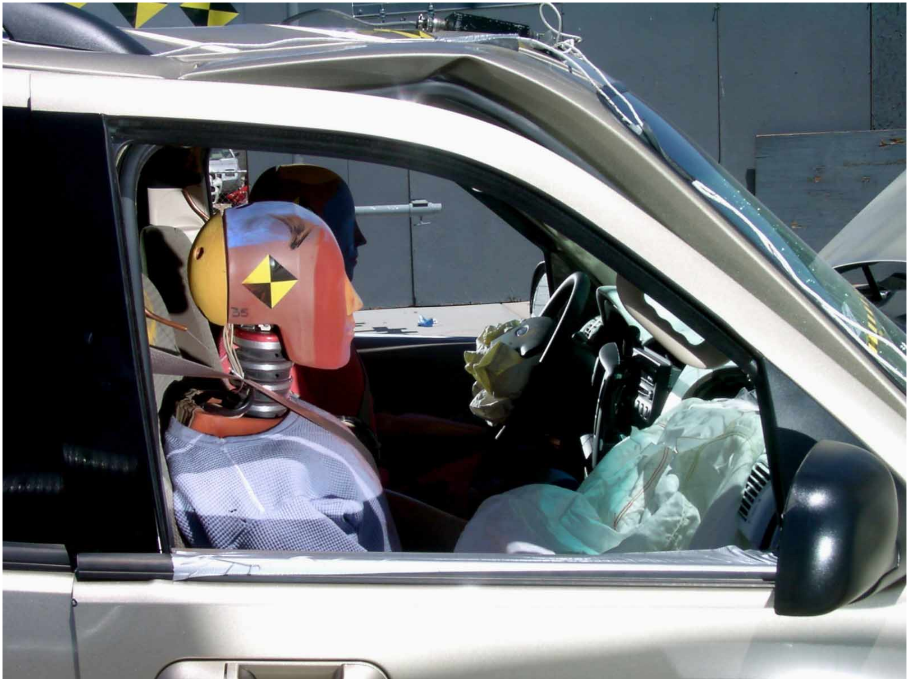
Figure A-44: Passenger Dummy Through Window, Post-Test
