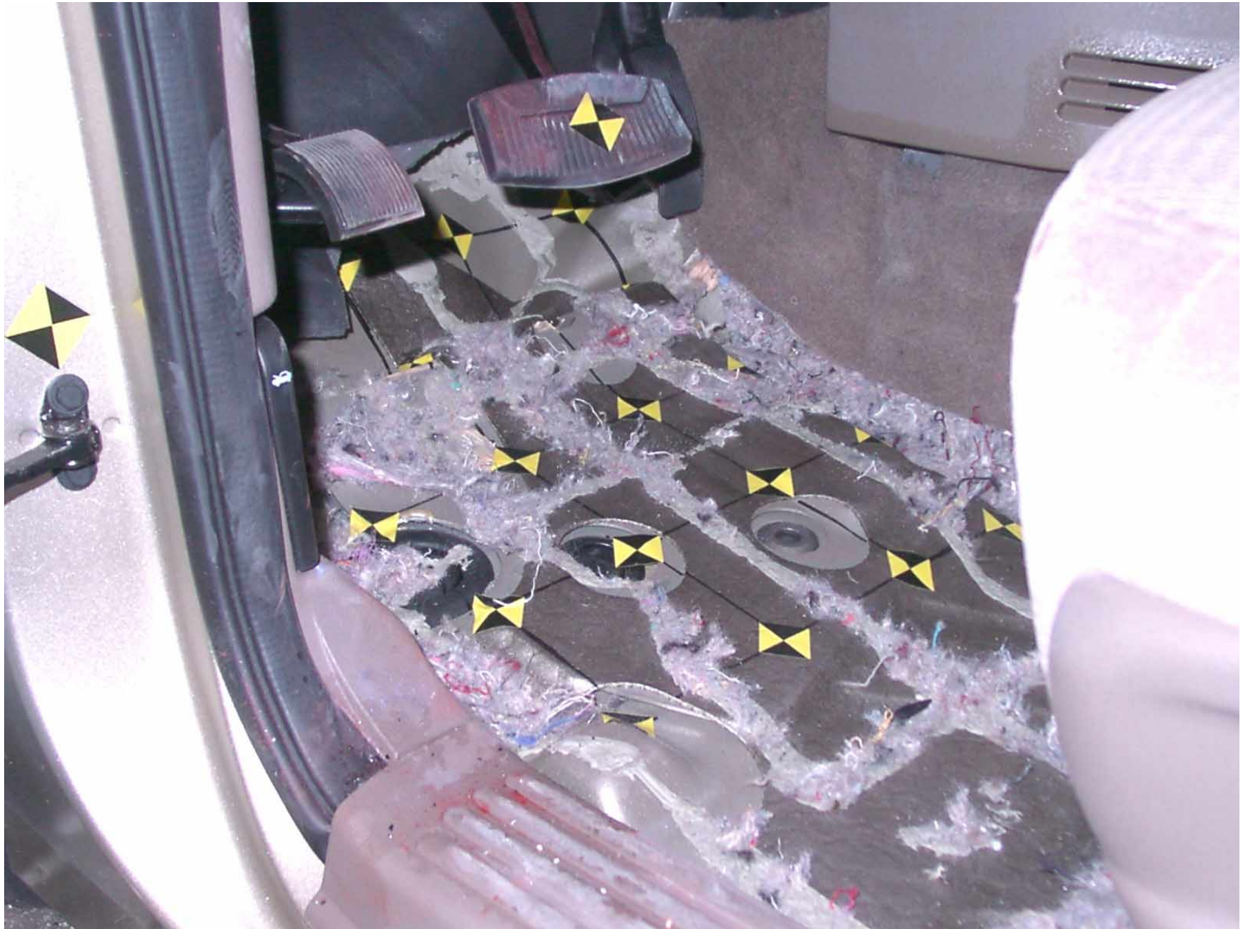
Figure A-38: Driver Side Floor Pan, Post-Test
