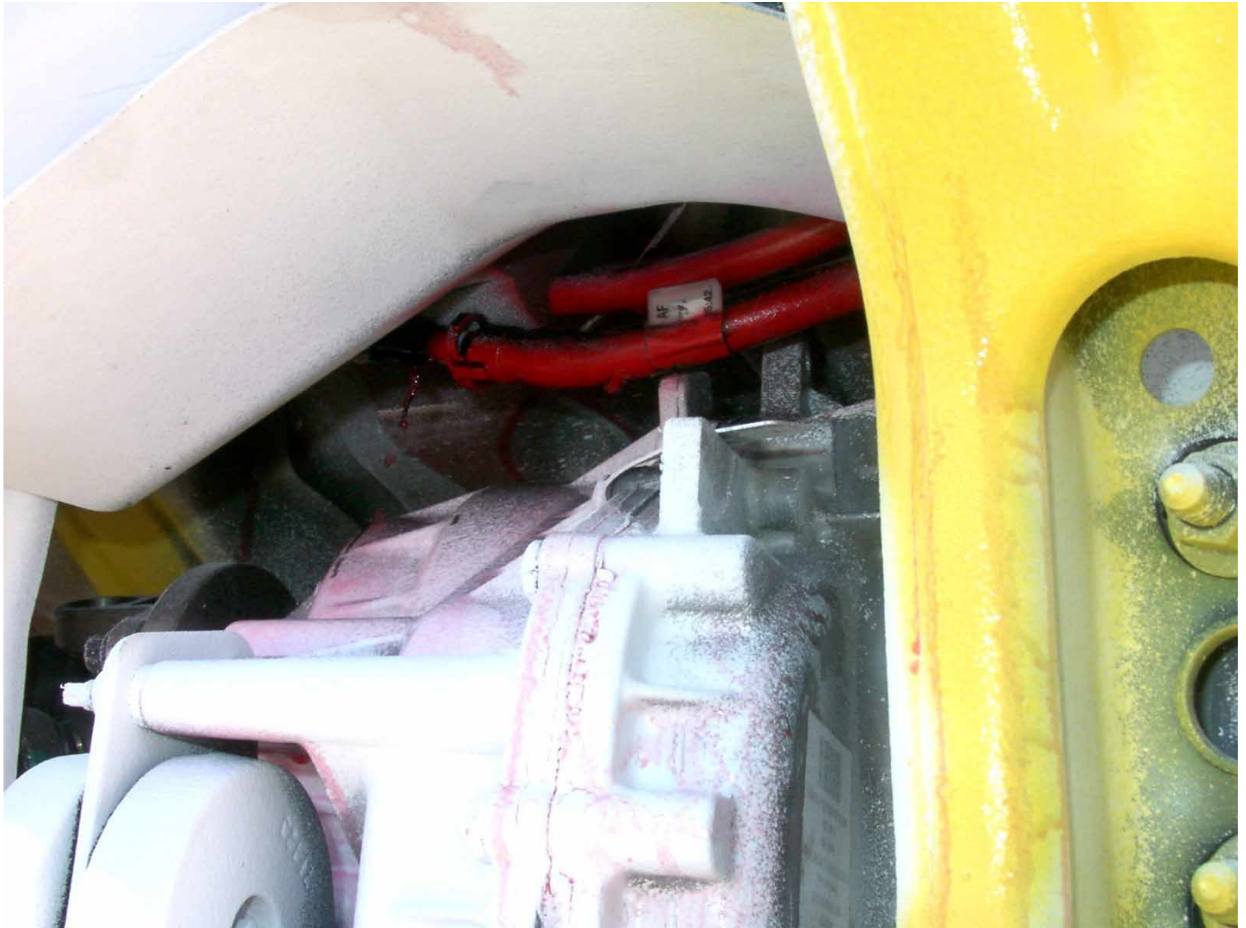
Figure A-59: Fuel System Spillage Detail
