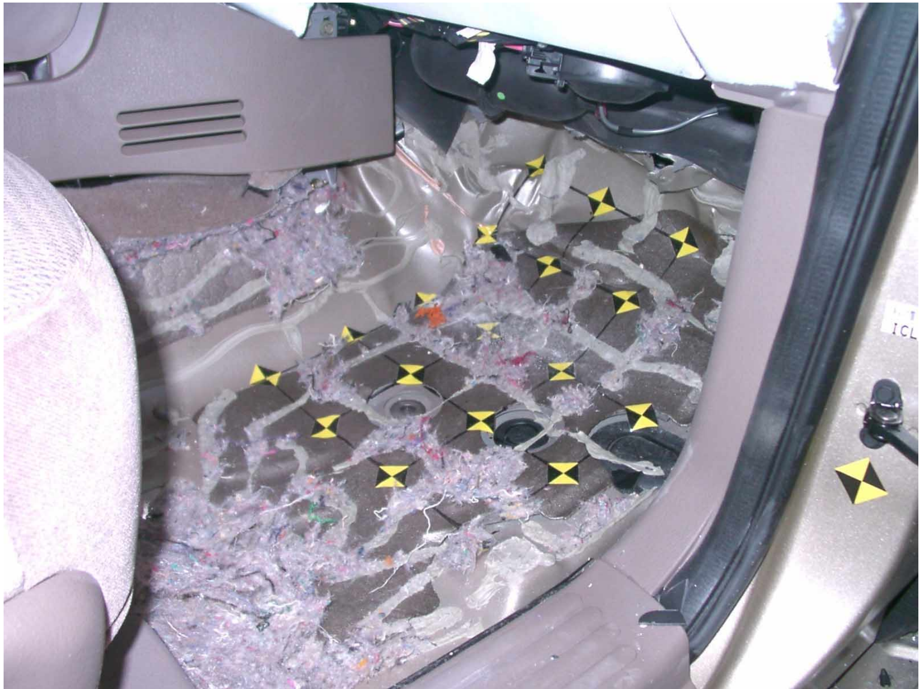
Figure A-52: Passenger Side Floor Pan, Post-Test
