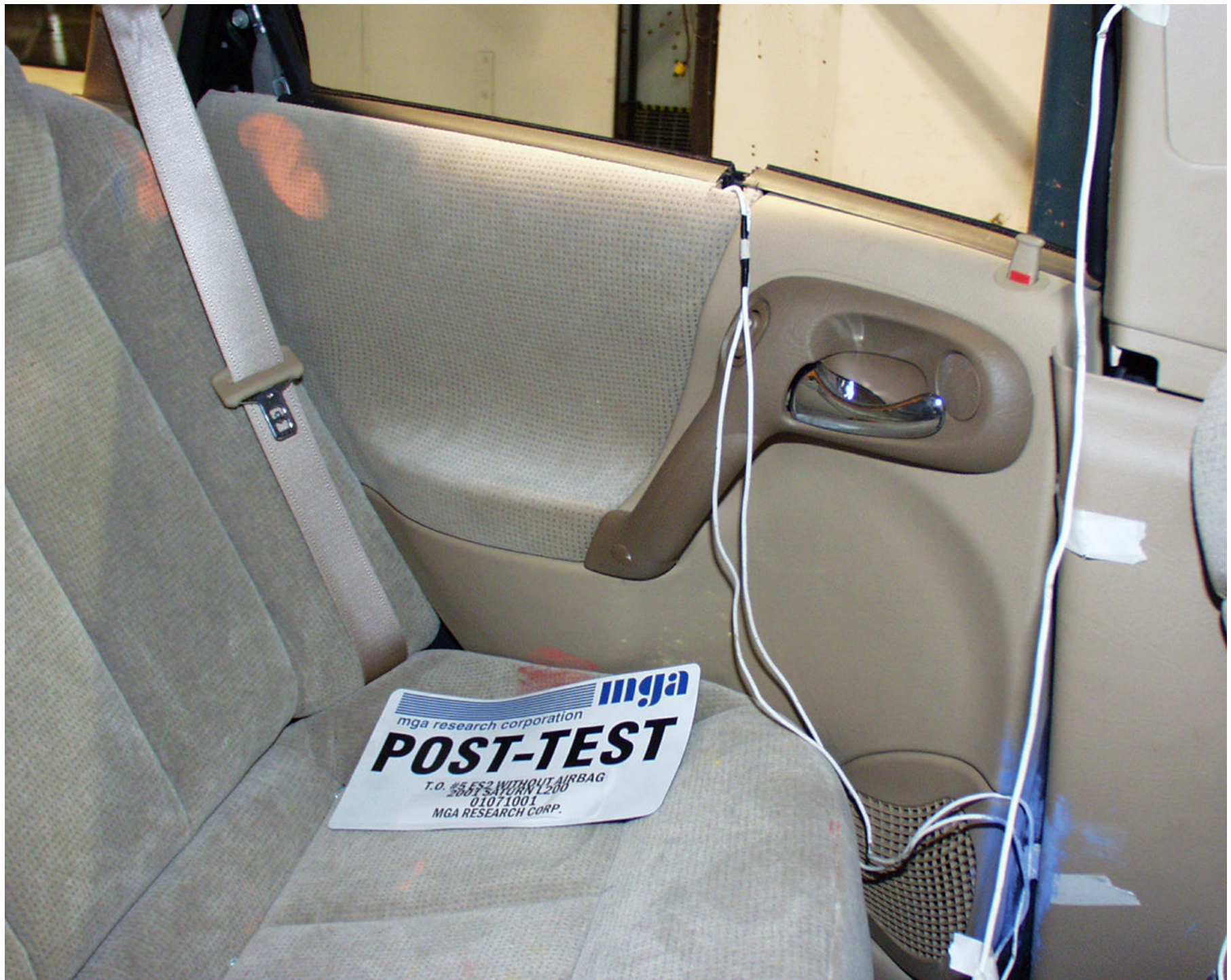
Photo No. A-31 – Post-Test Left Rear Passenger Head Contact
