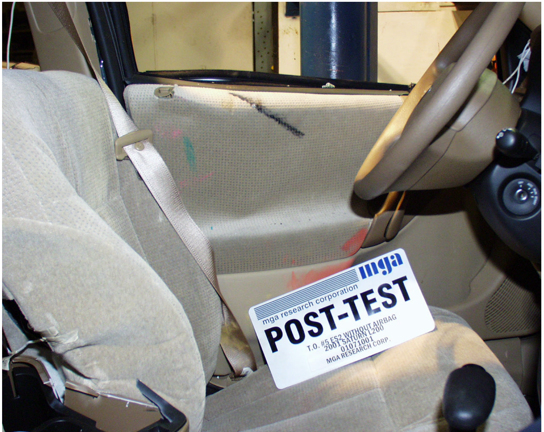
Photo No. A-30 - Post-Test Driver Contact
