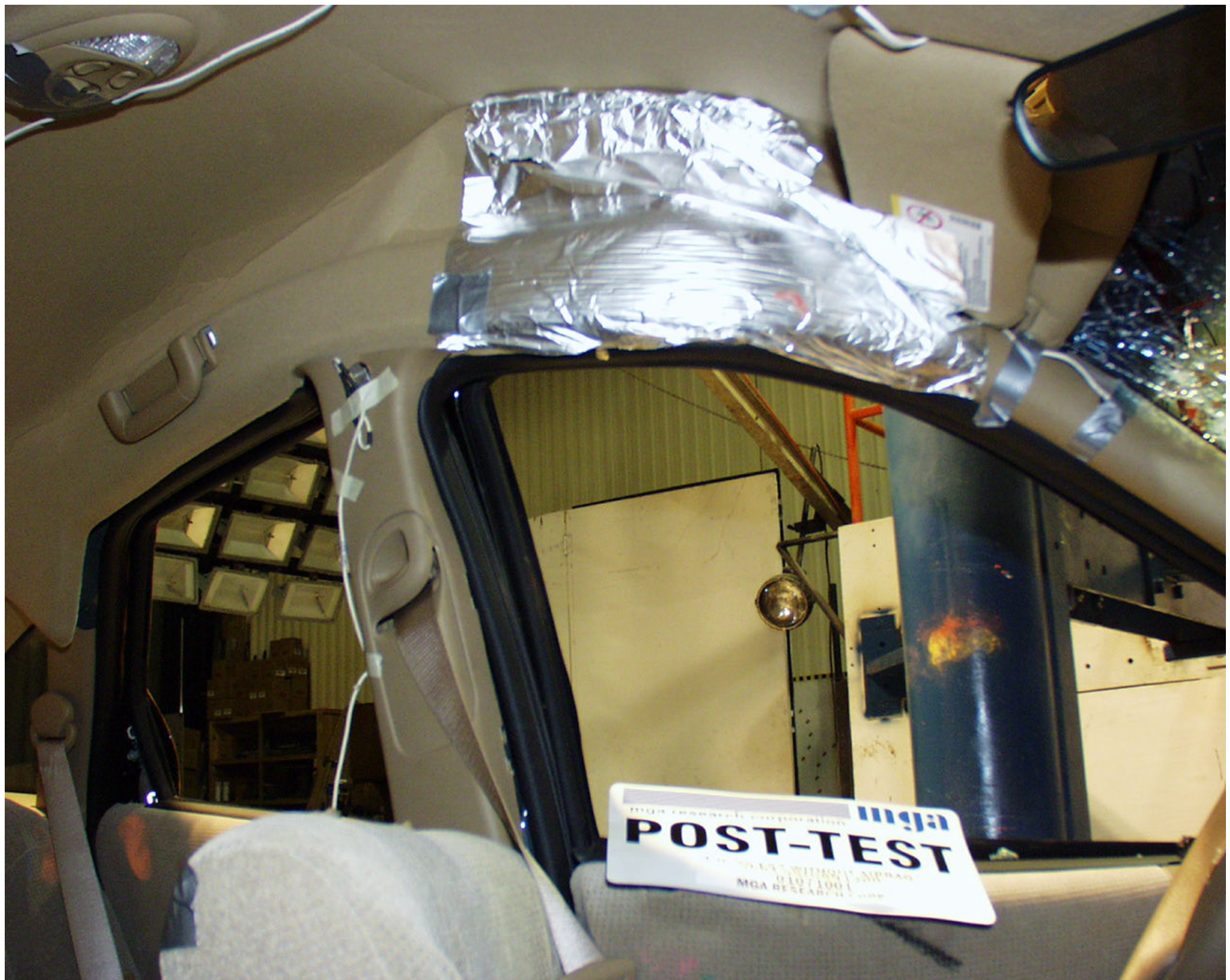
Photo No. A-29 – Post-Test Driver Head Contact
