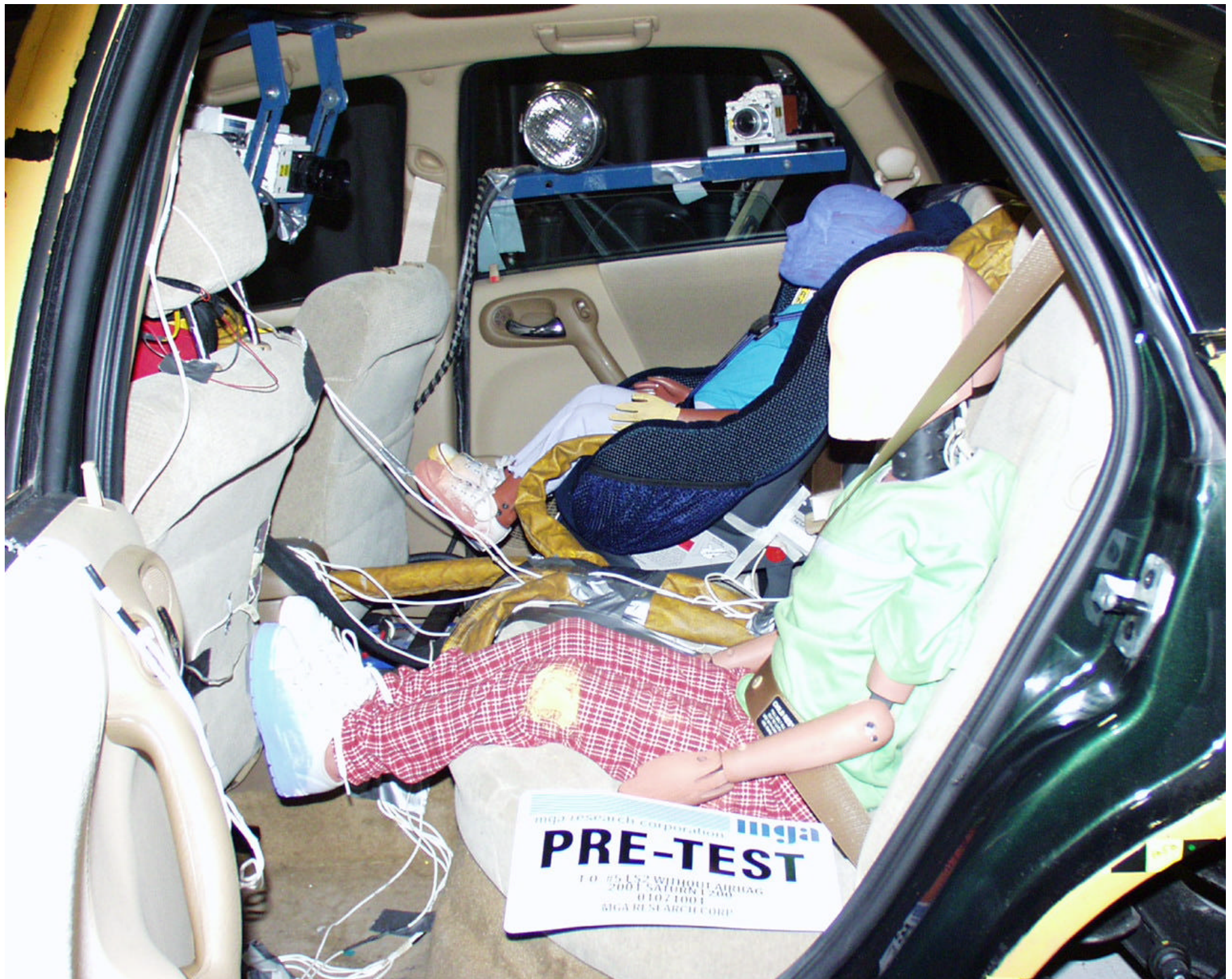
Photo No. A-24 - Pre-Test Rear Passenger Dummies Left Side View (Door Open)
