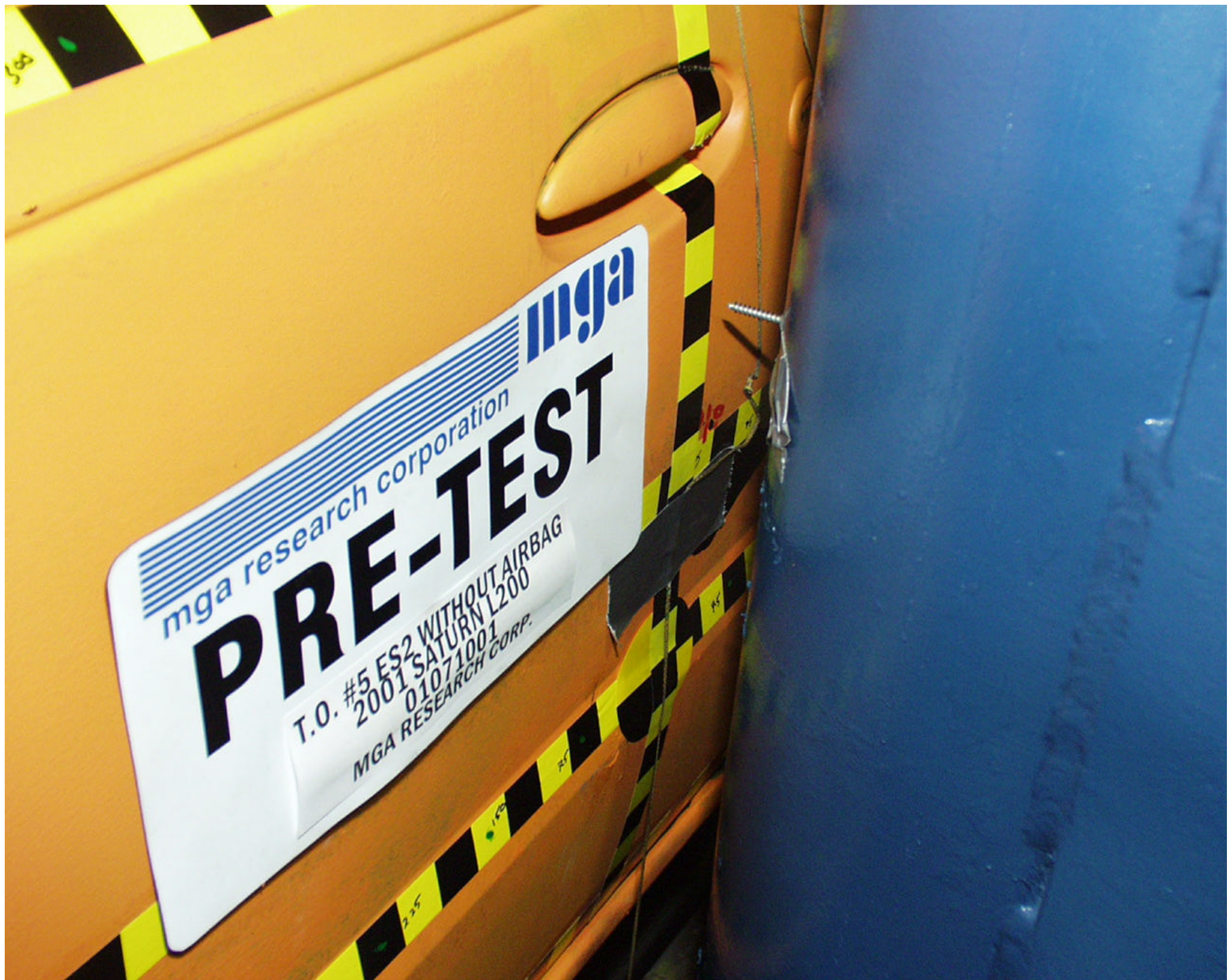
Photo No. A-27 - Pre-Test Impact Point on Vehicle
