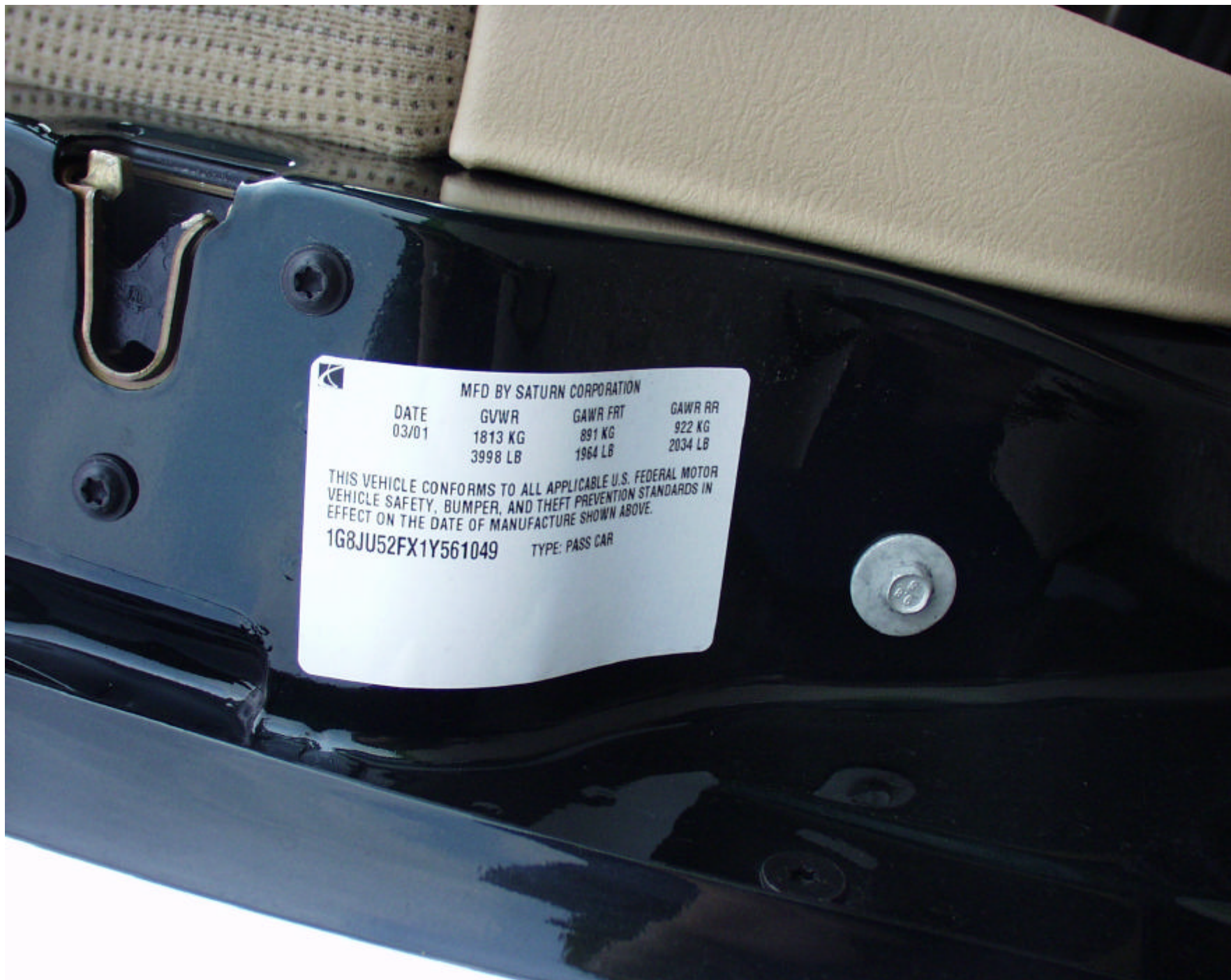
Photo No. A-33 –Vehicle Certification Label
