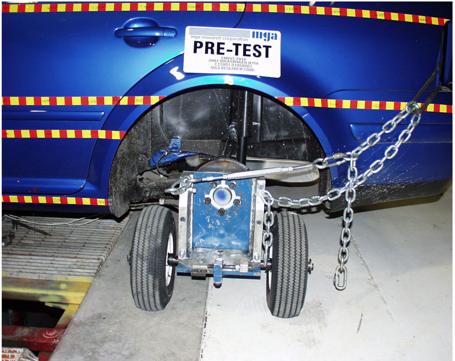
Photo No. A-30 - Pre-Test Left Rear Wheel Dolly
