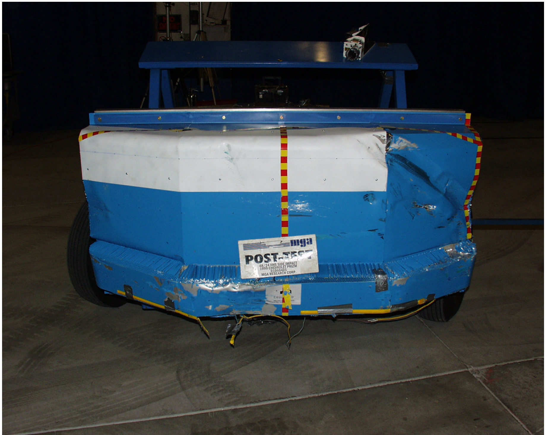
Photo No. A-16 - Post-Test MDB Front View
