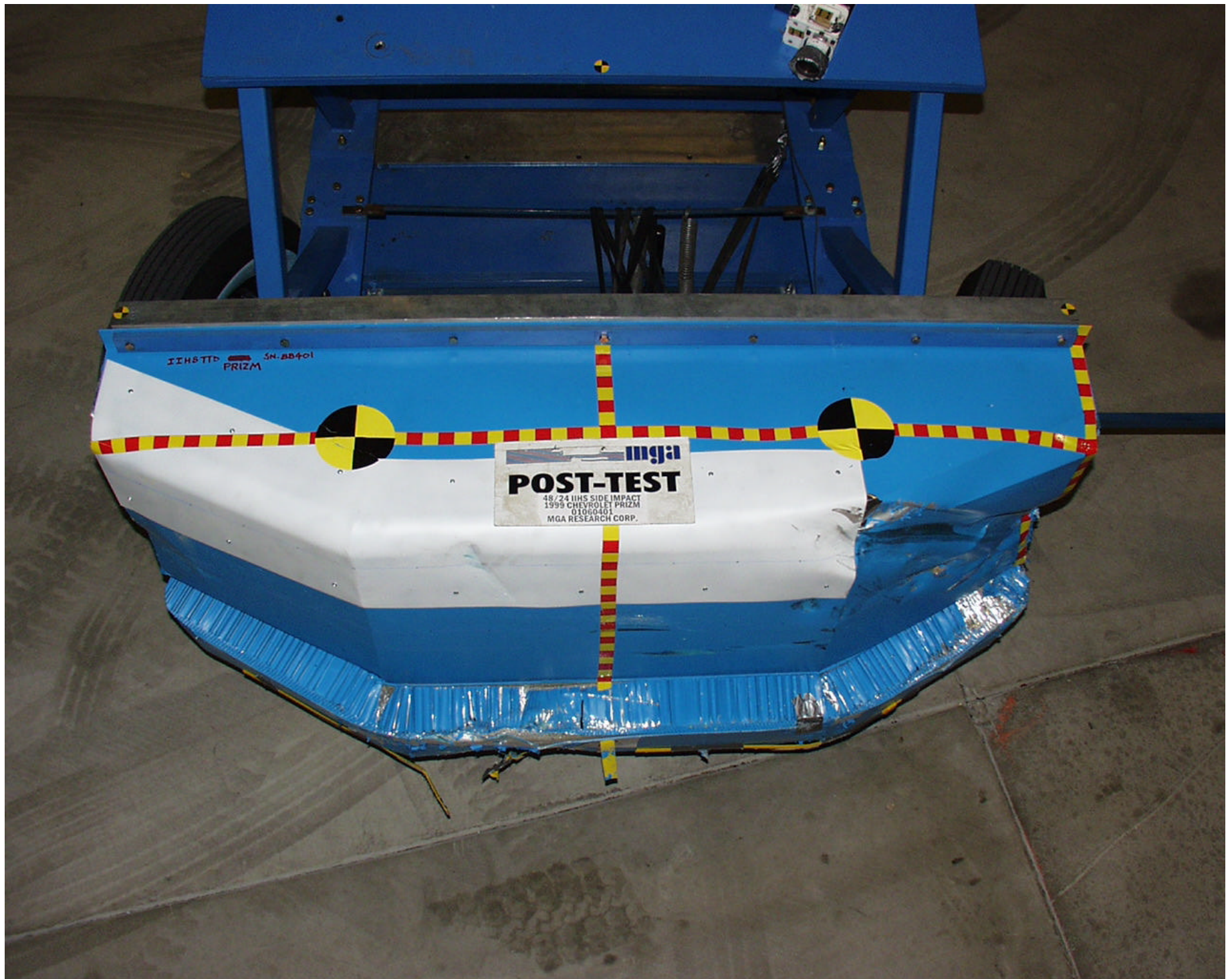
Photo No. A-14 - Post-Test MDB Top View
