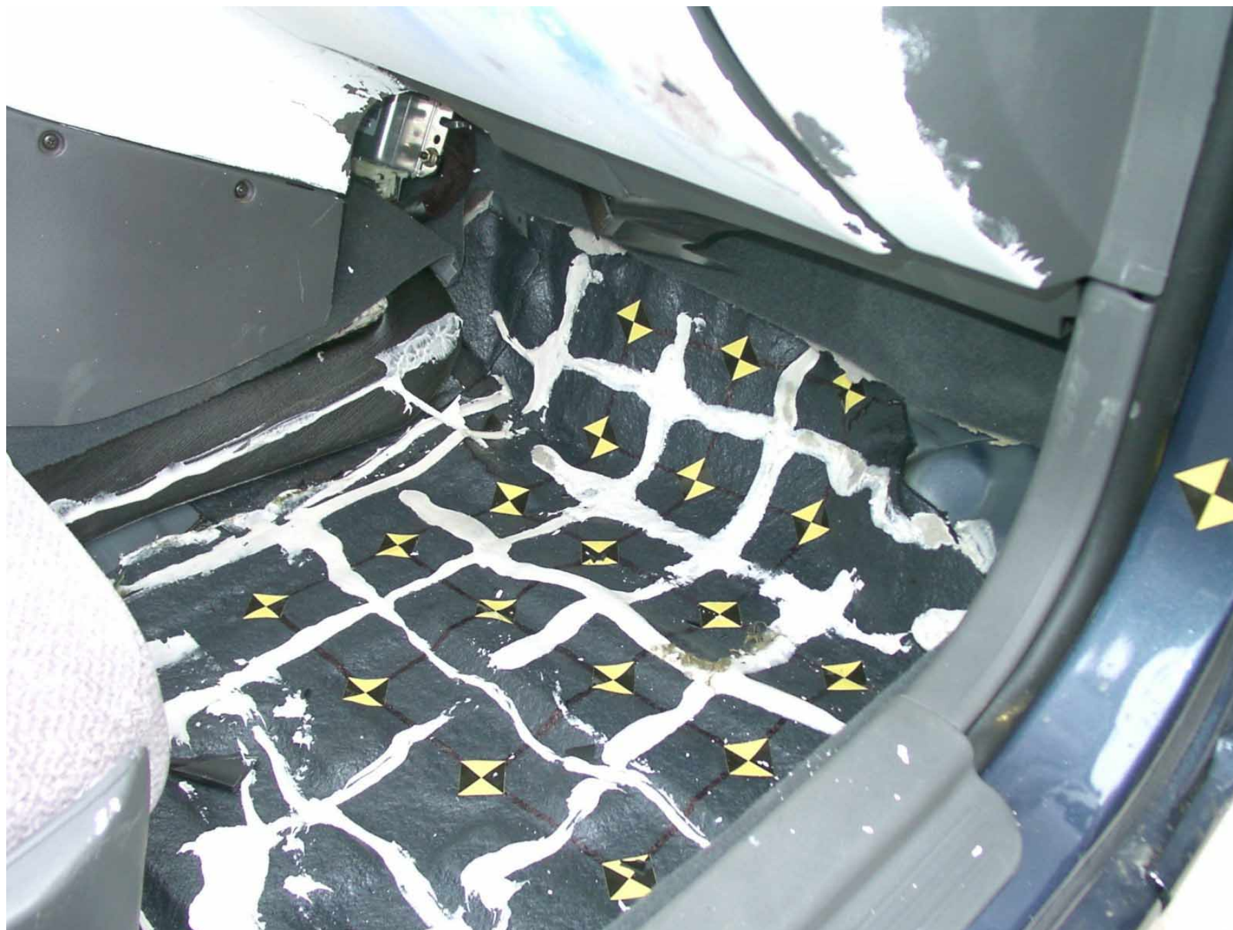
Figure A-52: Passenger Side Floor Pan, Post-Test
