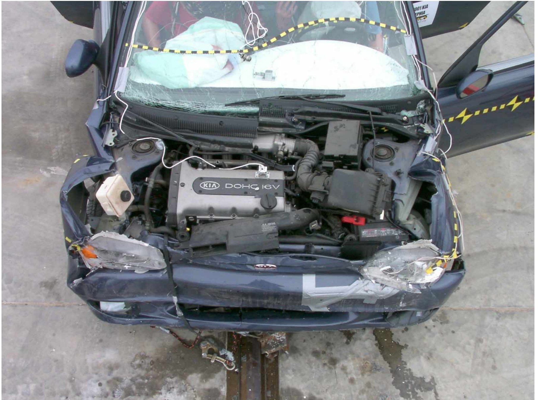
Figure A-18: Engine Compartment, Post-Test
