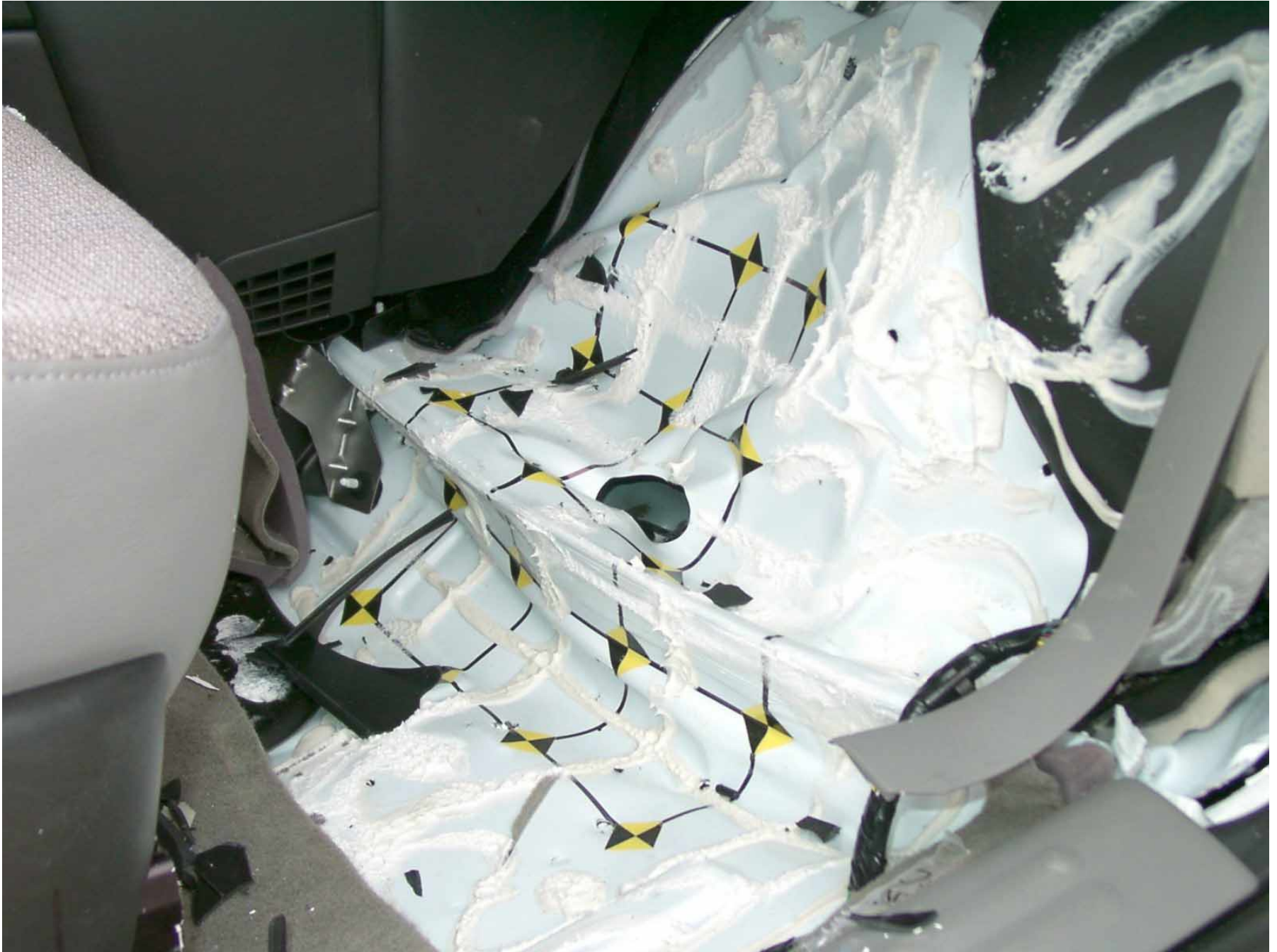
Figure A-52: Passenger Side Floor Pan, Post-Test
