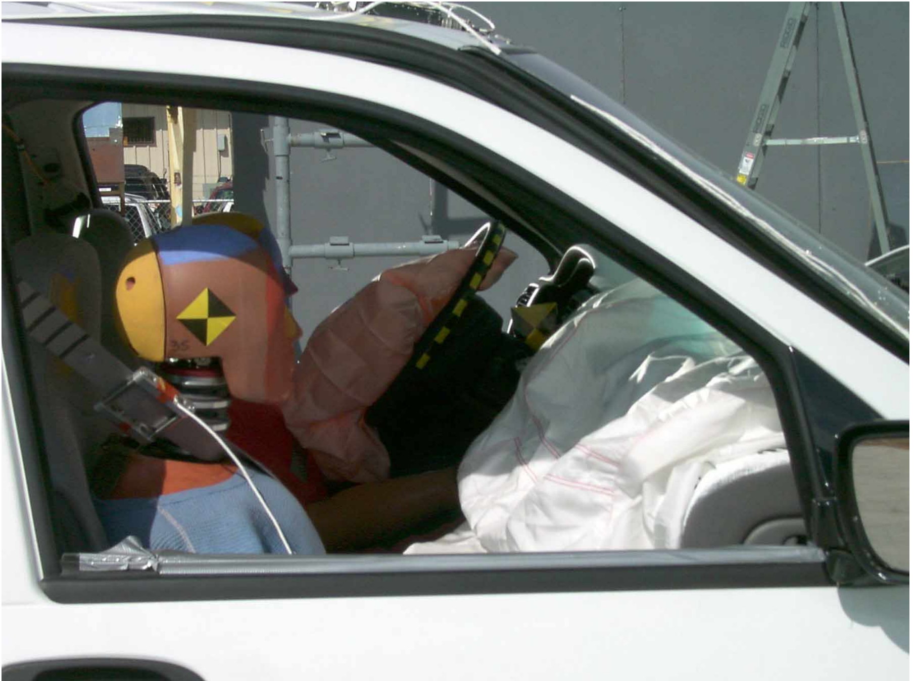
Figure A-44: Passenger Dummy Through Window, Post-Test
