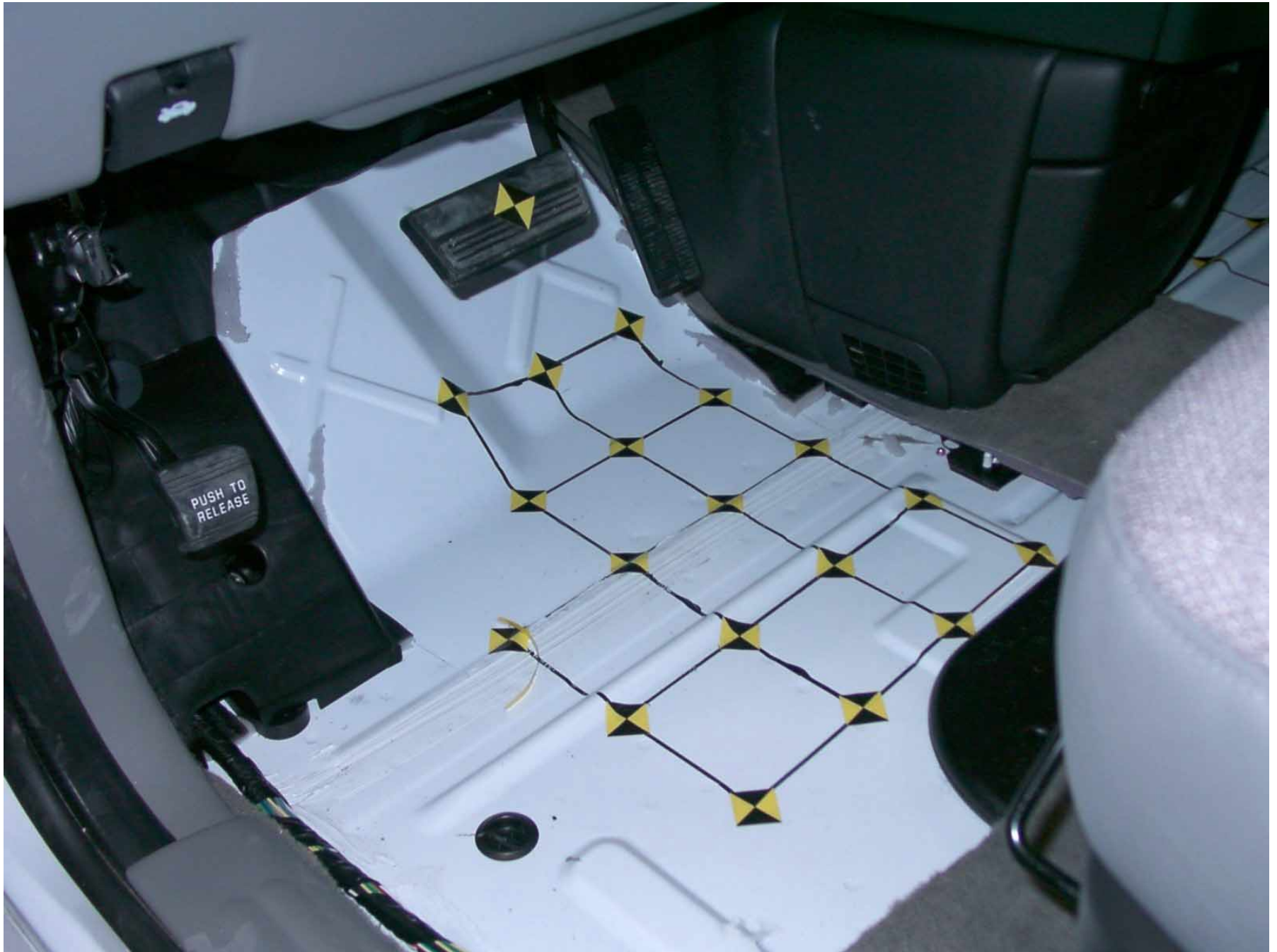
Figure A-37: Driver Side Floor Pan, Pre-Test
