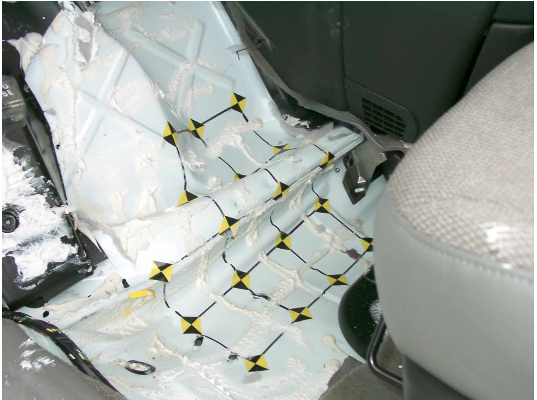
Figure A-38: Driver Side Floor Pan, Post-Test
