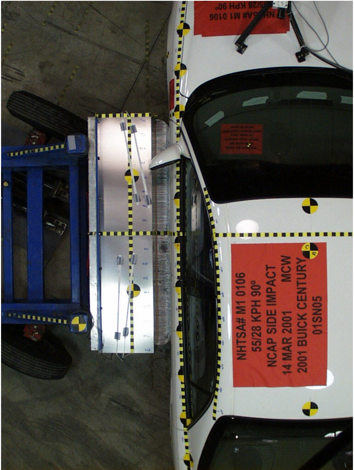
Figure A-25: PRE-TEST OVERHEAD VIEW OF MDB IN IMPACT POSITION
