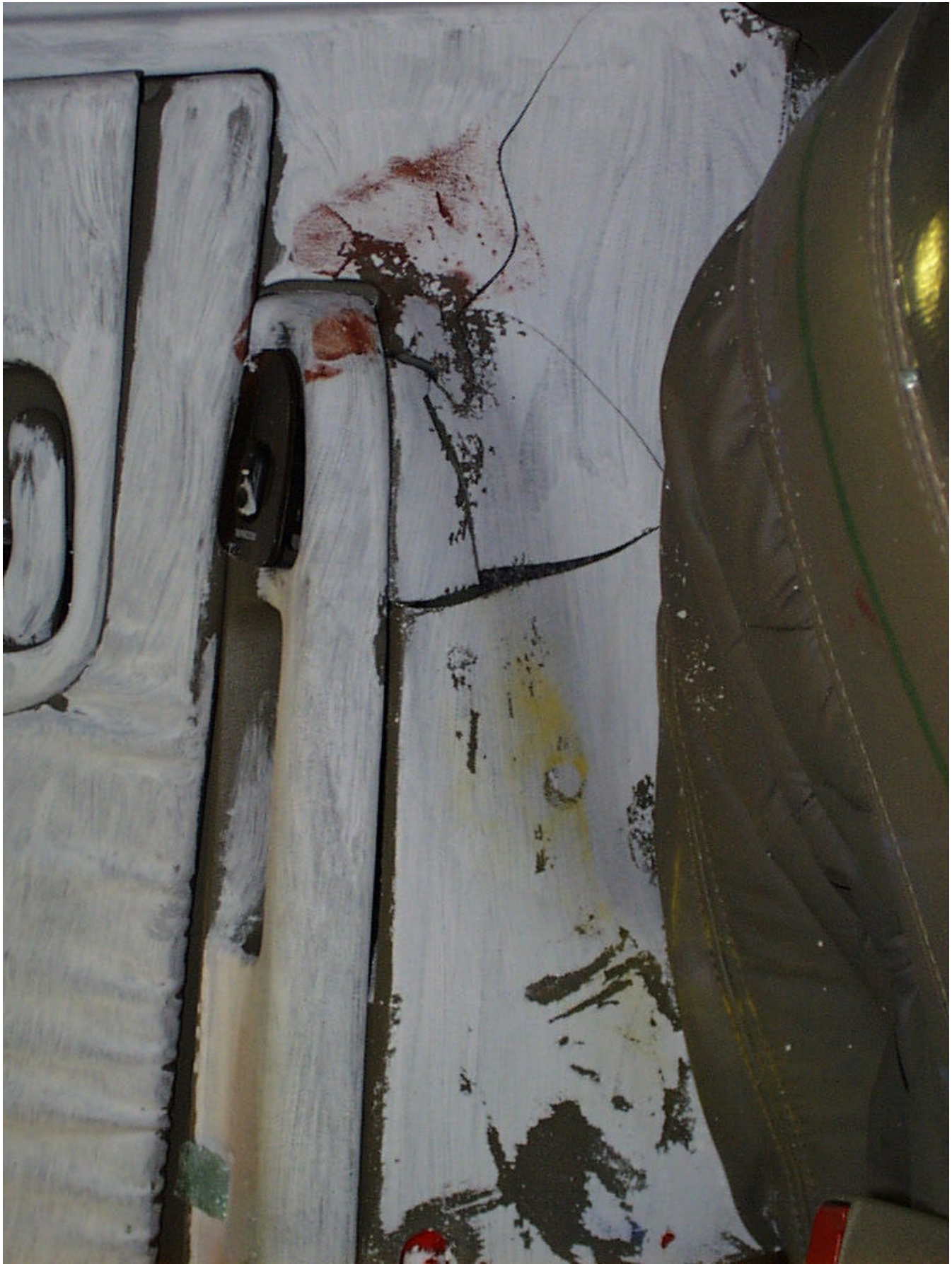
Figure A-20: POST-TEST INTERIOR OF REAR DOOR SHOWING SID IMPACT LOCATIONS
