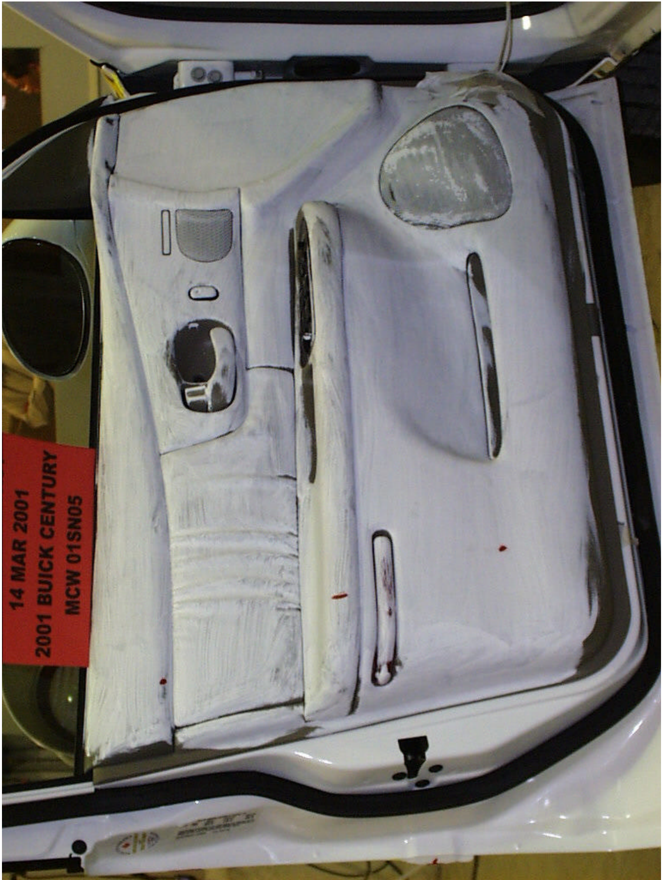
Figure A-17: PRE-TEST INTERIOR OF FRONT DOOR
