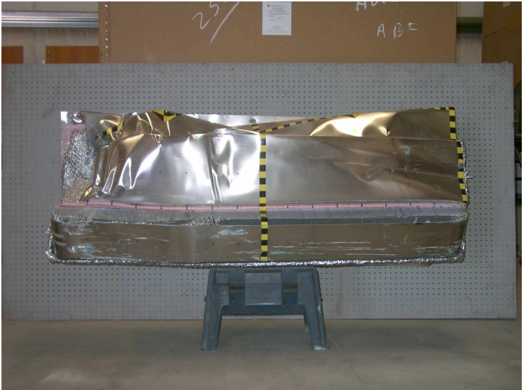
Figure A-28: Front View of Deformable Barrier, Post-Test
