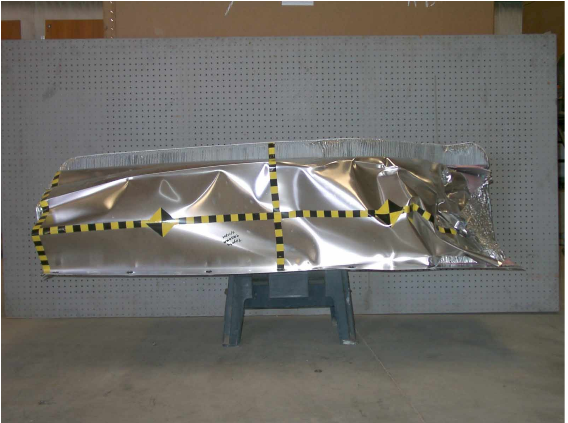
Figure A-30: Top View Deformable Barrier, Post-Test
