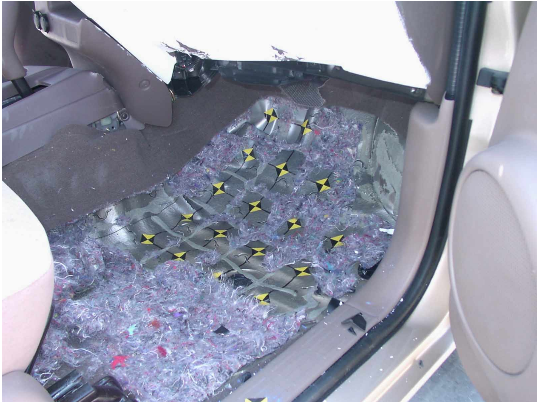
Figure A-52: Passenger Side Floor Pan, Post-Test
