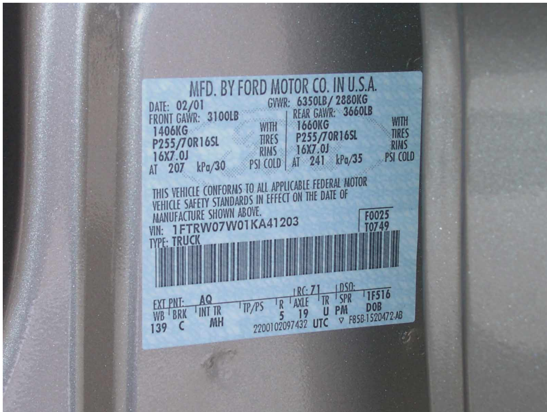
Figure A-4: Vehicle Tire Label
