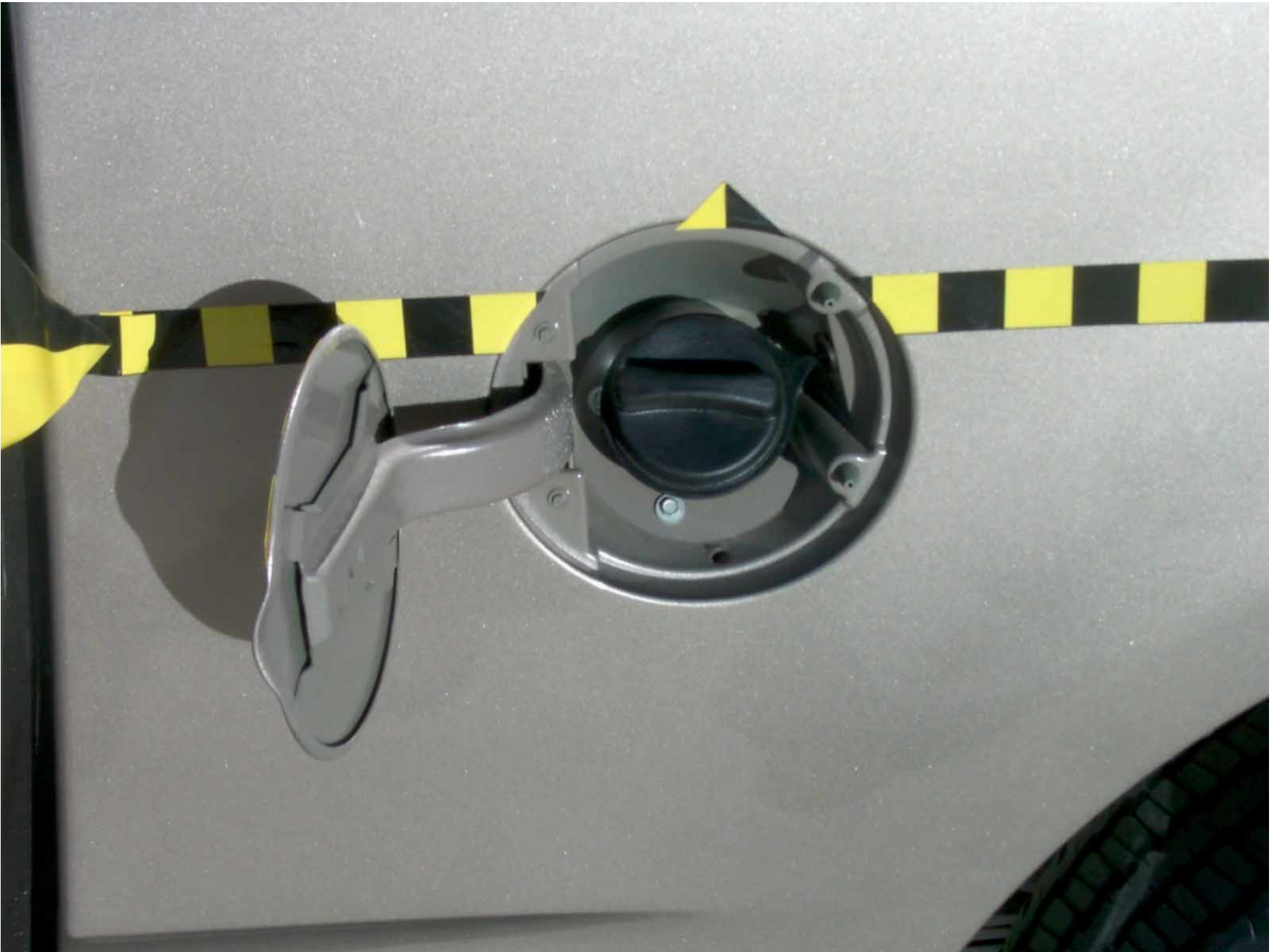
Figure A-20: Fuel Cap, Post-Test
