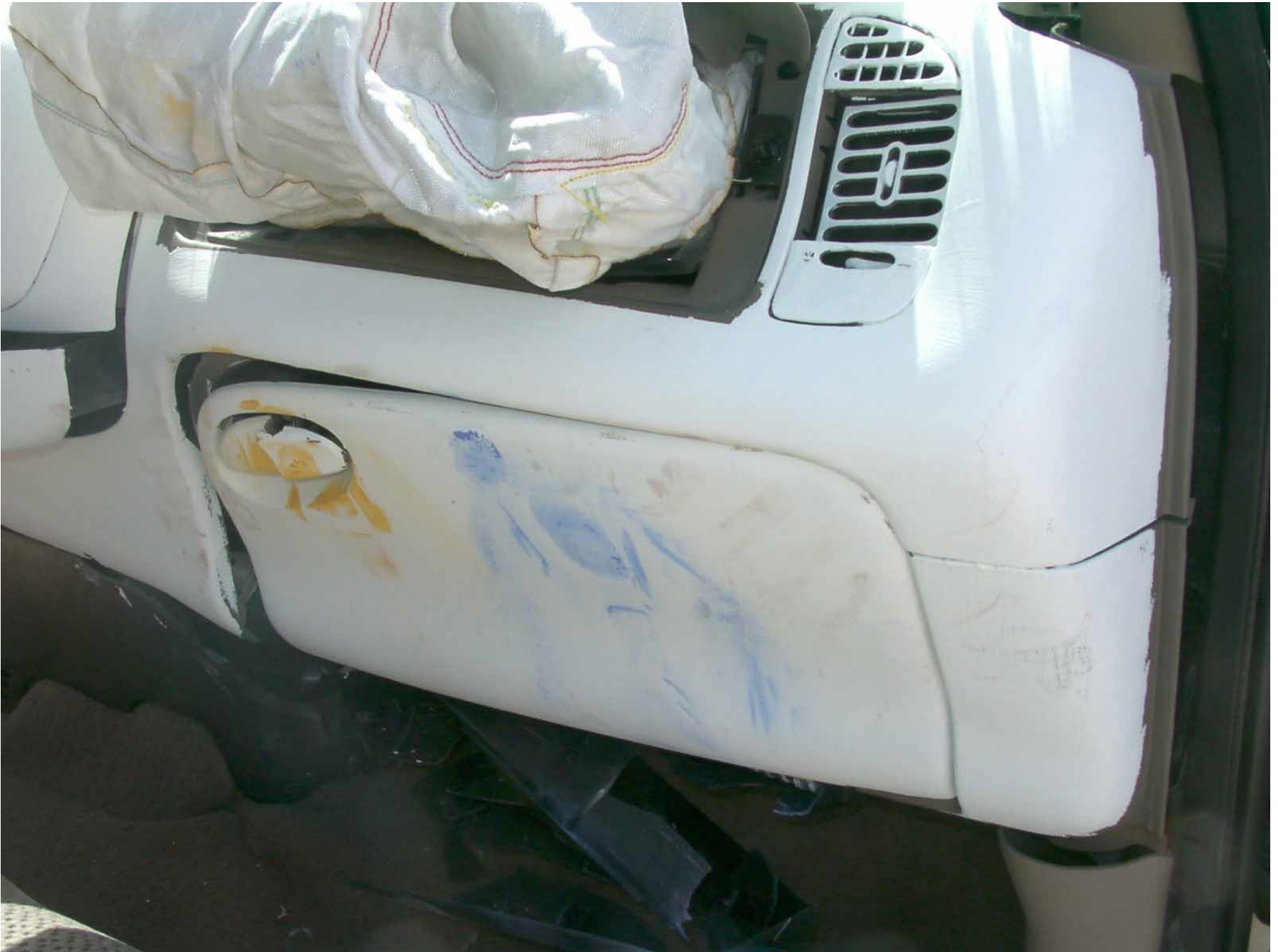
Figure A-54: Passenger Side Knee Bolster, Post-Test
