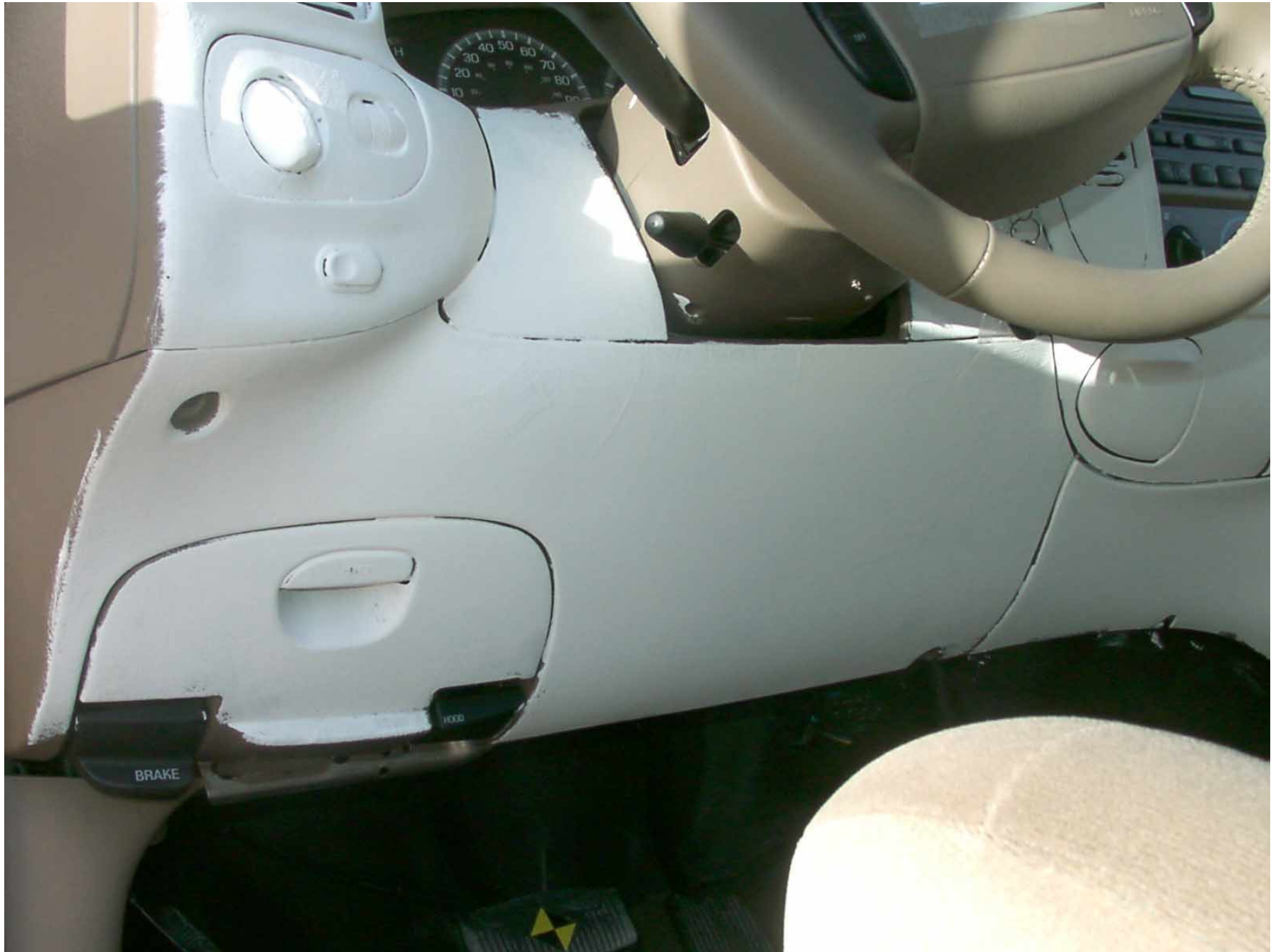
Figure A-35: Driver Side Knee Bolster, Pre-Test
