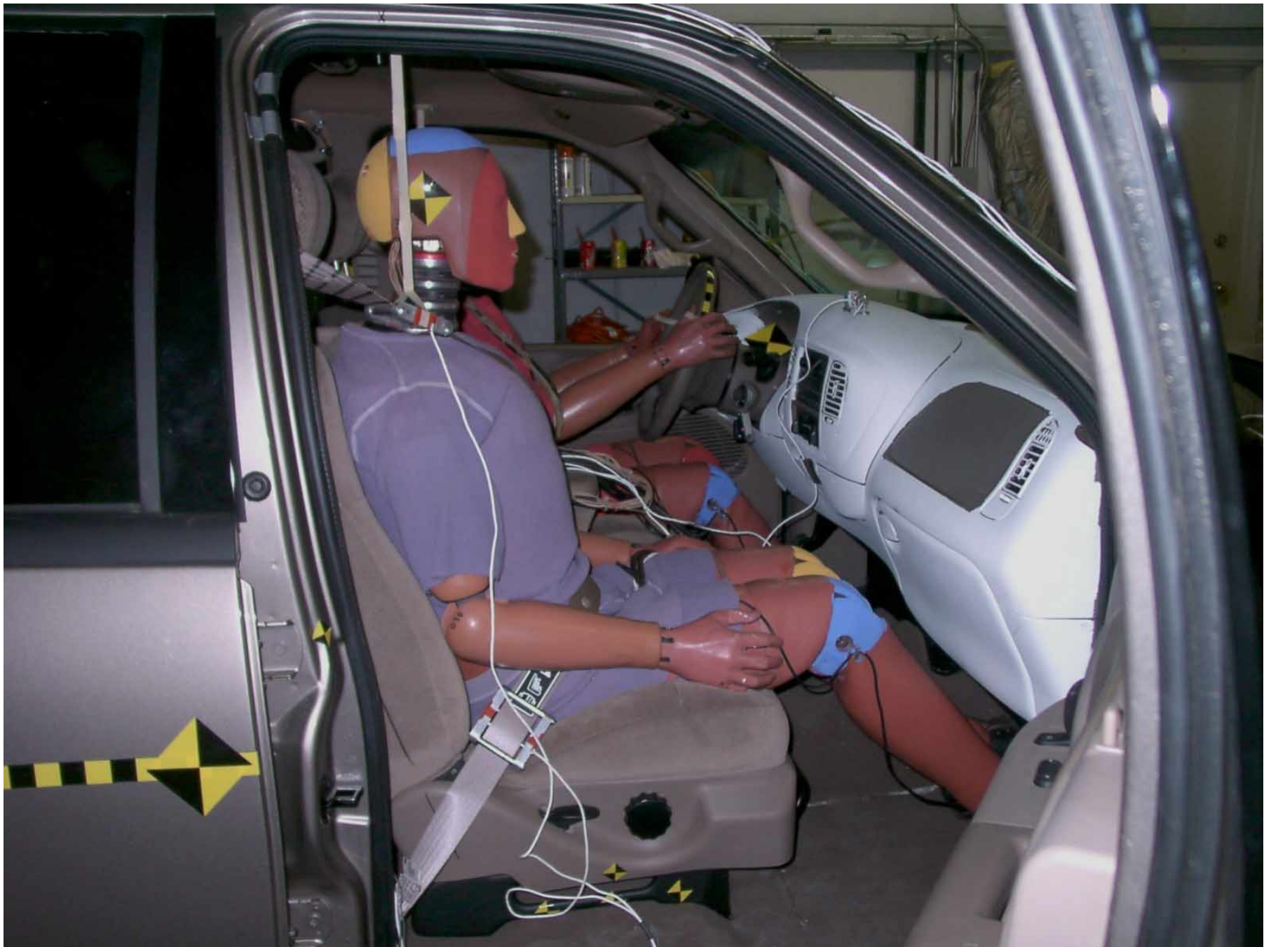
Figure A-47: Passenger Dummy 90° To Vehicle, Pre-Test
