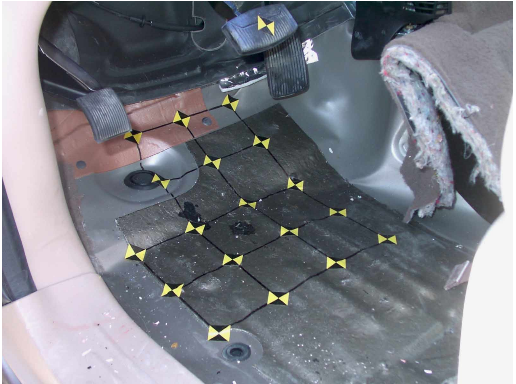
Figure A-38: Driver Side Floor Pan, Post-Test
