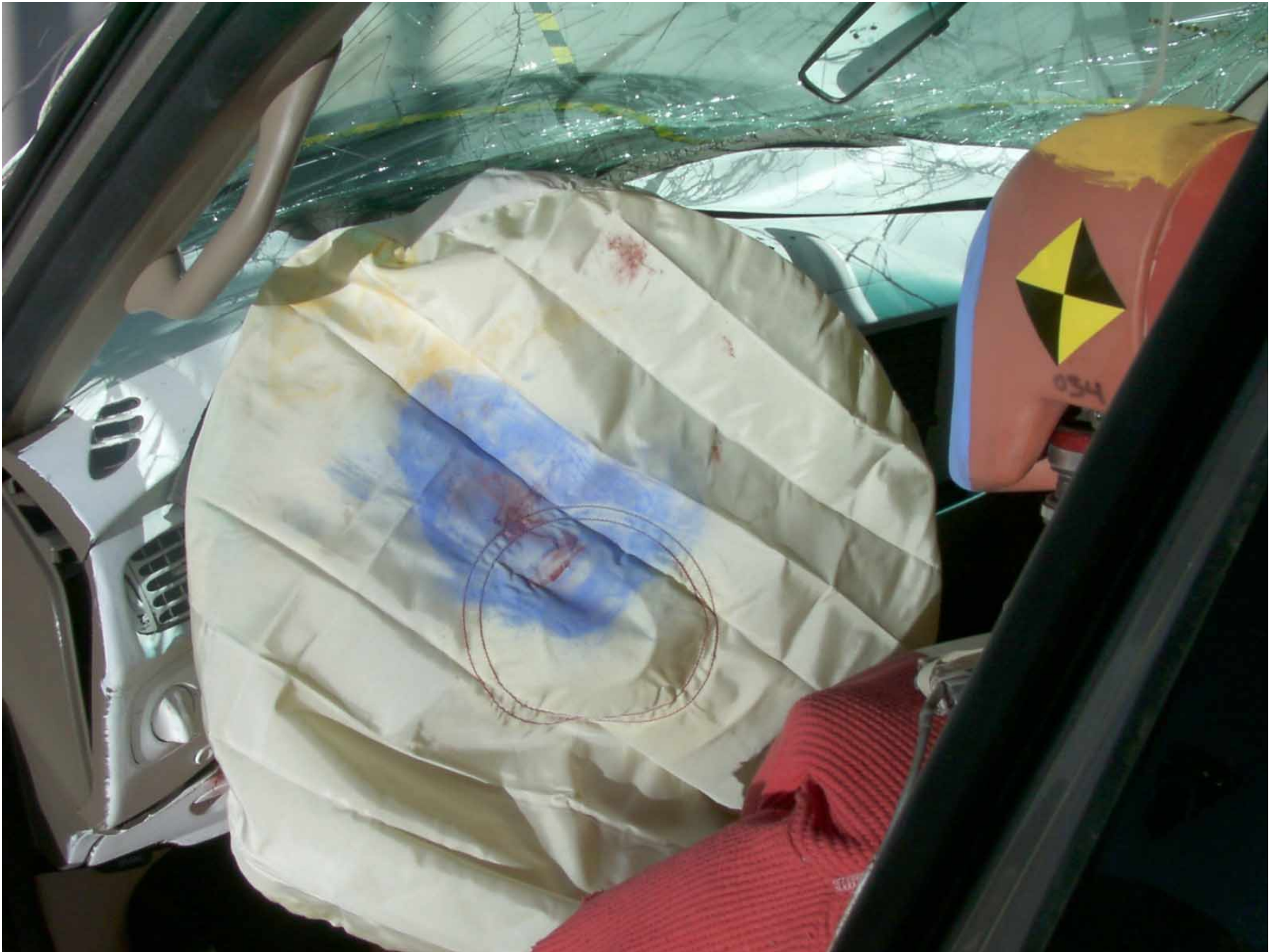
Figure A-40: Driver Dummy Contact, Post-Test
