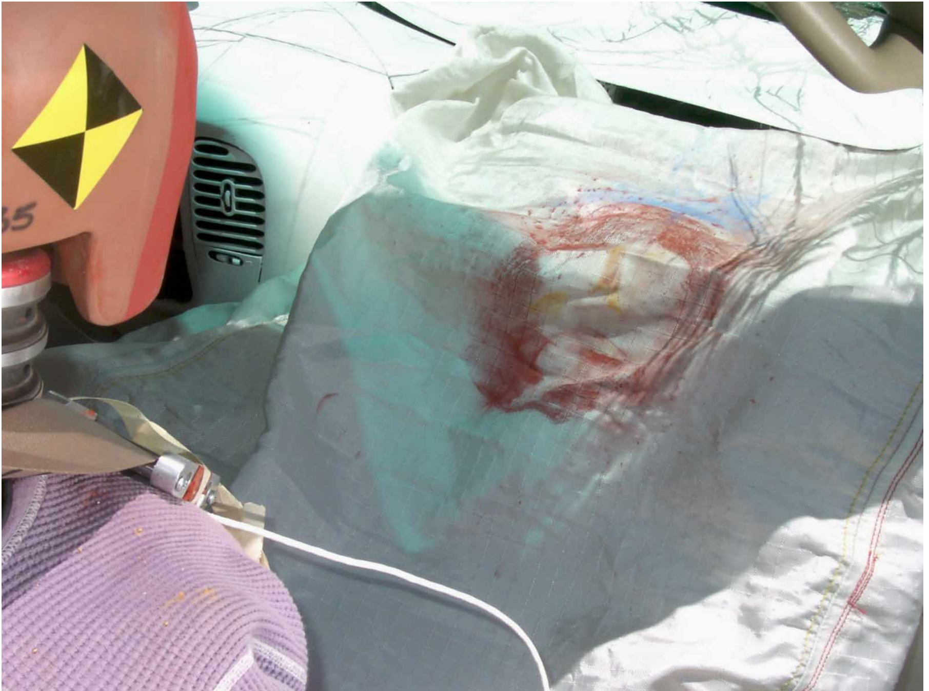
Figure A-56: Passenger Dummy Contact, Post-Test
