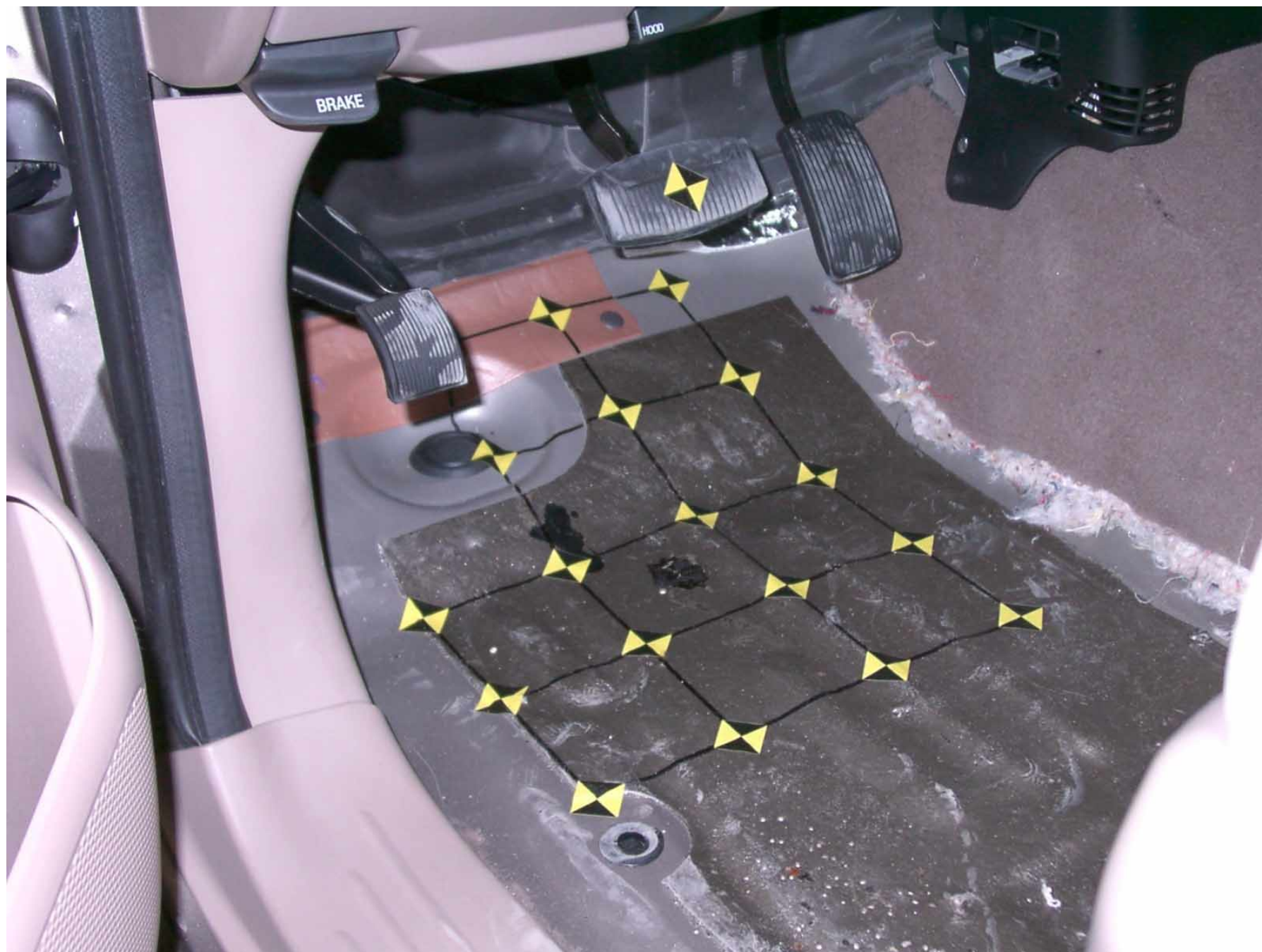
Figure A-37: Driver Side Floor Pan, Pre-Test
