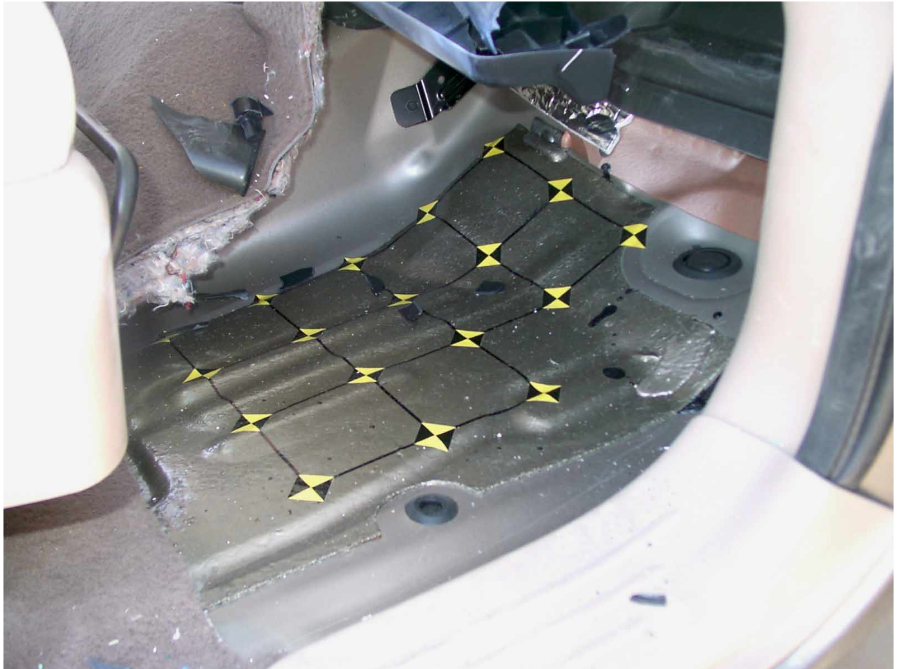
Figure A-52: Passenger Side Floor Pan, Post-Test
