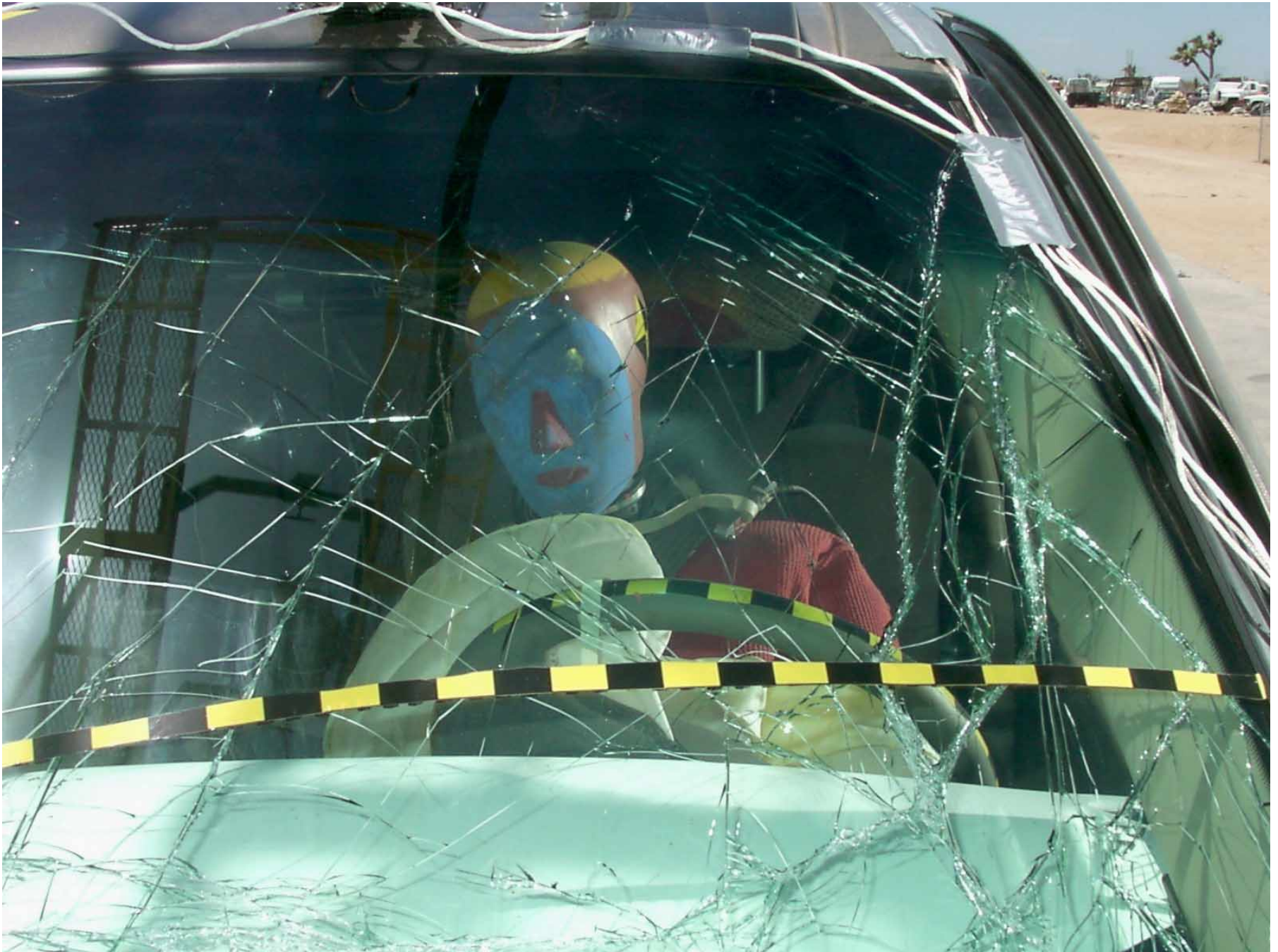
Figure A-26: Driver Dummy Front View, Post-Test
