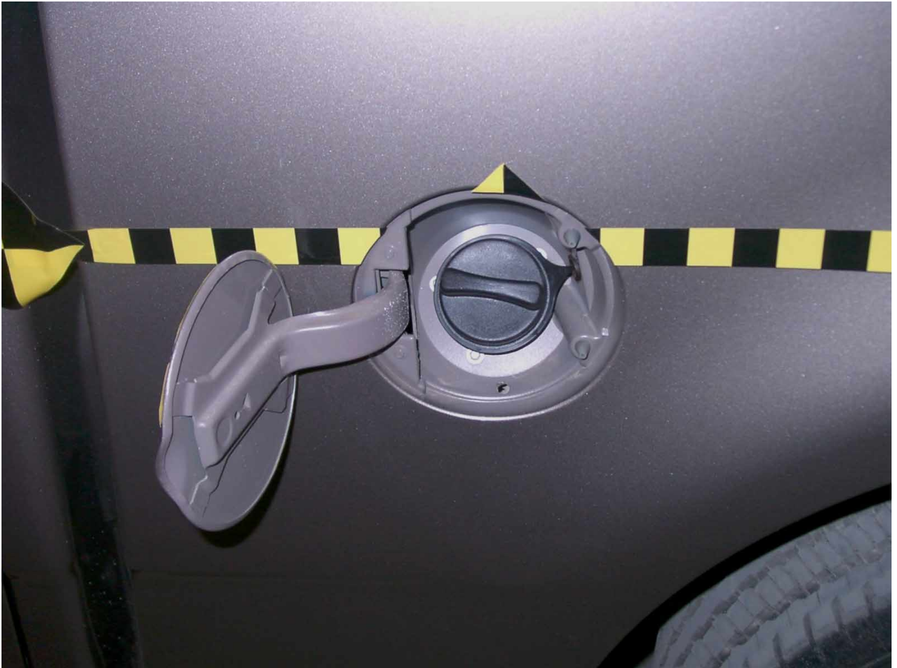
Figure A-19: Fuel Cap, Pre-test
