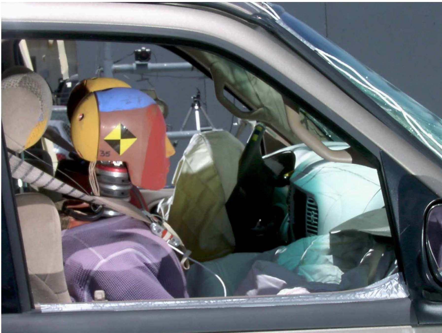
Figure A-44: Passenger Dummy Through Window, Post-Test
