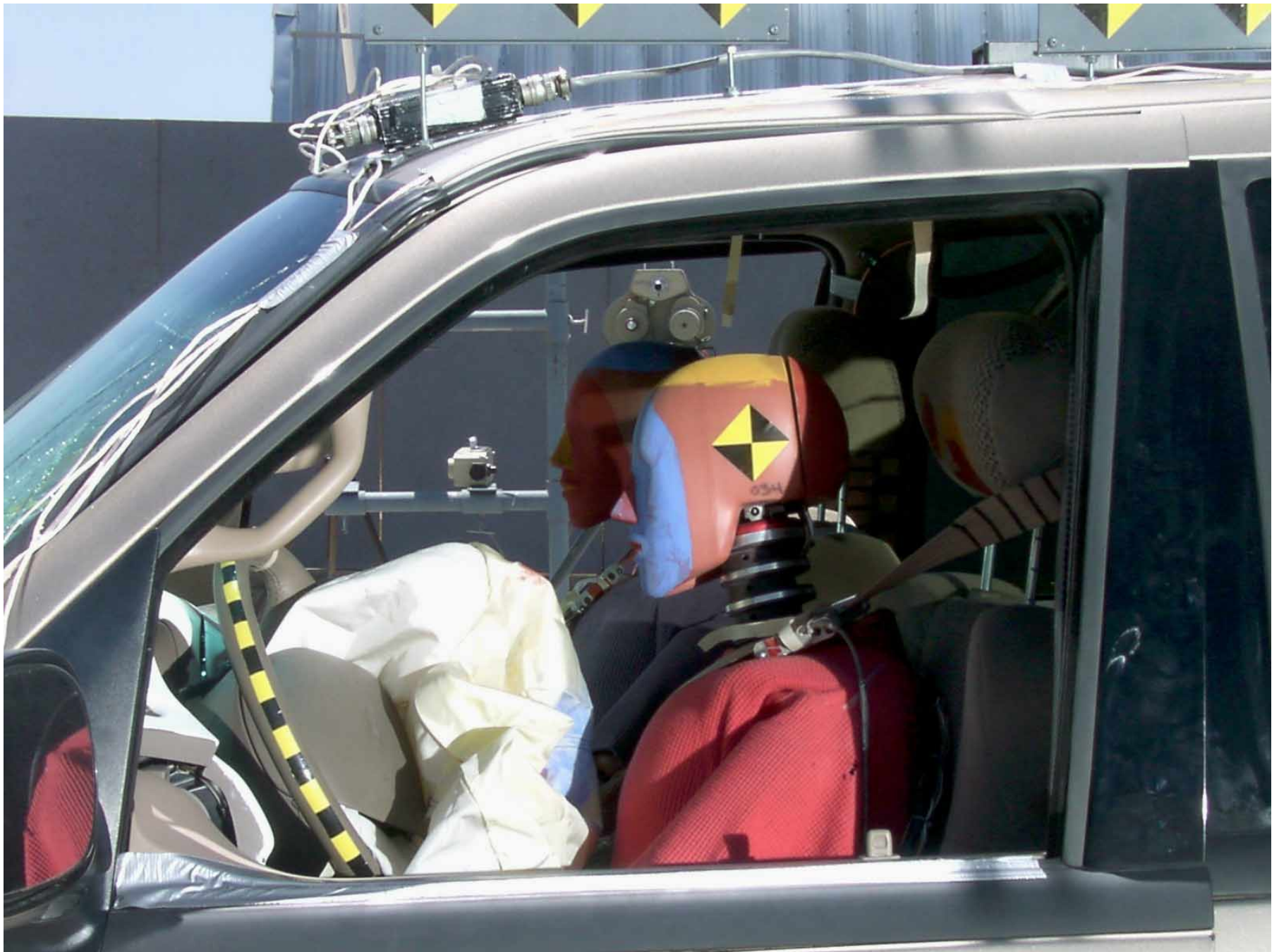
Figure A-28: Driver Dummy Through Window, Post-Test
