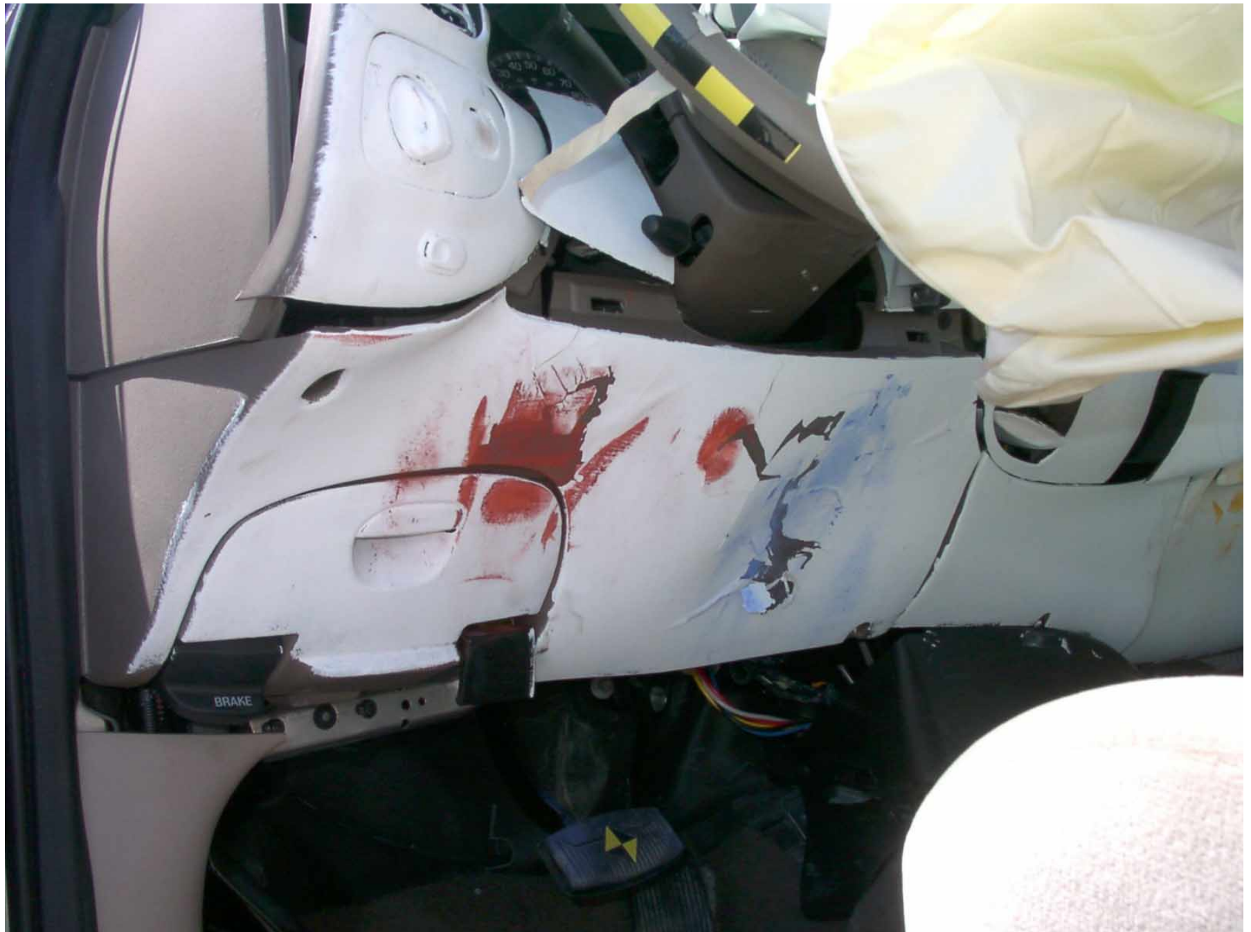
Figure A-36: Driver Side Knee Bolster, Post-Test
