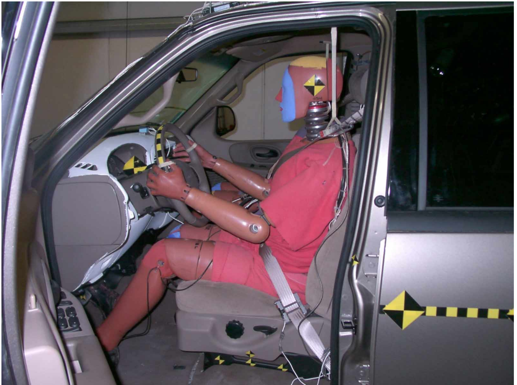
Figure A-31: Driver Dummy 90° To Vehicle, Pre-Test
