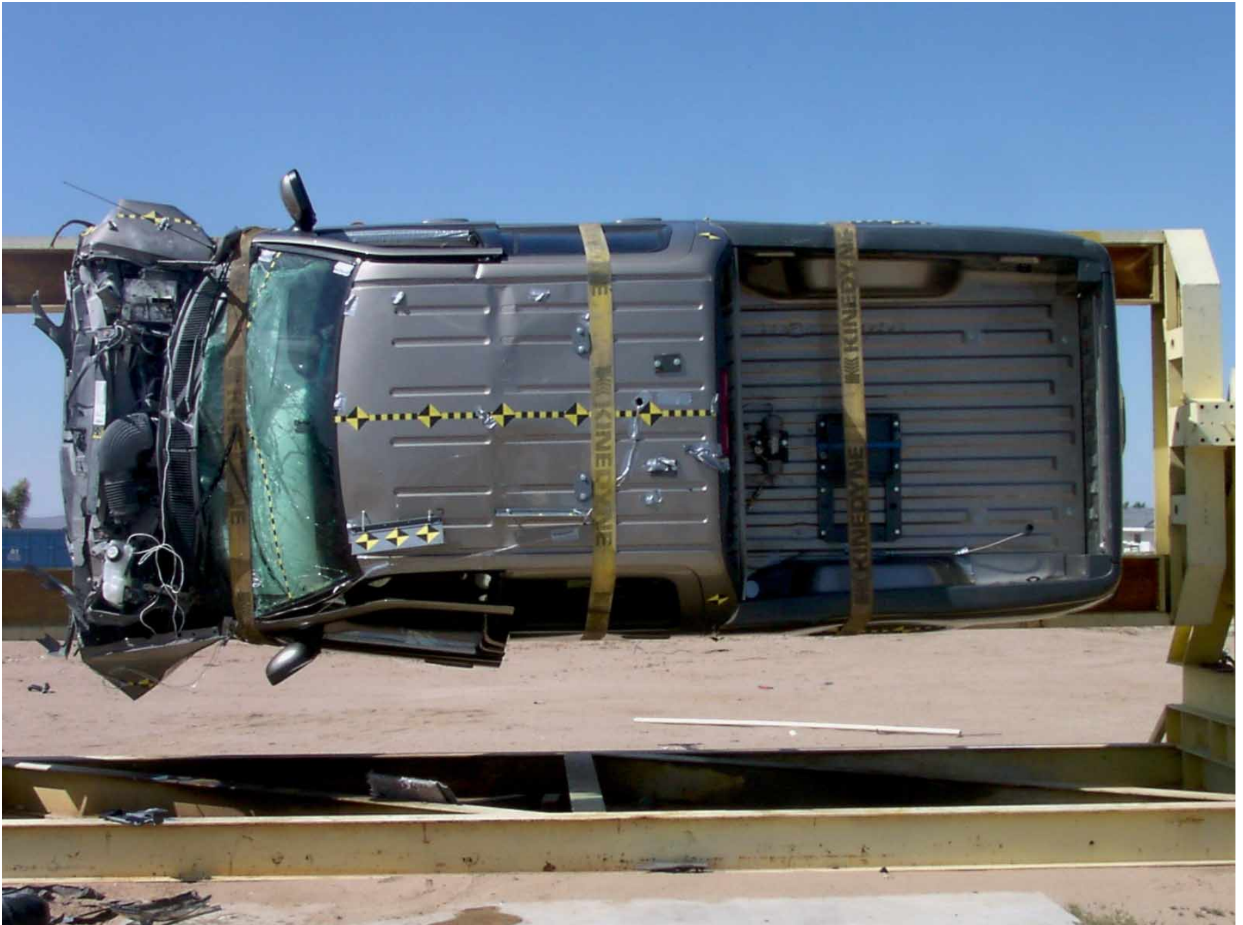
Figure A-57: Vehicle on Rollover Device
