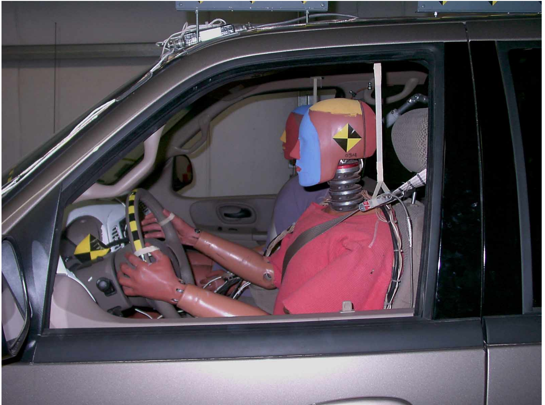
Figure A-27: Driver Dummy Through Window, Pre-Test
