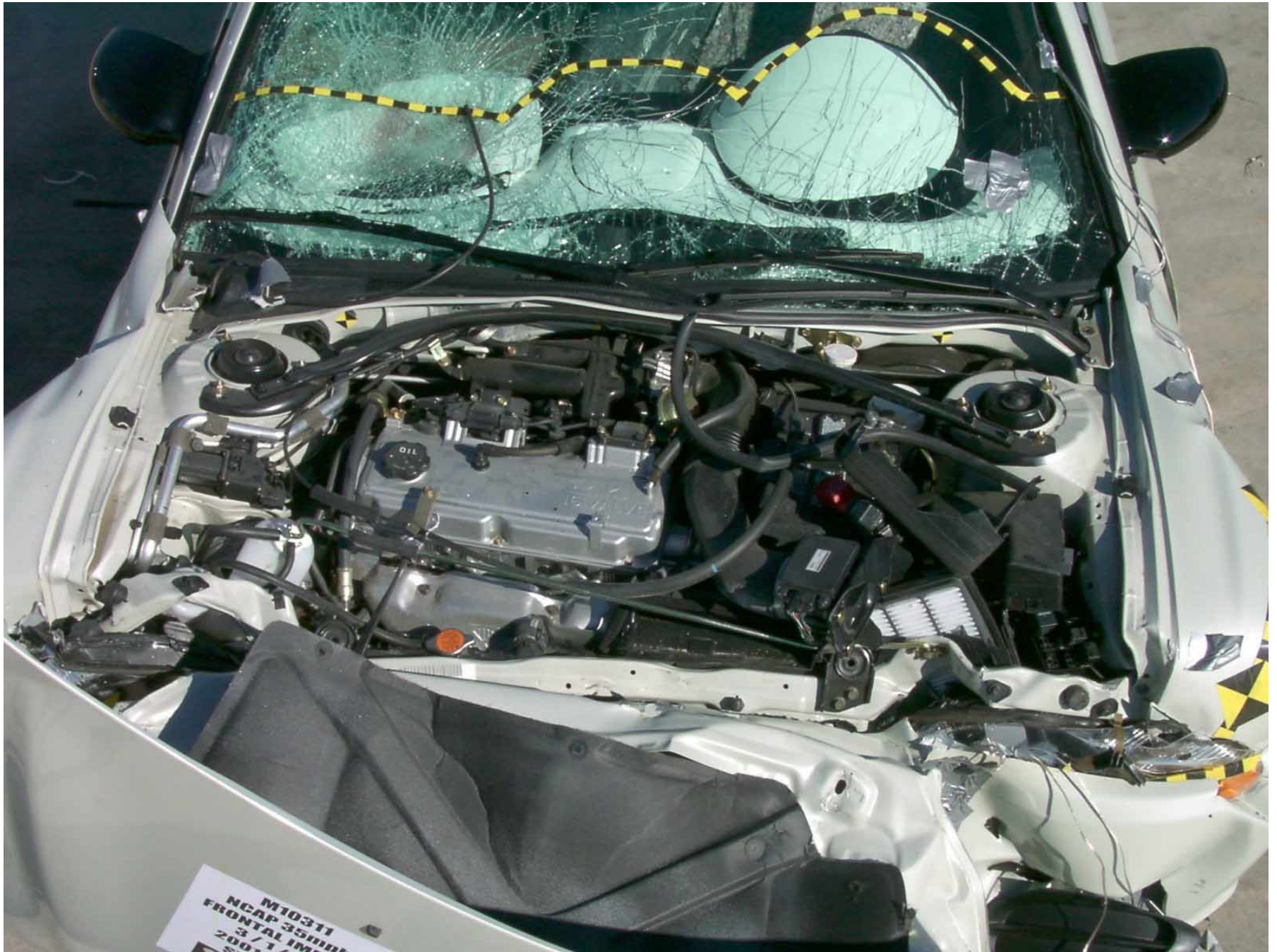
Figure A-18: Engine Compartment, Post-Test
