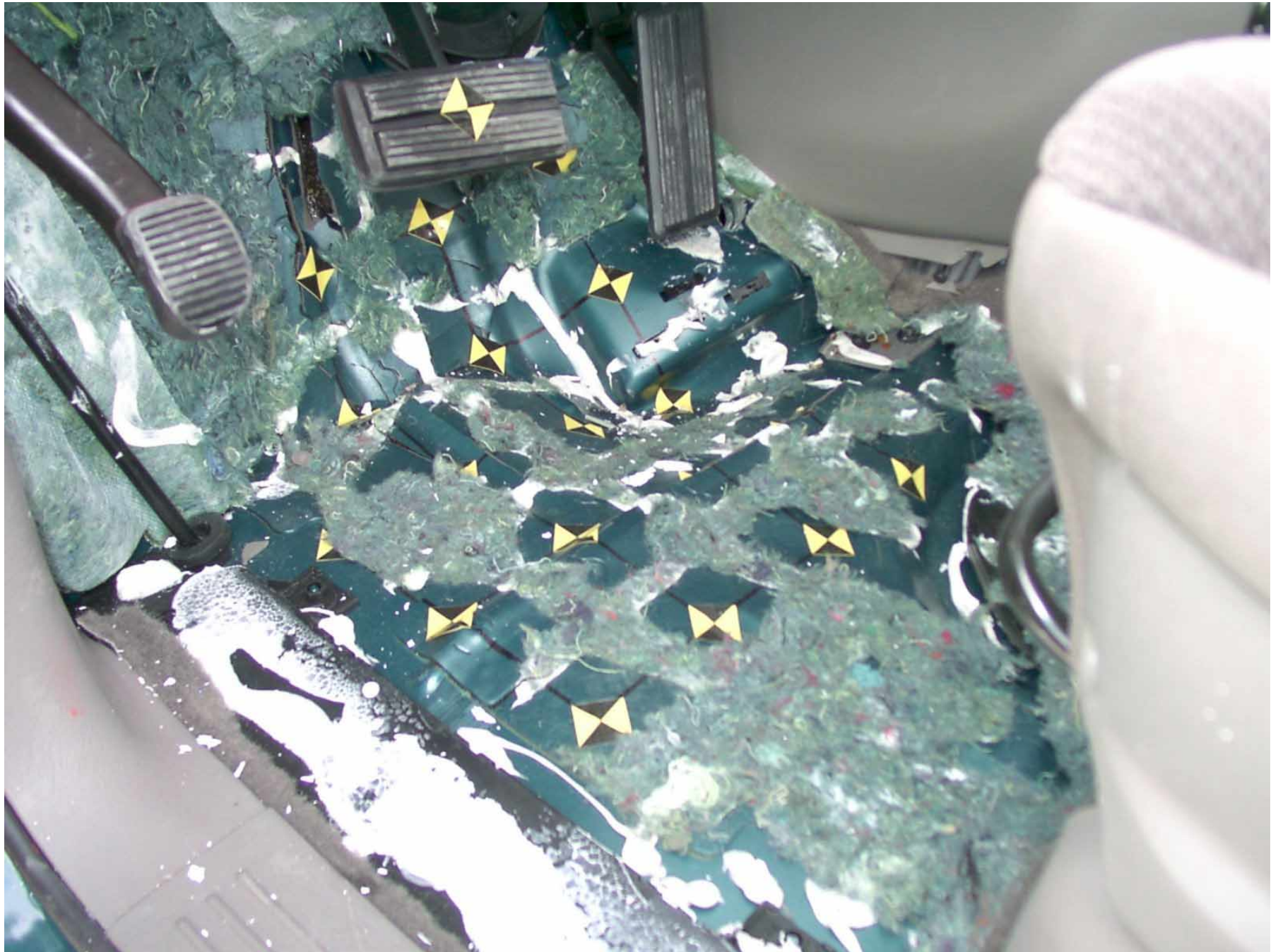
Figure A-38: Driver Side Floor Pan, Post-Test
