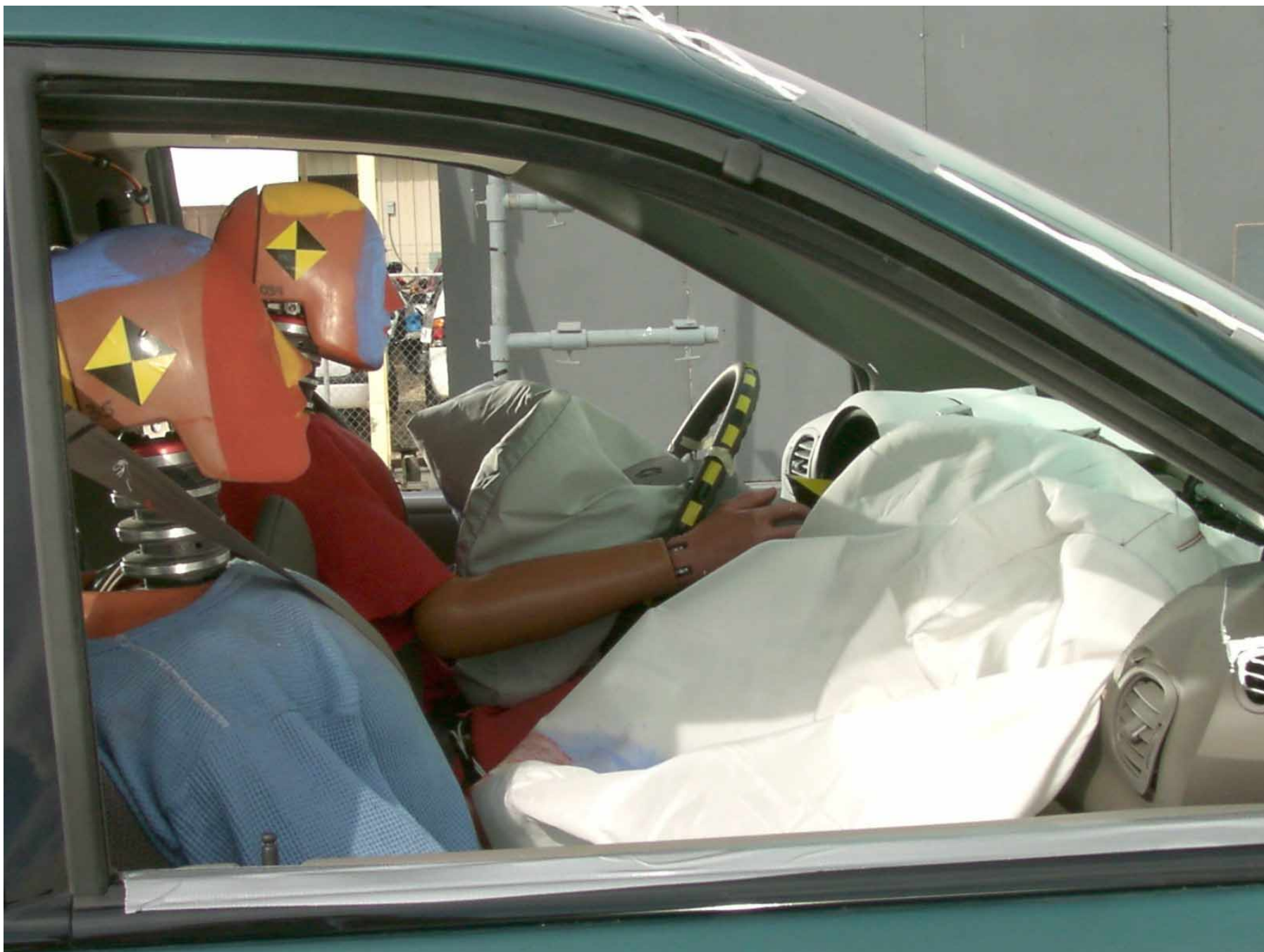
Figure A-44: Passenger Dummy Through Window, Post-Test
