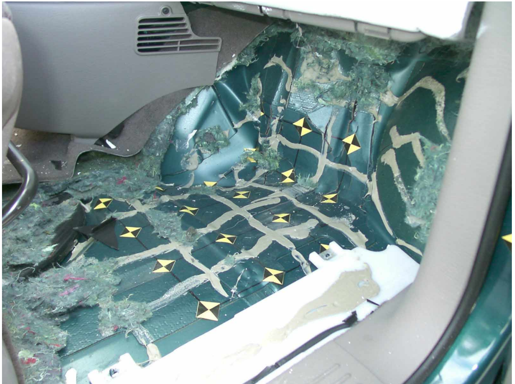
Figure A-52: Passenger Side Floor Pan, Post-Test
