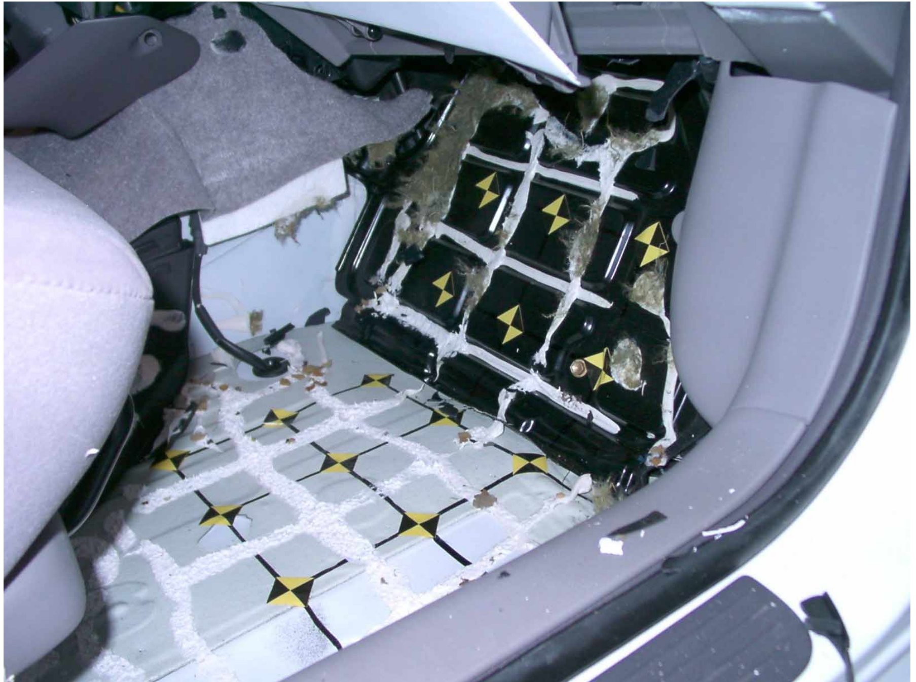
Figure A-52: Passenger Side Floor Pan, Post-Test
