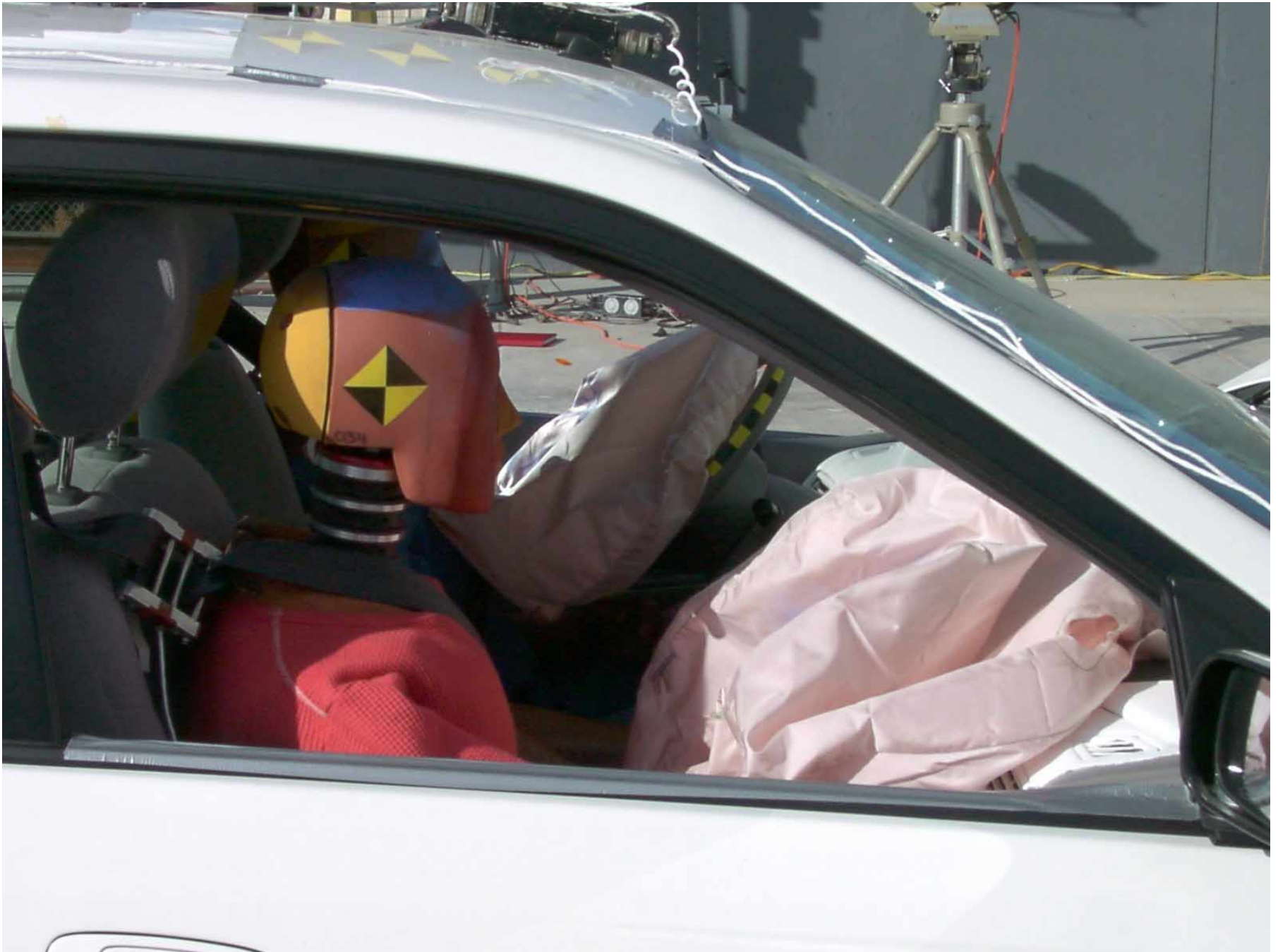
Figure A-44: Passenger Dummy Through Window, Post-Test
