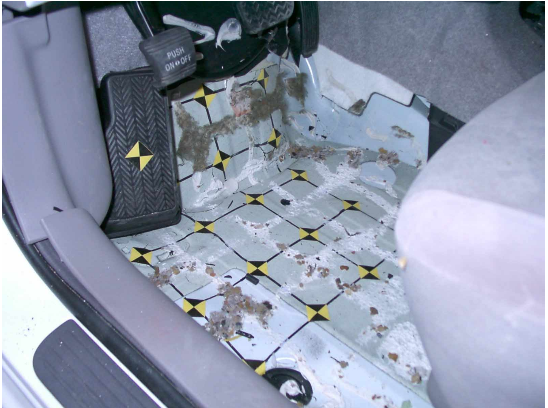
Figure A-38: Driver Side Floor Pan, Post-Test
