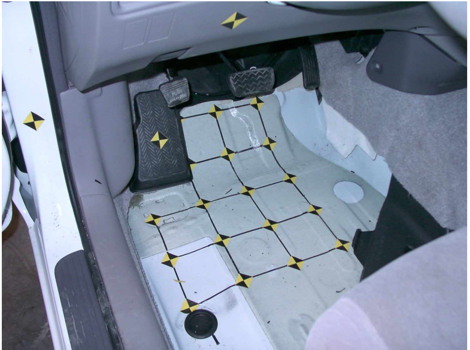
Figure A-37: Driver Side Floor Pan, Pre-Test
