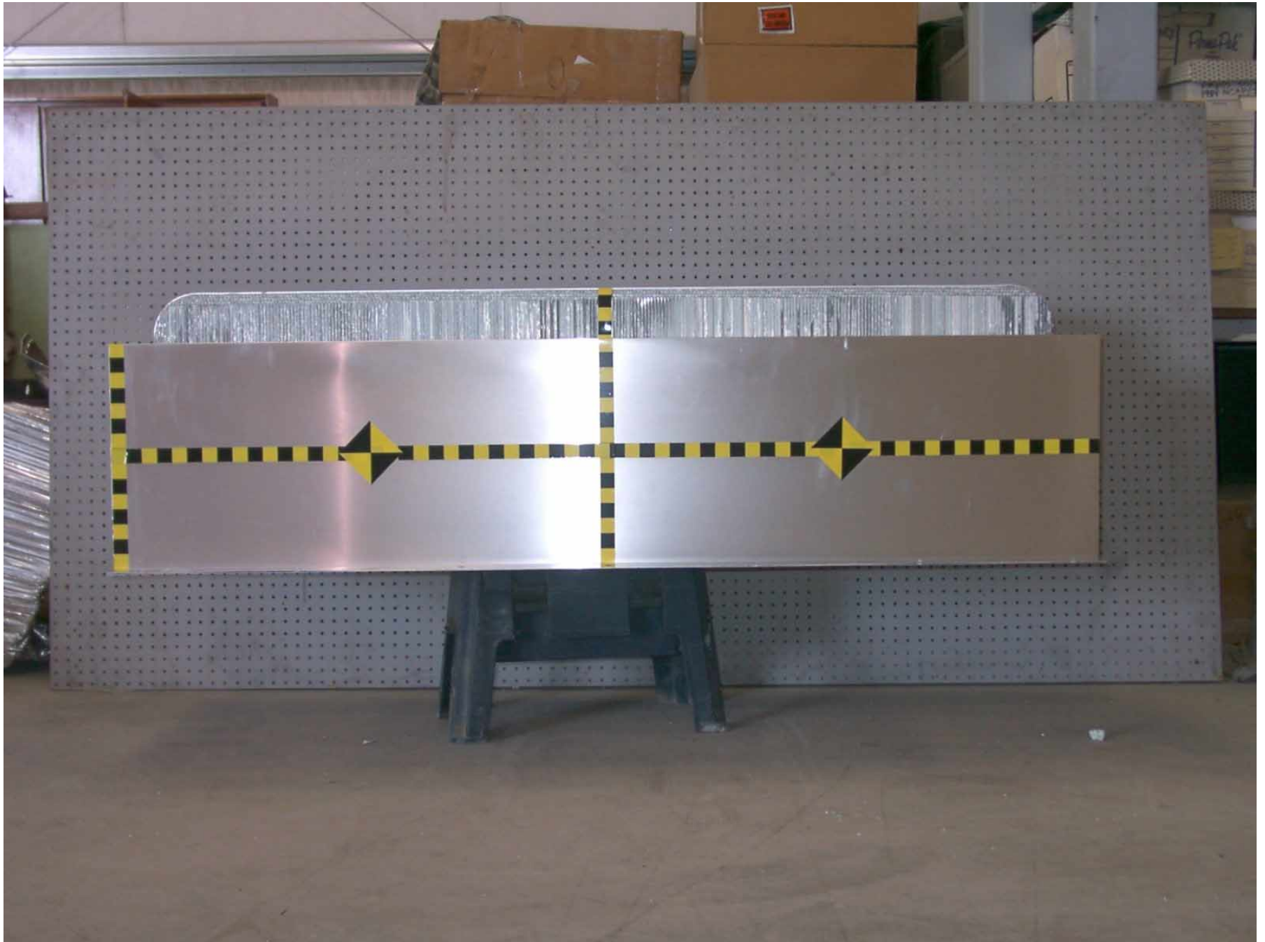
Figure A-38: Top View of Deformable Barrier, Pre-Test
