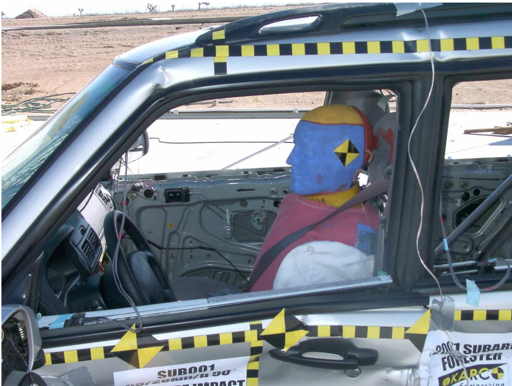
Figure A-20: Driver Dummy Left Side, Post-Test
