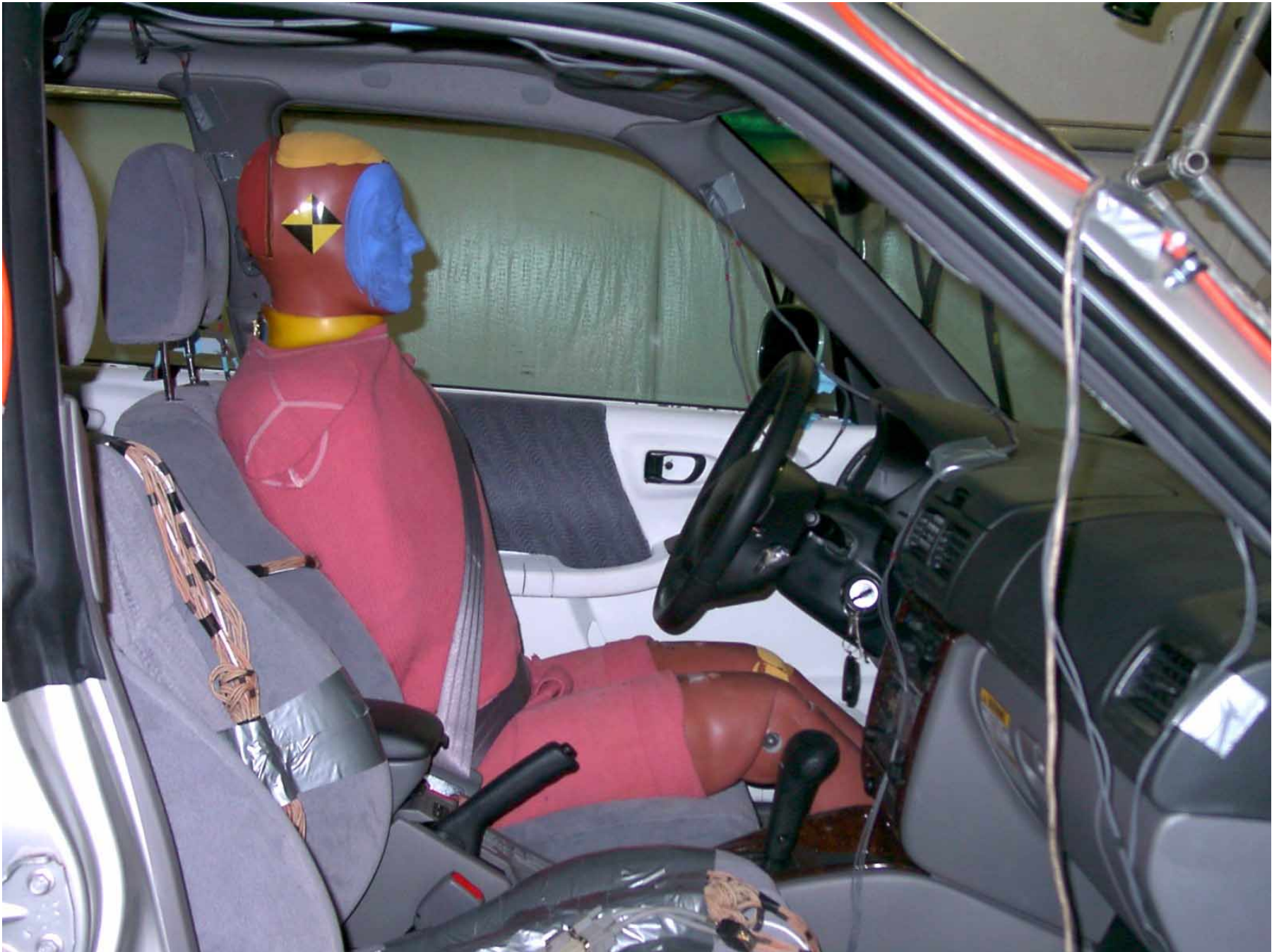
Figure A-23: Driver Dummy Inside View, Pre-Test
