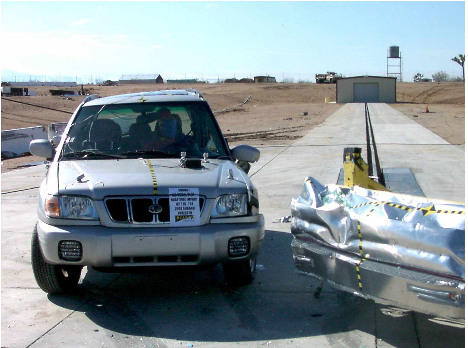
Figure A-6: Front View, Post-Test
