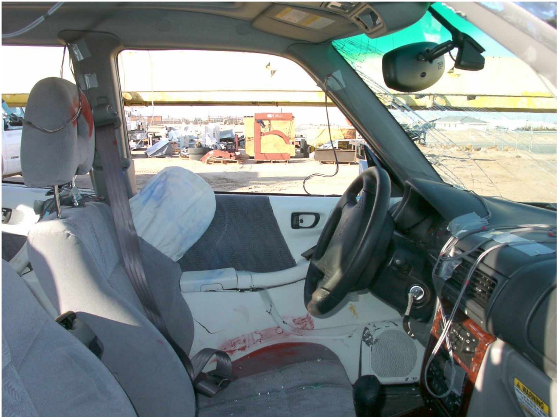
Figure A-26: Driver Dummy Contact Points Inside View, Post-Test
