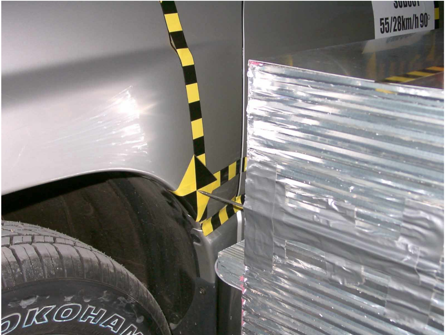
Figure A-16: Impact Point Target Close-up, Pre-Test
