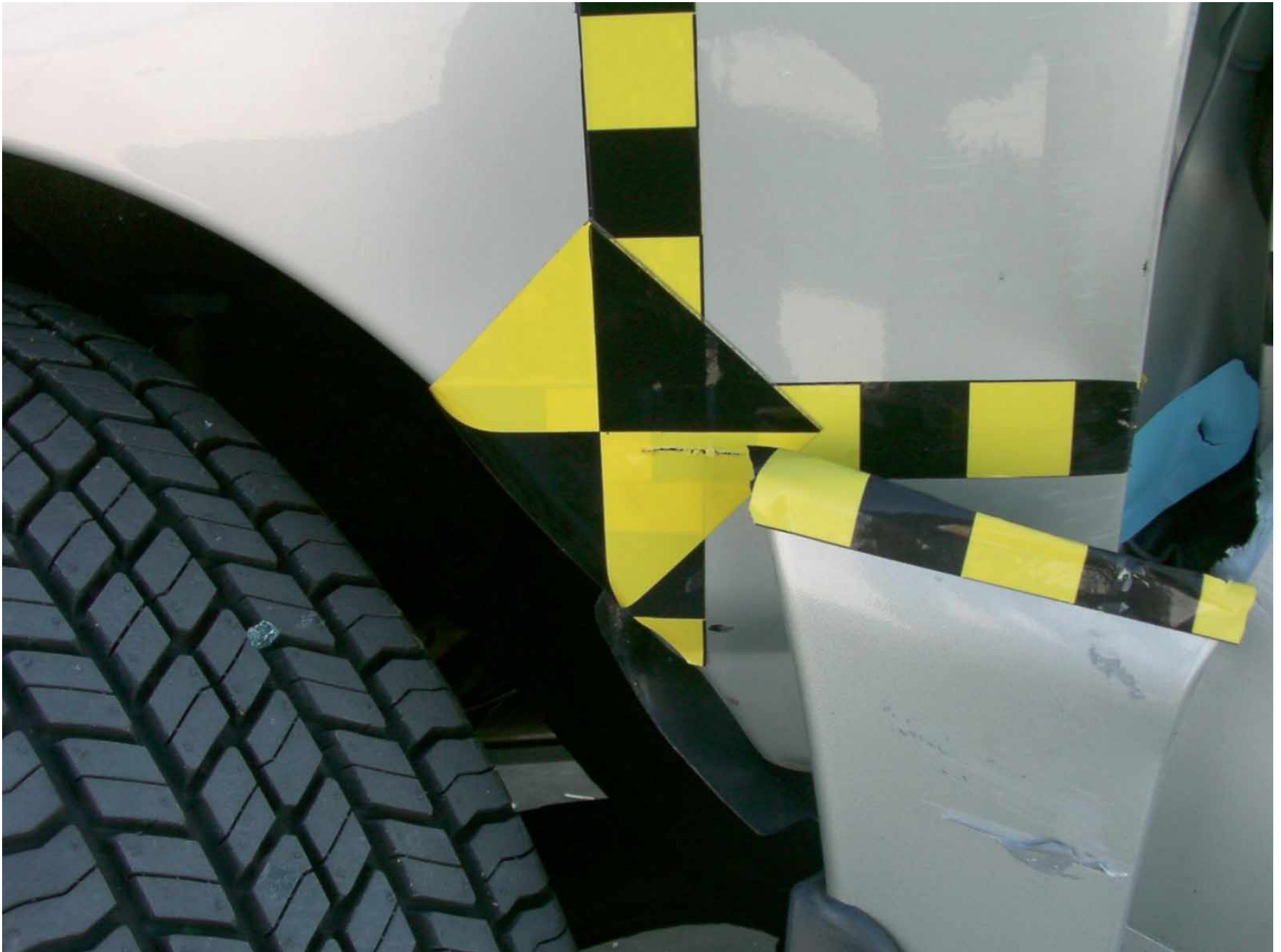
Figure A-17: Impact Point Target Close-up, Post-Test
