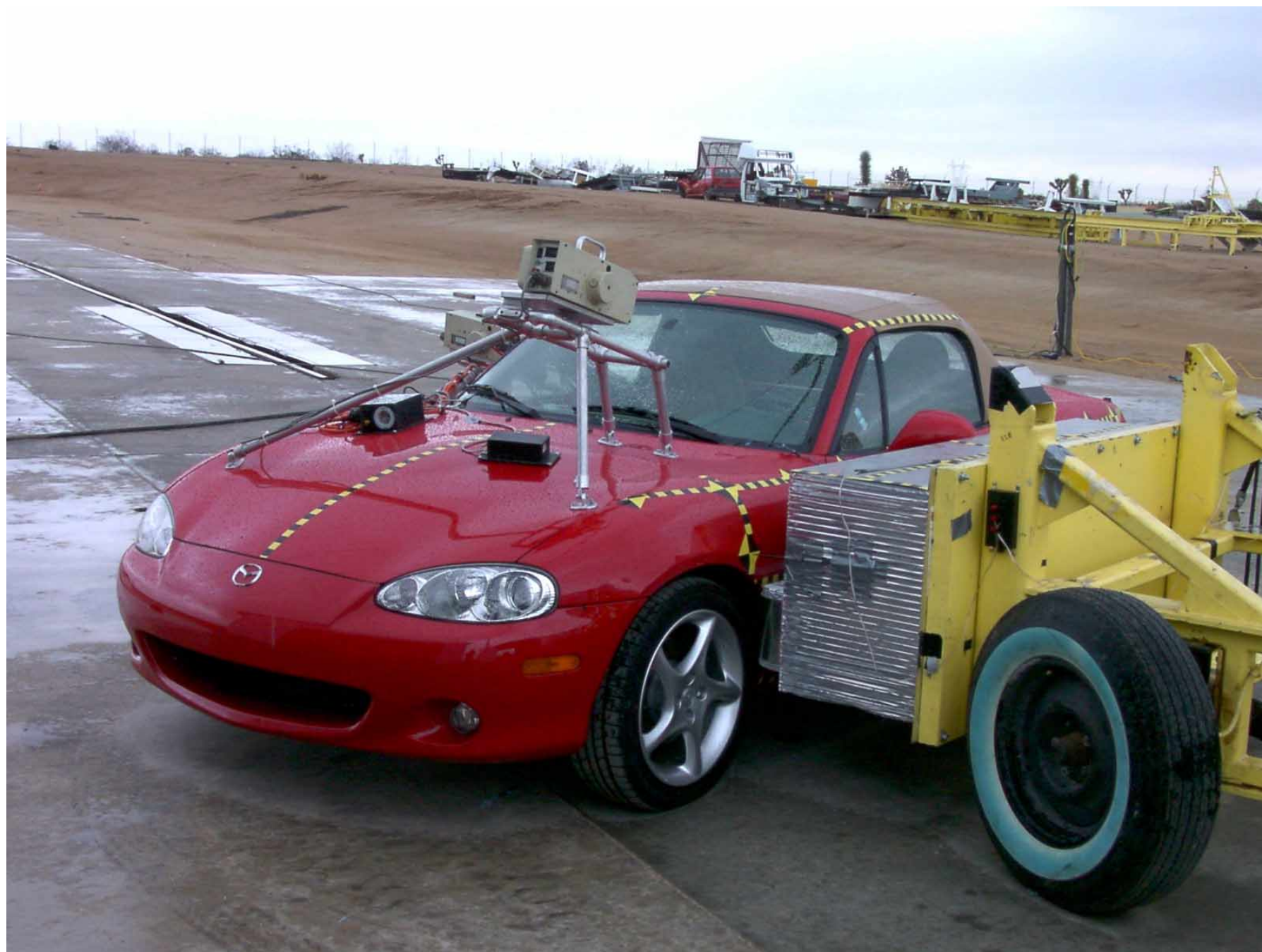
Figure A-14: MDB Left Side View (At Impact Position), Pre-Test
