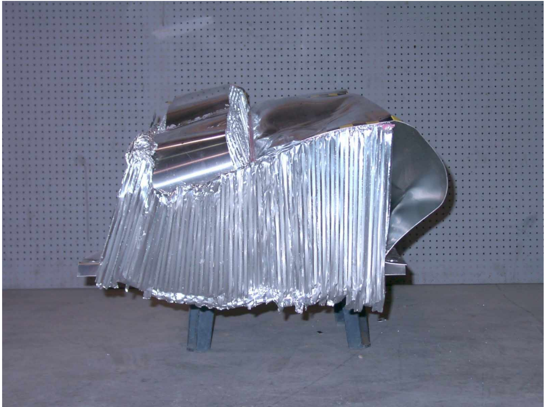
Figure A-34: Left Side of Deformable Barrier, Post-Test
