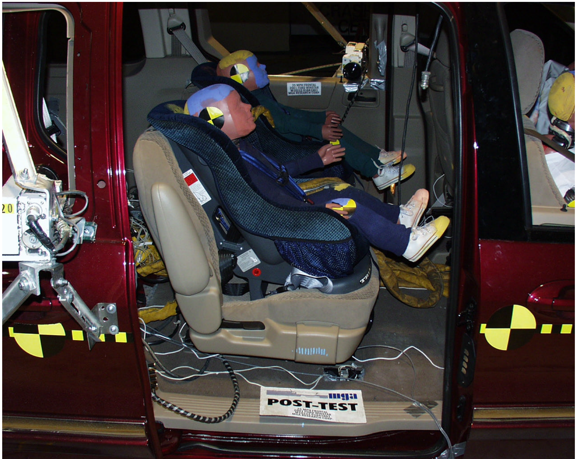
Photo 10 - Post-Test RRS 3 Year Old Right Side View (Door Open)
