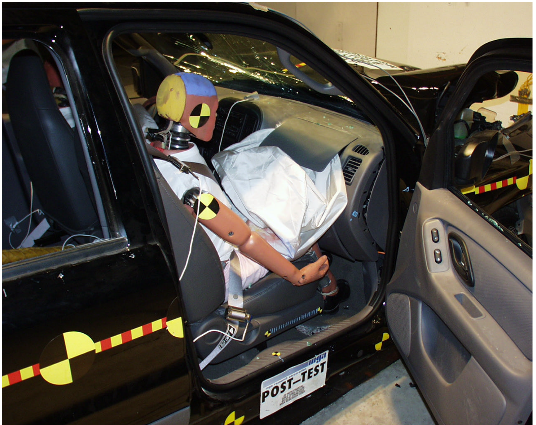
Photo No. A-30 - Post-Test Passenger Dummy Position Right Side View (Door Open)
