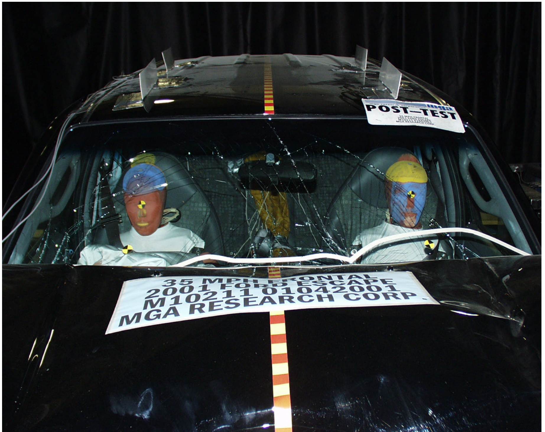
Photo No. A-15 - Post-Test Windshield View
