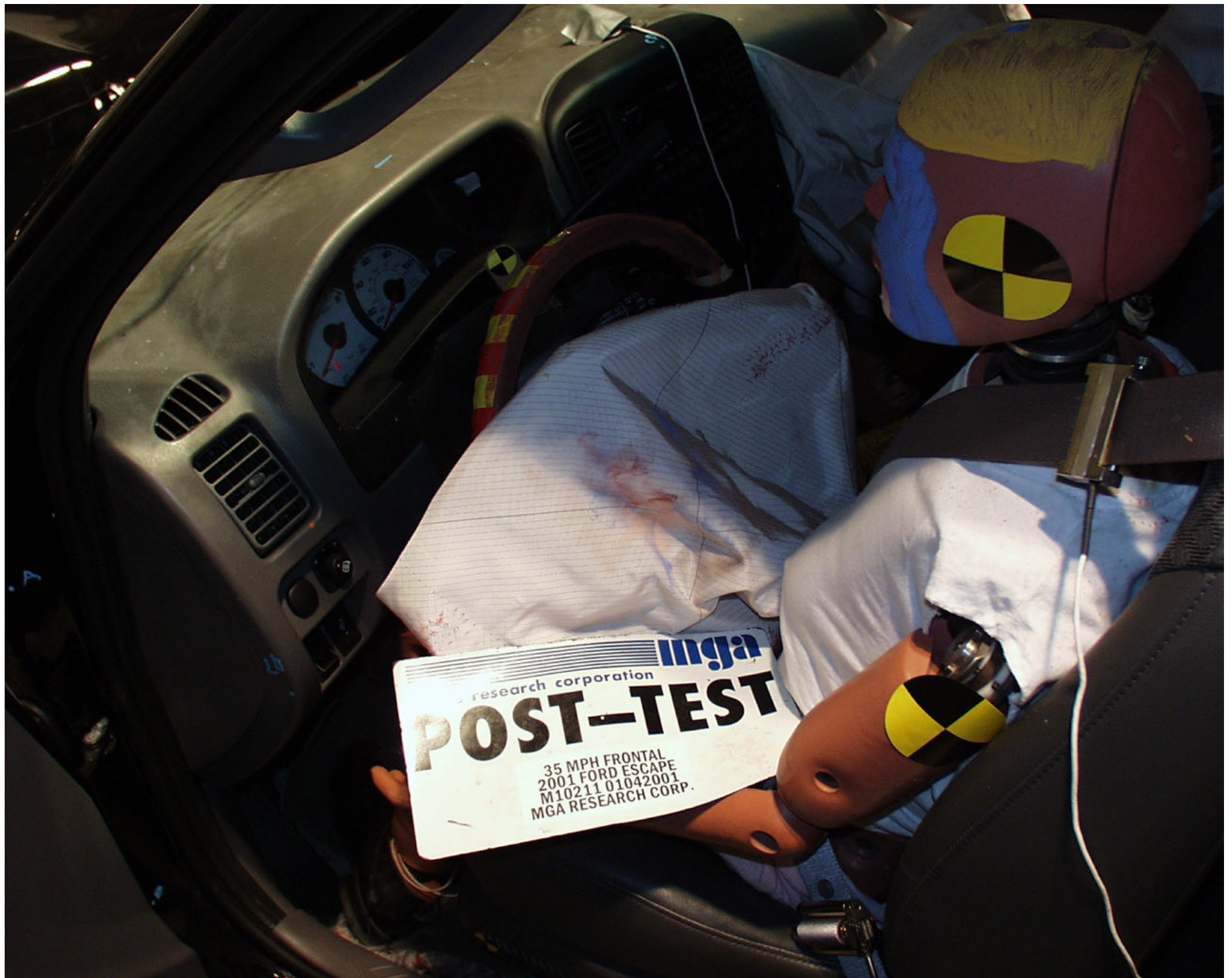
Photo No. A-24 - Post-Test Driver Airbag Contact
