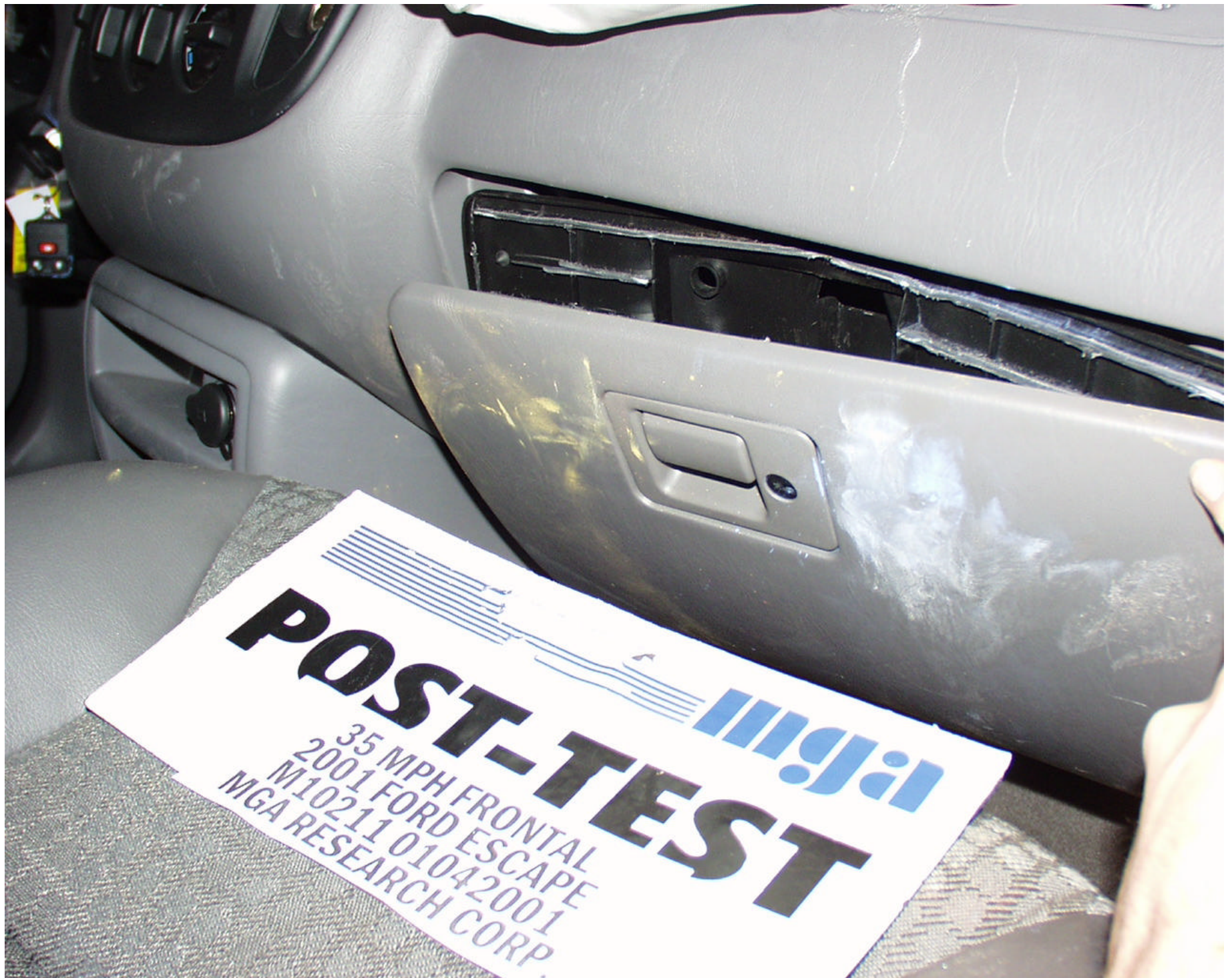
Photo No. A-36 - Post-Test Passenger Knee Contact View
