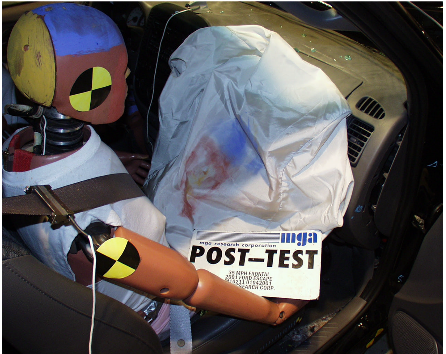
Photo No. A-35 - Post-Test Passenger Airbag Contact
