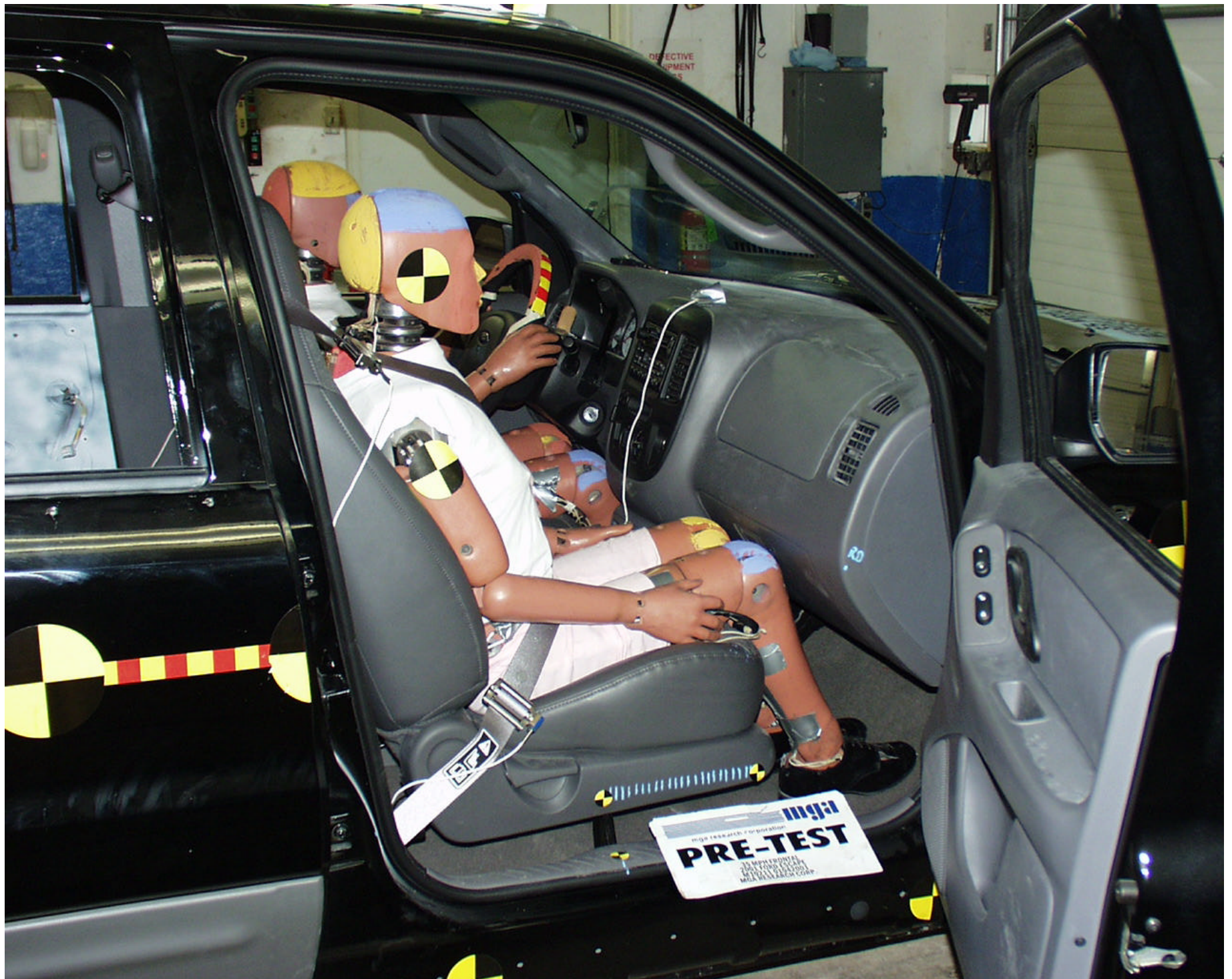
Photo No. A-29 - Pre-Test Passenger Dummy Position Right Side View (Door Open)
