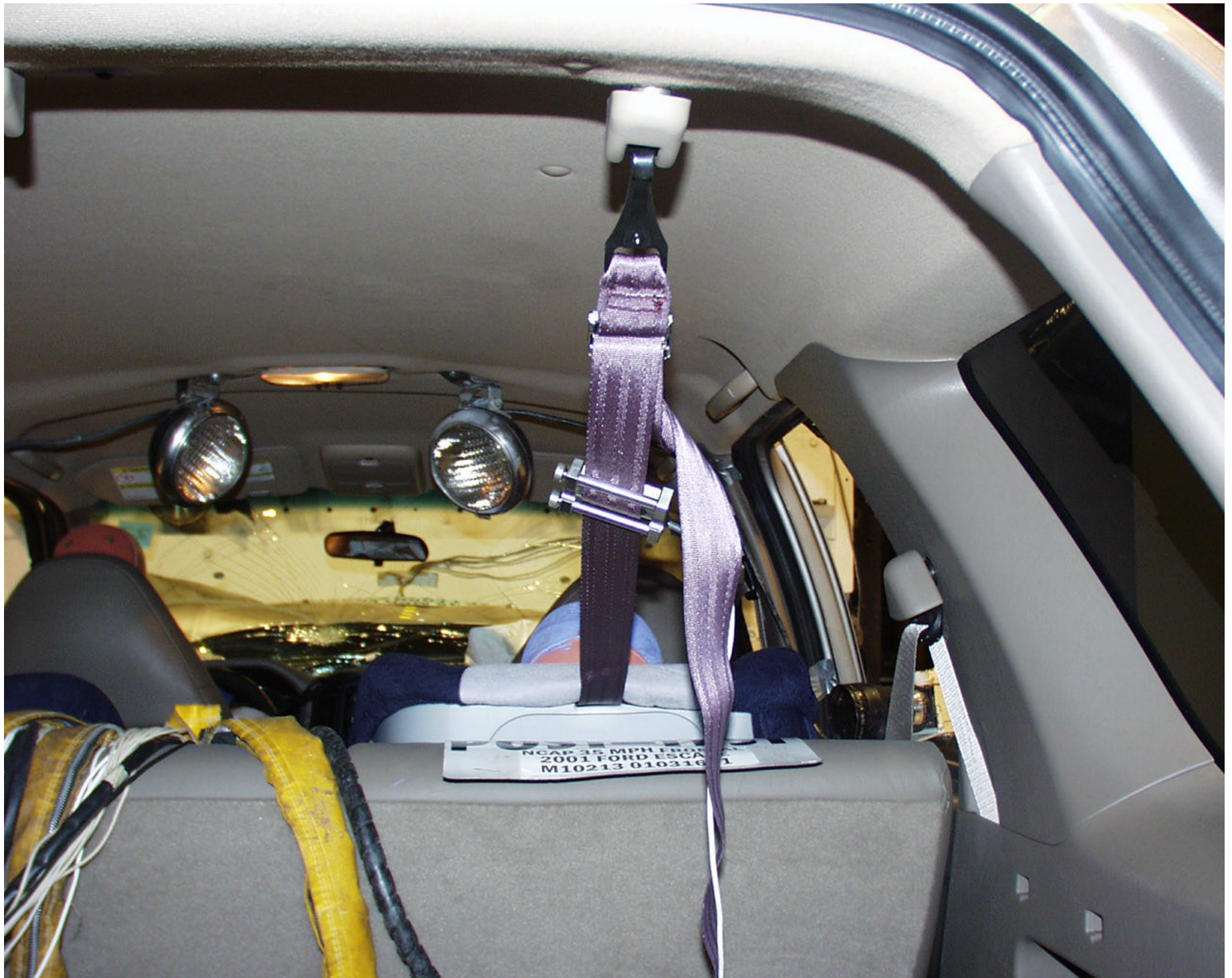
Photo 14 - Post-Test Right Side Tether Strap View
