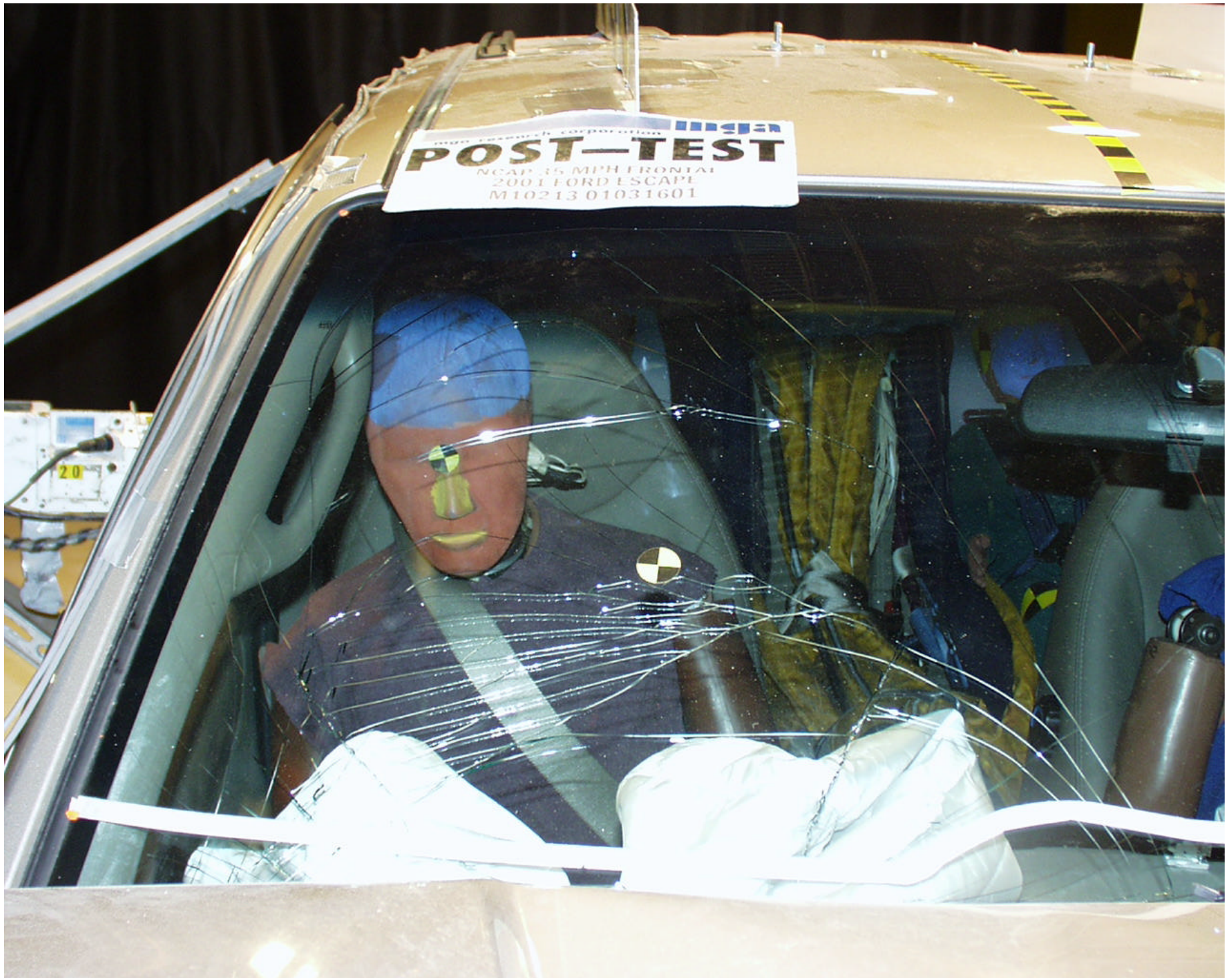
Photo No. A-45 - Post-Test Passenger Windshield View
