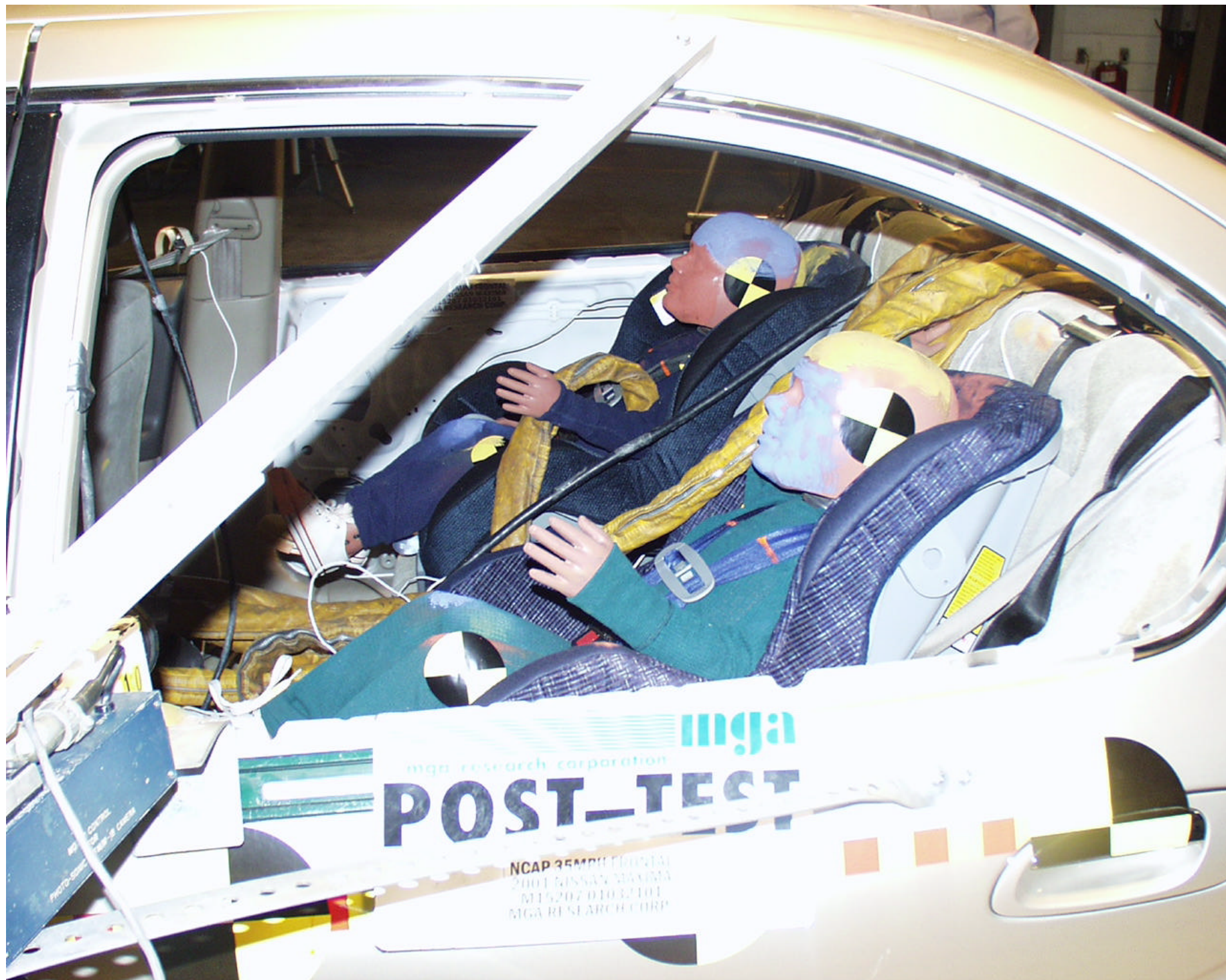
Photo 2 - Post-Test LRS 3 Year Old Left Side View
