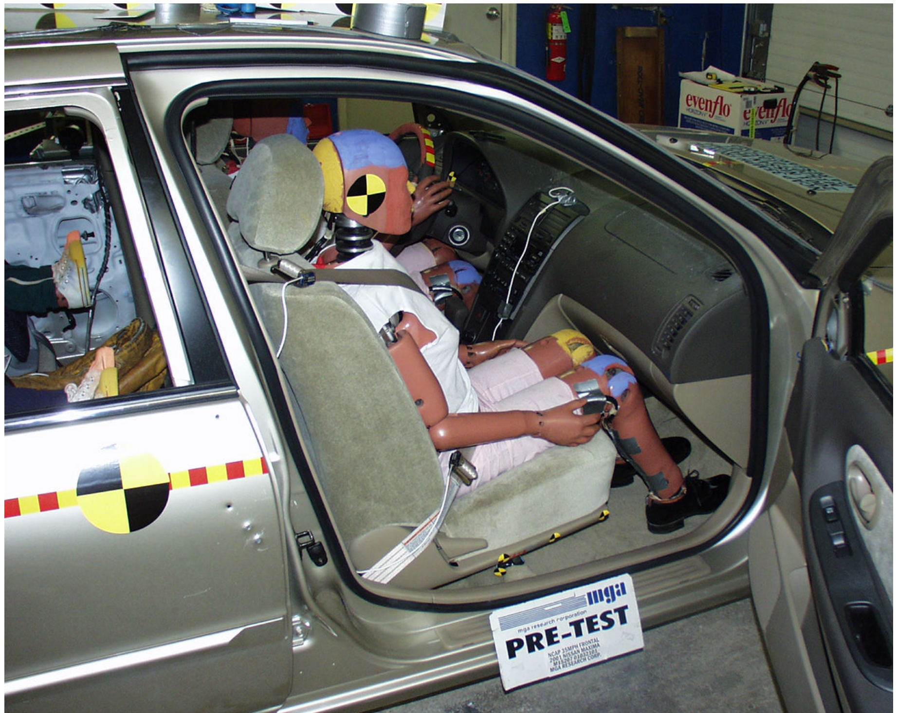
Photo No. A-36 - Pre-Test Passenger Dummy Position Right Side View (Door Open)
