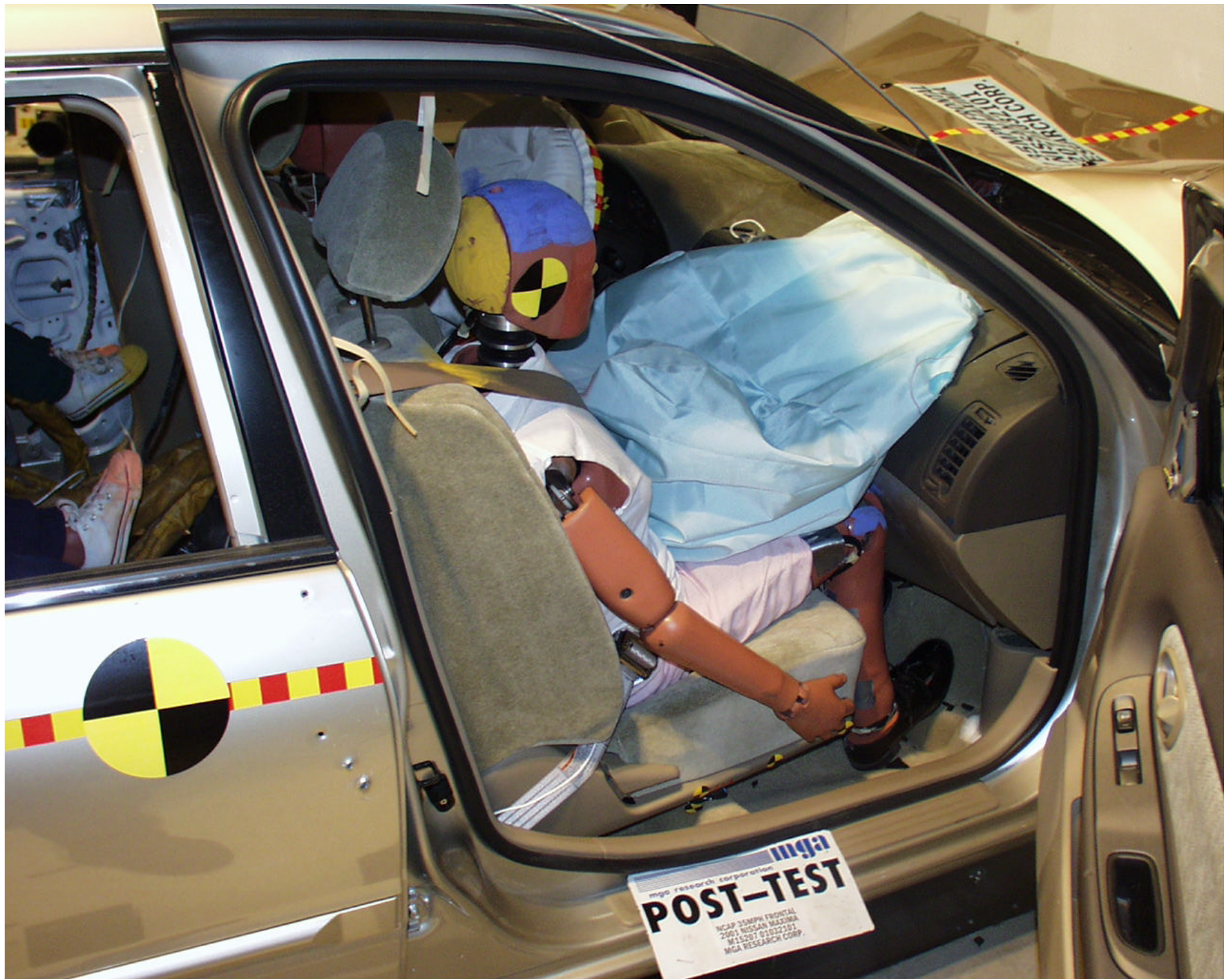
Photo No. A-37 - Post-Test Passenger Dummy Position Right Side View (Door Open)
