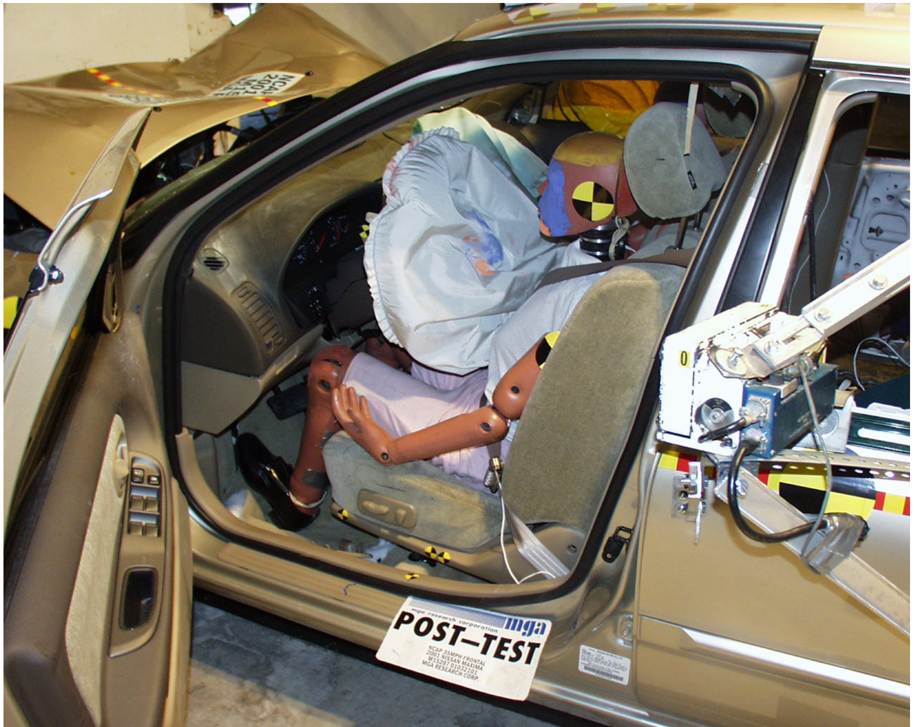
Photo No. A-25 - Post-Test Driver Dummy Position Left Side View (Door Open)
