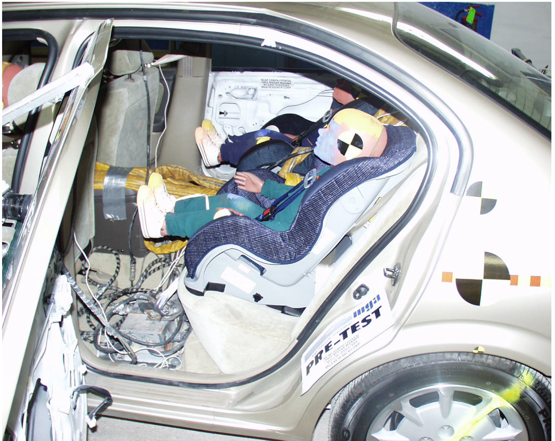
Photo 3 - Pre-Test LRS 3 Year Old Left Side View (Door Open)
