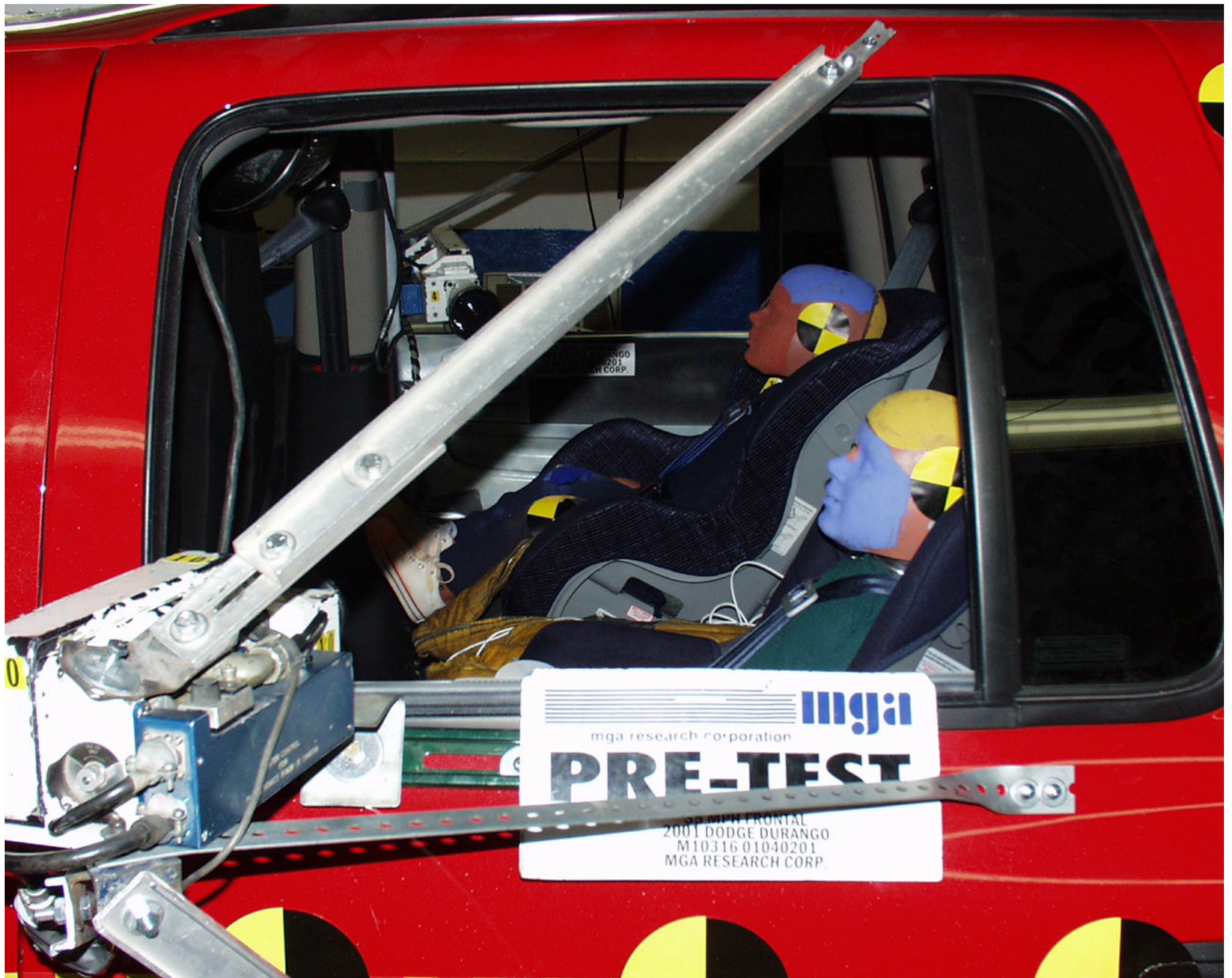
Photo 1 - Pre-Test LRS 3 Year Old Left Side View
