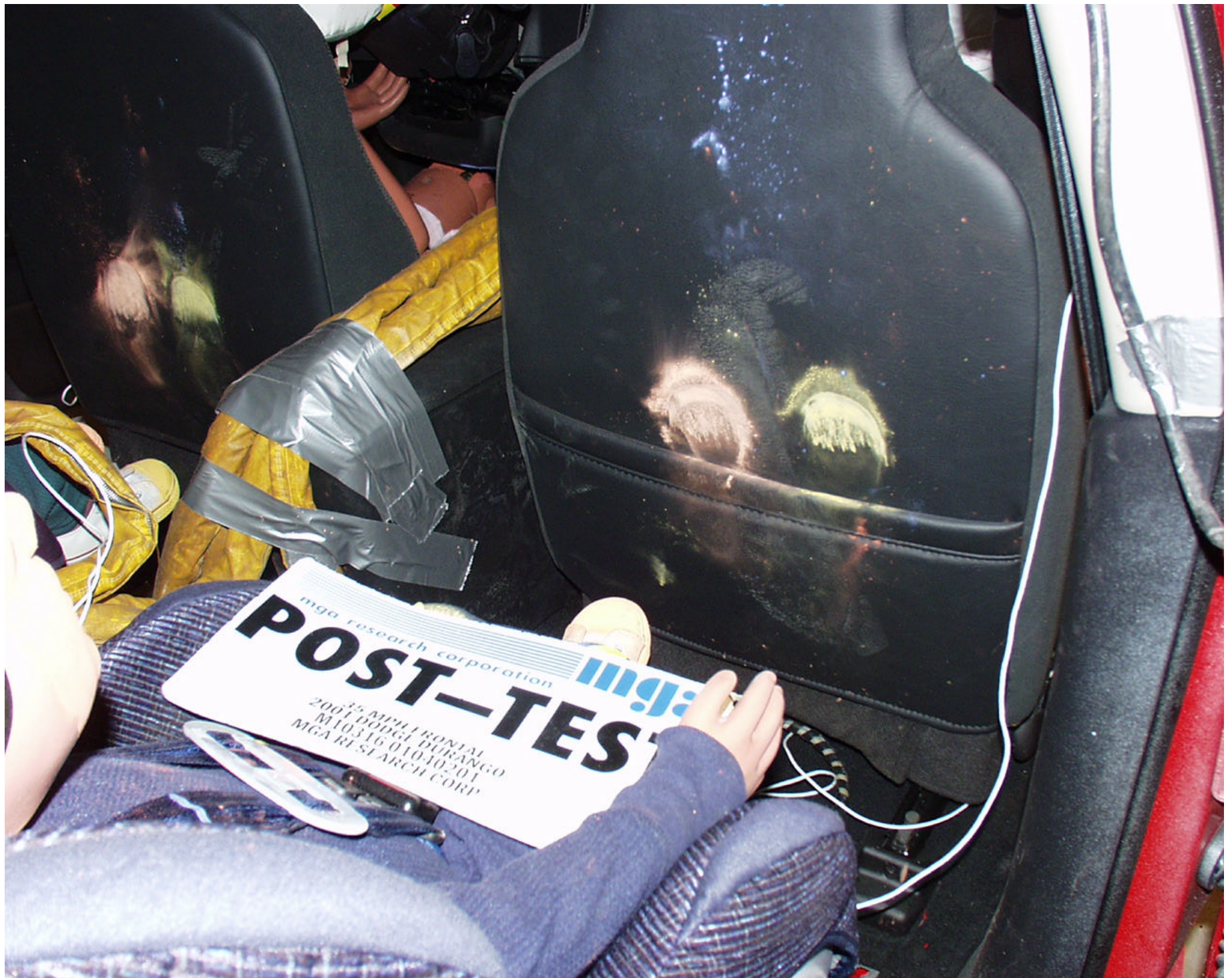
Photo 14 - Post-Test RRS Feet Contact View
