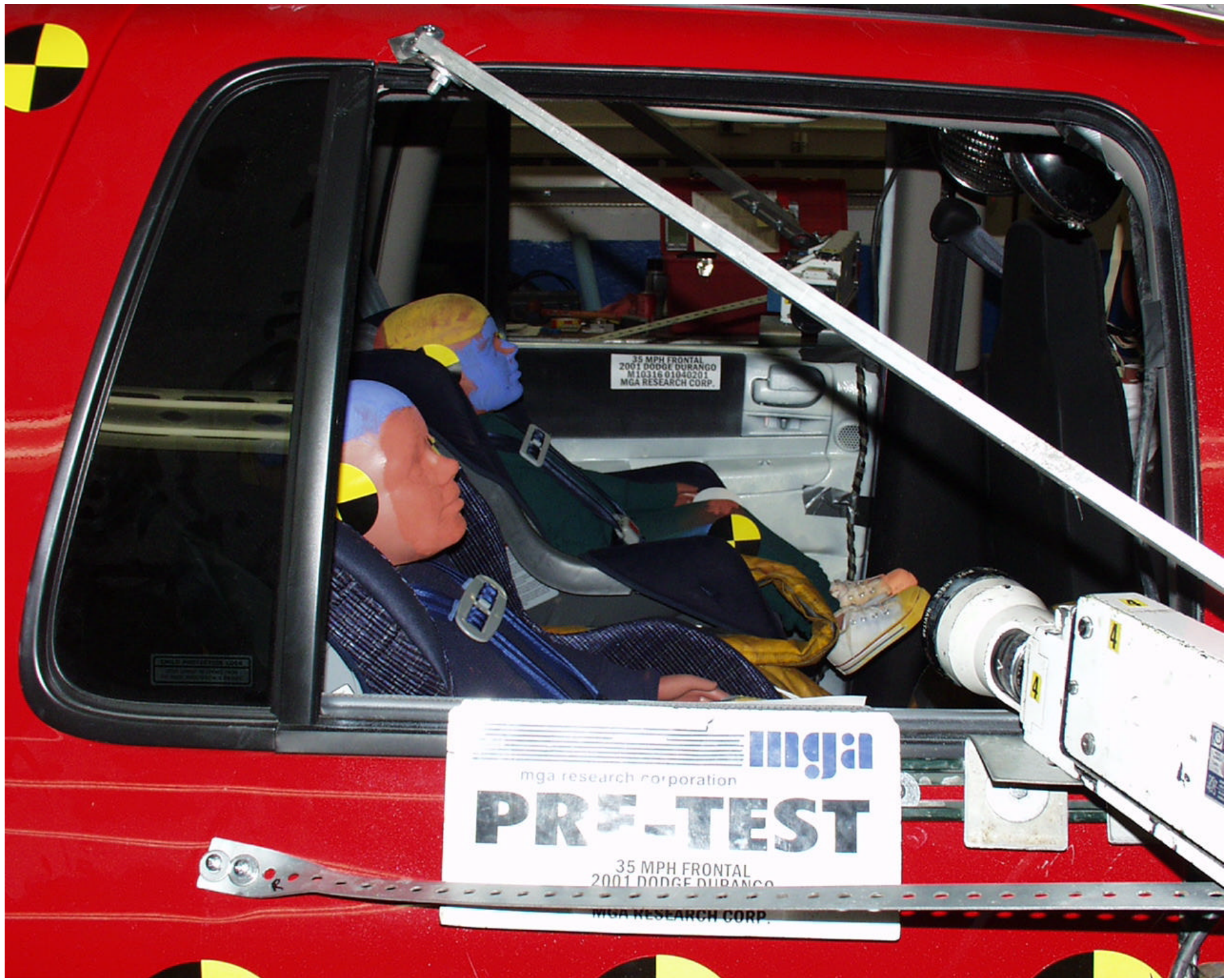
Photo 5 - Pre-Test RRS 3 Year Old Right Side View
