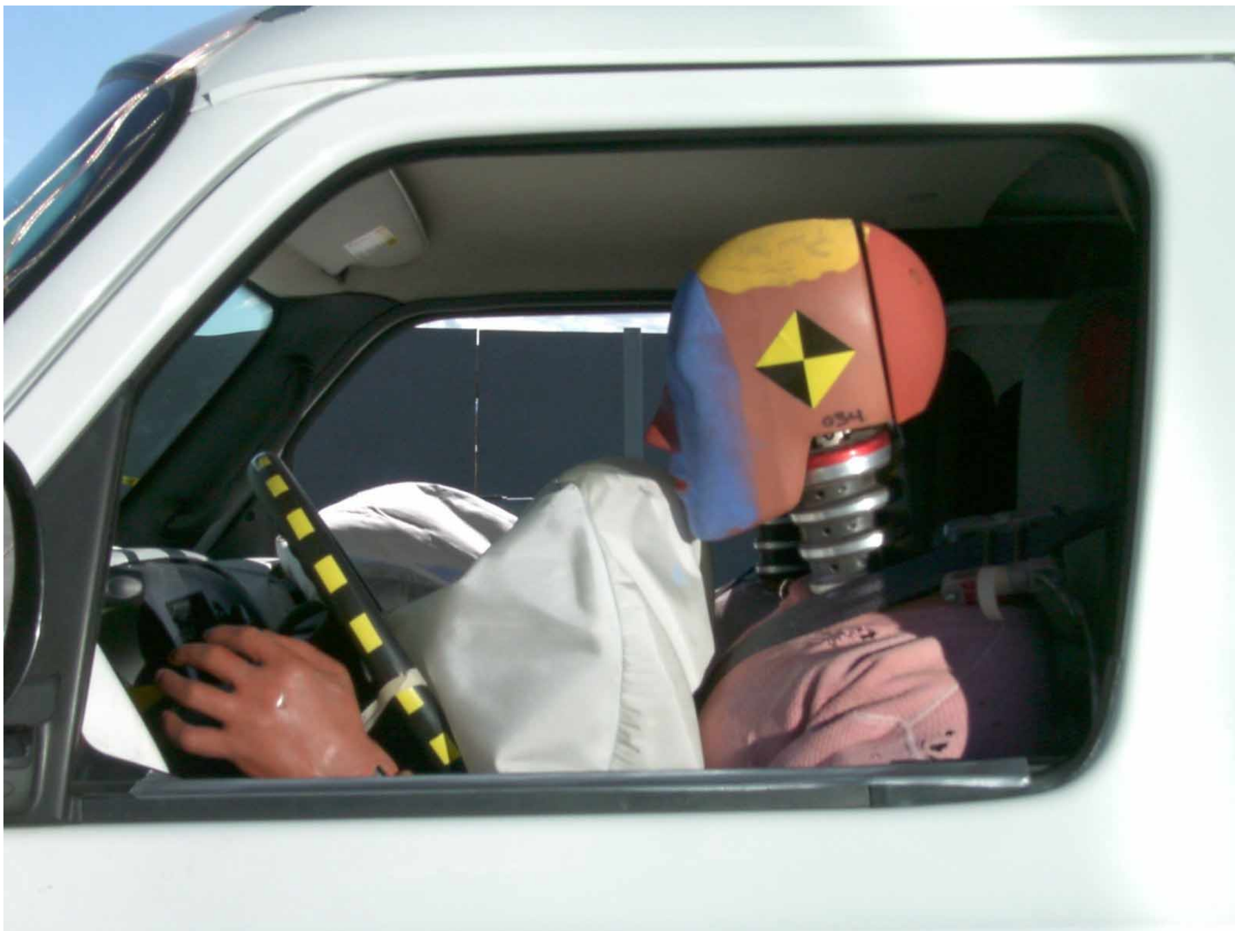
Figure A-28: Driver Dummy Through Window, Post-Test
