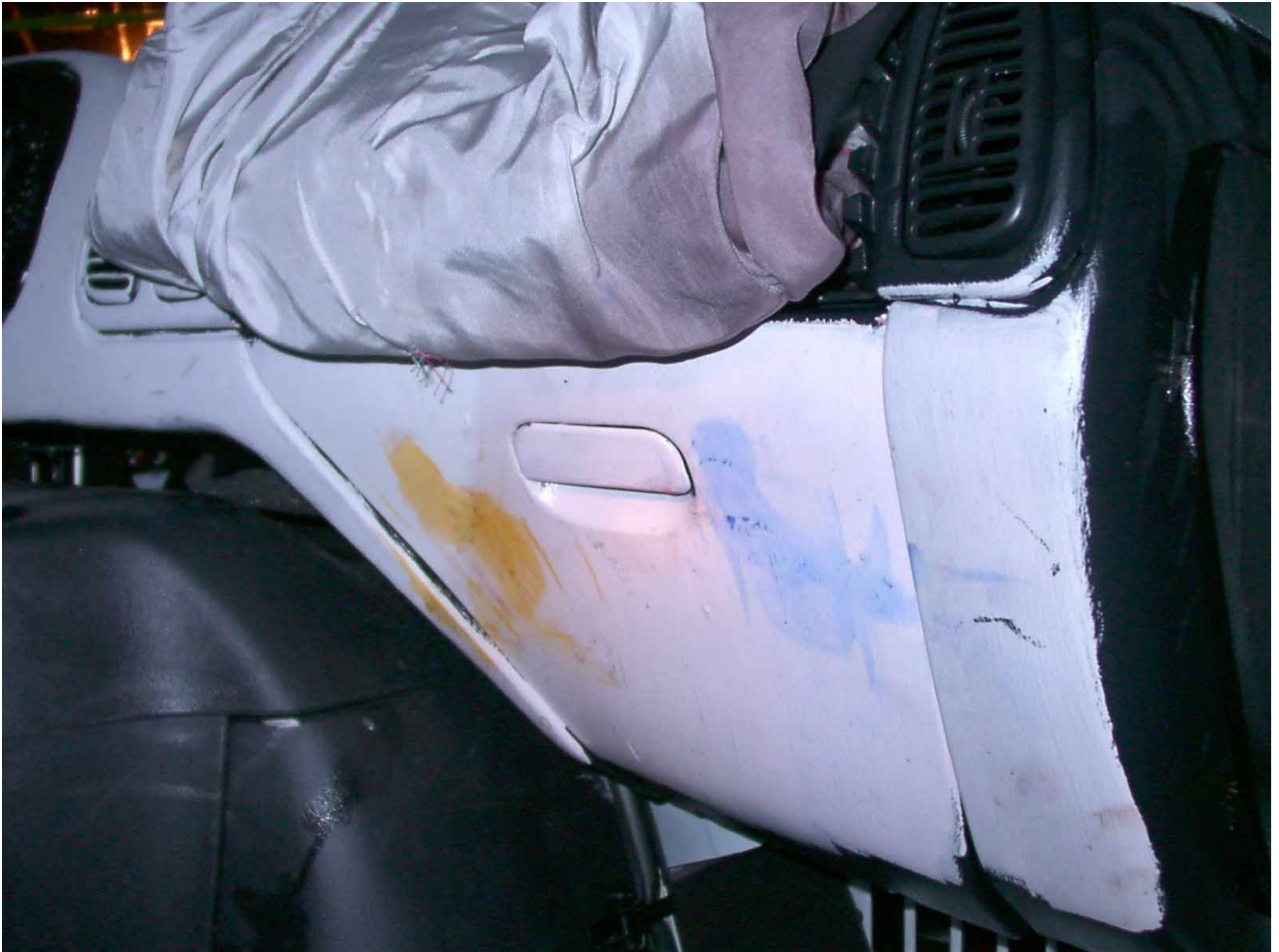
Figure A-54: Passenger Side Knee Bolster, Post-Test
