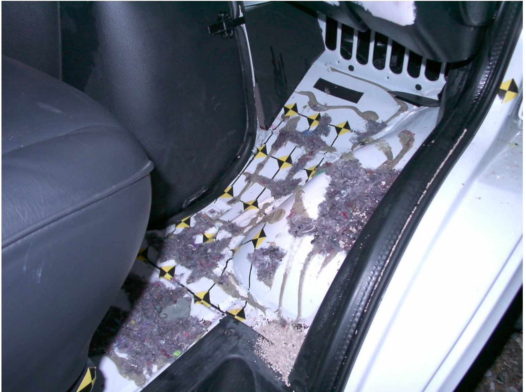
Figure A-52: Passenger Side Floor Pan, Post-Test
