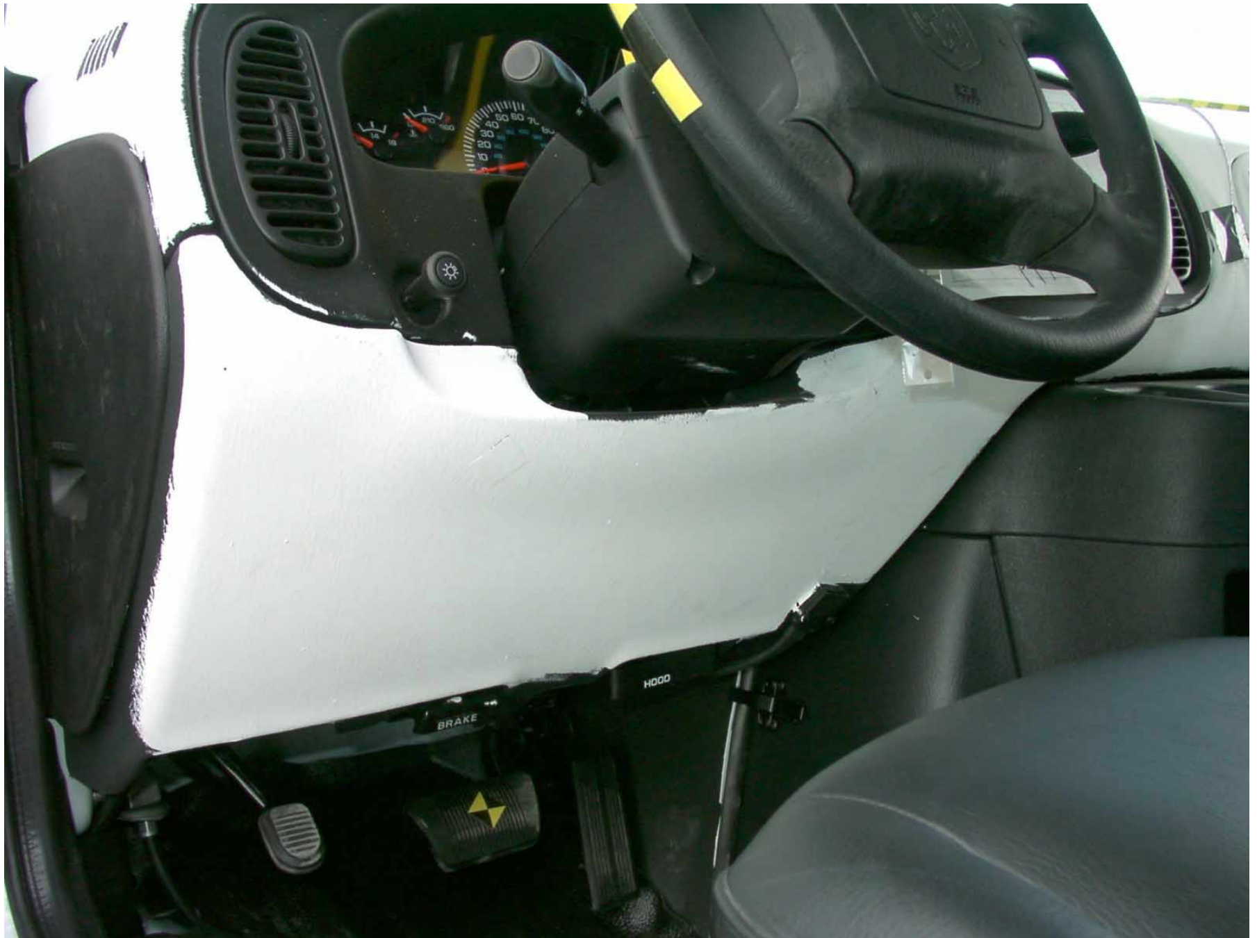
Figure A-35: Driver Side Knee Bolster, Pre-Test
