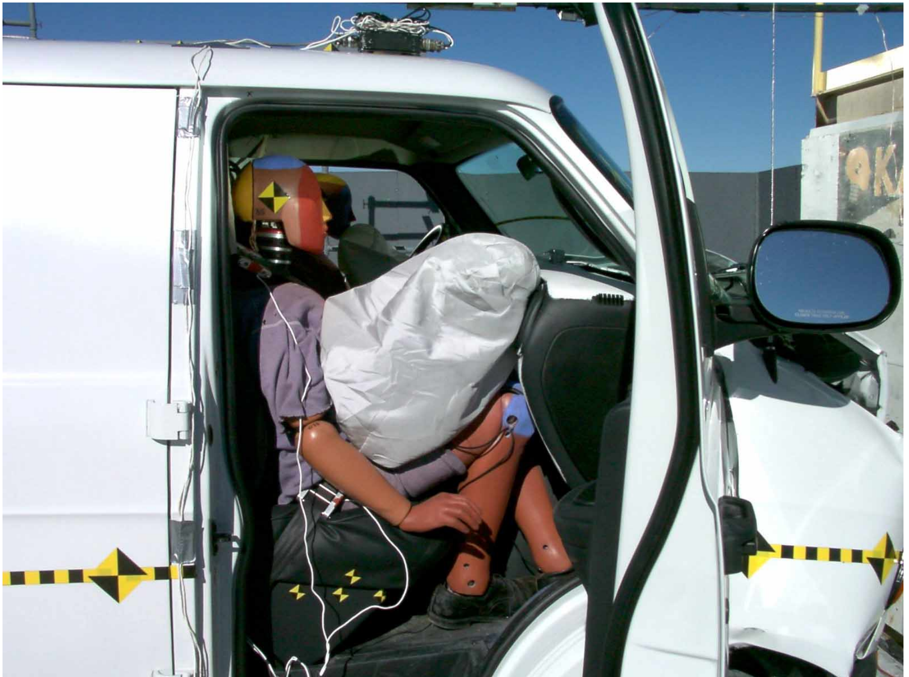
Figure A-48: Passenger Dummy 90° To Vehicle, Post-Test
