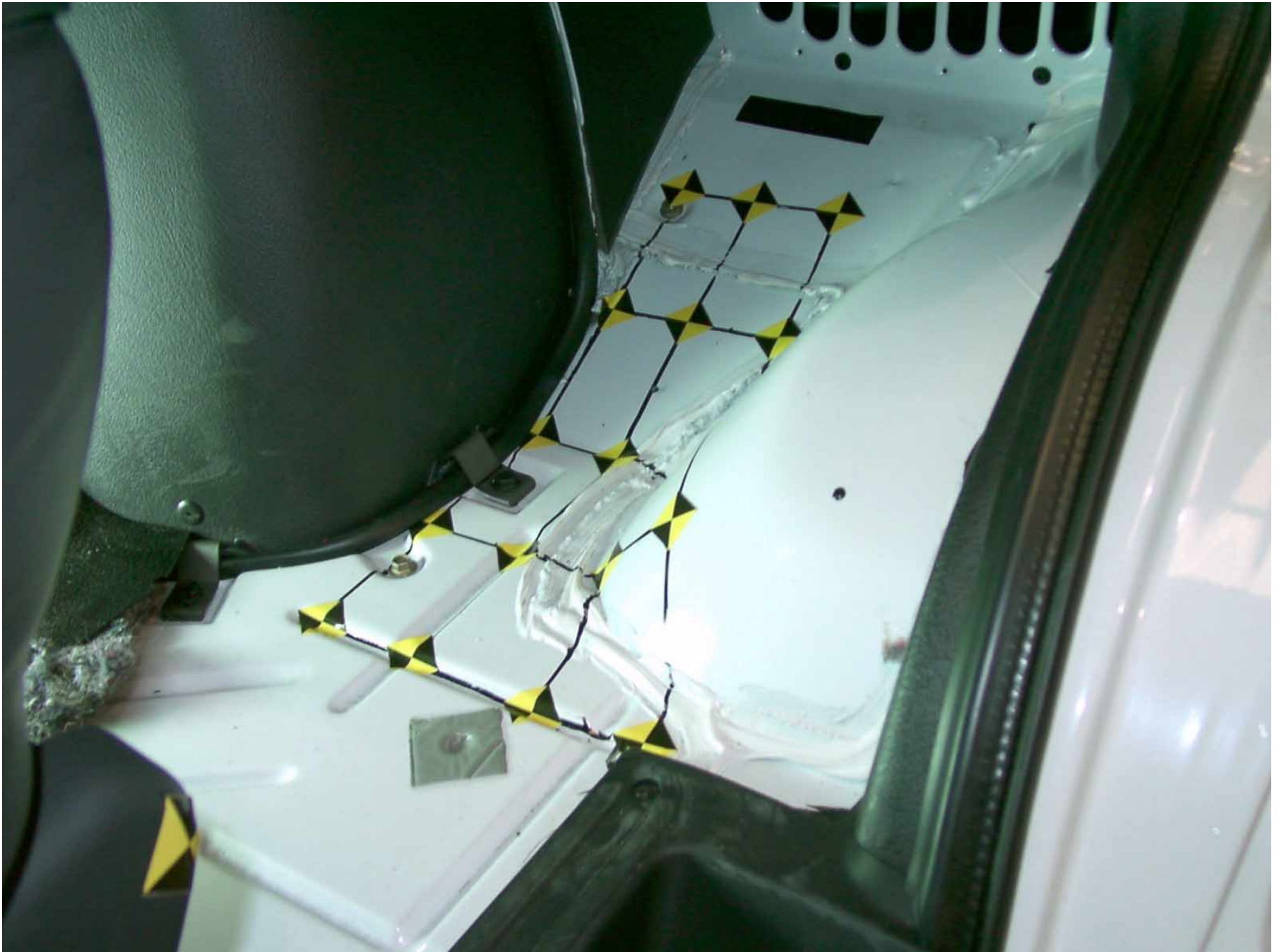
Figure A-51: Passenger Side Floor Pan, Pre-Test
