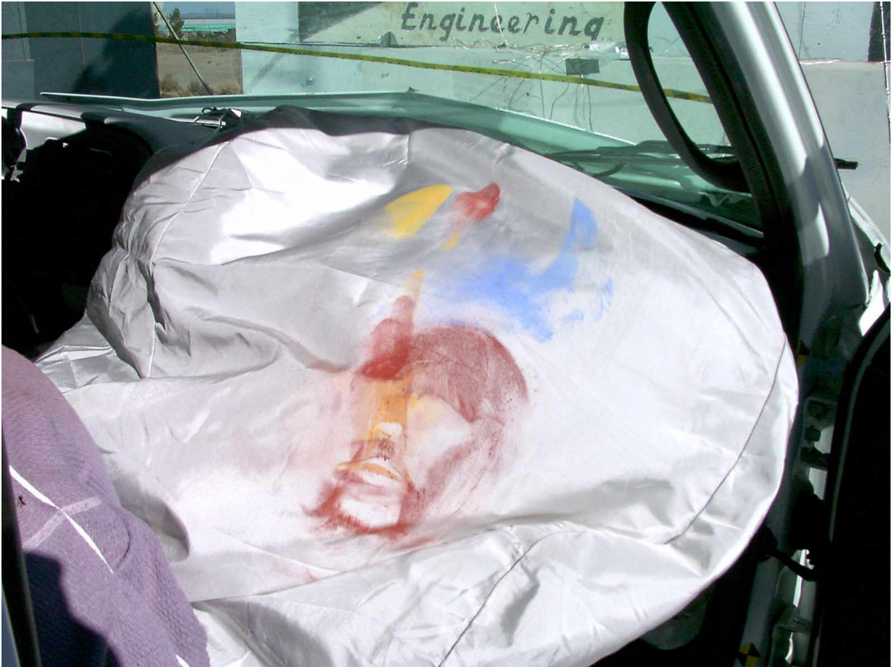
Figure A-56: Passenger Dummy Contact, Post-Test
