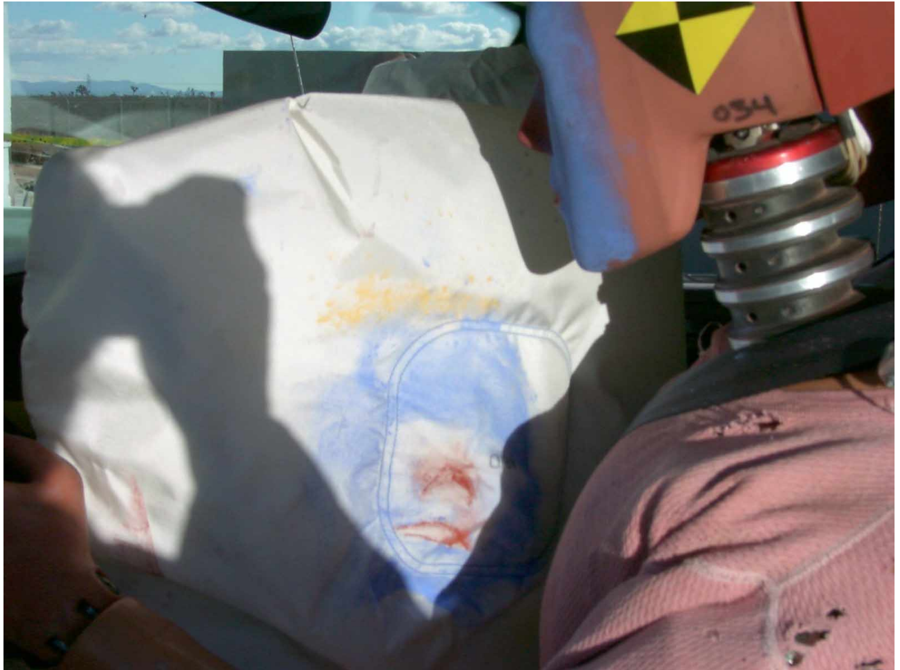
Figure A-40: Driver Dummy Contact, Post-Test
