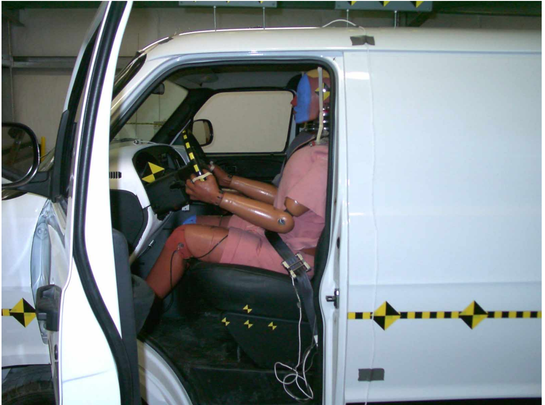
Figure A-31: Driver Dummy 90° To Vehicle, Pre-Test
