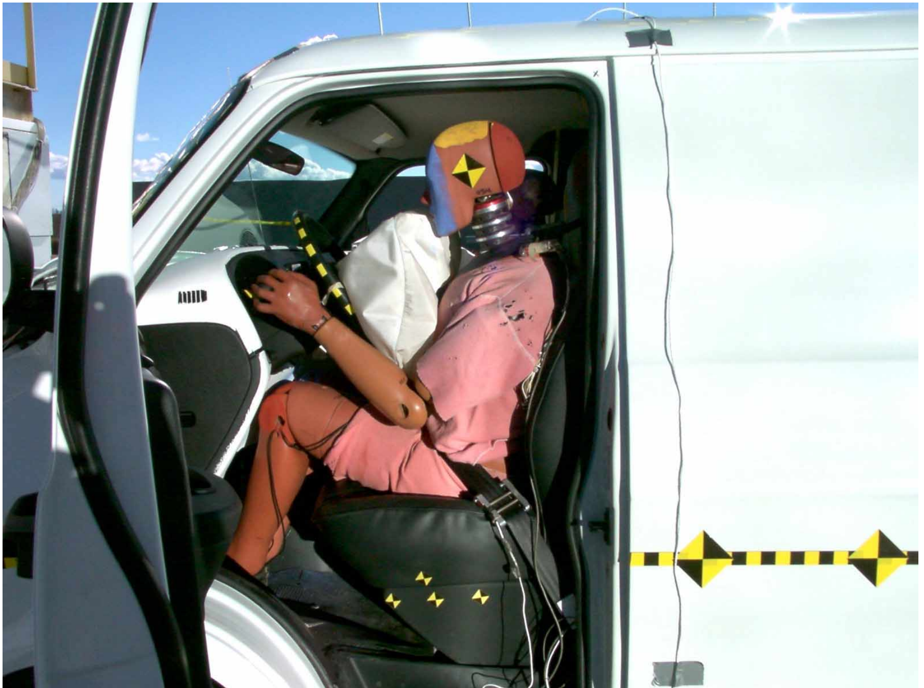
Figure A-32: Driver Dummy 90° To Vehicle, Post-Test
