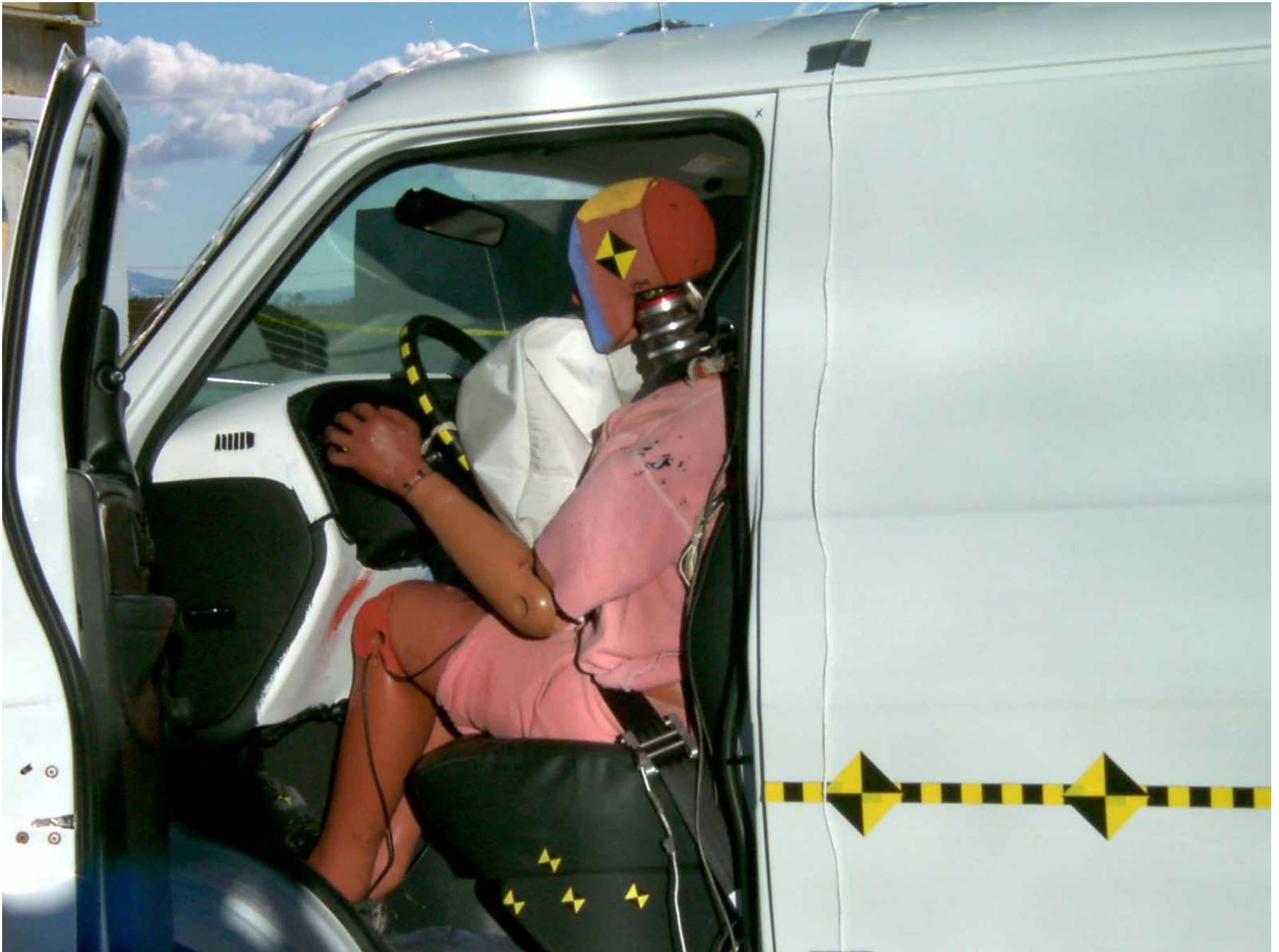
Figure A-30: Driver Dummy Door Open, Post-Test
