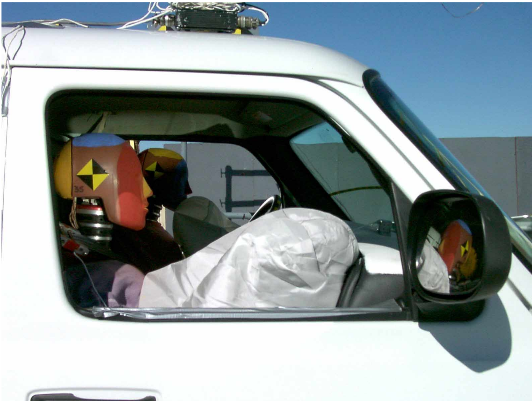
Figure A-44: Passenger Dummy Through Window, Post-Test
