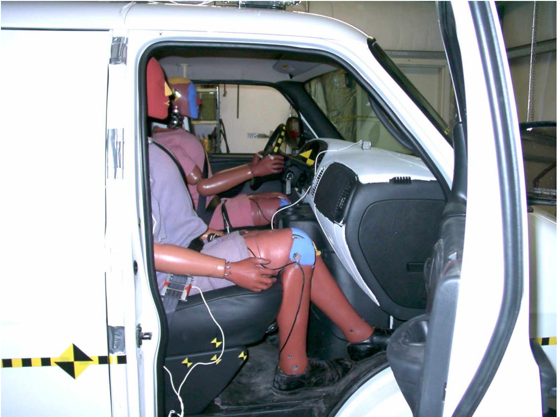
Figure A-47: Passenger Dummy 90° To Vehicle, Pre-Test
