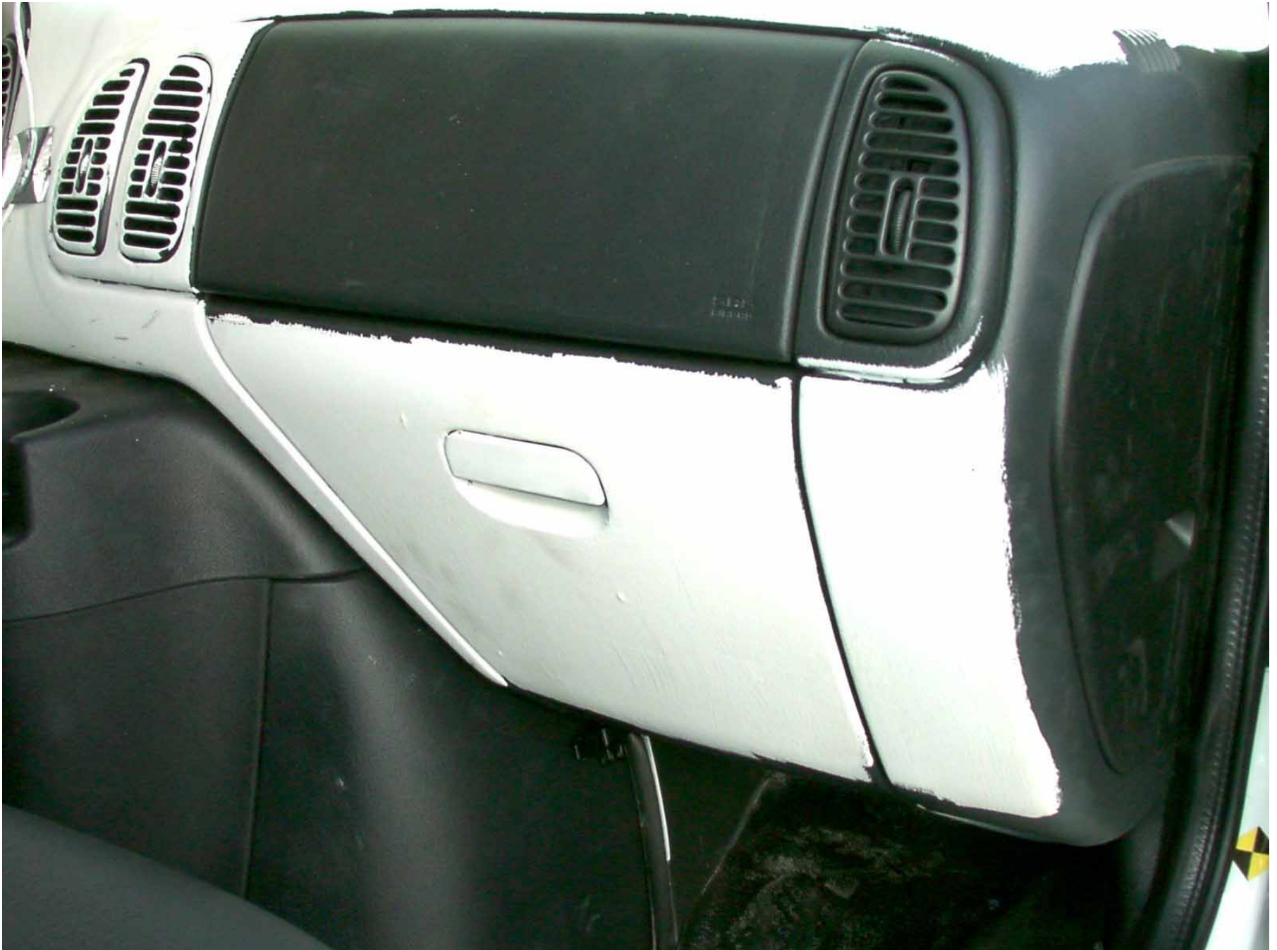
Figure A-53: Passenger Side Knee Bolster, Pre-Test
