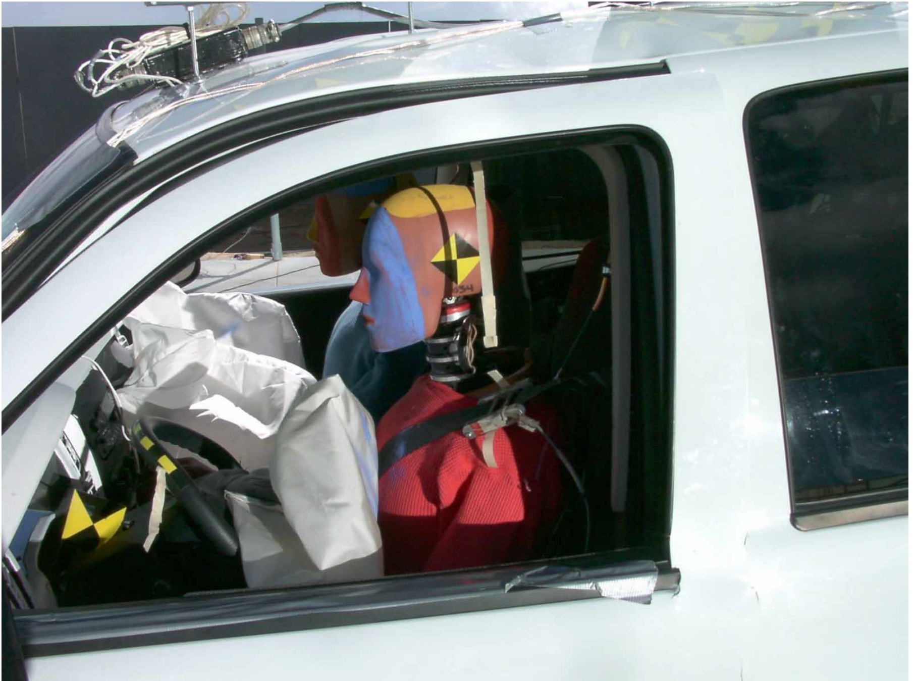
Figure A-28: Driver Dummy Through Window, Post-Test
