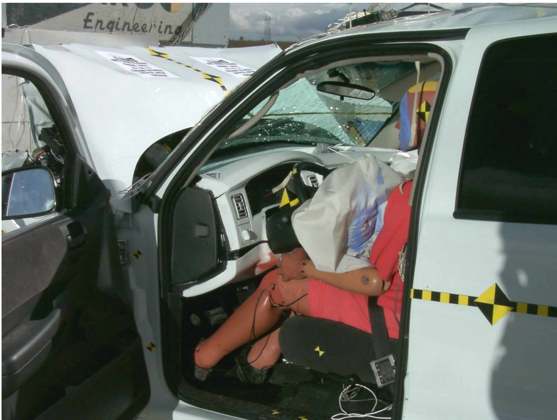
Figure A-30: Driver Dummy Door Open, Post-Test
