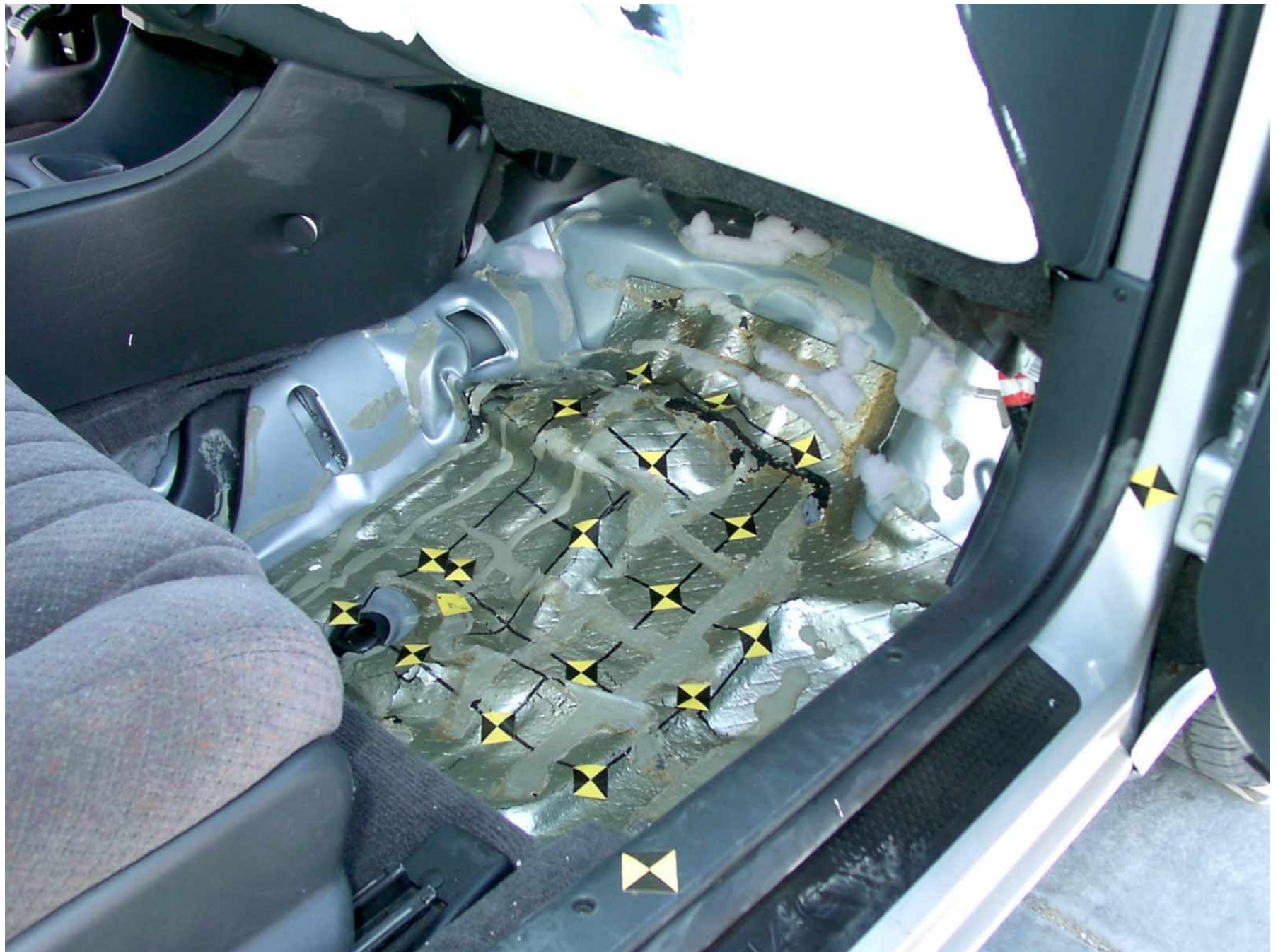
Figure A-52: Passenger Side Floor Pan, Post-Test
