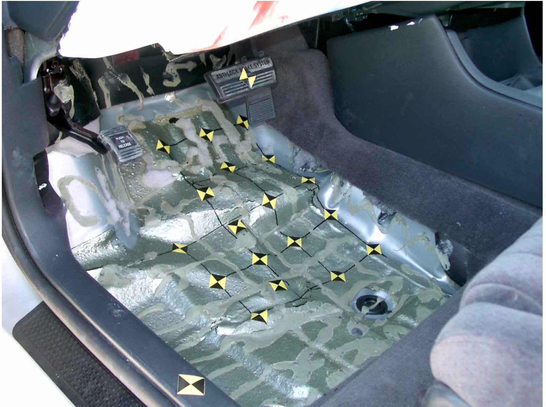
Figure A-38: Driver Side Floor Pan, Post-Test
