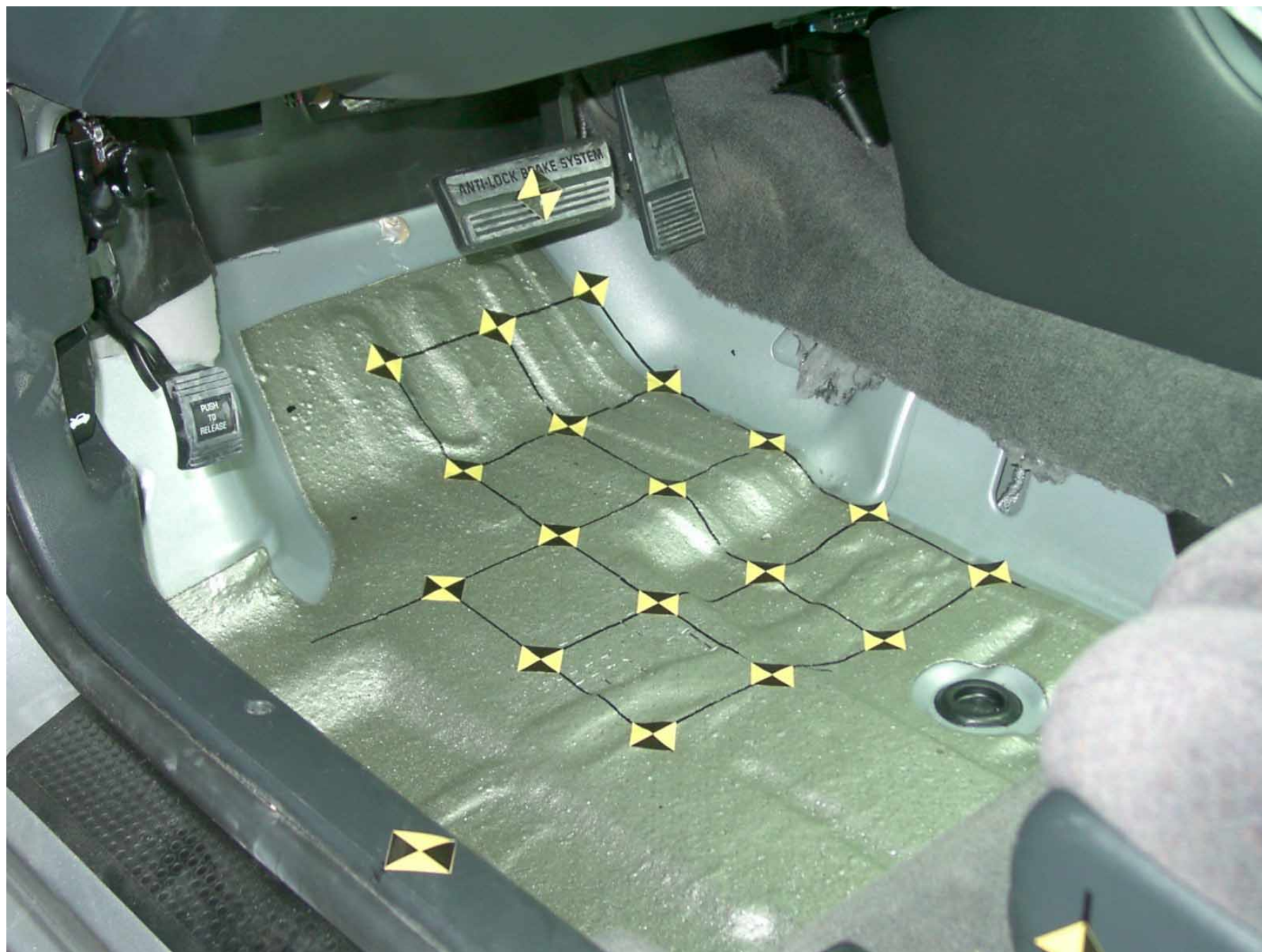
Figure A-37: Driver Side Floor Pan, Pre-Test
