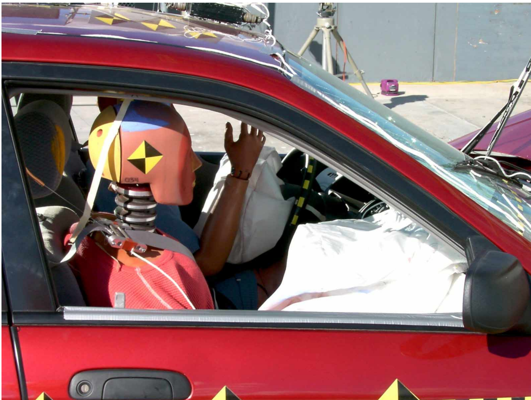
Figure A-44: Passenger Dummy Through Window, Post-Test
