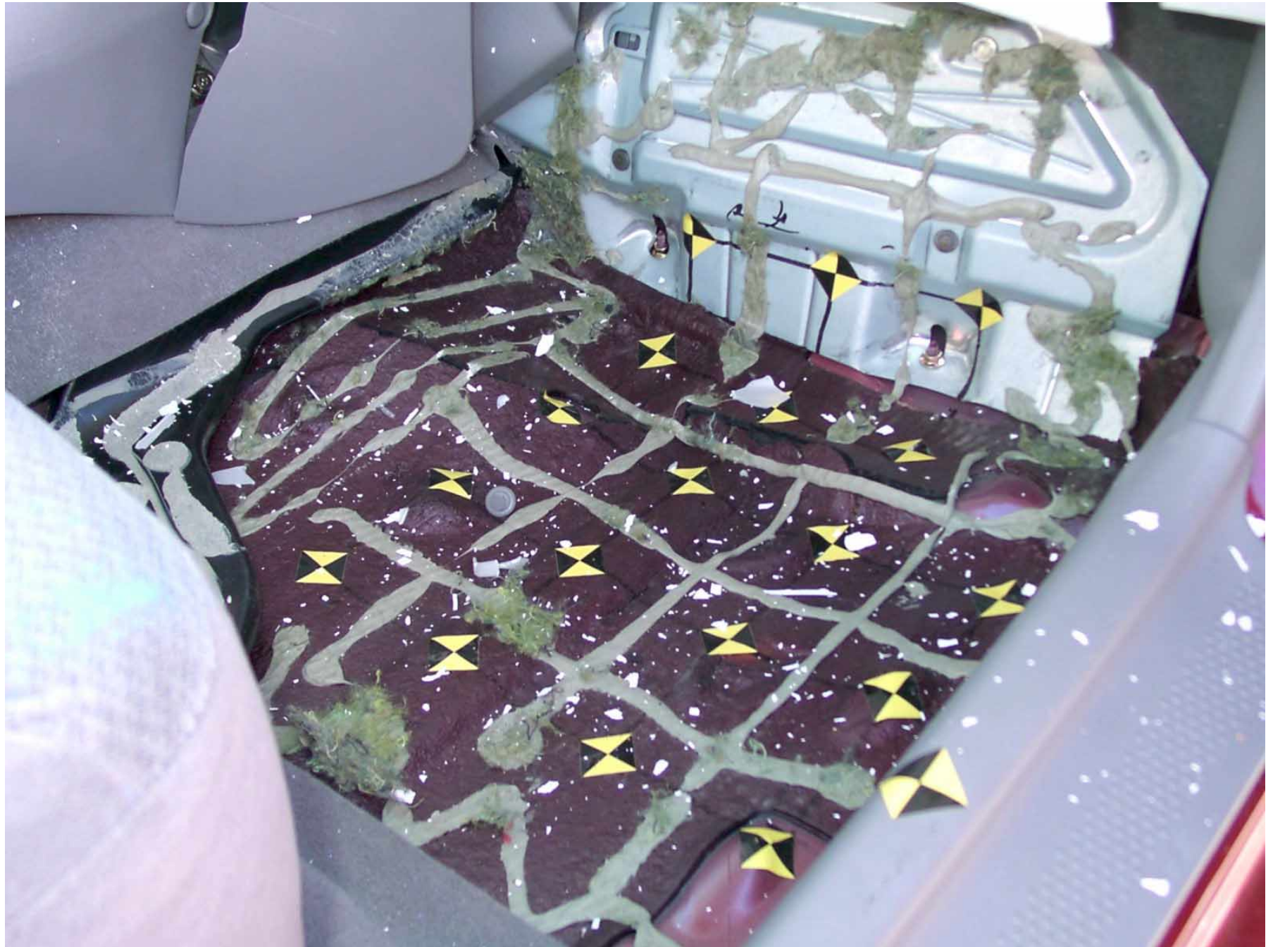
Figure A-52: Passenger Side Floor Pan, Post-Test
