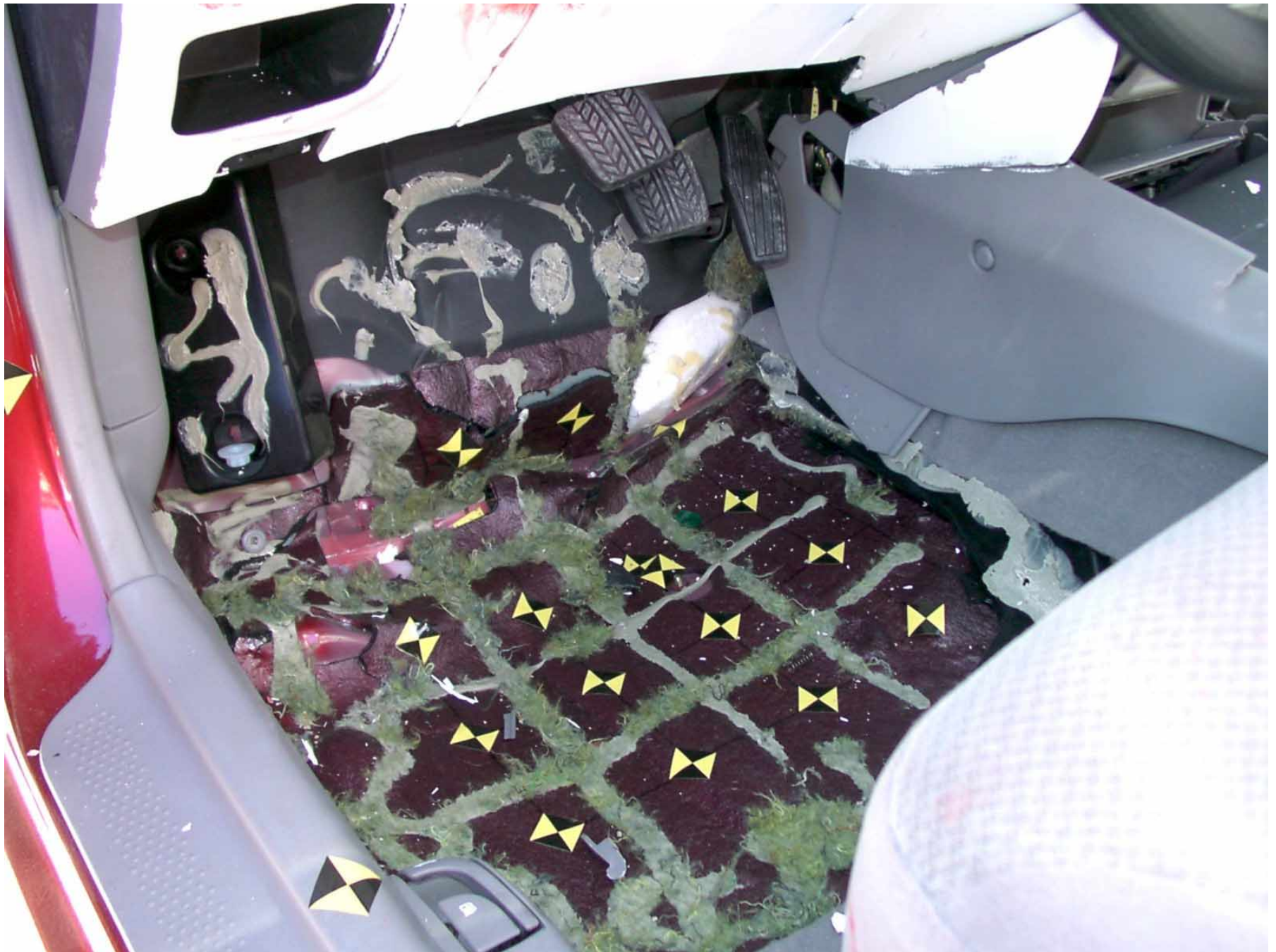
Figure A-38: Driver Side Floor Pan, Post-Test
