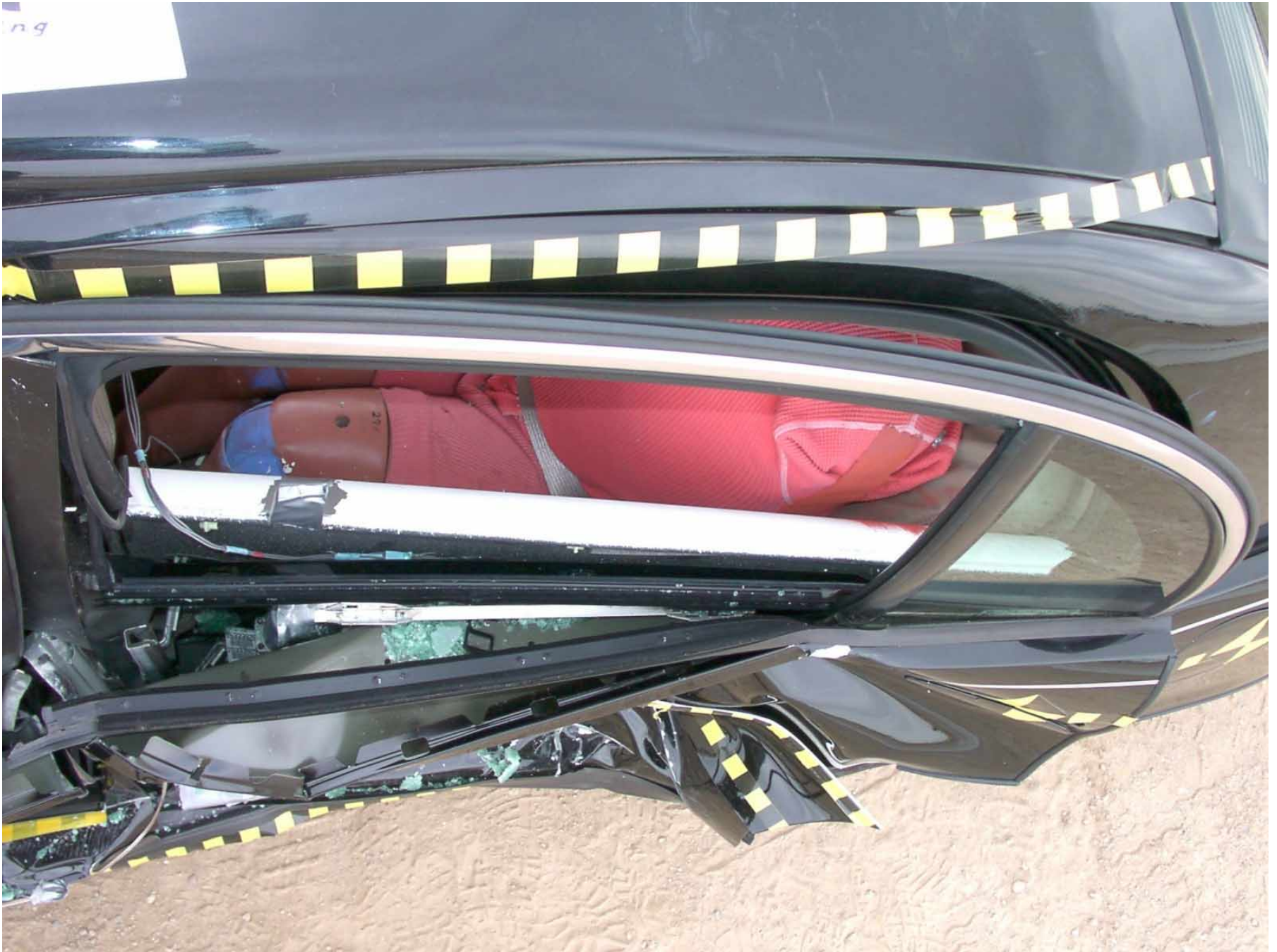
Figure A-31: Passenger Dummy Clearance, Post-Test
