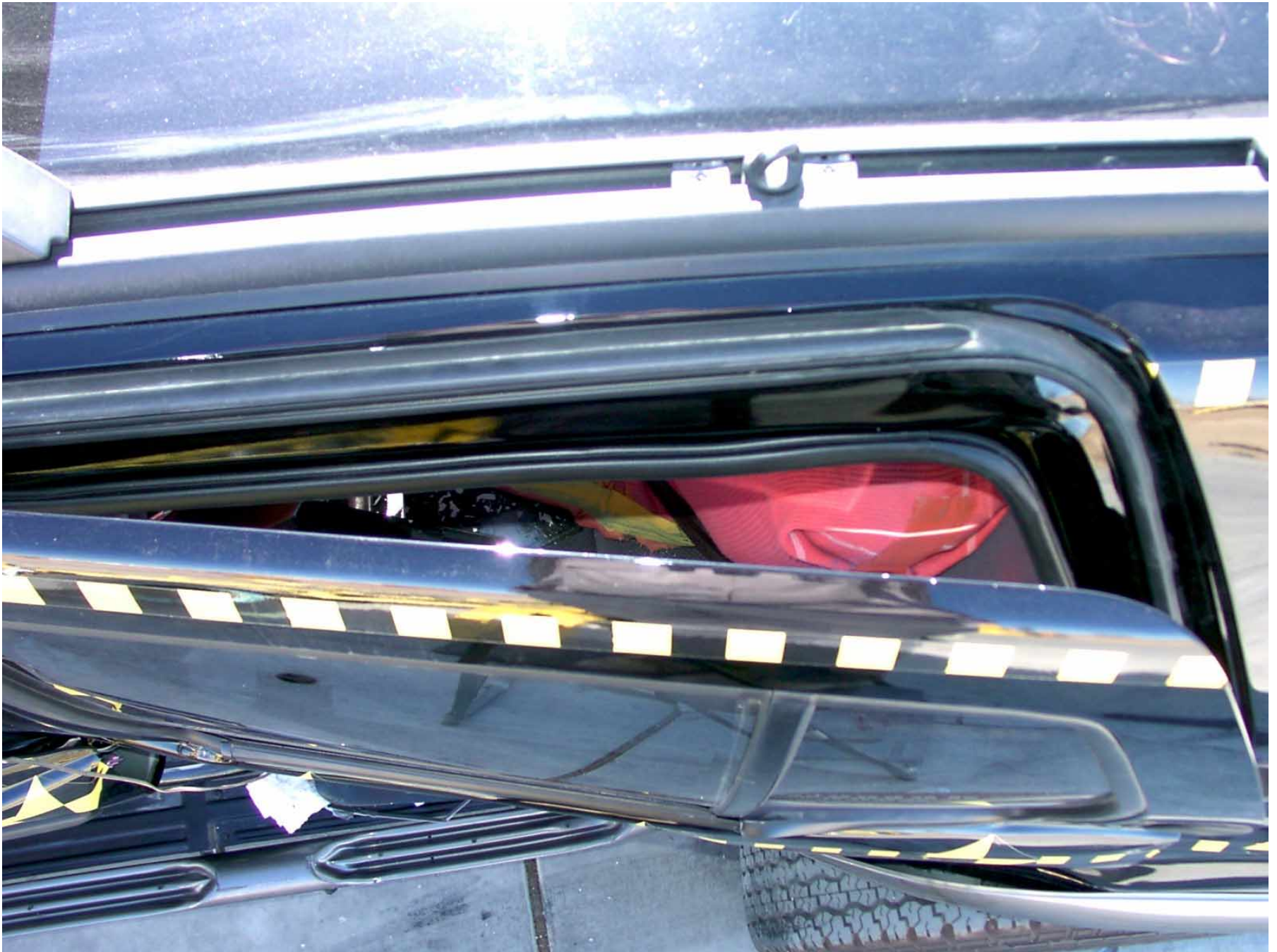
Figure A-31: Passenger Dummy Clearance, Post-Test
