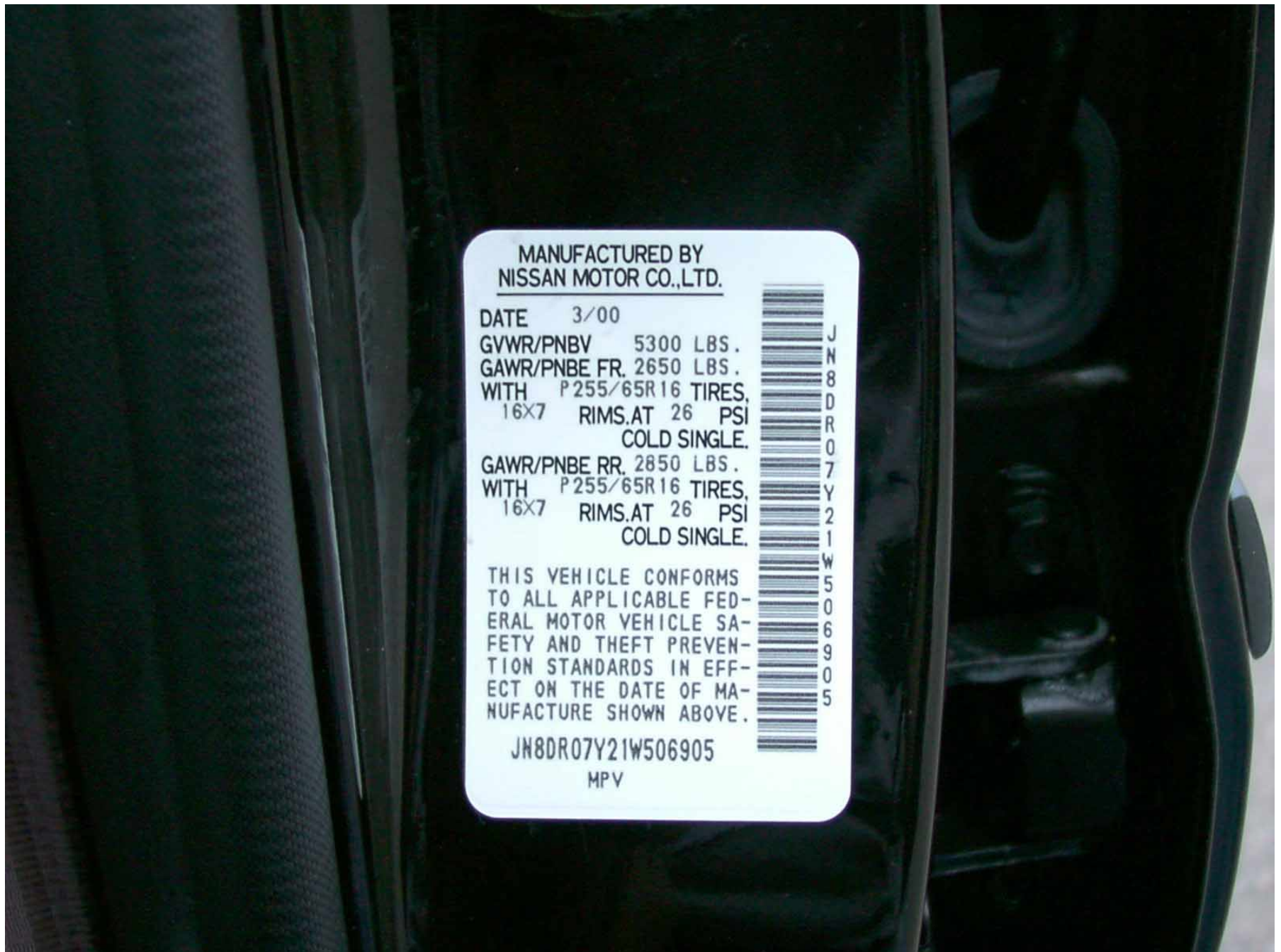
Figure A-3: Vehicle Certification Label
