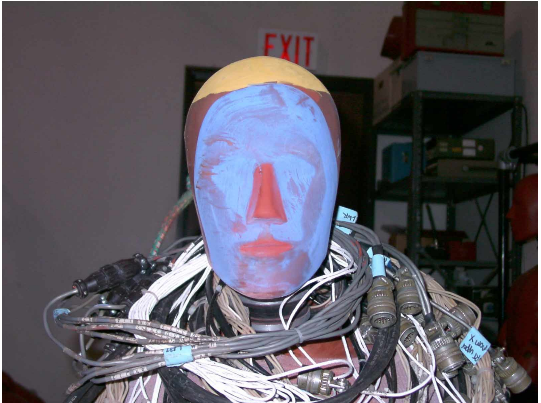
Figure A-39: Driver Dummy Head, Post-Test
