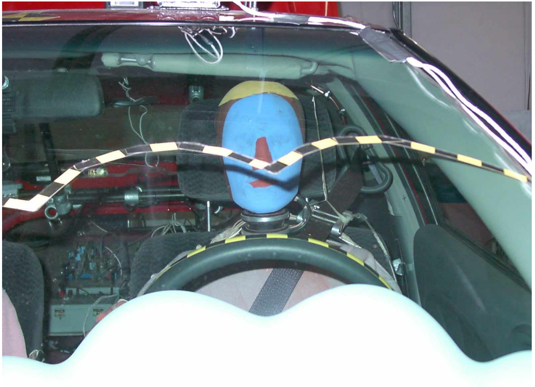
Figure A-25: Driver Dummy Front View, Pre-Test
