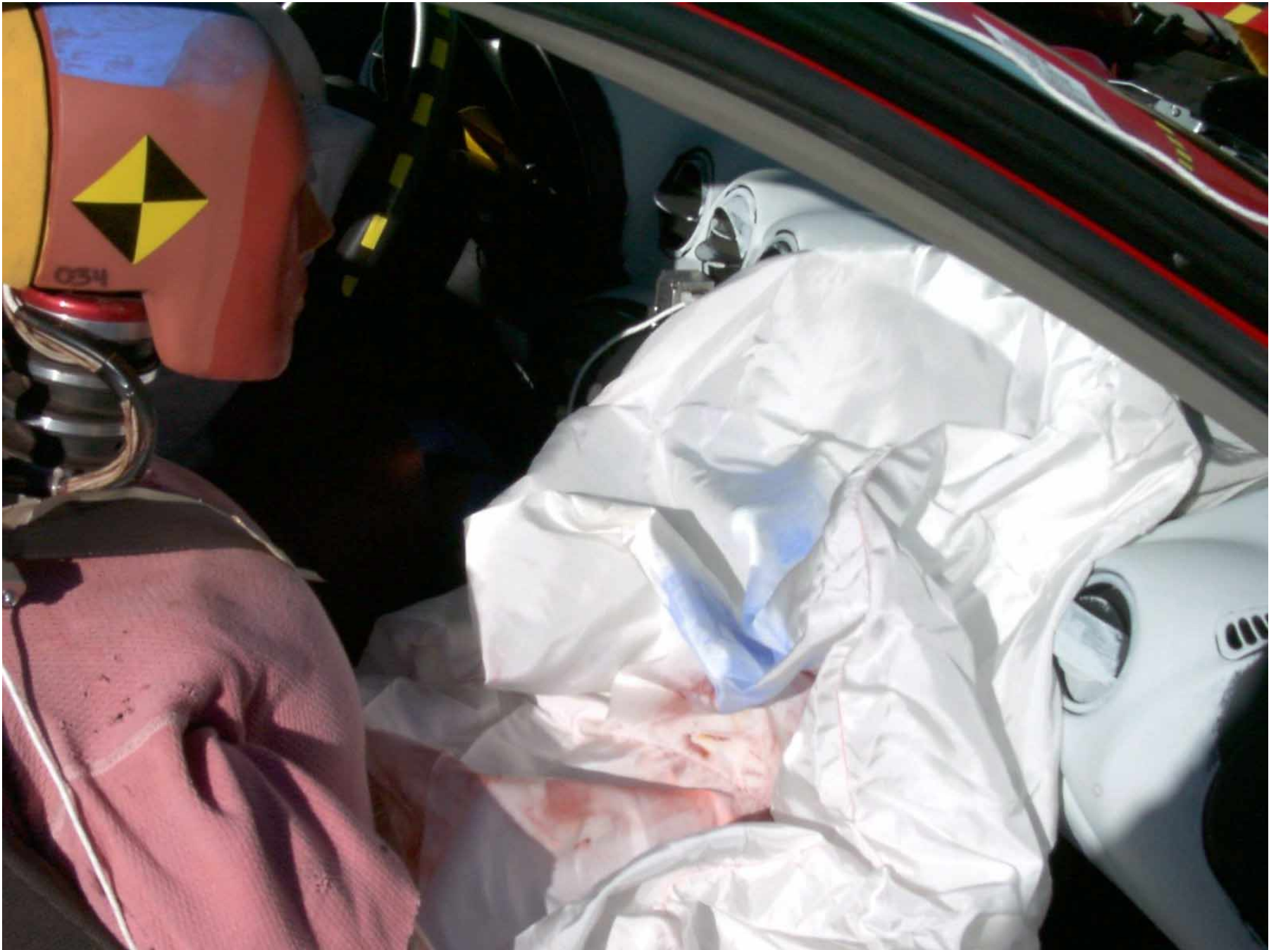
Figure A-56: Passenger Dummy Contact, Post-Test
