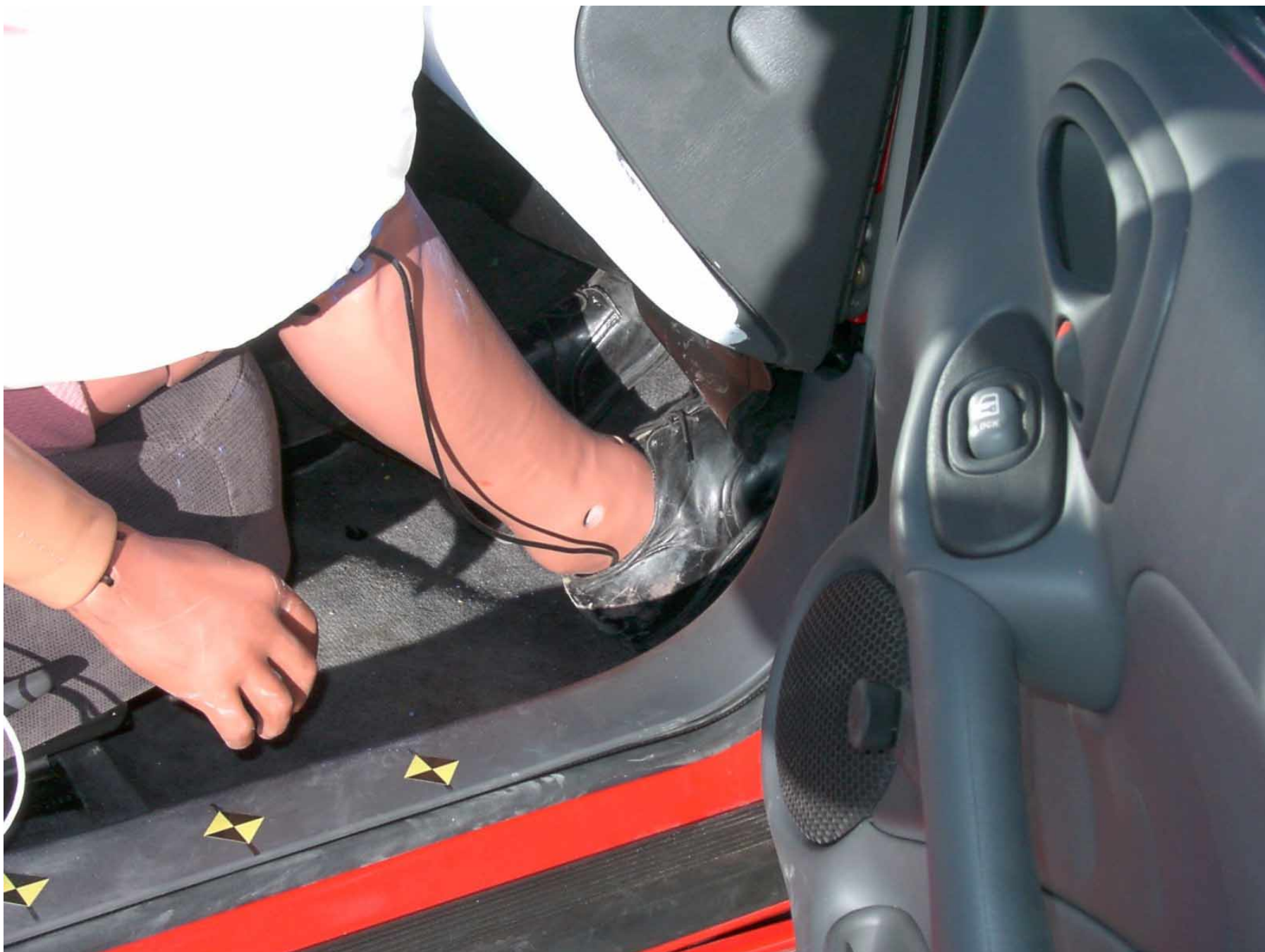
Figure A-50: Passenger Dummy Feet and Knee Contact, Post-Test
