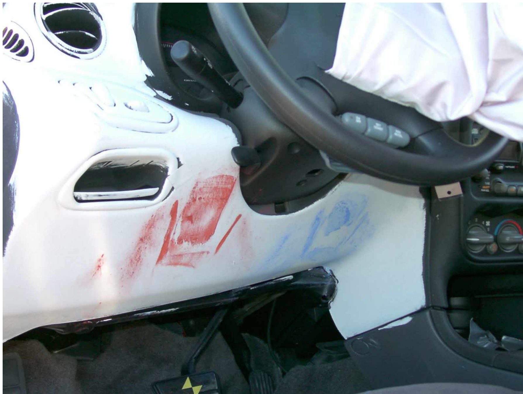
Figure A-36: Driver Side Knee Bolster, Post-Test
