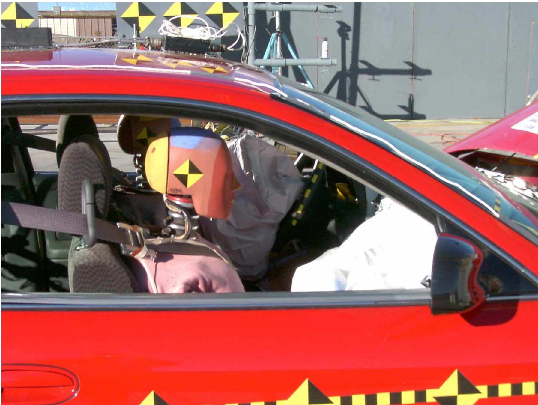
Figure A-44: Passenger Dummy Through Window, Post-Test
