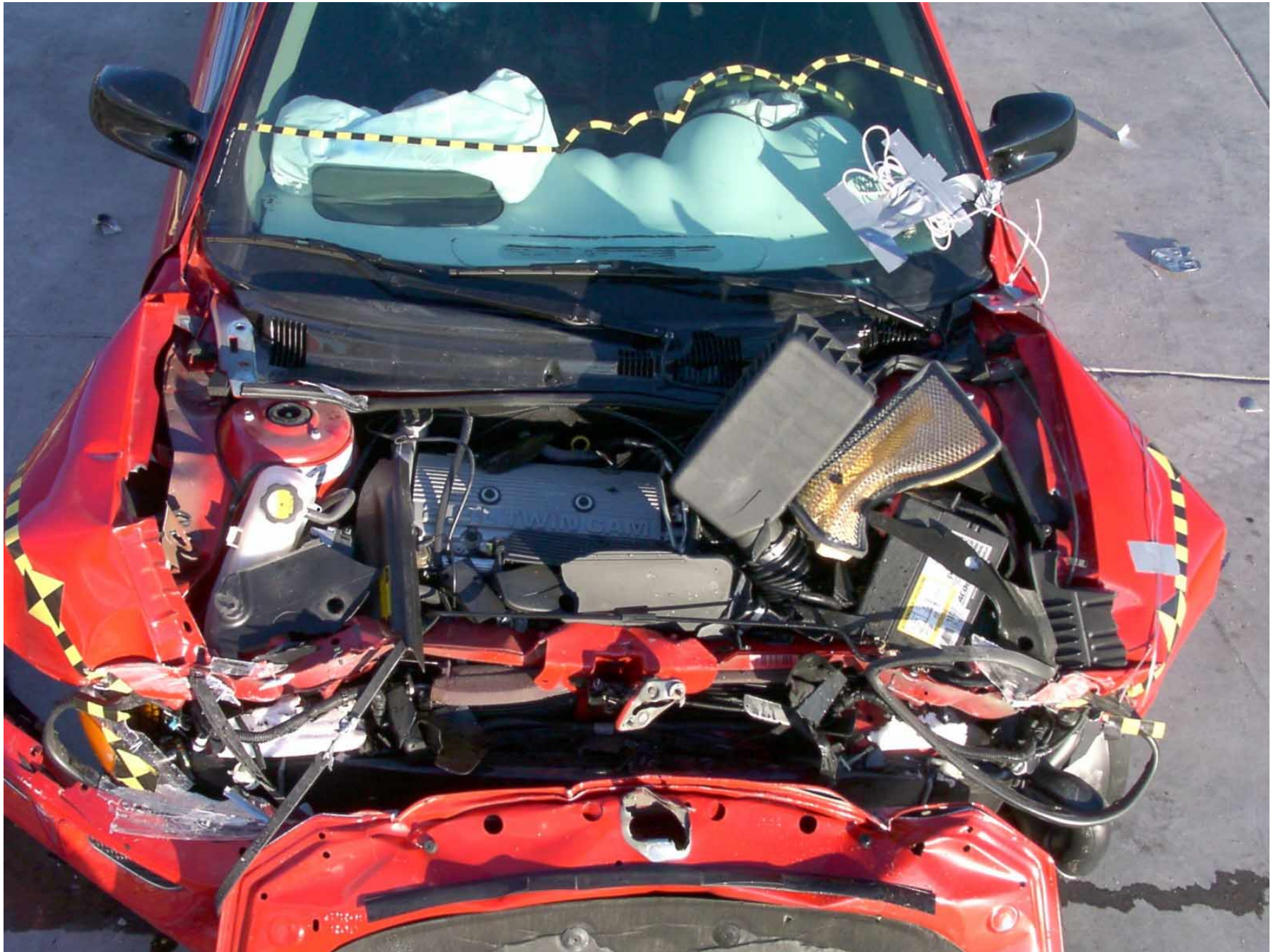
Figure A-18: Engine Compartment, Post-Test
