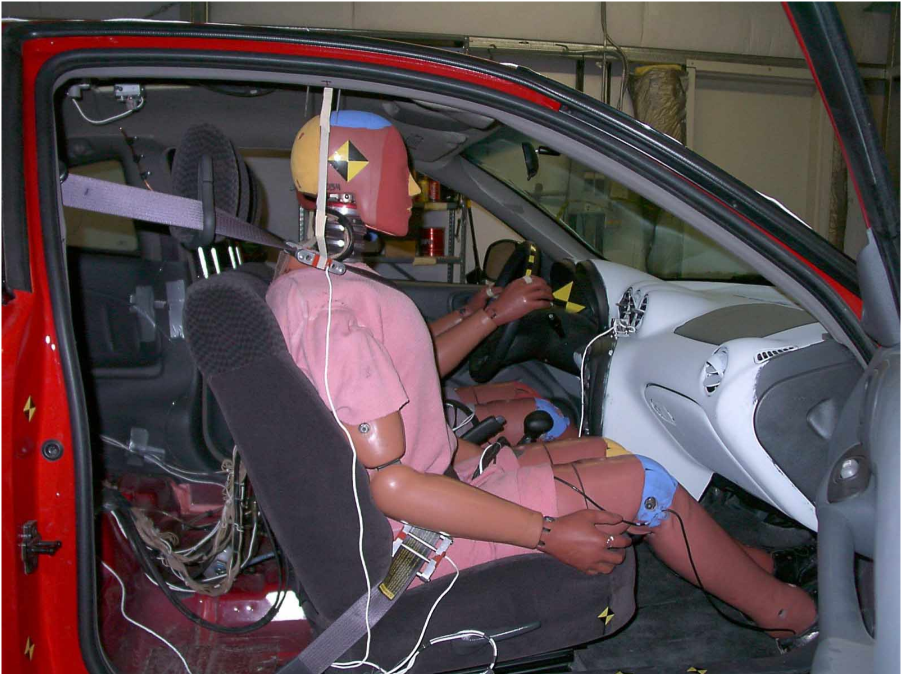
Figure A-47: Passenger Dummy 90° To Vehicle, Pre-Test
