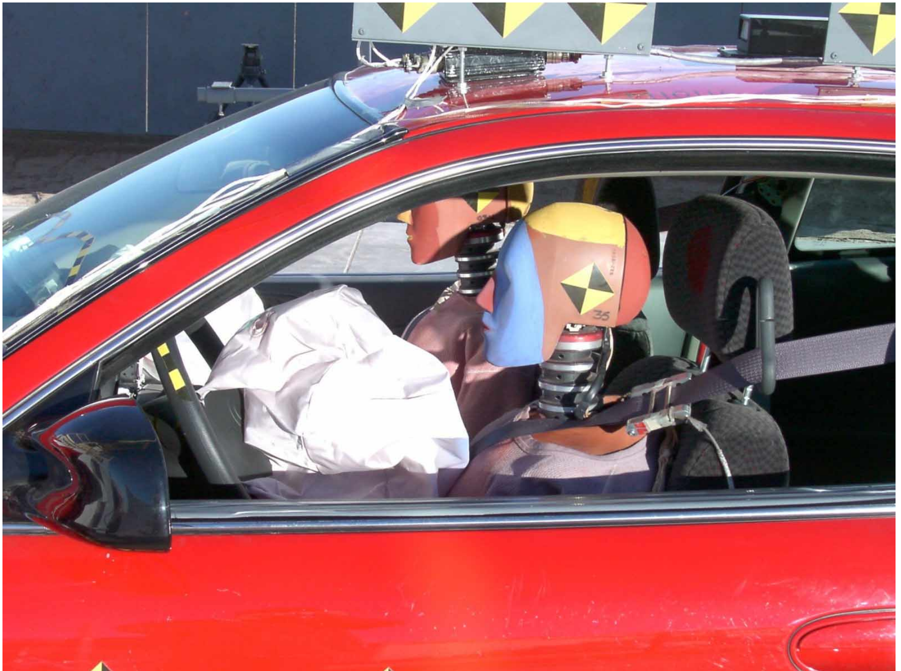
Figure A-28: Driver Dummy Through Window, Post-Test
