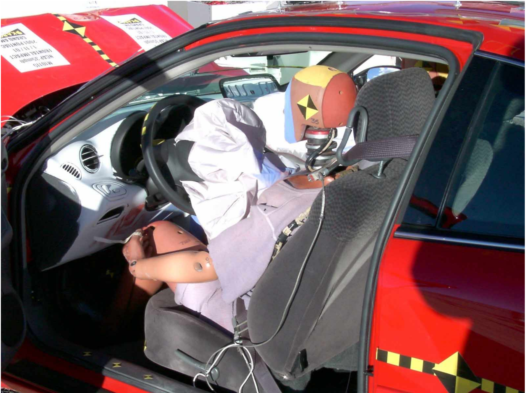
Figure A-30: Driver Dummy Door Open, Post-Test
