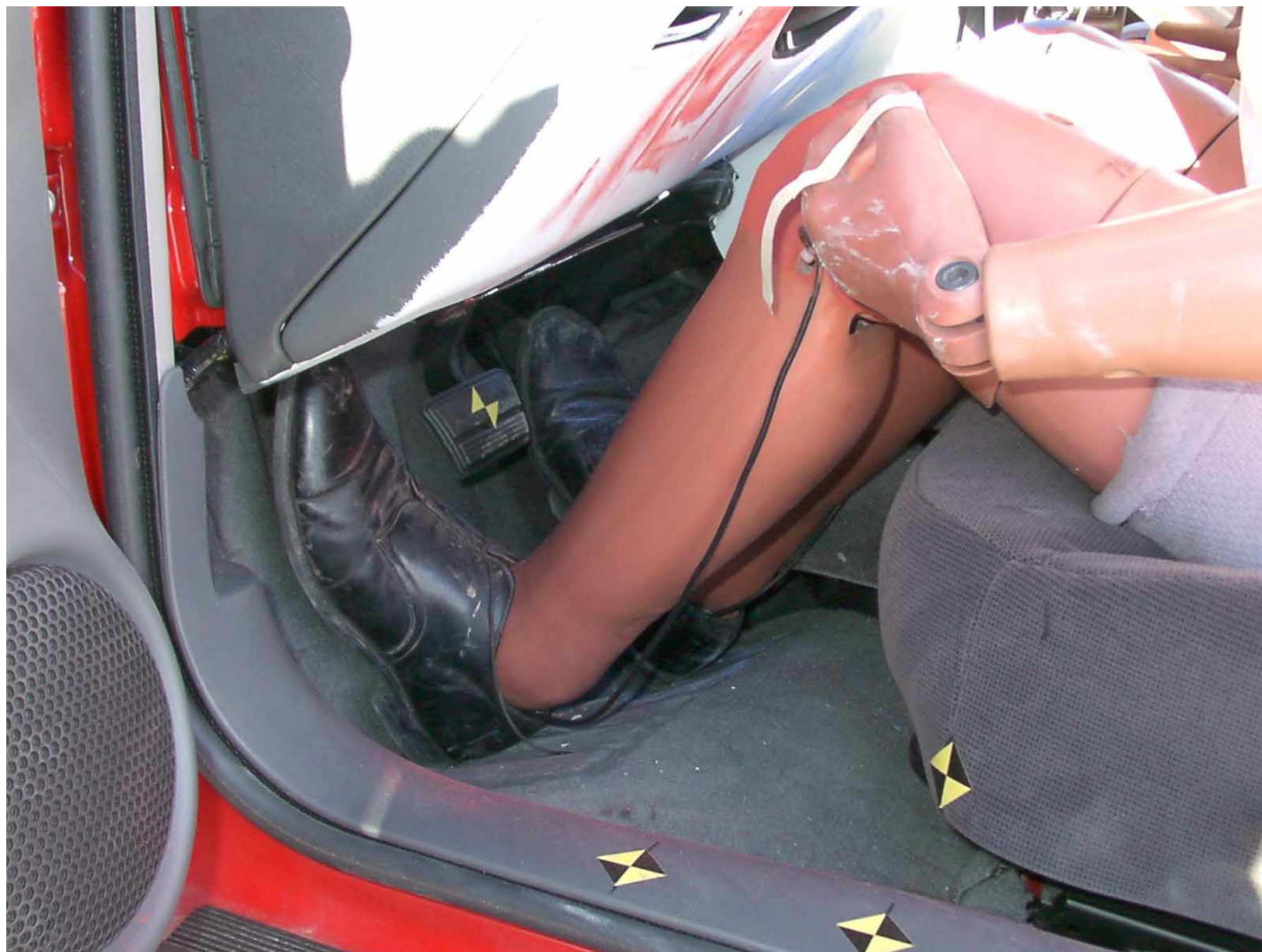
Figure A-34: Driver Dummy Feet and Knee Contact, Post-Test
