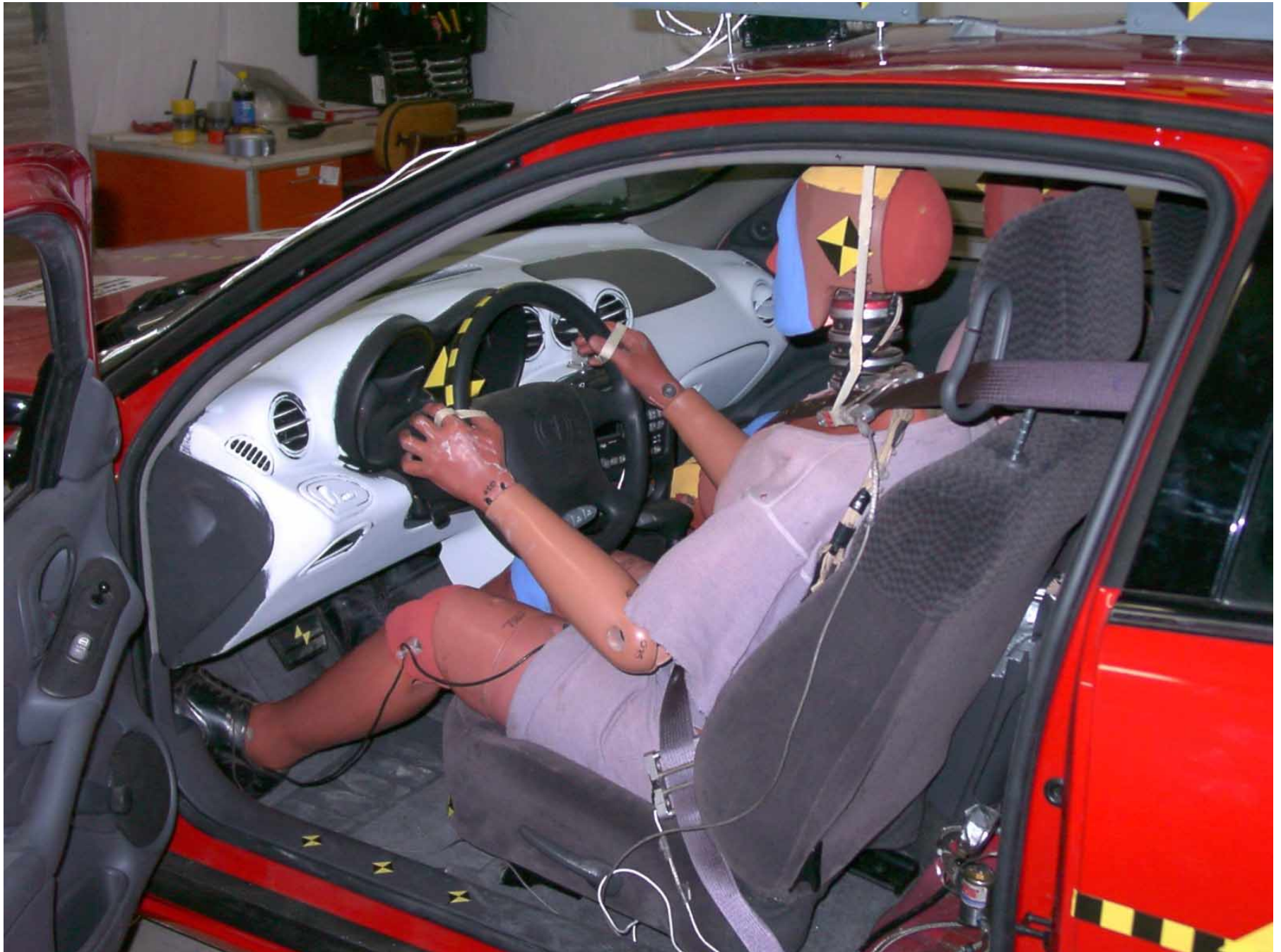
Figure A-29: Driver Dummy Door Open, Pre-Test
