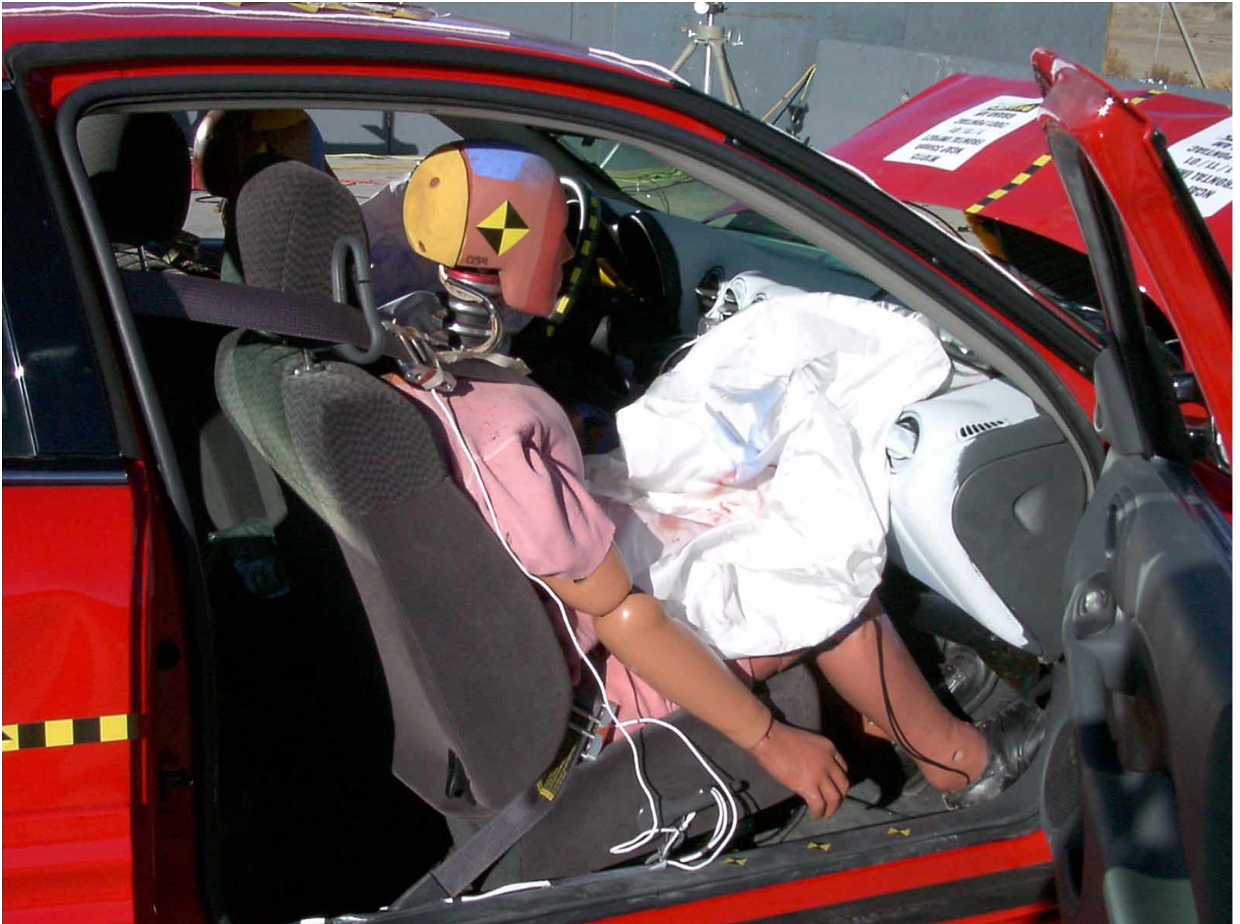
Figure A-48: Passenger Dummy 90° To Vehicle, Post-Test
