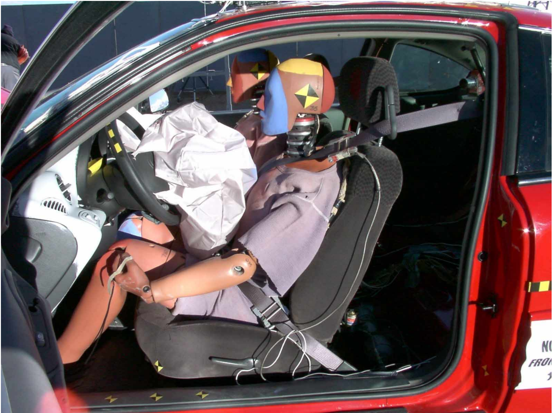
Figure A-32: Driver Dummy 90° To Vehicle, Post-Test
