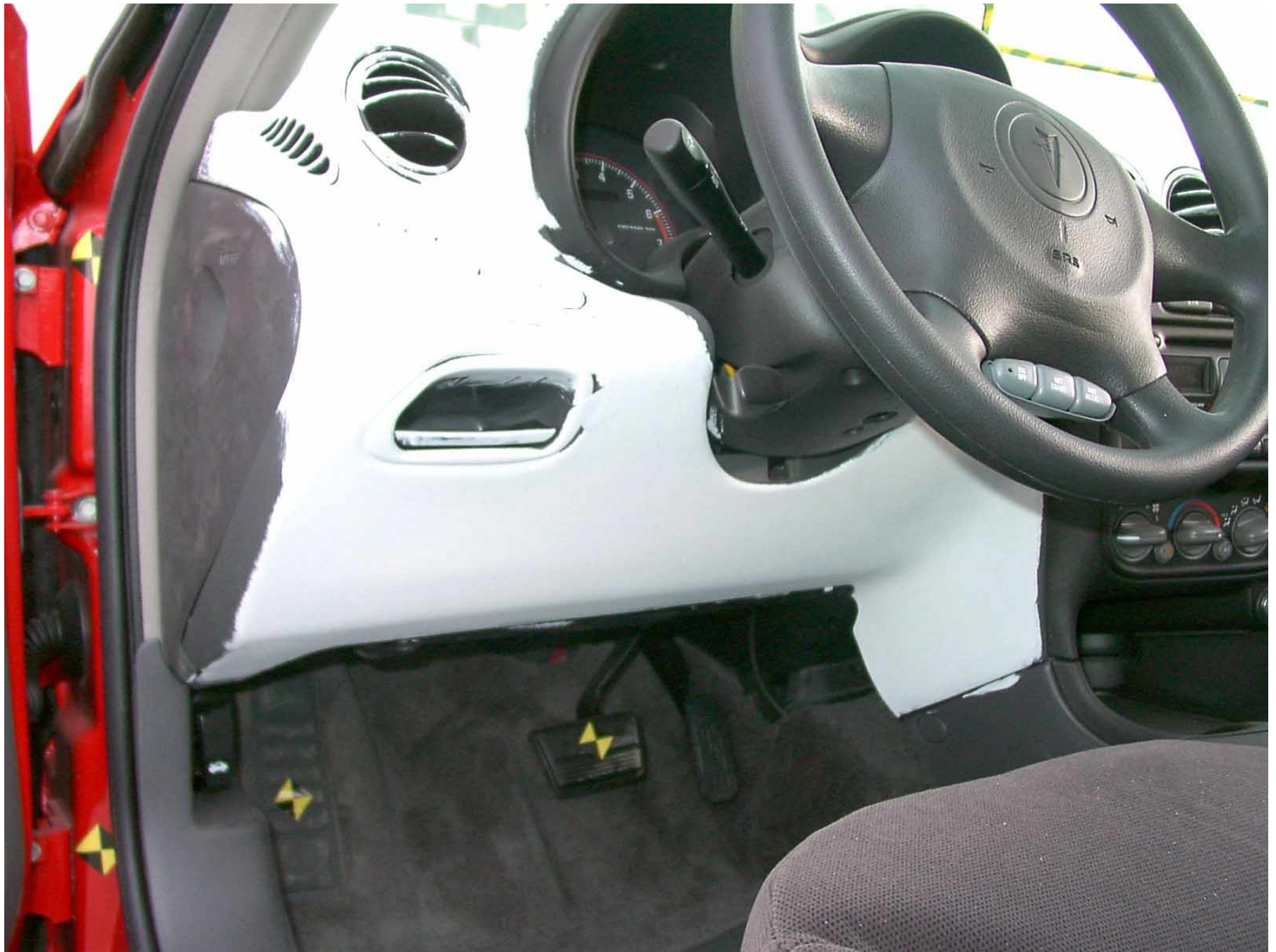
Figure A-35: Driver Side Knee Bolster, Pre-Test
