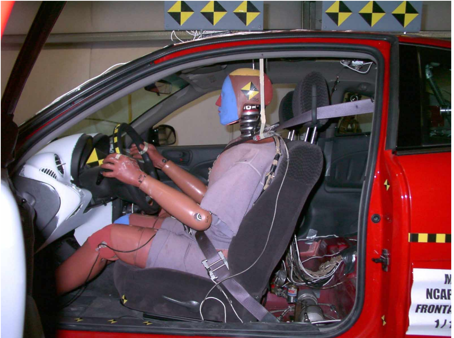
Figure A-31: Driver Dummy 90° To Vehicle, Pre-Test
