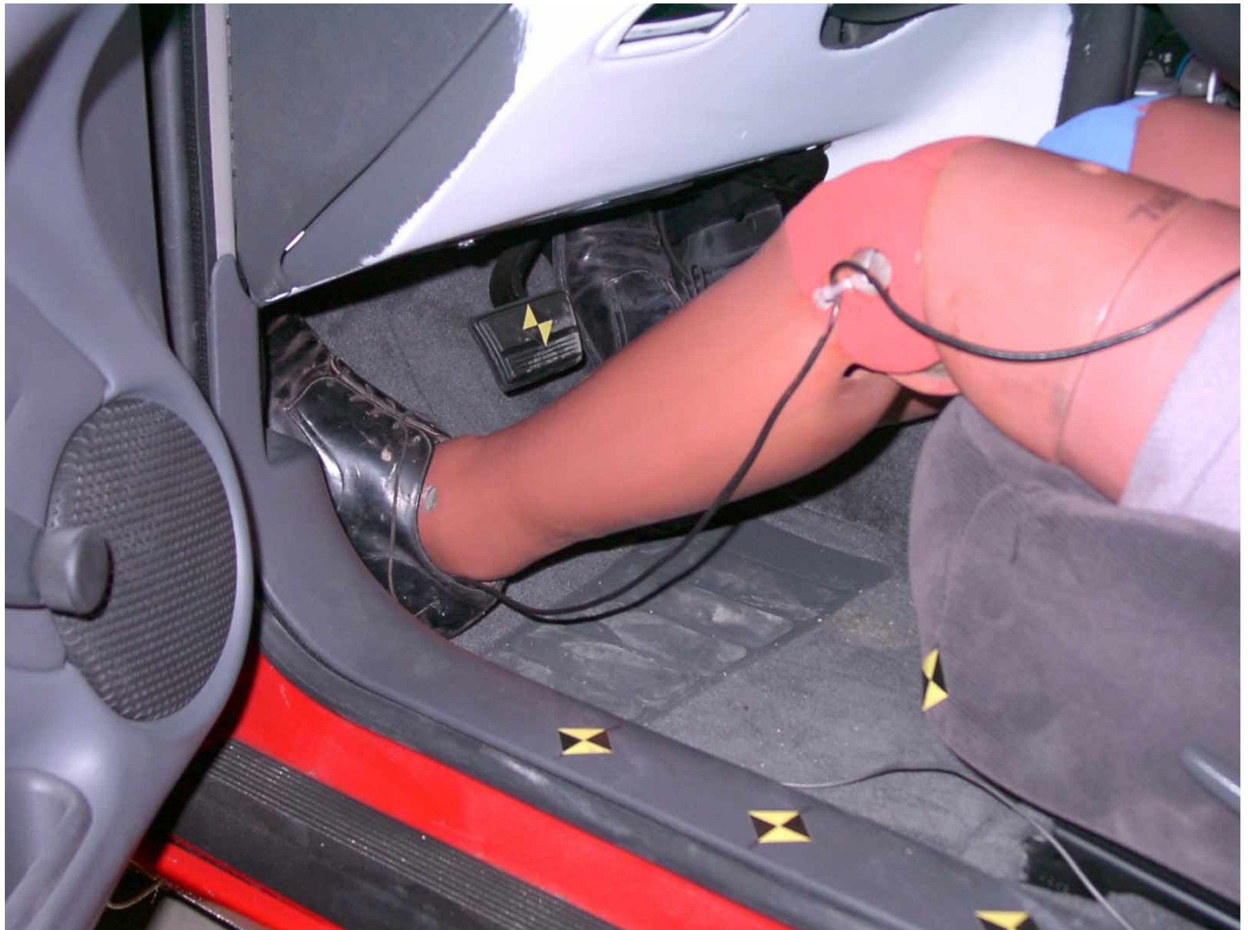
Figure A-33: Driver Dummy Feet, Pre-Test
