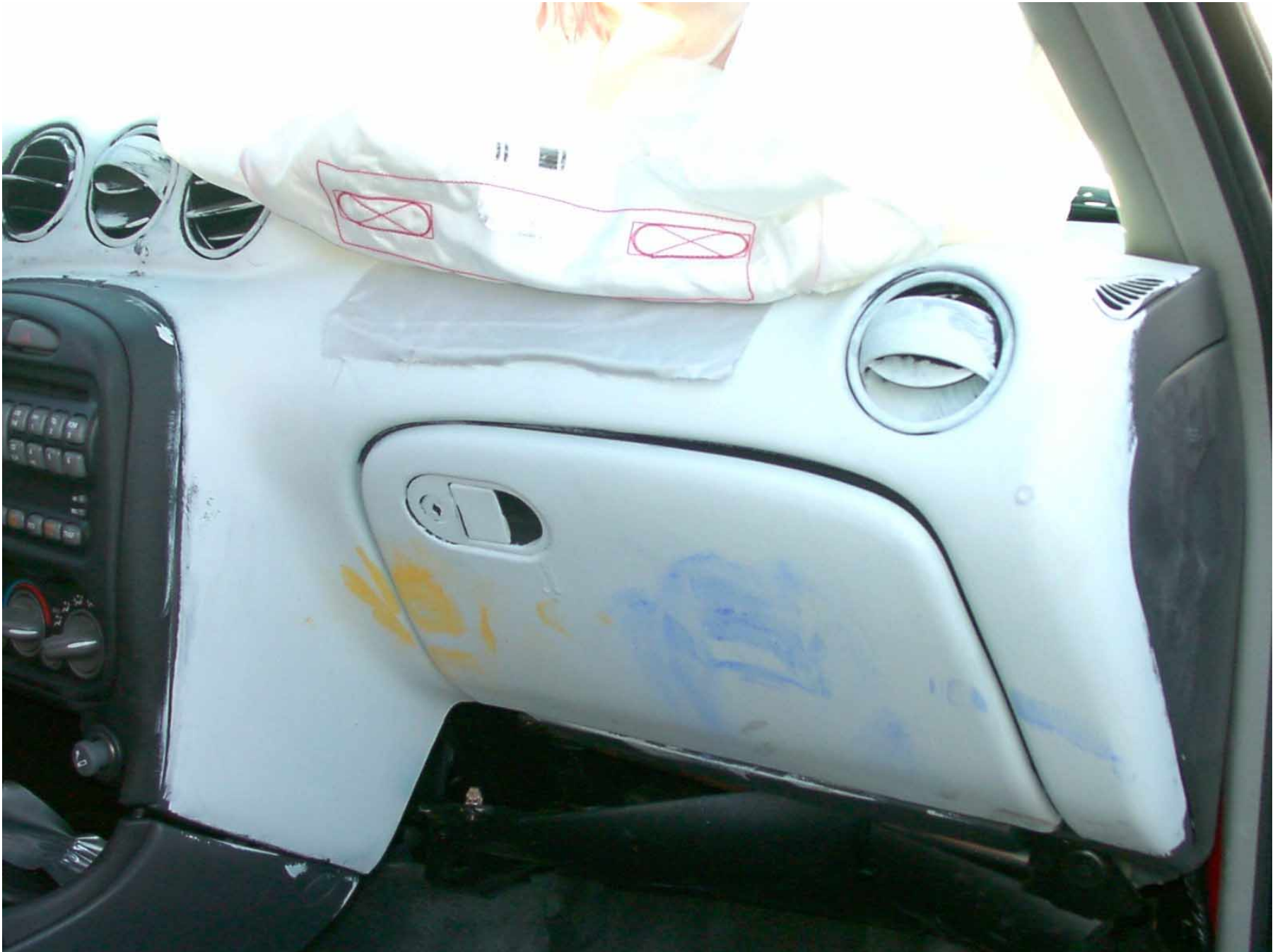
Figure A-54: Passenger Side Knee Bolster, Post-Test
