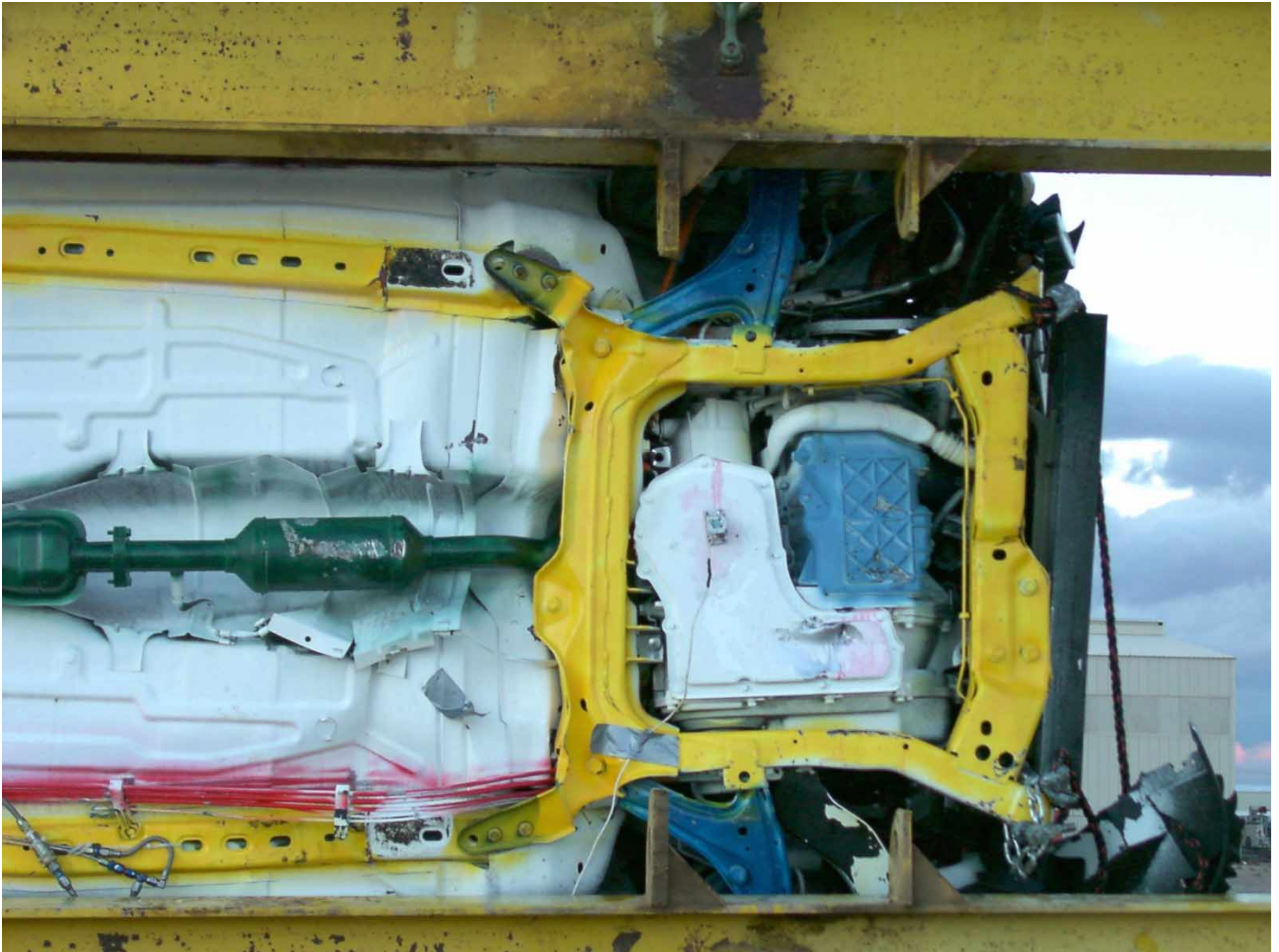
Figure A-22: Front Underside, Post-Test
