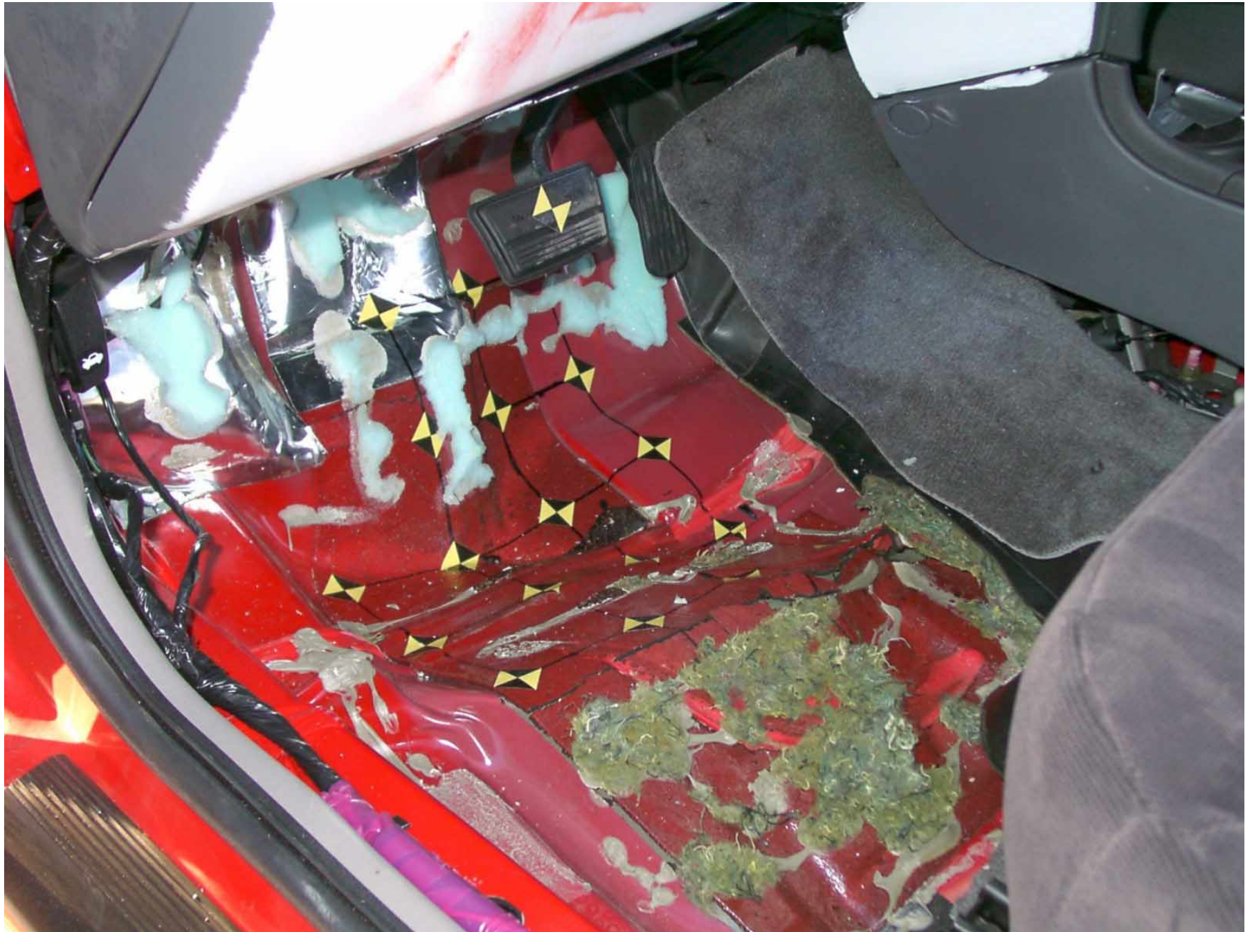
Figure A-38: Driver Side Floor Pan, Post-Test
