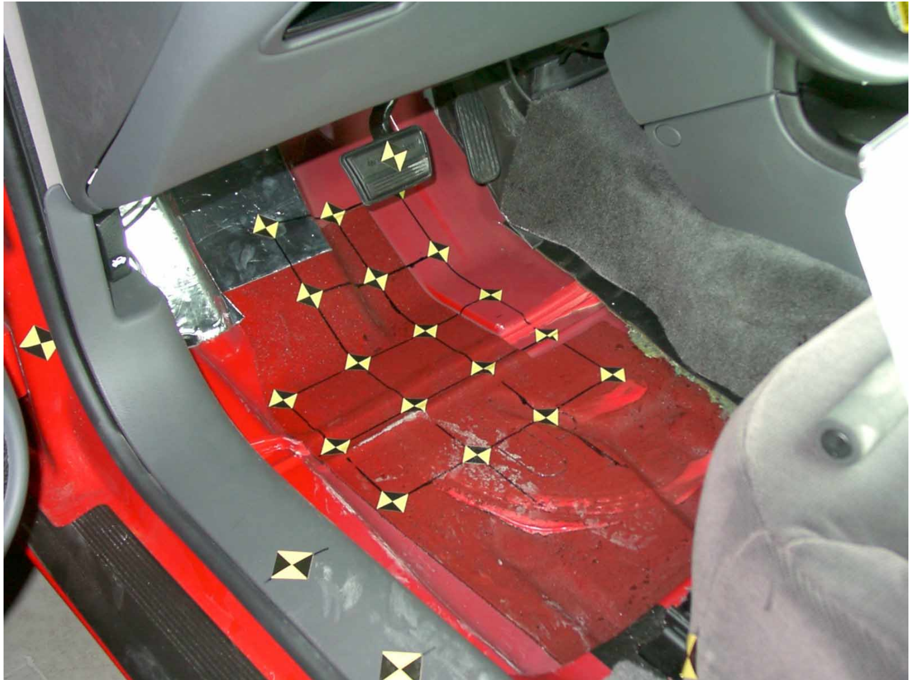
Figure A-37: Driver Side Floor Pan, Pre-Test
