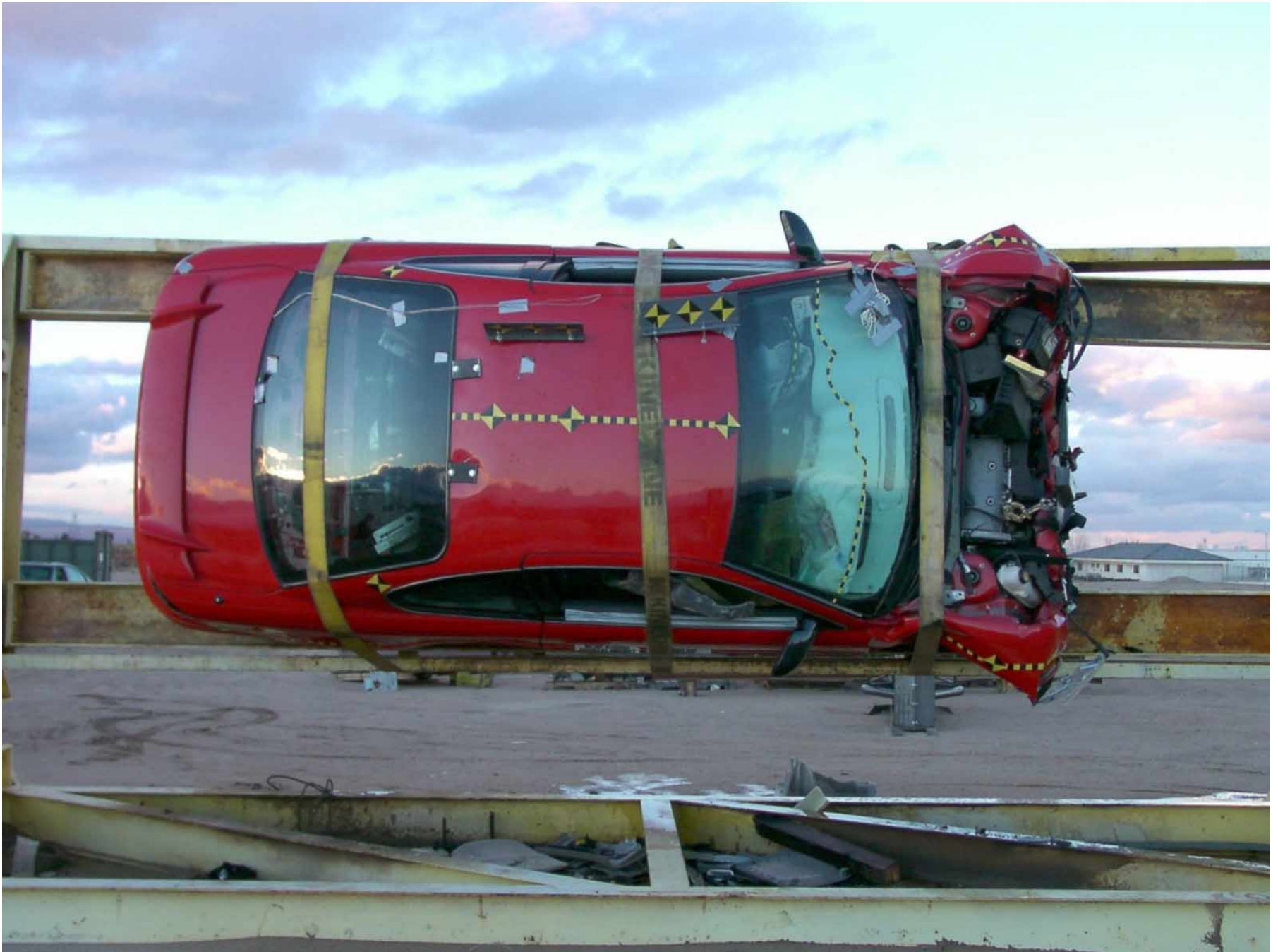
Figure A-57: Vehicle on Rollover Device
