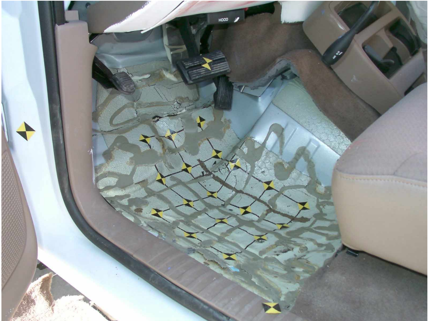
Figure A-38: Driver Side Floor Pan, Post-Test
