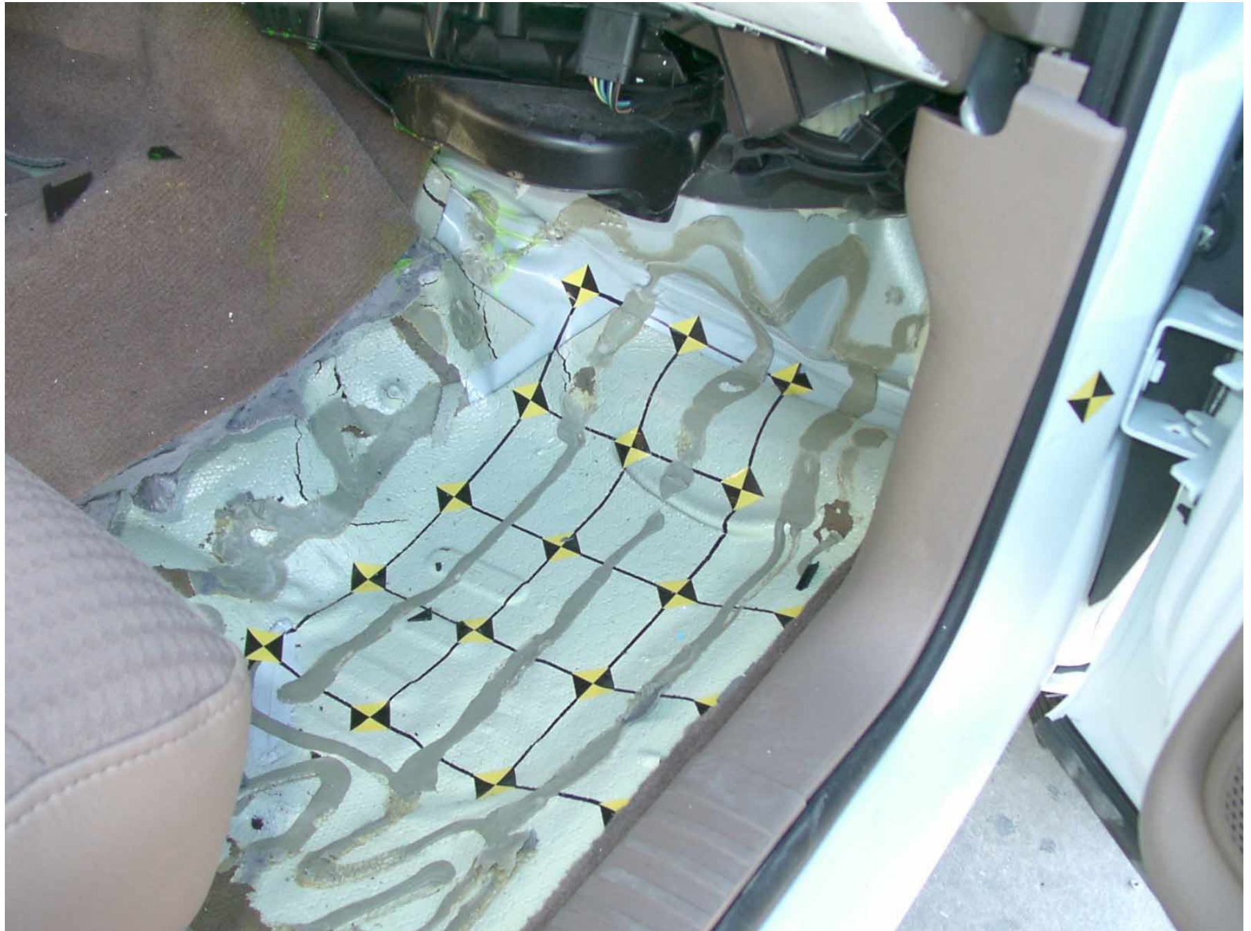
Figure A-52: Passenger Side Floor Pan, Post-Test
