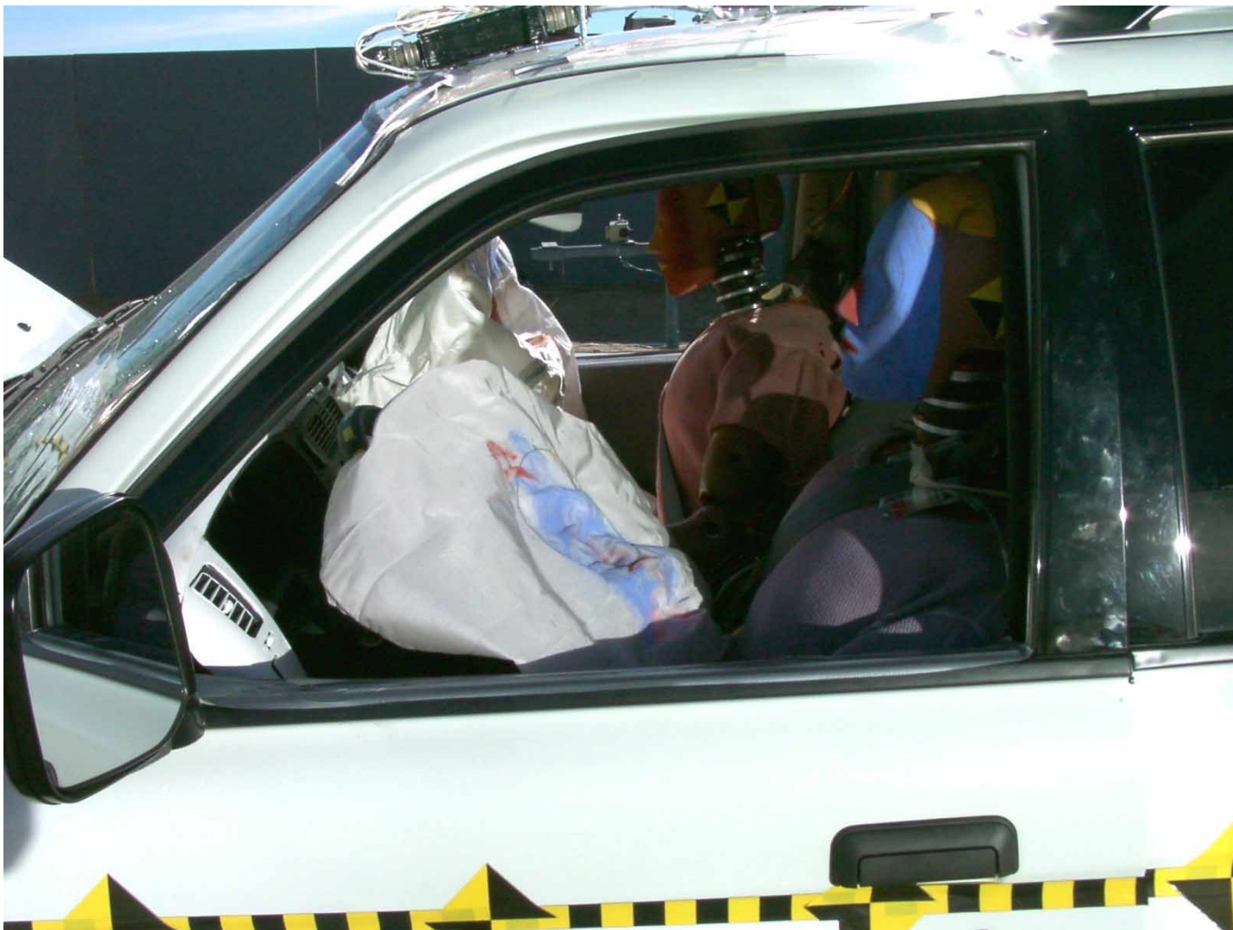
Figure A-28: Driver Dummy Through Window, Post-Test
