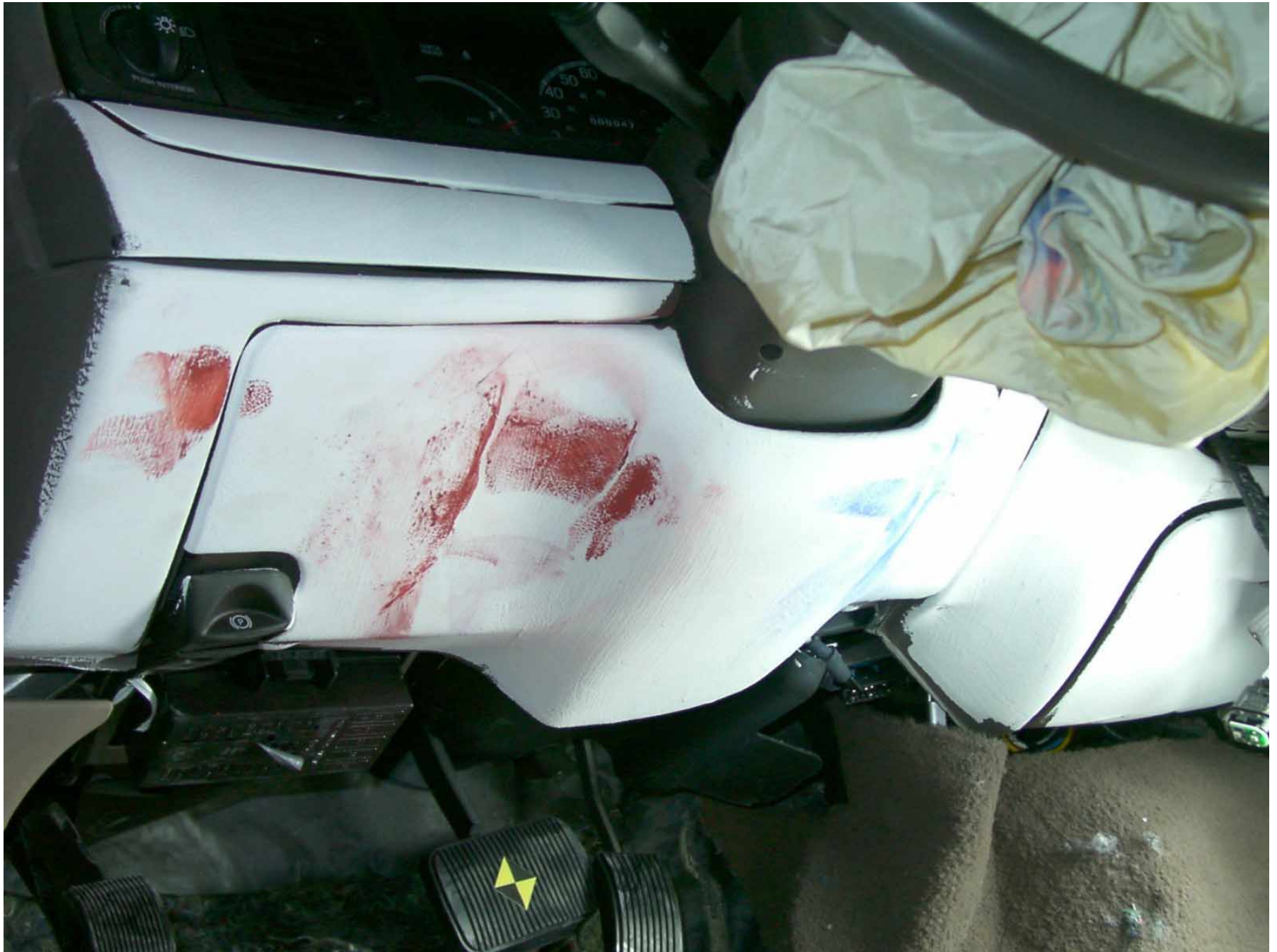
Figure A-36: Driver Side Knee Bolster, Post-Test
