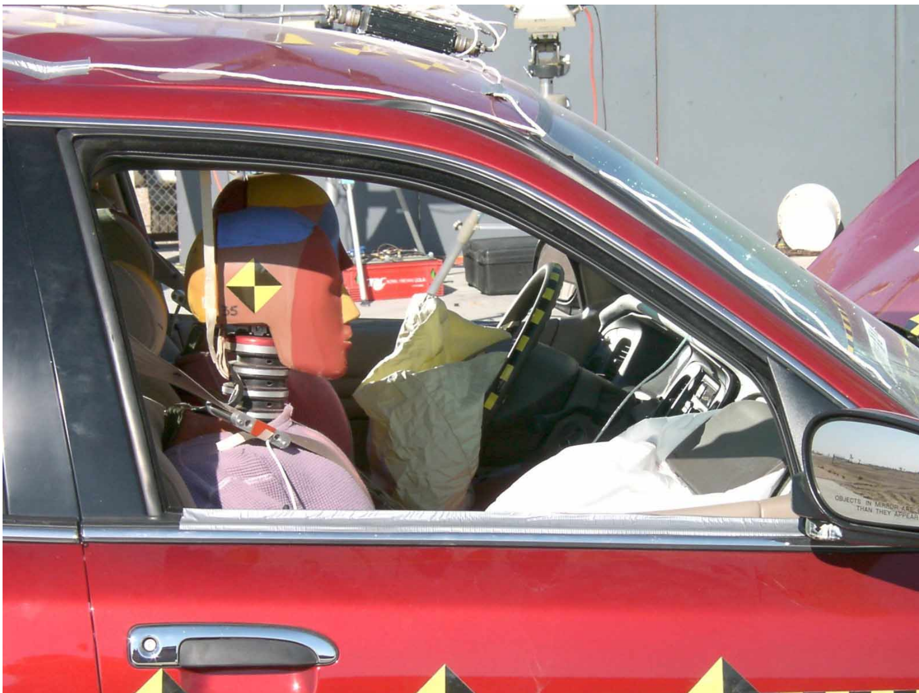
Figure A-44: Passenger Dummy Through Window, Post-Test
