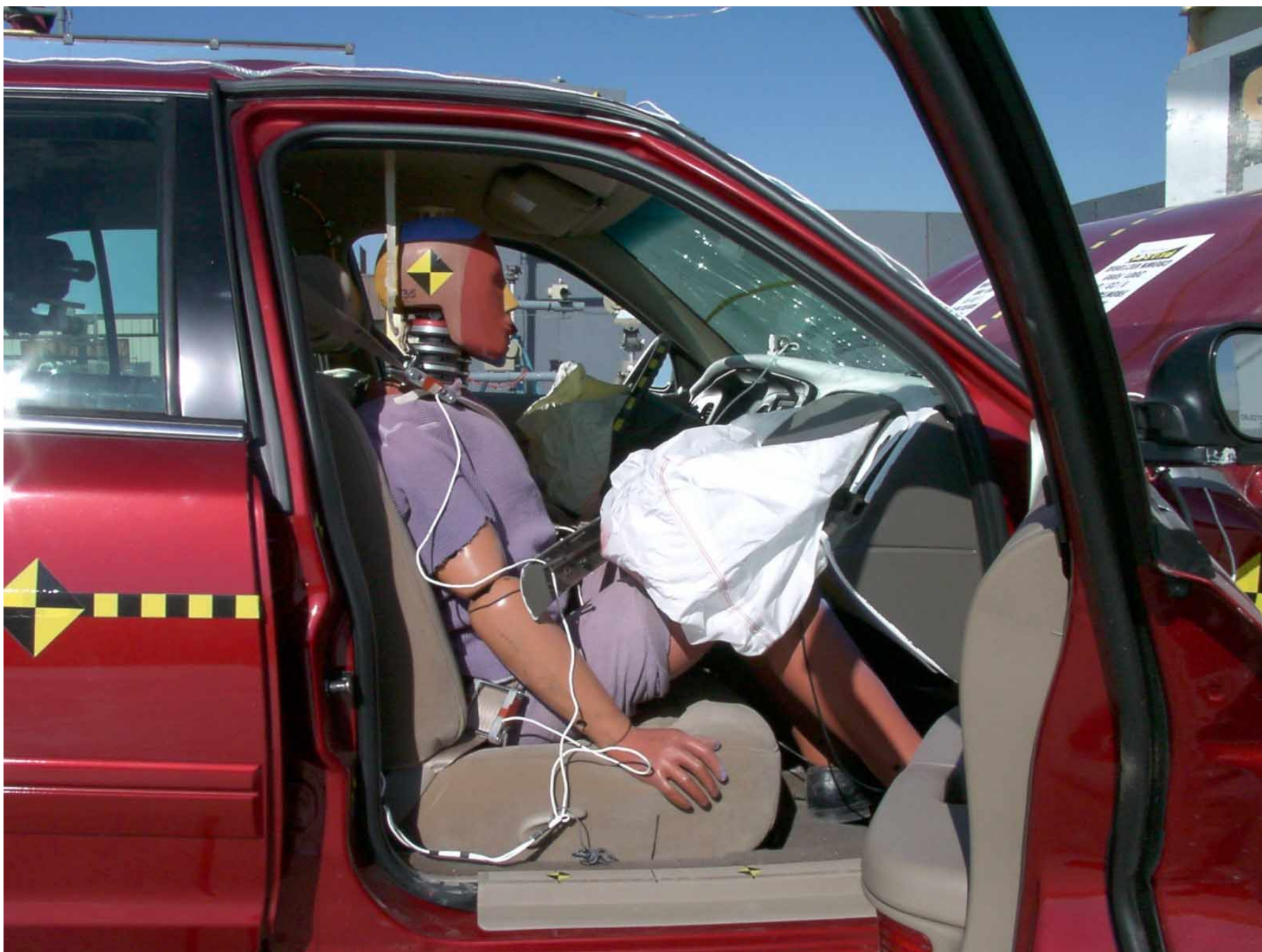
Figure A-48: Passenger Dummy 90° To Vehicle, Post-Test
