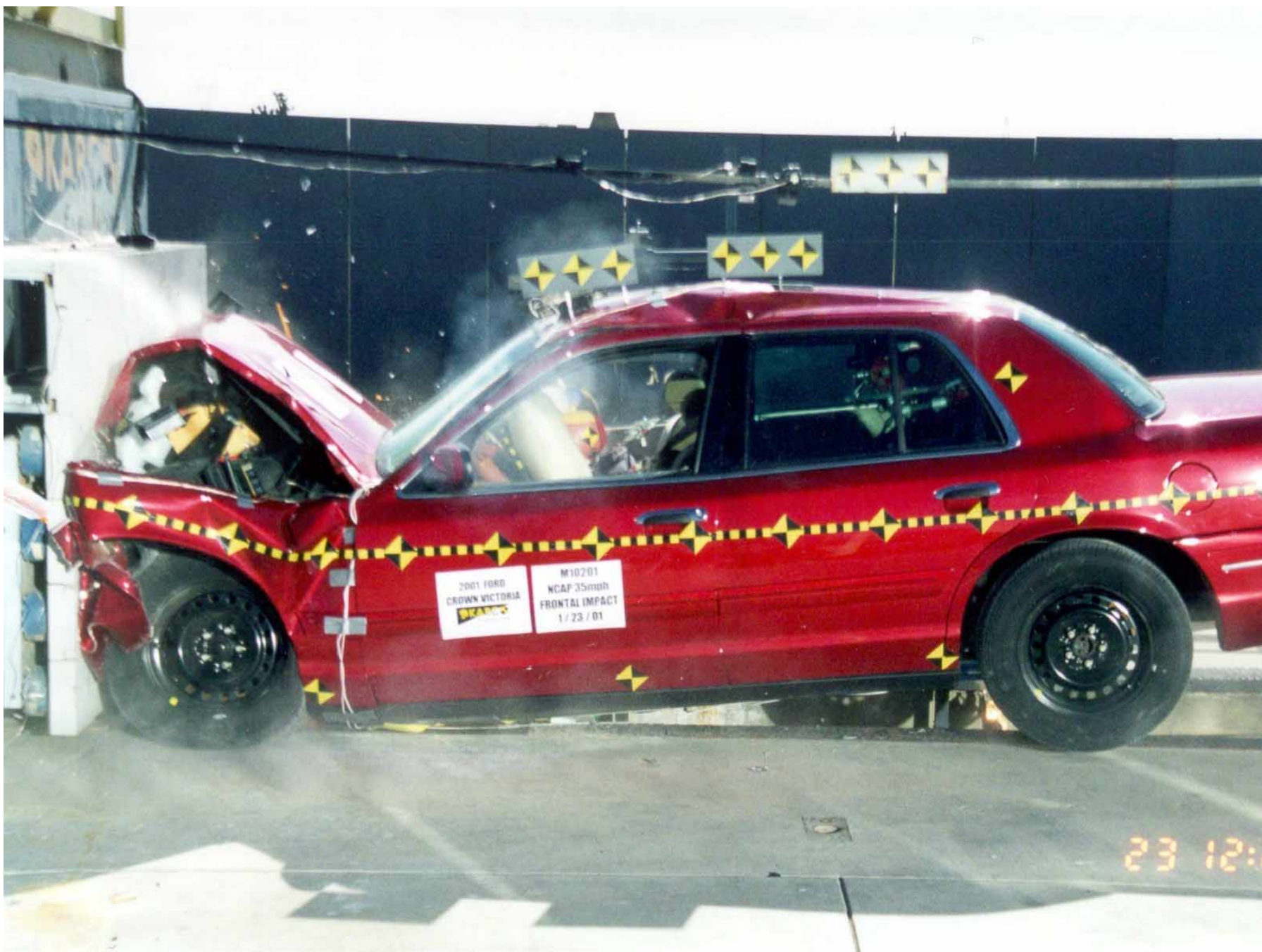
Figure A-58: Vehicle During Impact
