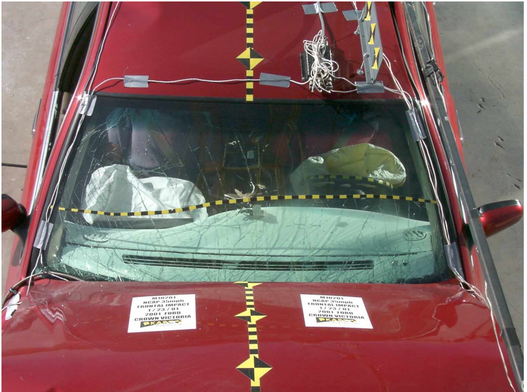
Figure A-16: Windshield, Post-Test
