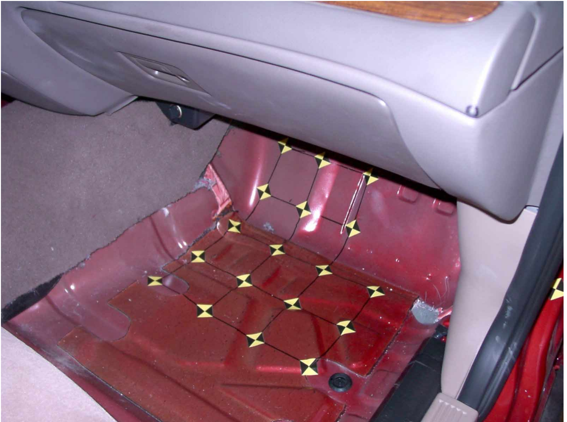
Figure A-51: Passenger Side Floor Pan, Pre-Test
