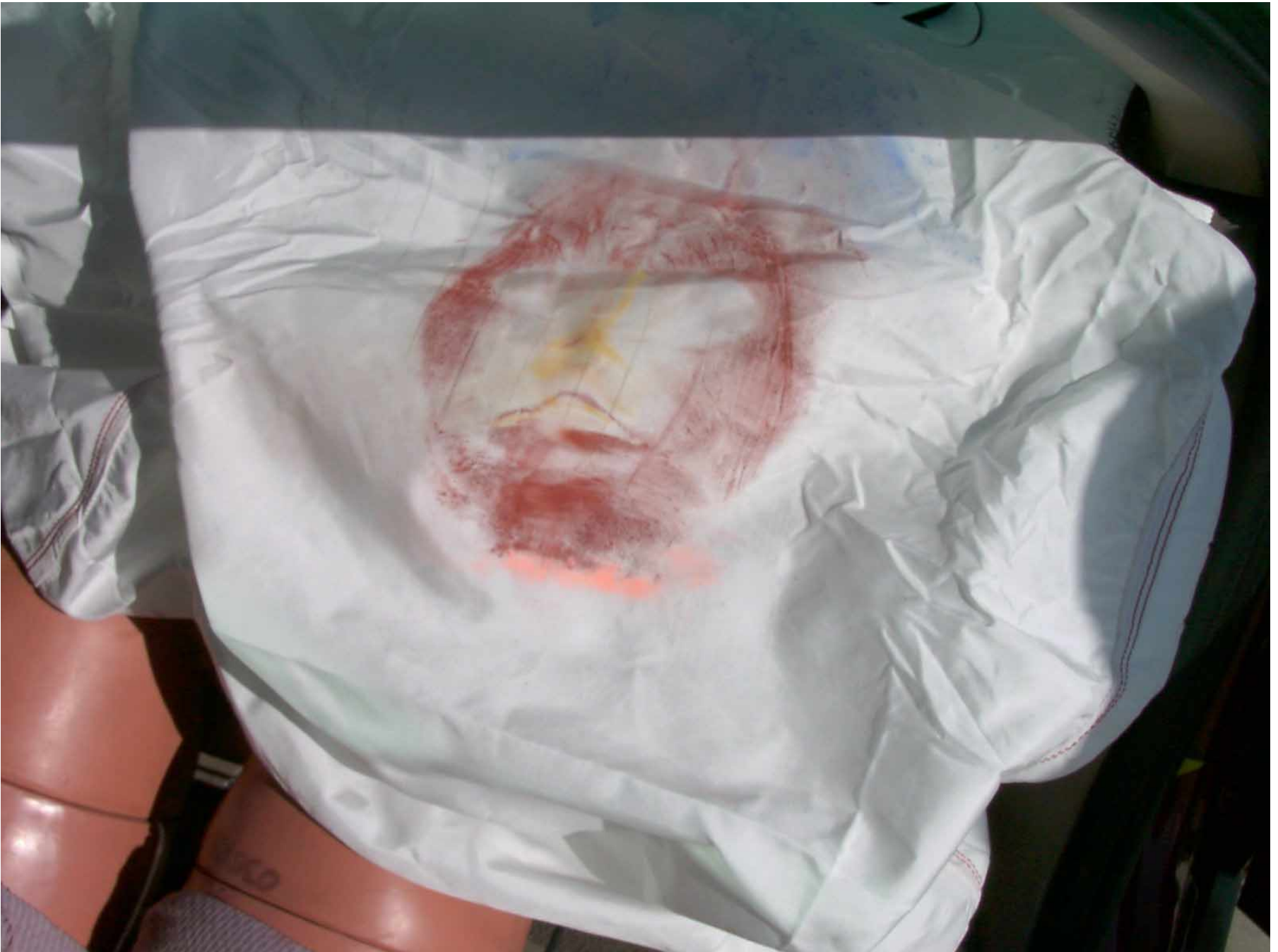
Figure A-56: Passenger Dummy Contact, Post-Test
