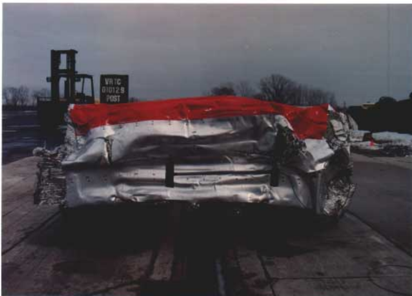
Figure A-33 Post-Test Moving Deformable Barrier Front View
