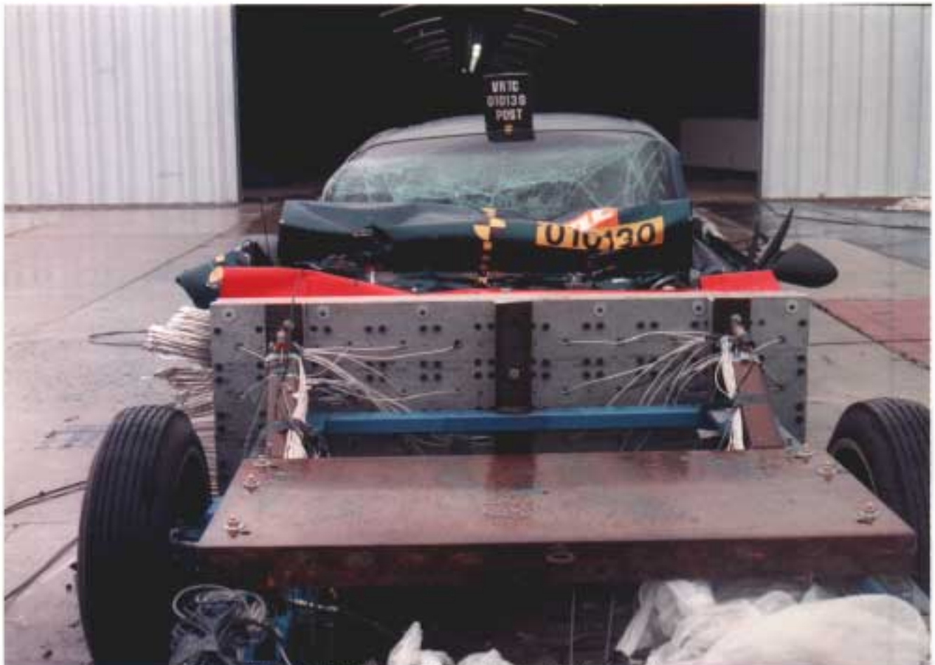
Figure A-4 Post-Test Target Vehicle Front with Barrier View
