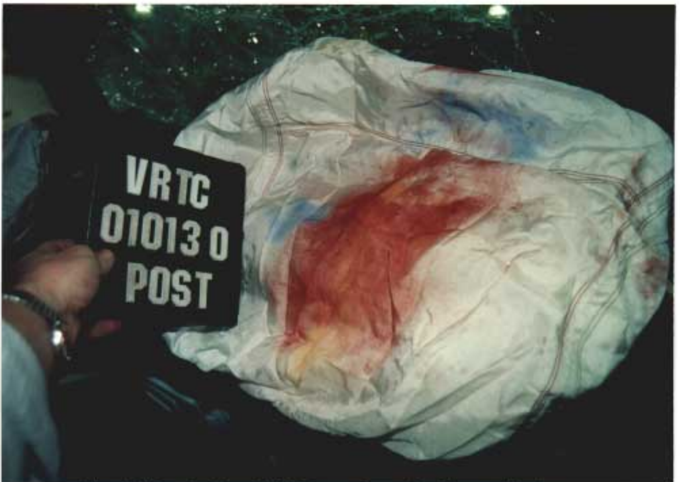
Figure A-55 Post-Test Target Vehicle Passenger Dummy Head Contact - View 1
