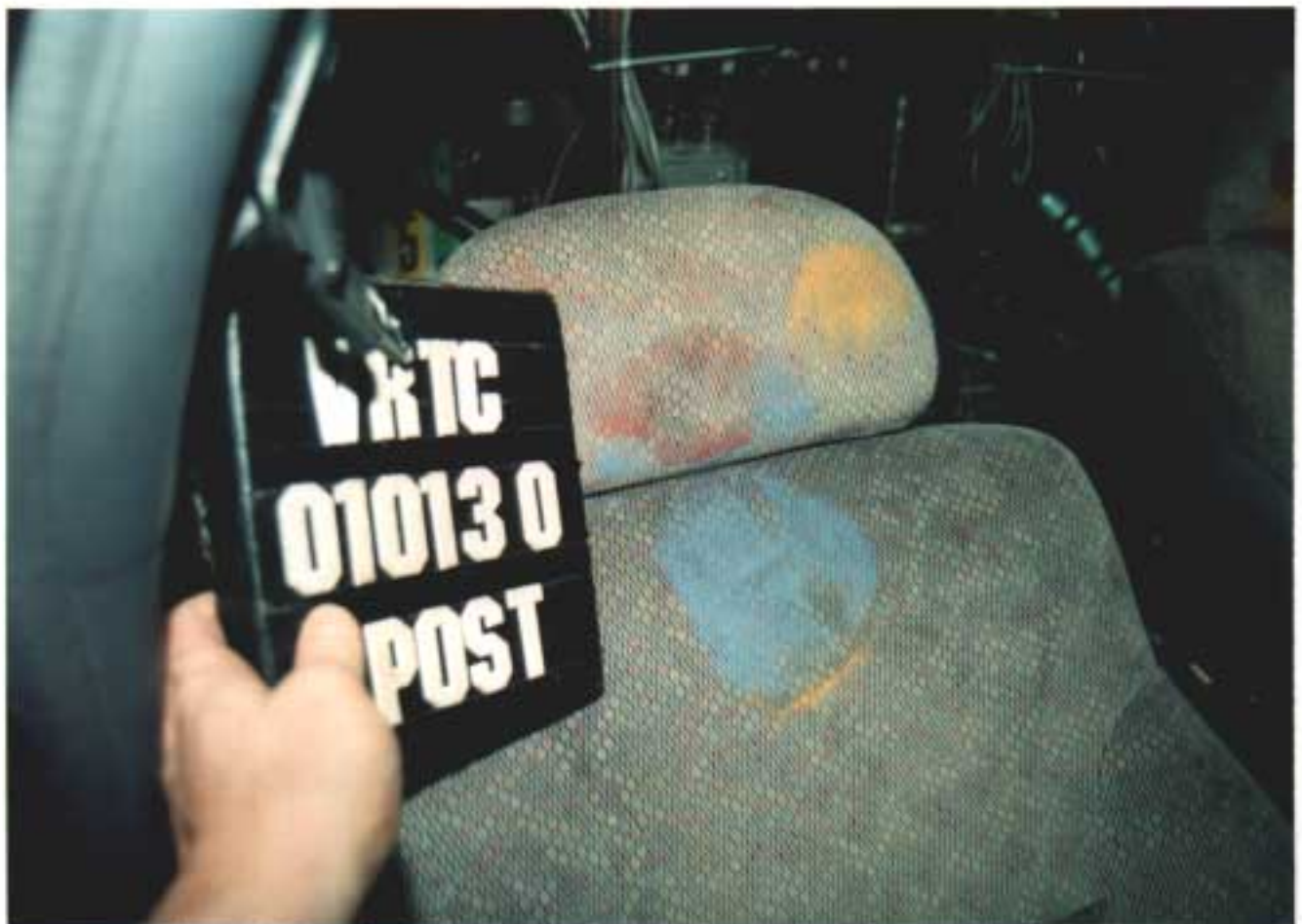
Figure A-57 Post-Test Target Vehicle Passenger Dummy Head Contact - View 3
