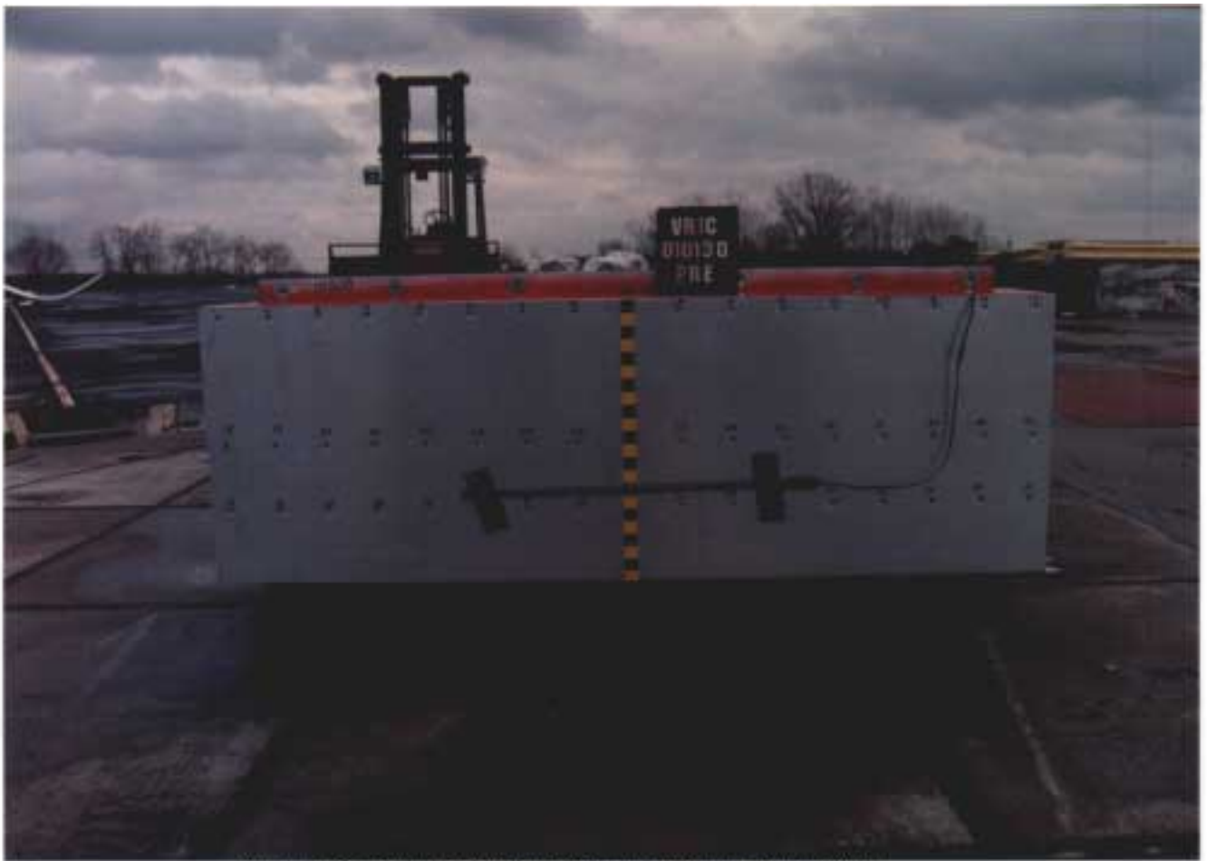
Figure A-31 Pre-Test Moving Deformable Barrier Front View
