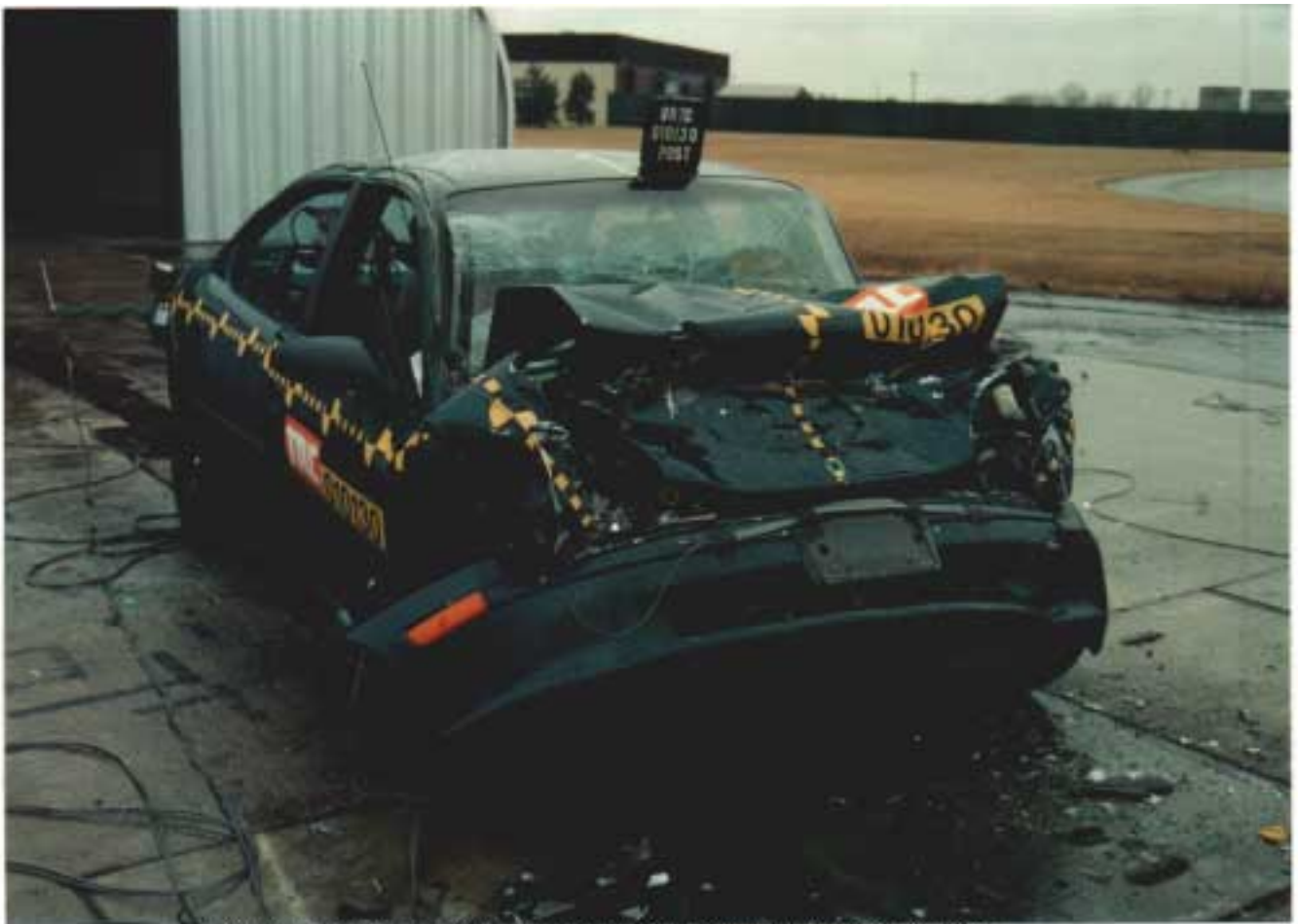
Figure A-21 Post-Test Target Vehicle Right Front Three-Quarter View
