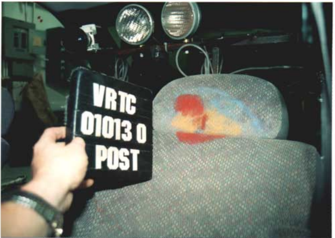
Figure A-45 Post-Test Target Vehicle Driver Dummy Head Contact - View 2
