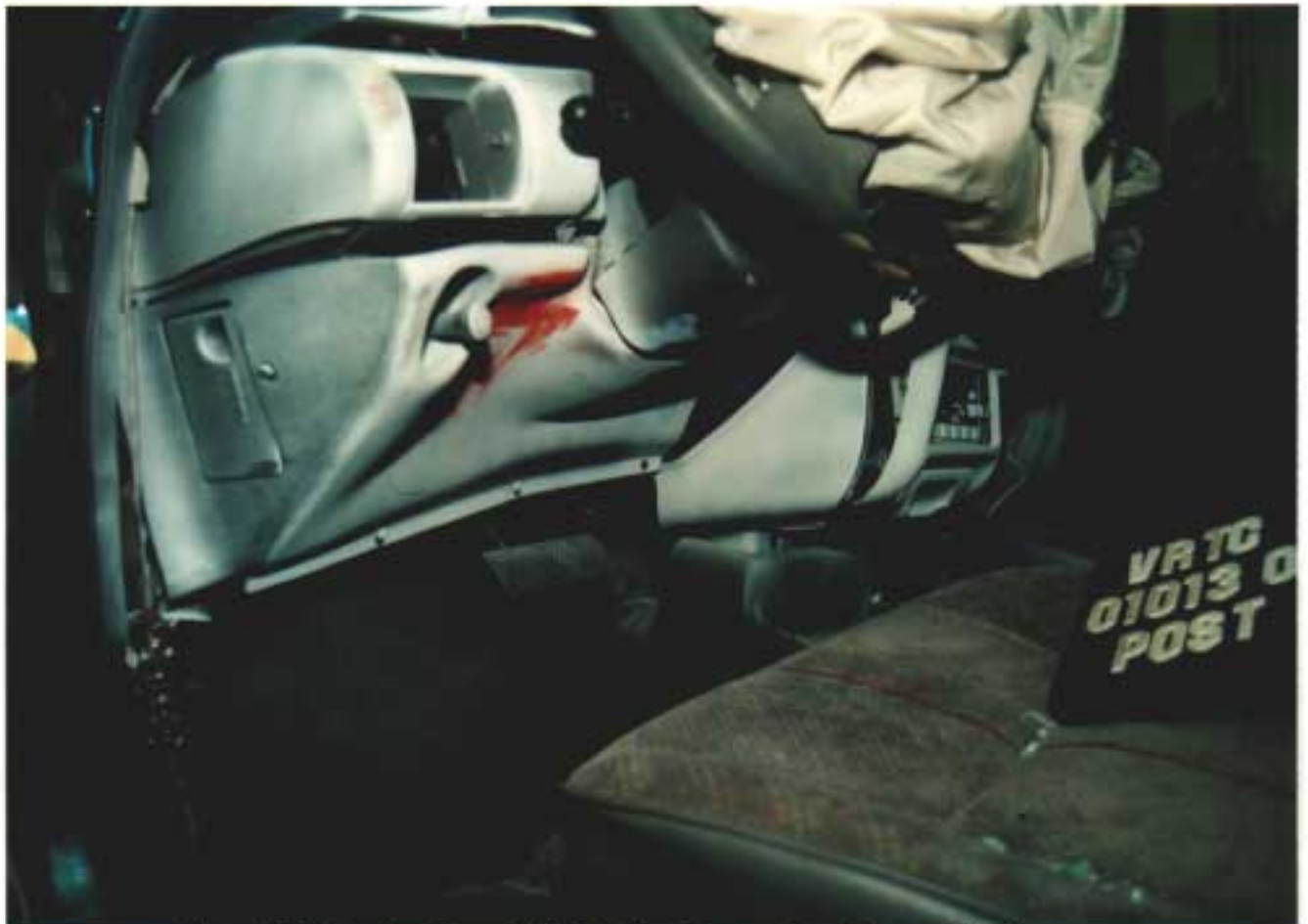
Figure A-46 Post-Test Target Vehicle Driver Dummy Knee Contact - View 1
