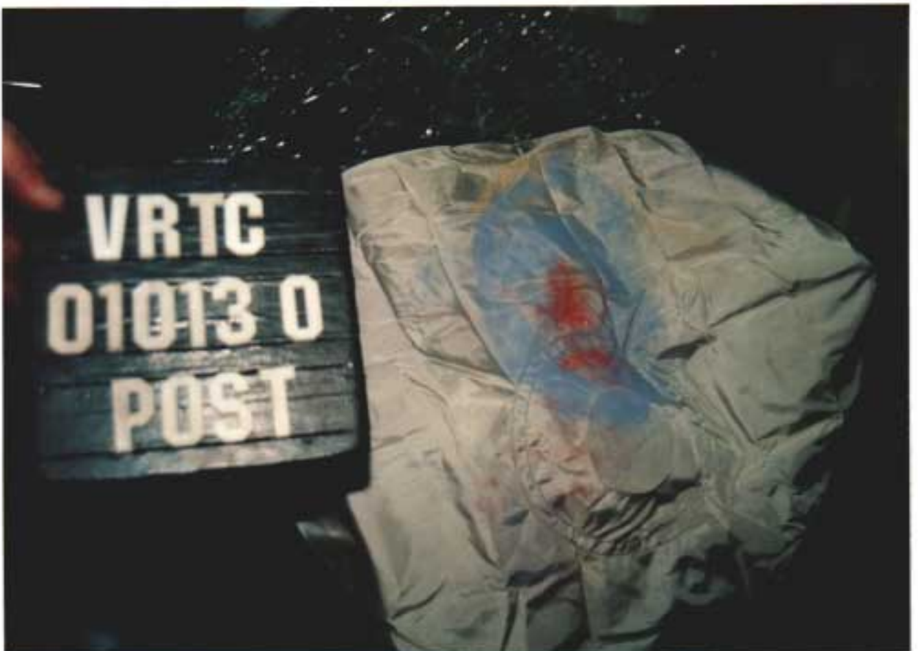
Figure A-44 Post-Test Target Vehicle Driver Dummy Head Contact - View 1
