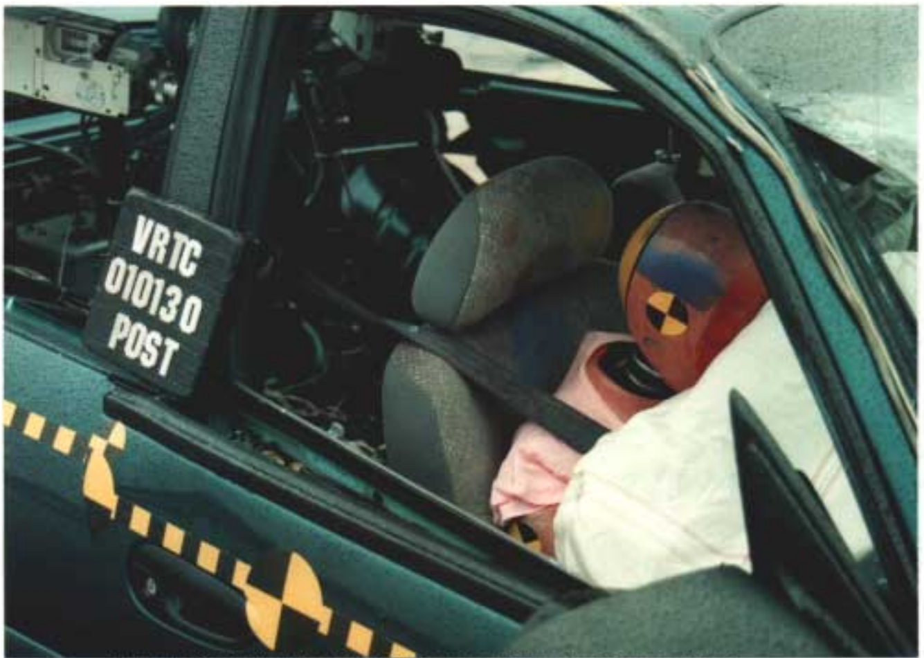
Figure A-56 Post-Test Target Vehicle Passenger Dummy Head Contact - View 2
