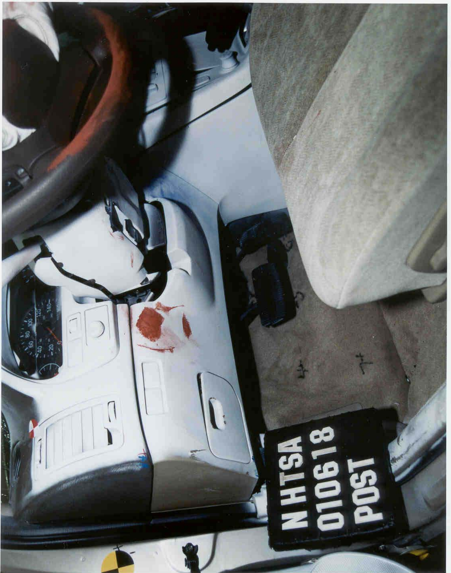
Figure 3-49 Post-Test Driver Dummy Knee Contact - View 2
