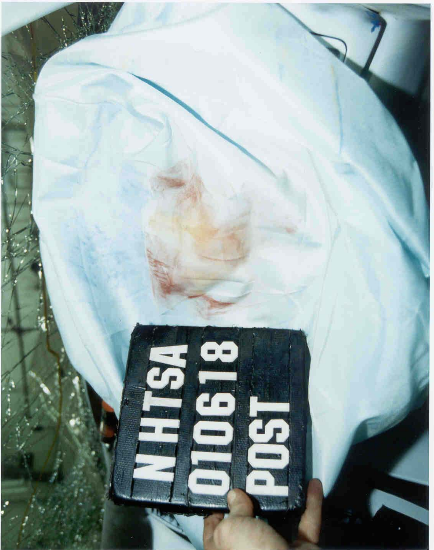
Figure 3-52 Post-Test Passenger Dummy Head Contact - View 2
