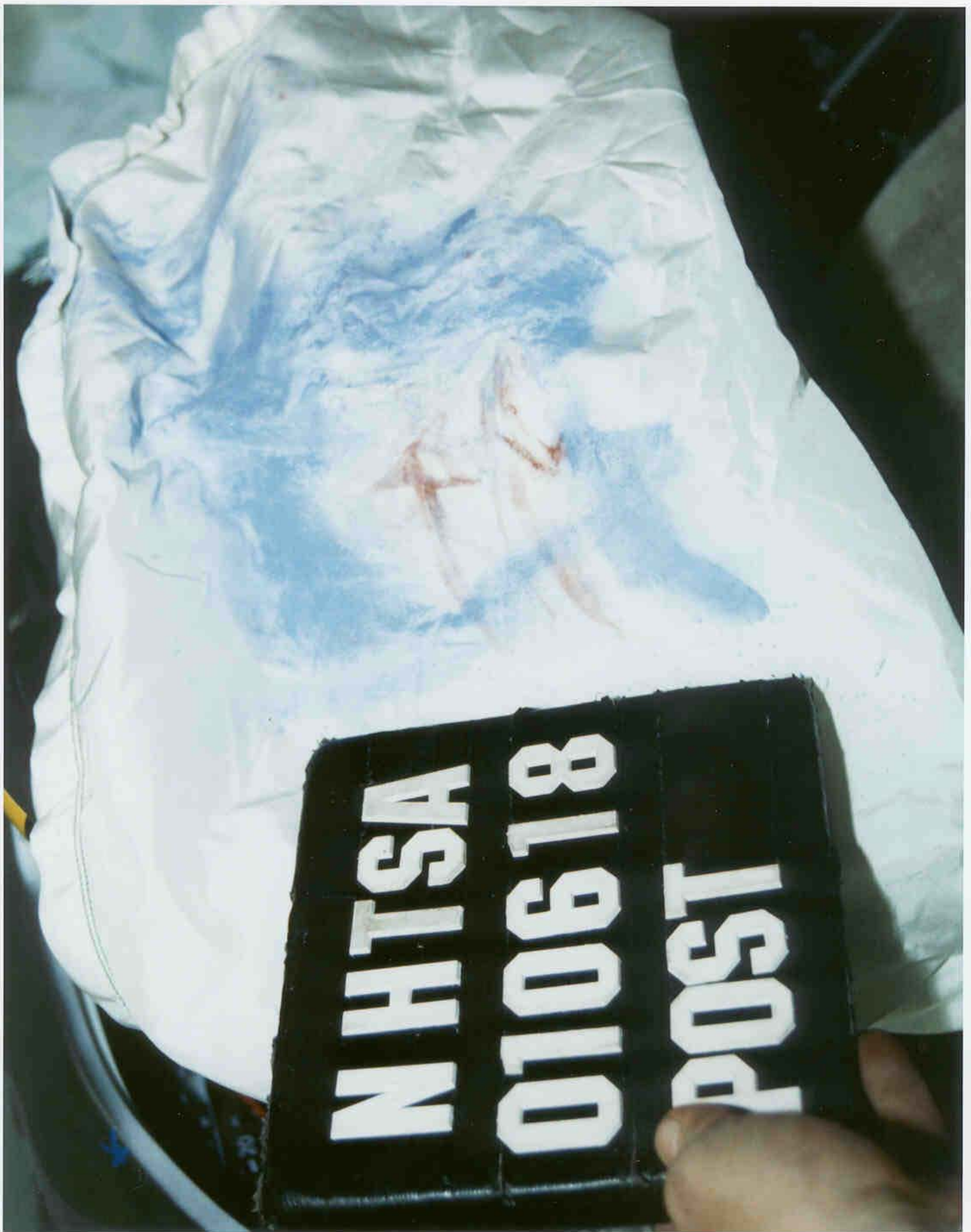
Figure 3-46 Post-Test Driver Dummy Head Contact - View 2
