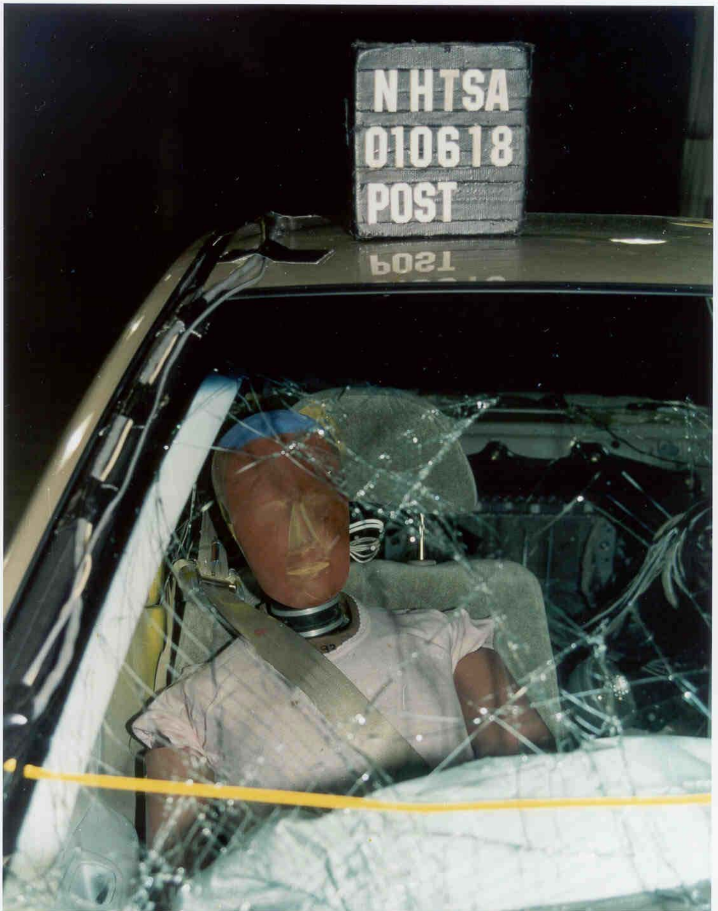
Figure 3-33 Post-Test Passenger Dummy Position - View 1
