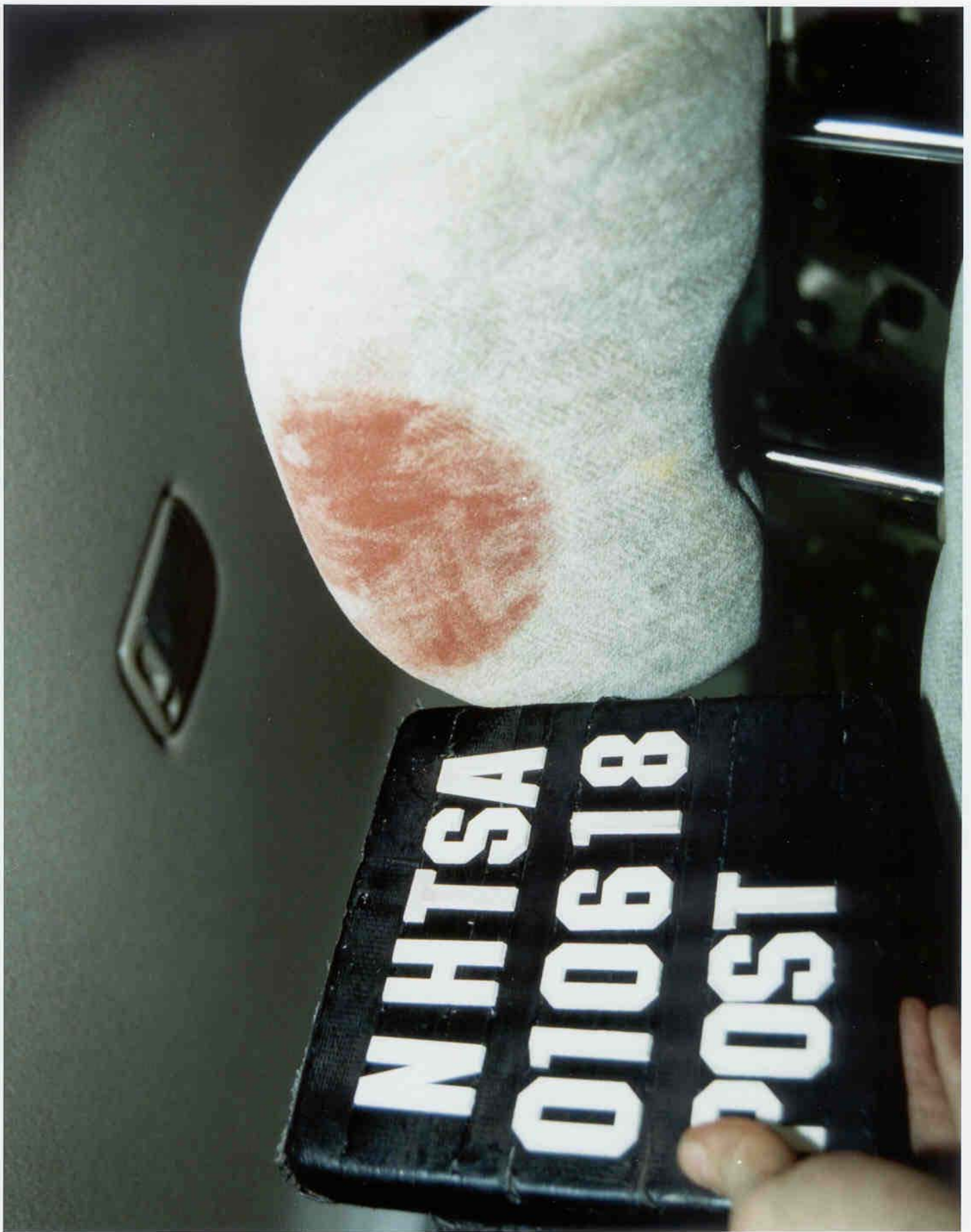
Figure 3-47 Post-Test Driver Dummy Head Contact - View 3 3-48
