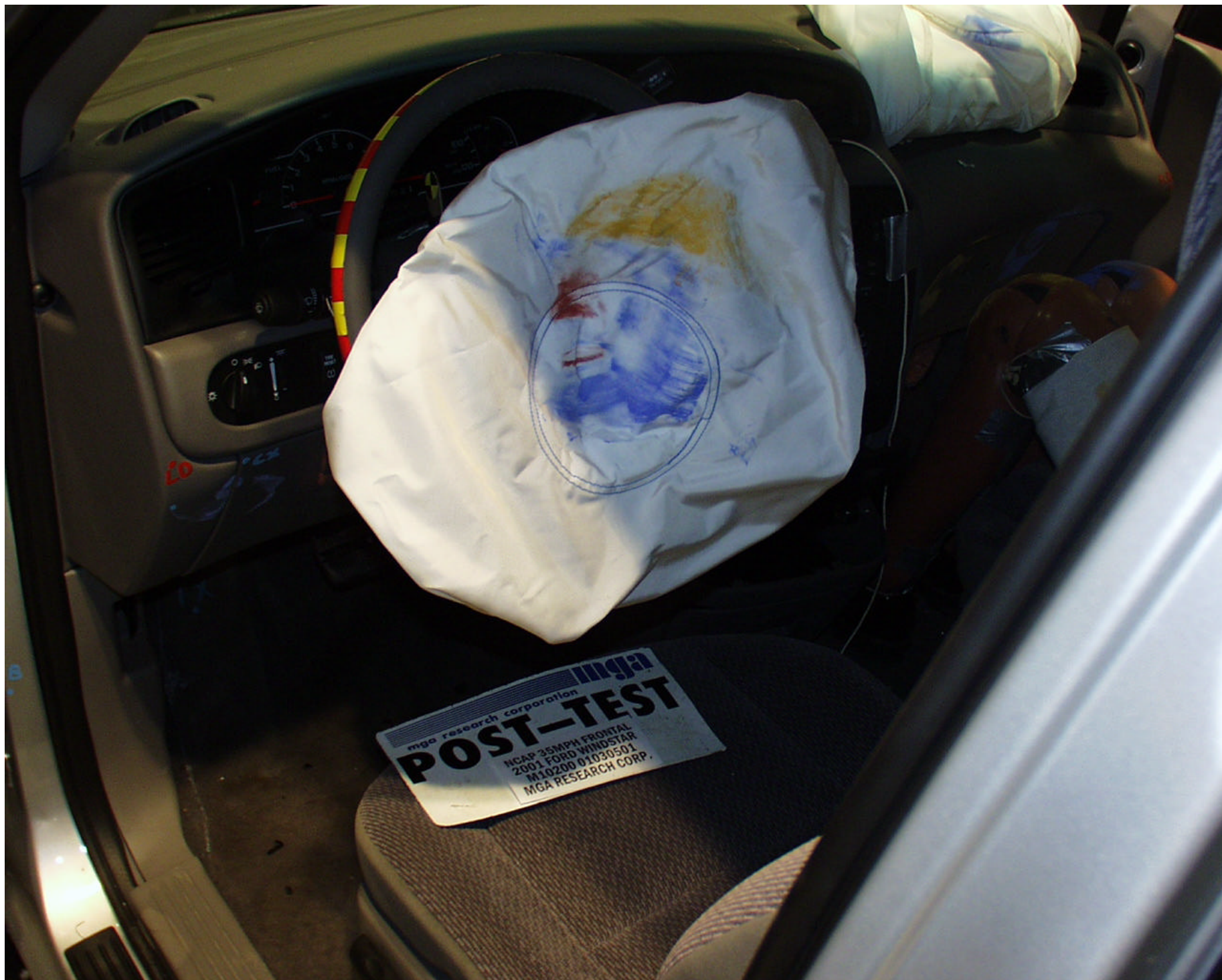
Photo No. A-29 - Post-Test Driver Airbag Contact
