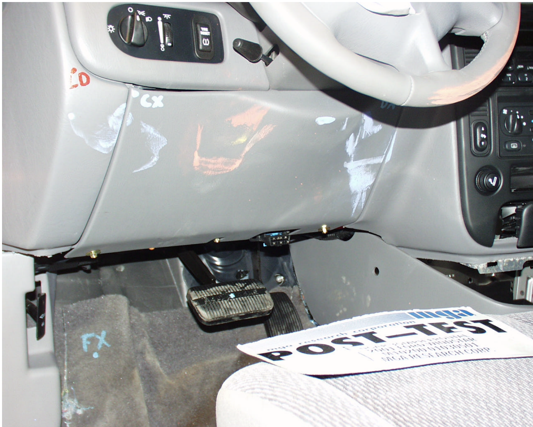
Photo No. A-30 - Post-Test Driver Knee Contact View
