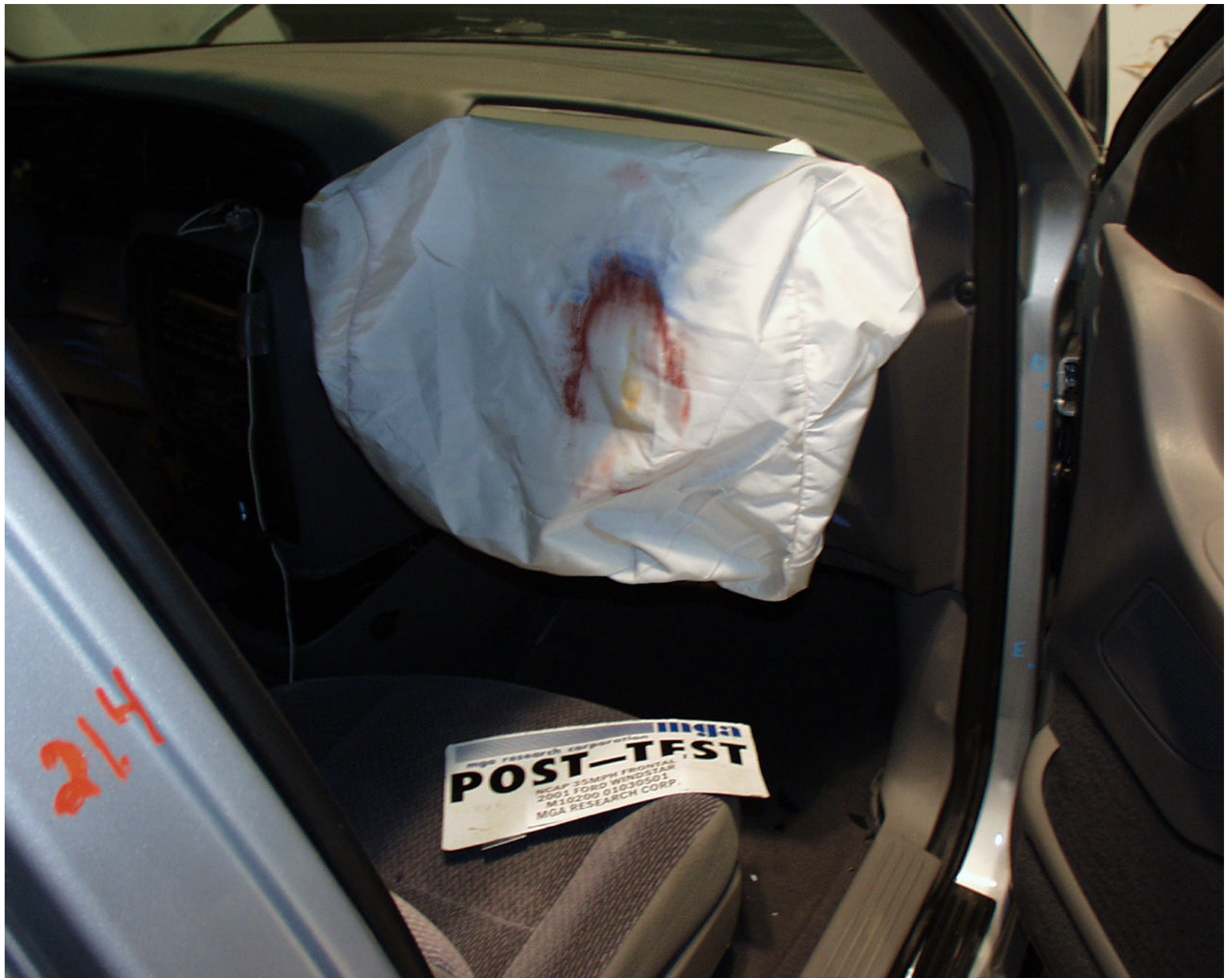
Photo No. A-41 - Post-Test Passenger Airbag Contact
