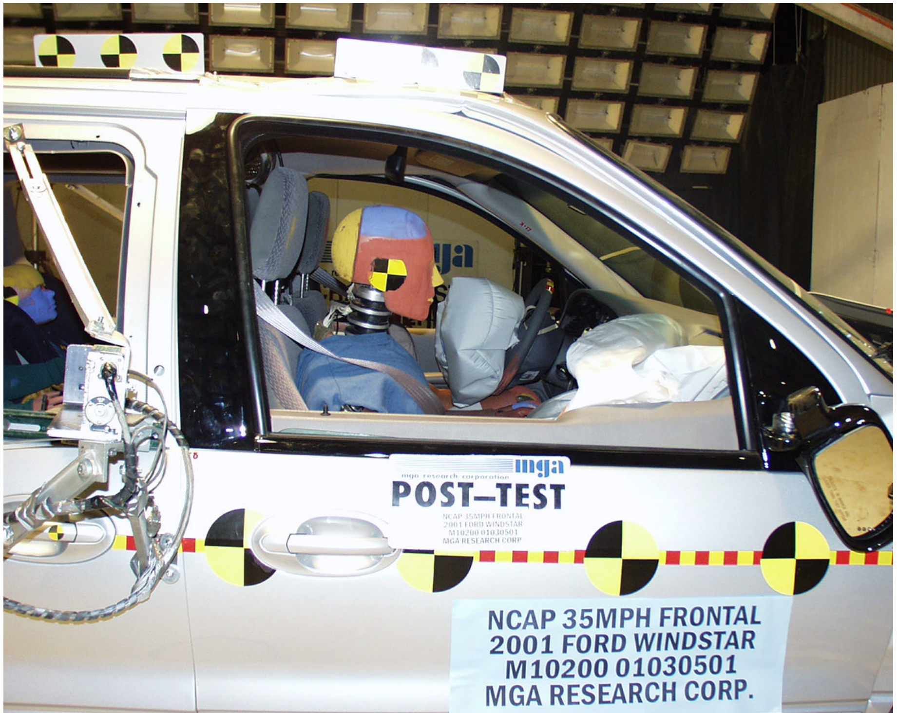
Photo No. A-34 - Post-Test Passenger Dummy Position Right Side View
