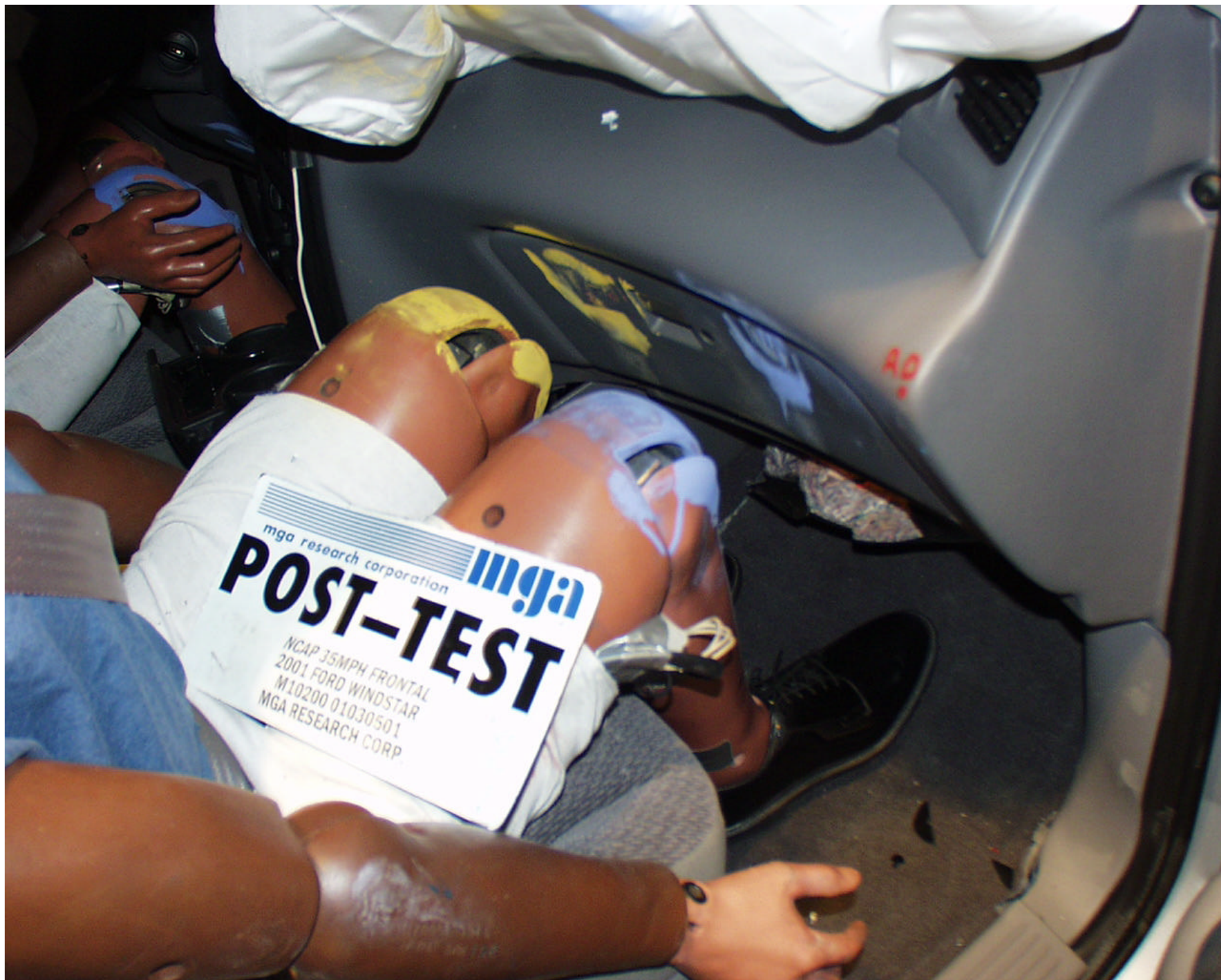
Photo No. A-40 - Post-Test Passenger Dummy Knee Position
