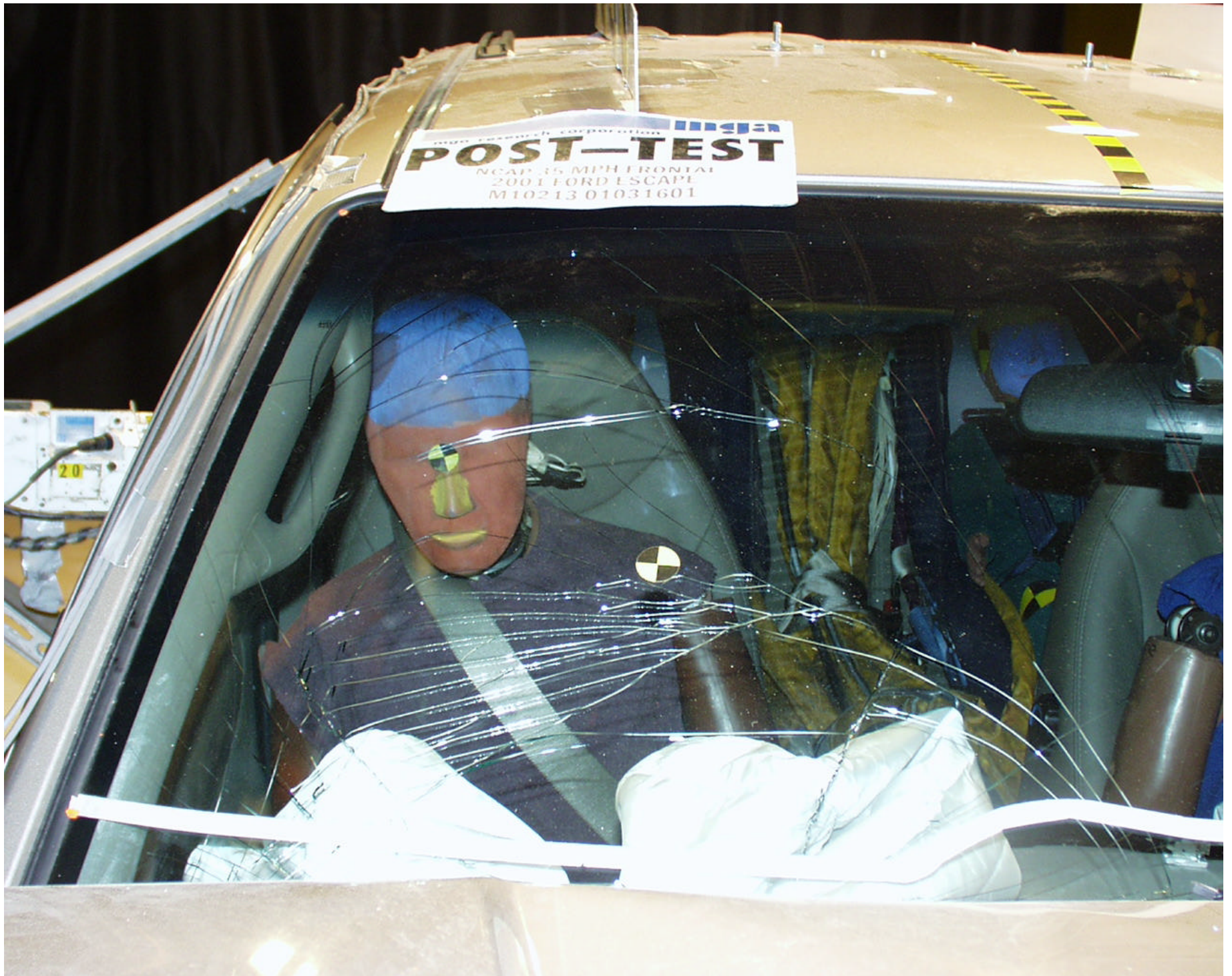
Photo No. A-45 - Post-Test Passenger Windshield View
