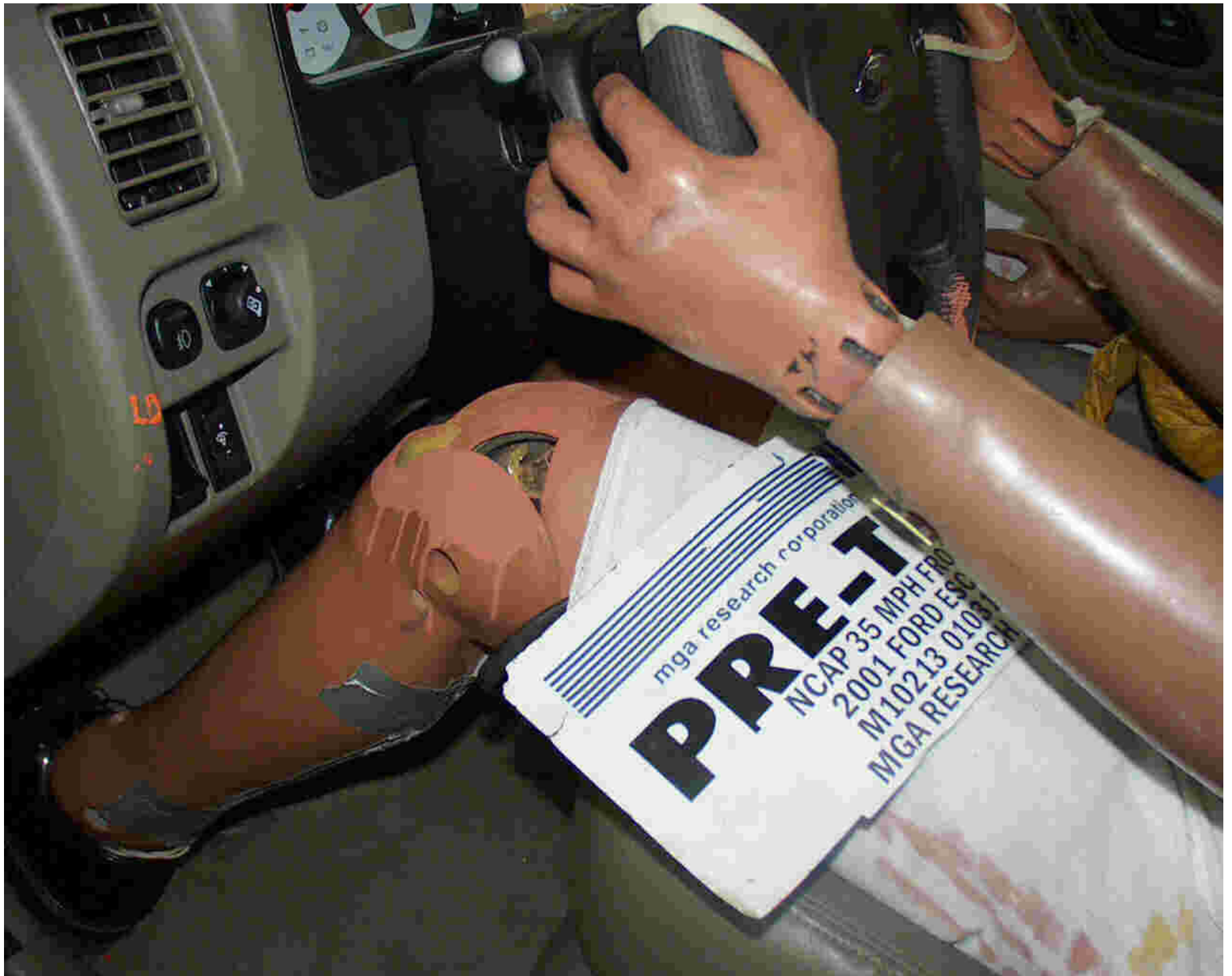
Photo No. A-28 - Pre-Test Driver Dummy Knee Position
