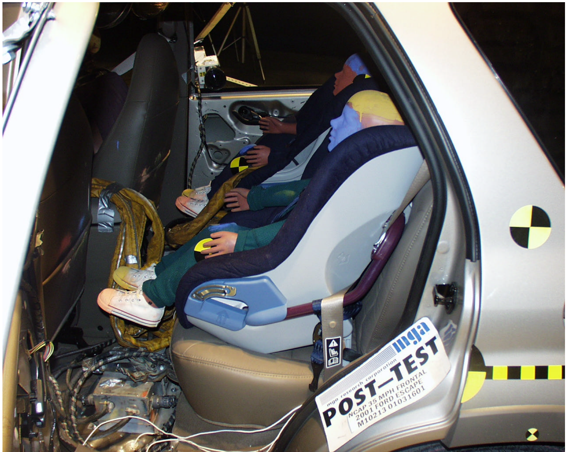
Photo 4 - Post-Test LRS 3 Year Old Left Side View (Door Open)
