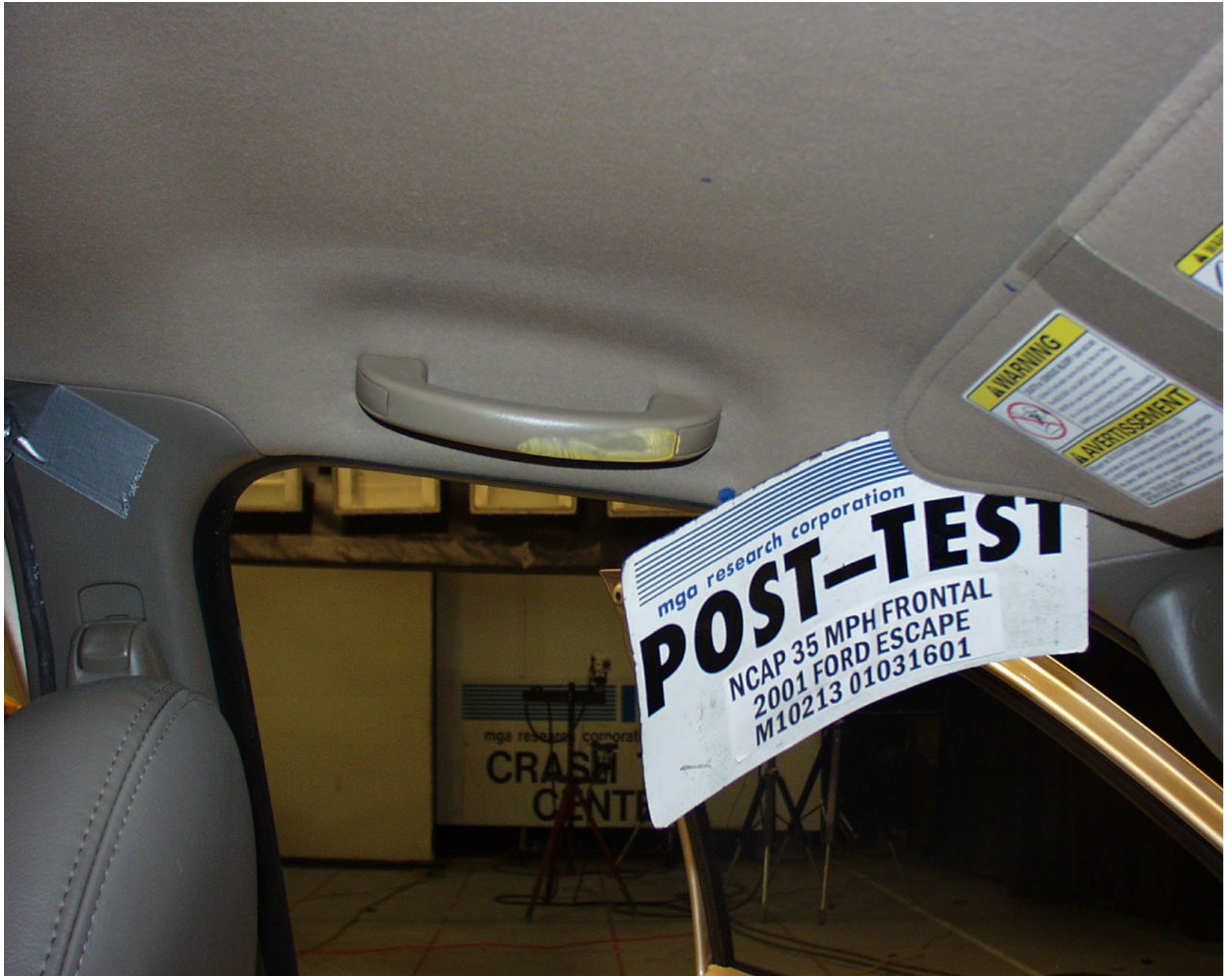
Photo No. A-32 - Post-Test Driver Head Contact View
