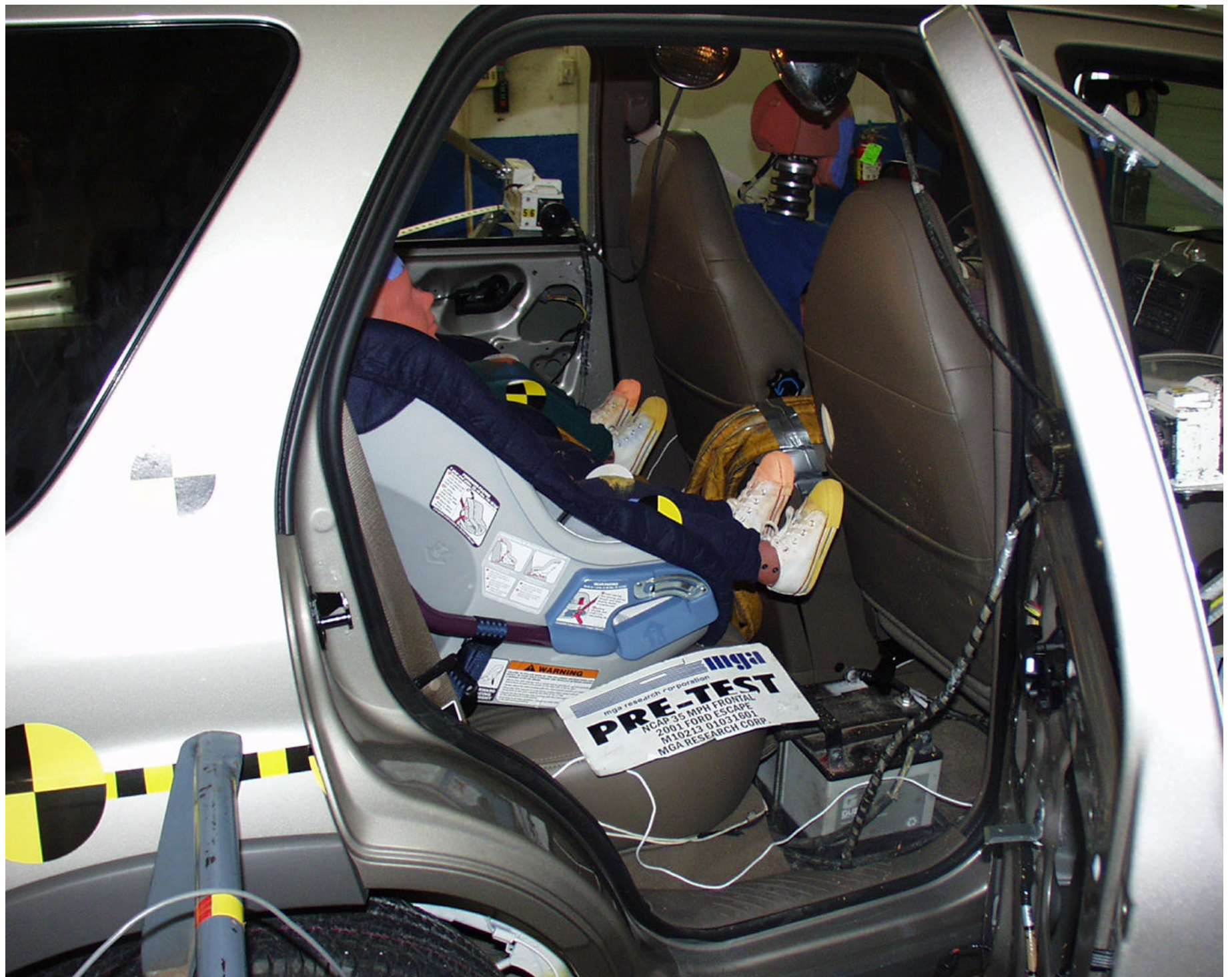
Photo 8 - Pre-Test RRS 3 Year Old Right Side View (Door Open)
